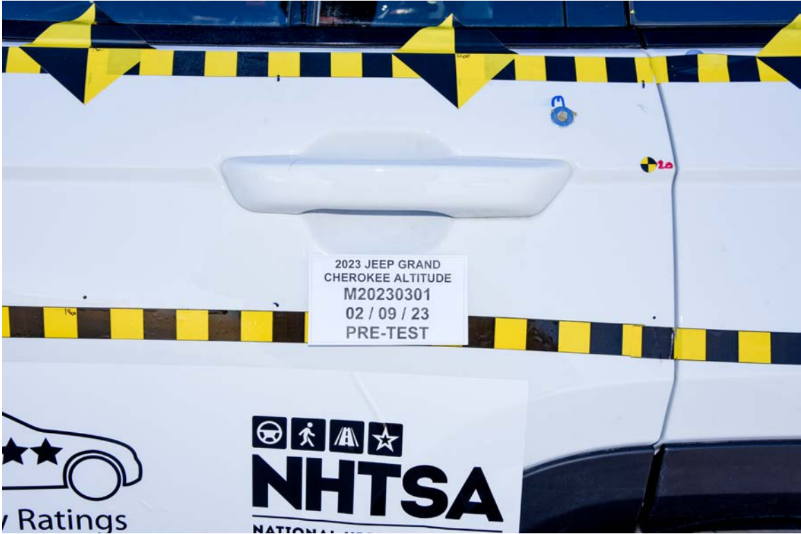
FIGURE 23. Pre-Test Left Rear Door Latch Close-Up
