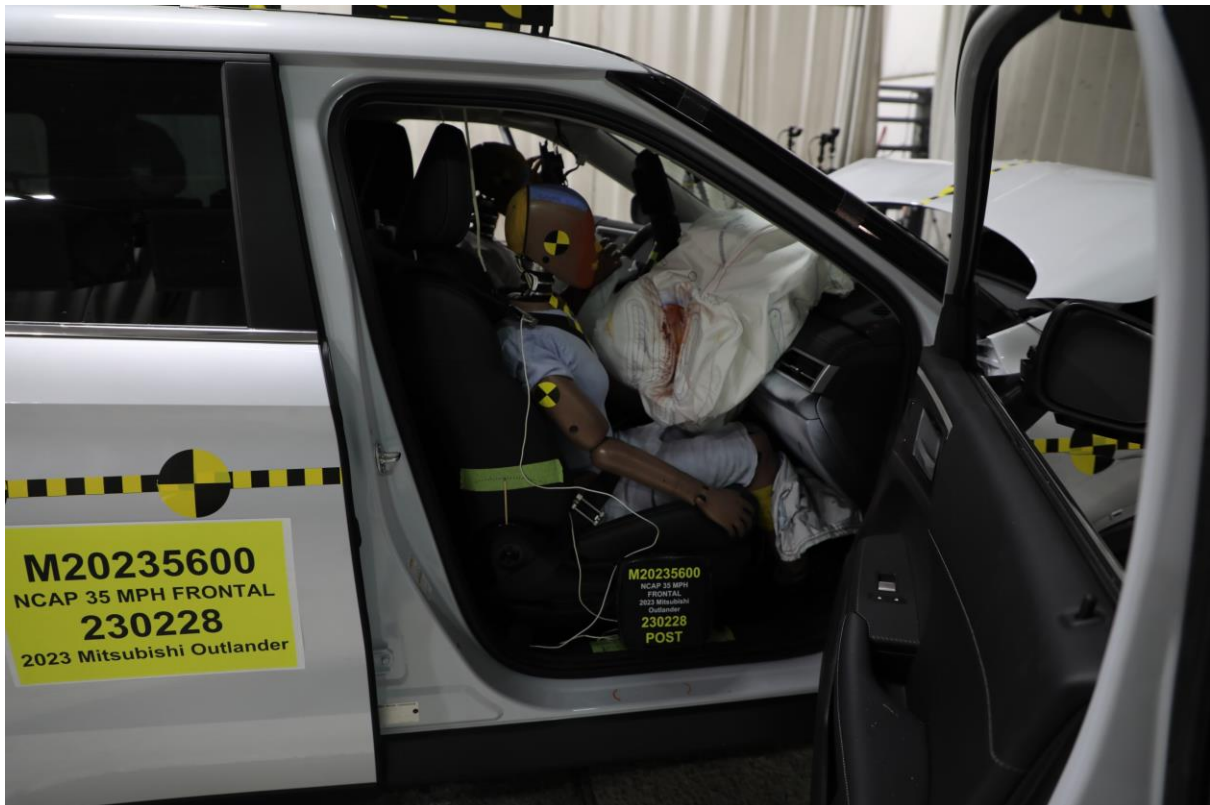
058 Post-Test Passenger Dummy and Vehicle Interior View
