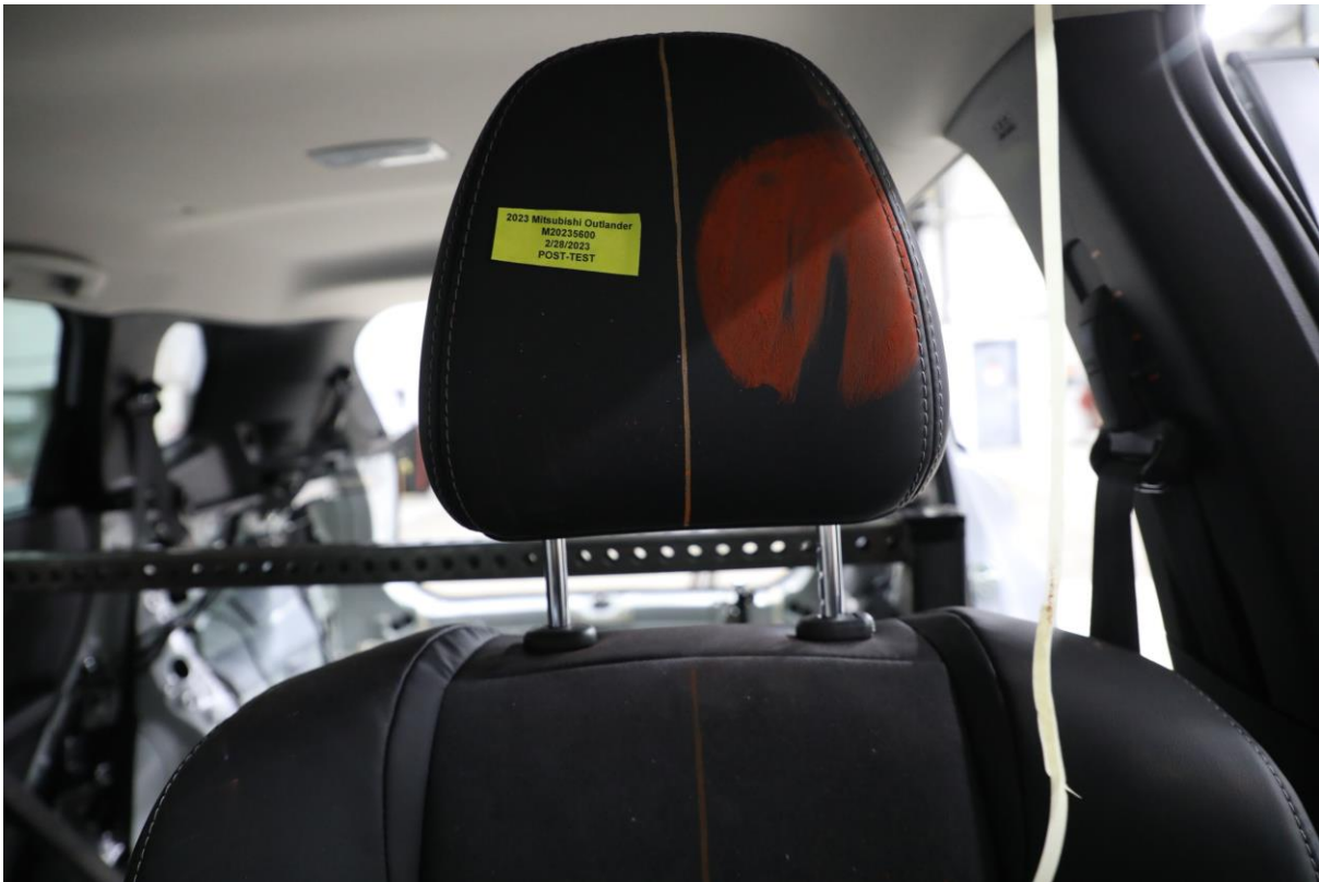
050 Post-Test Driver Dummy Contact with Headrest
