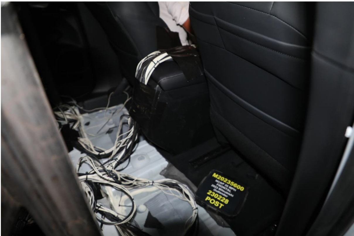
029 Post-Test Dummy Cable Routing
