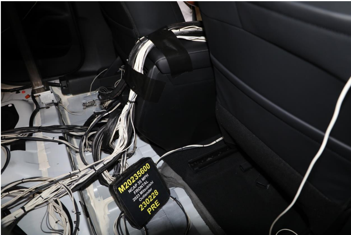
028 Pre-Test Dummy Cable Routing
