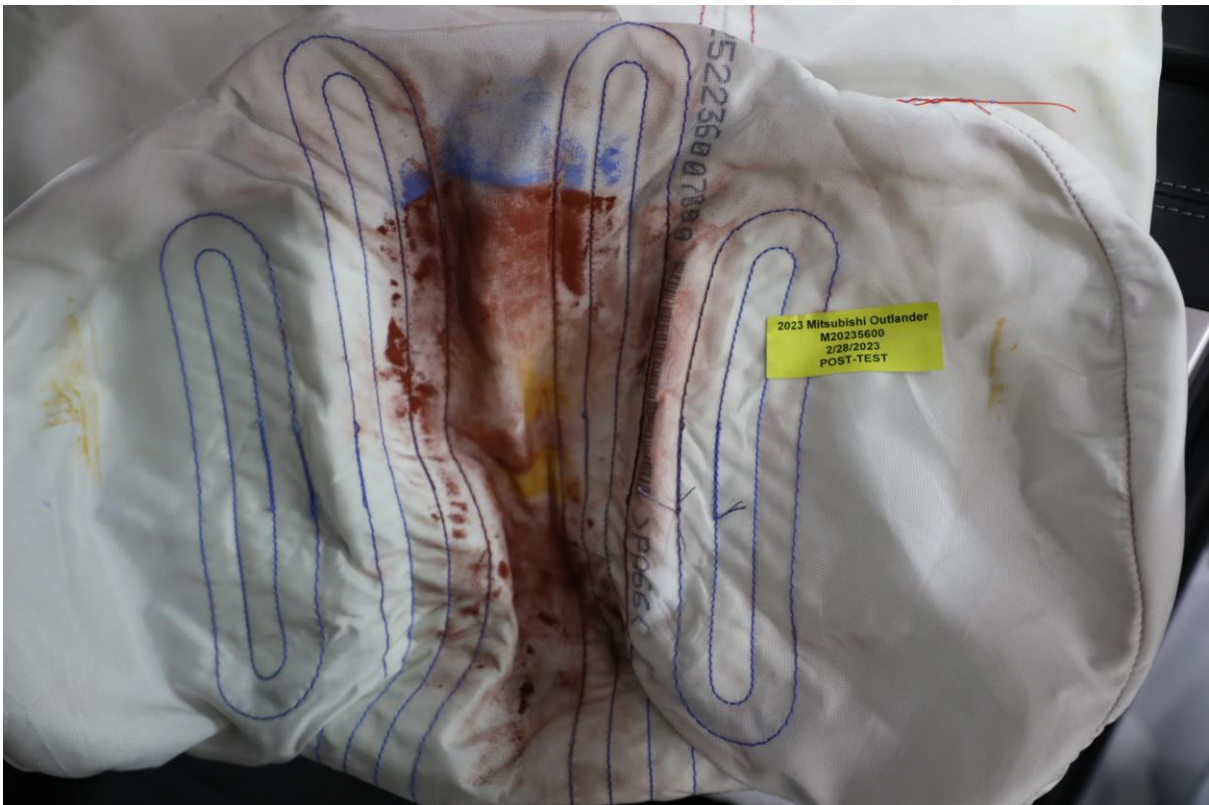
072 Post-Test Passenger Dummy Contact with Airbag
