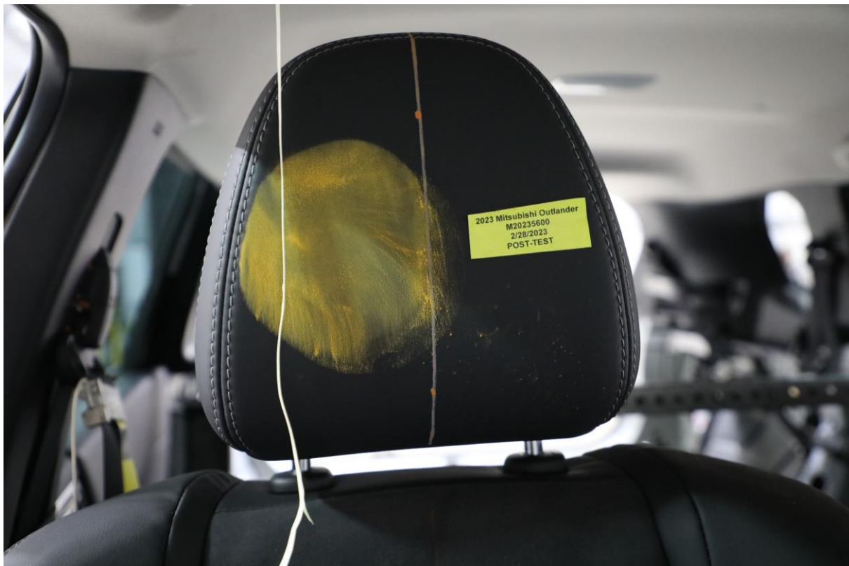
073 Post-Test Passenger Dummy Contact with Headrest
