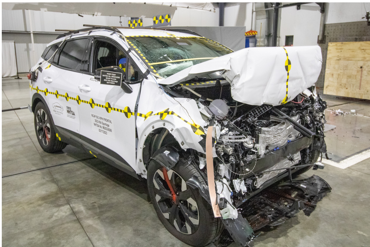
Figure A-15: Post-Test Right Front 3-4 View
