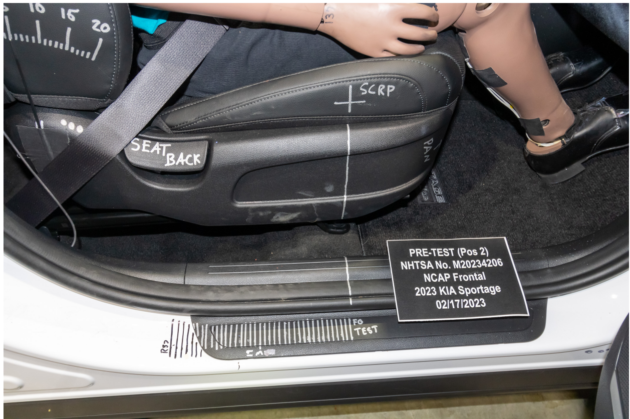
Figure A-59: Pre-Test Passenger's Seat Fore-Aft Markings
