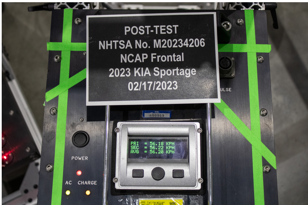
Figure A-76: Post-Test Speed Trap Read-Out
