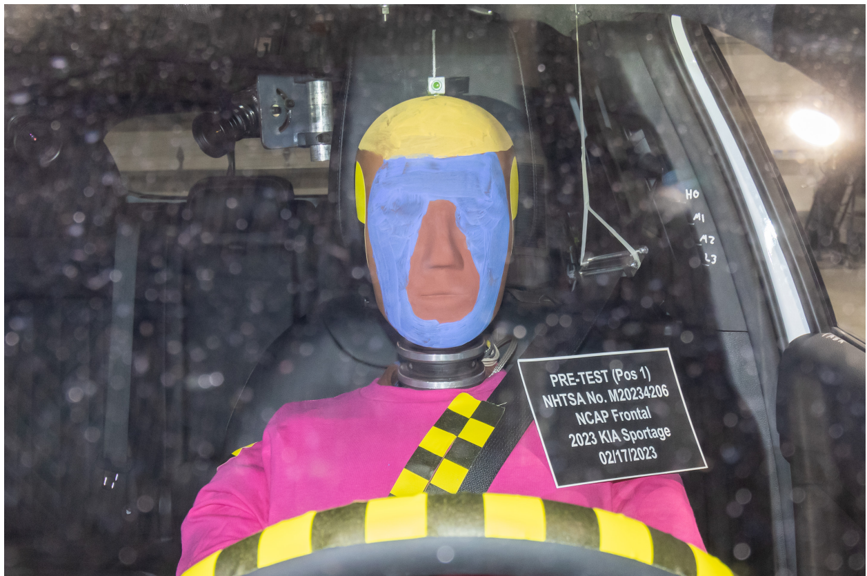
Figure A-30: Pre-Test Driver Dummy Front View
