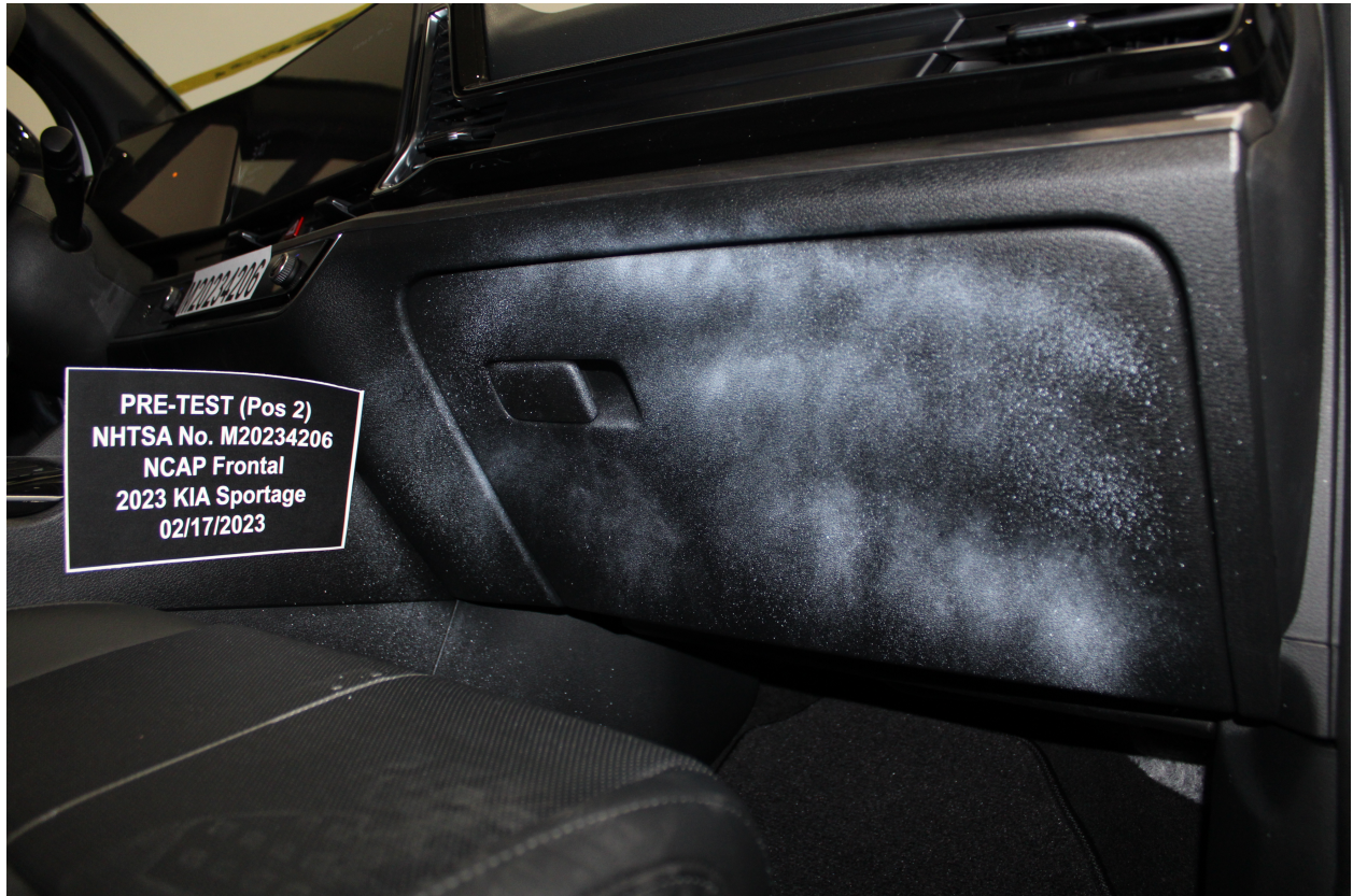
Figure A-67: Pre-Test Passenger's Side Knee Bolster
