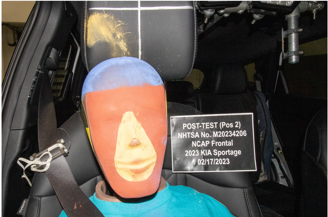
Figure A-71: Post-Test Passenger Dummy Face
