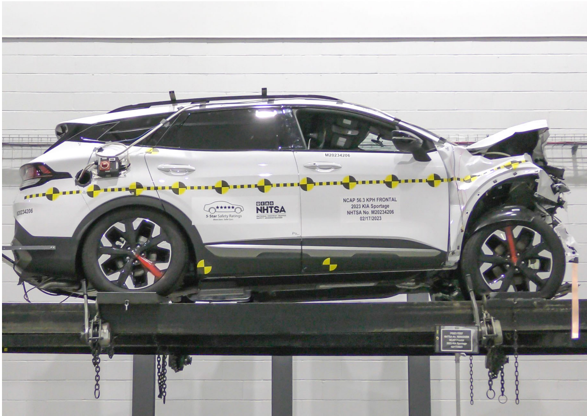
Figure A-81: Vehicle at 360° on Static Rollover Device
