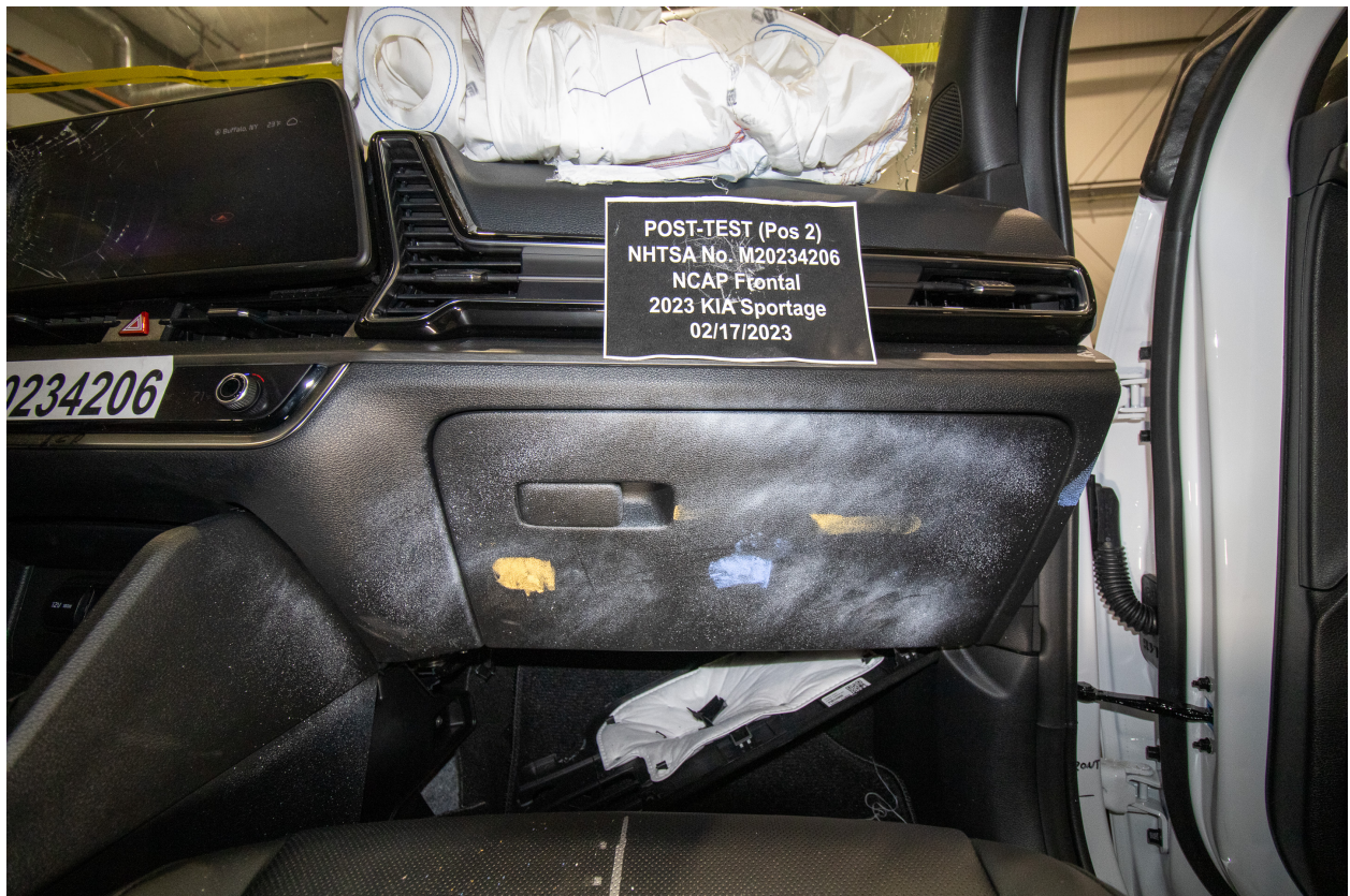
Figure A-68: Post-Test Passenger's Side Knee Bolster
