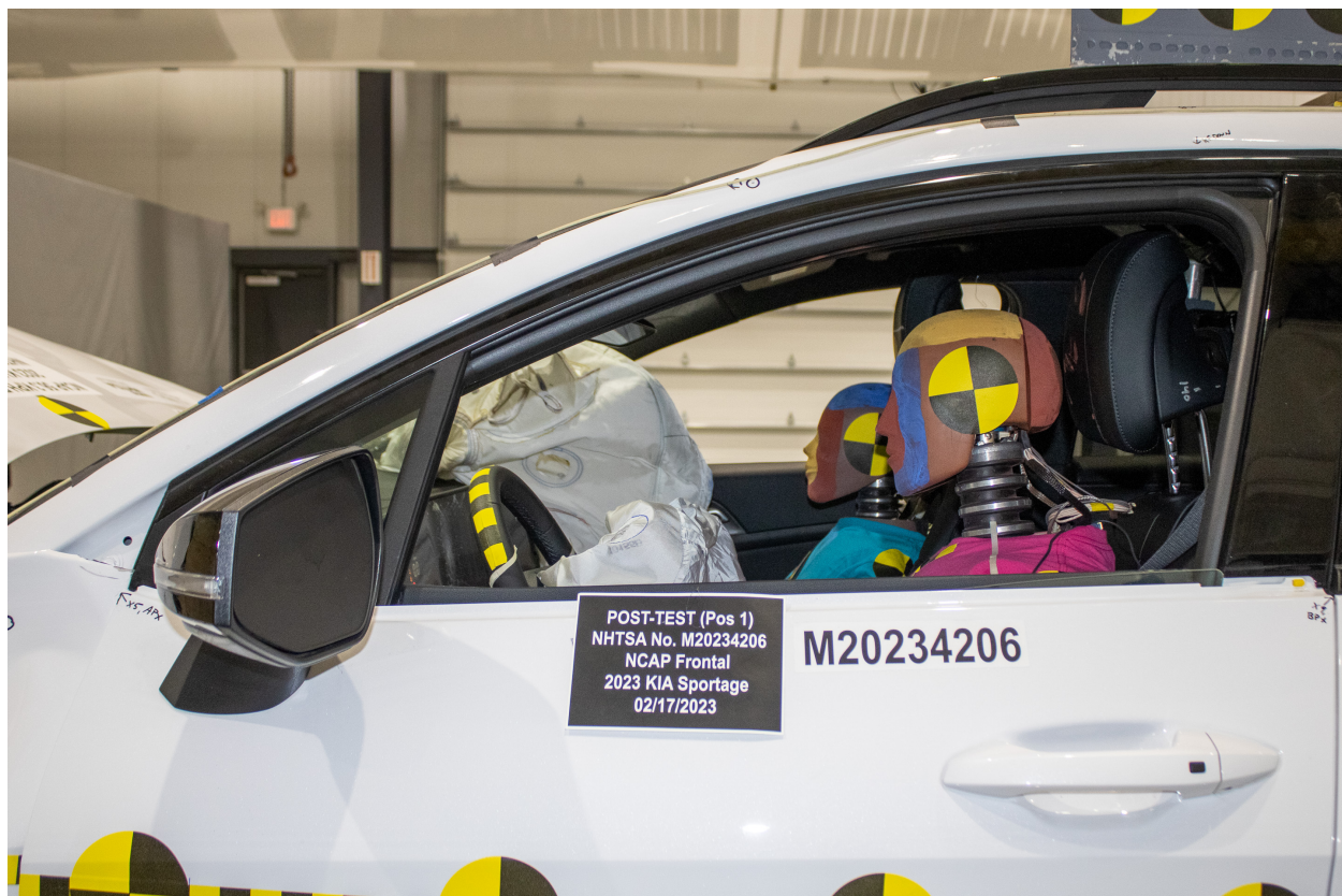
Figure A-33: Post-Test Driver Dummy Window View
