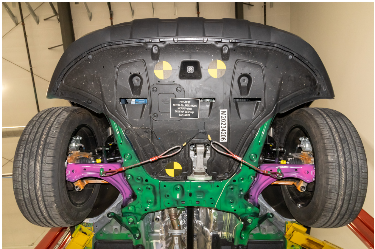
Figure A-24: Pre-Test Front Underbody View
