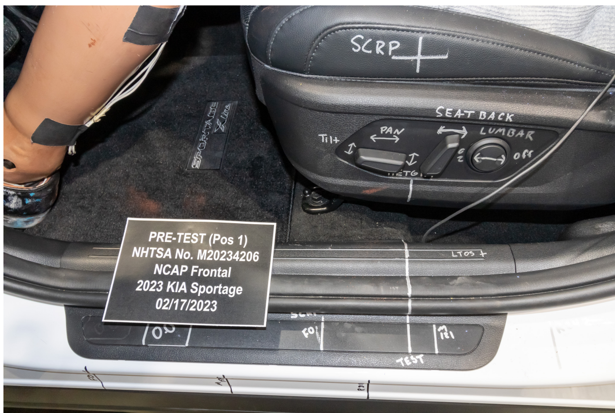
Figure A-36: Pre-Test Driver's Seat Fore-Aft Markings
