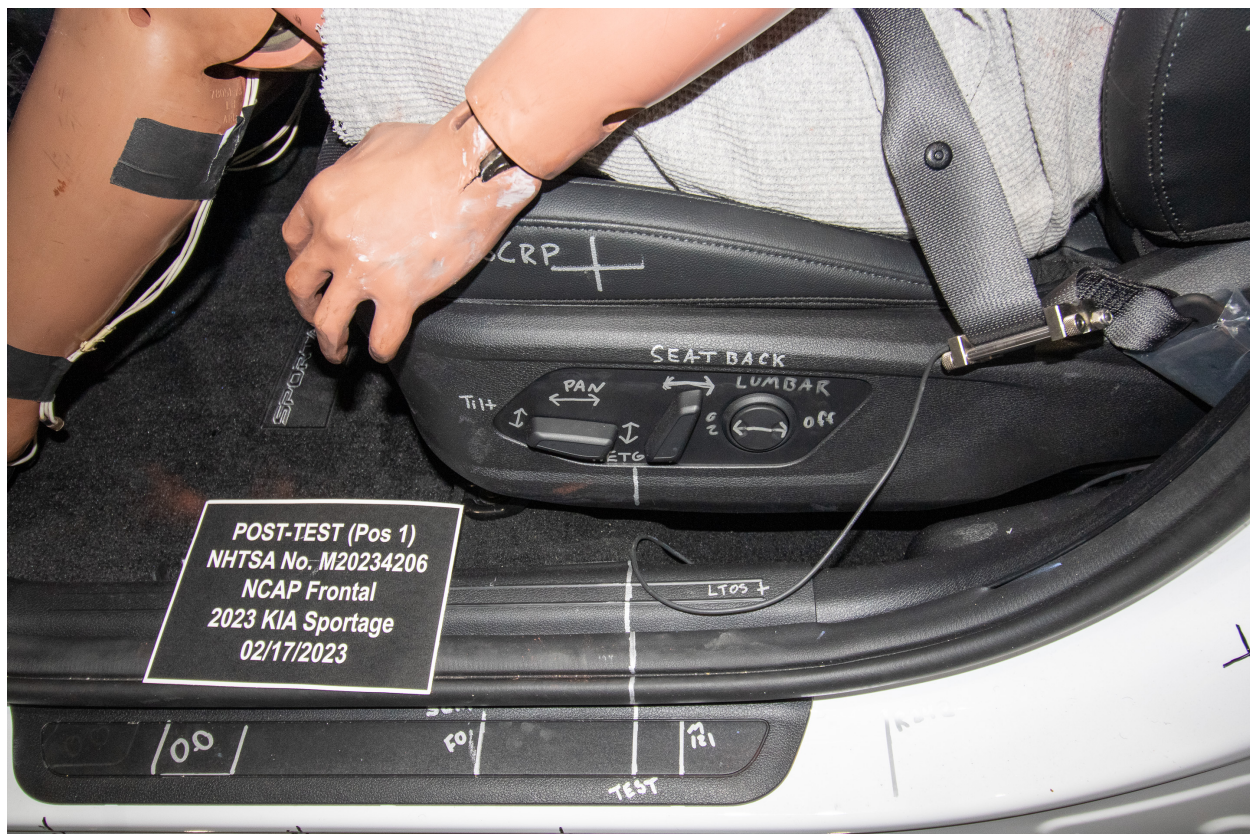
Figure A-37: Post-Test Driver's Seat Fore-Aft Markings
