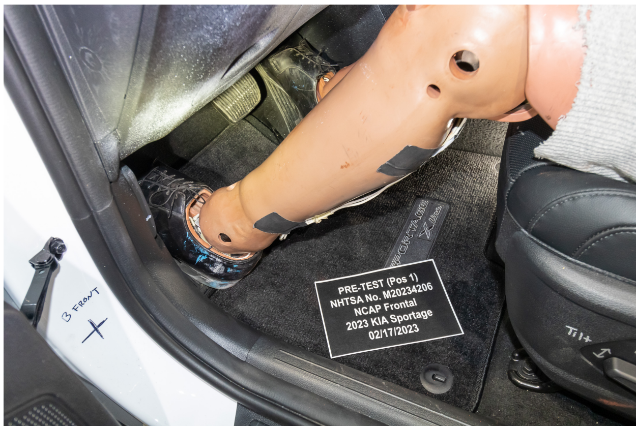
Figure A-42: Pre-Test Driver Dummy Feet
