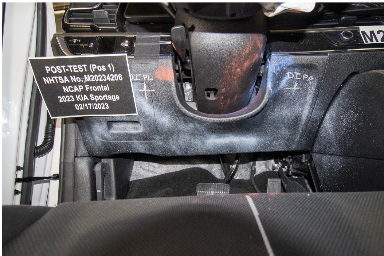
Figure A-45: Post-Test Driver's Side Knee Bolster
