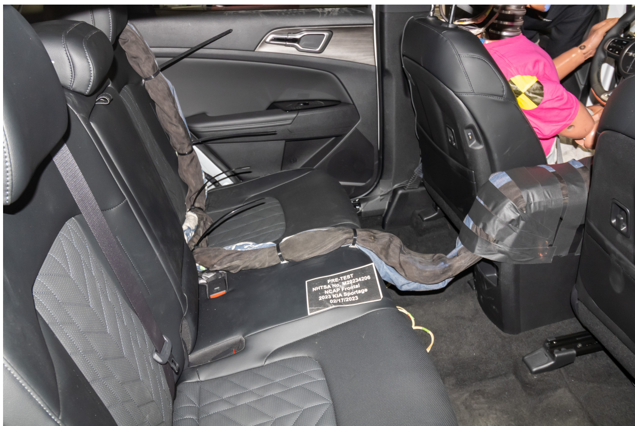
Figure A-28: Pre-Test Dummy Cable Routing
