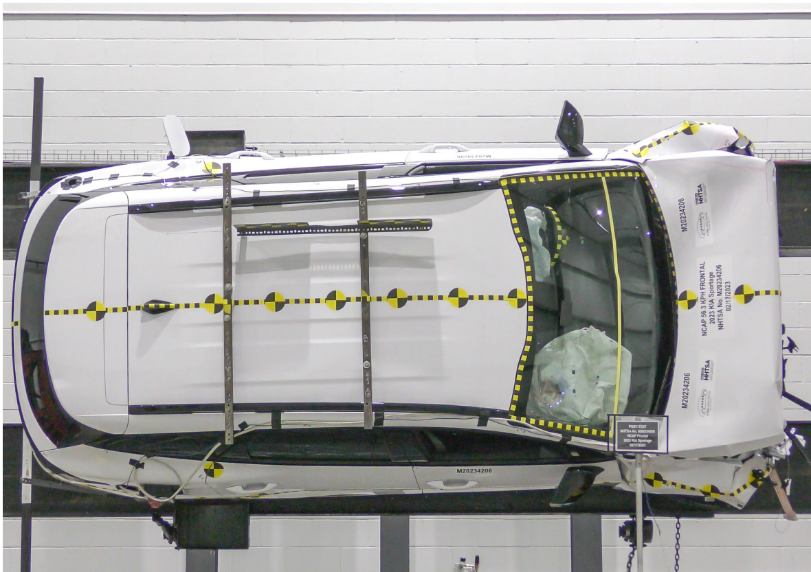
Figure A-80: Vehicle at 270° on Static Rollover Device
