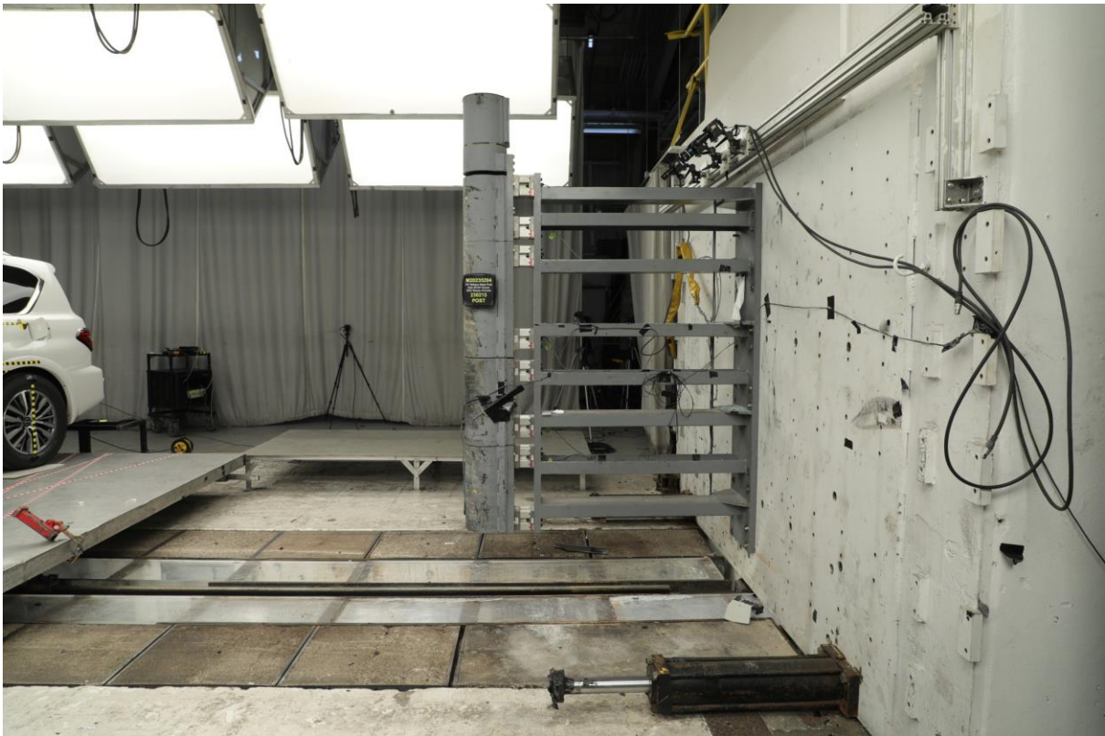
No. 062 Post-Test Pole Barrier Side View
