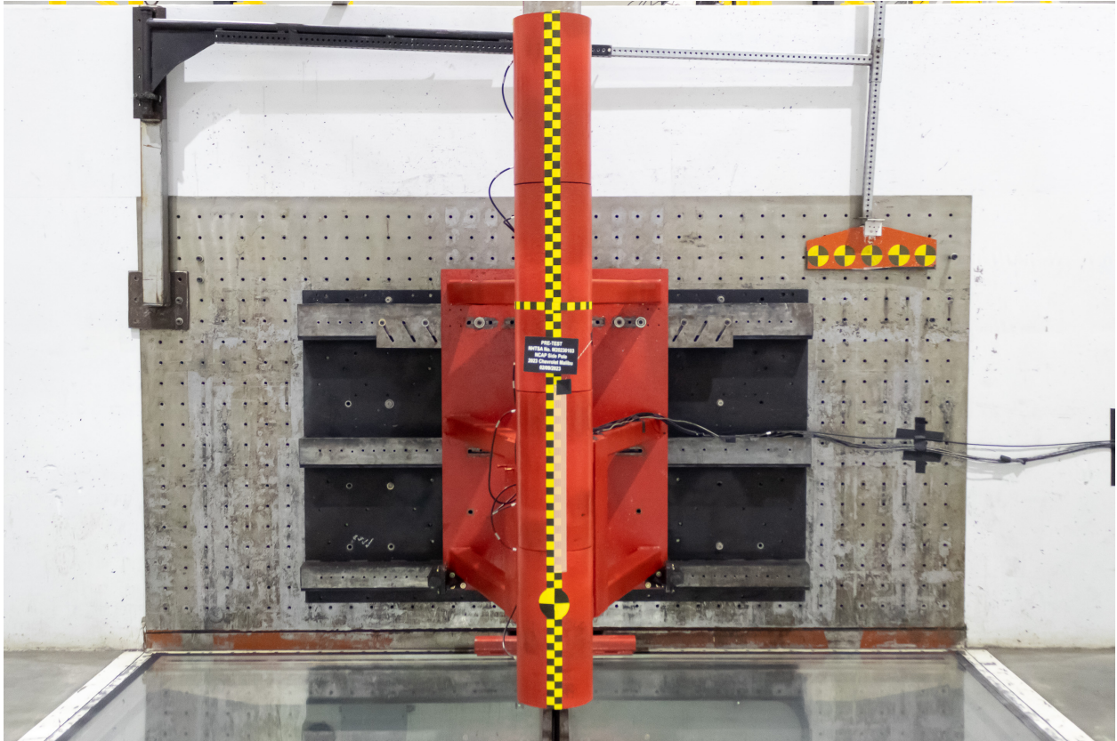
Figure A-59: Pre-Test Pole Barrier Front View
