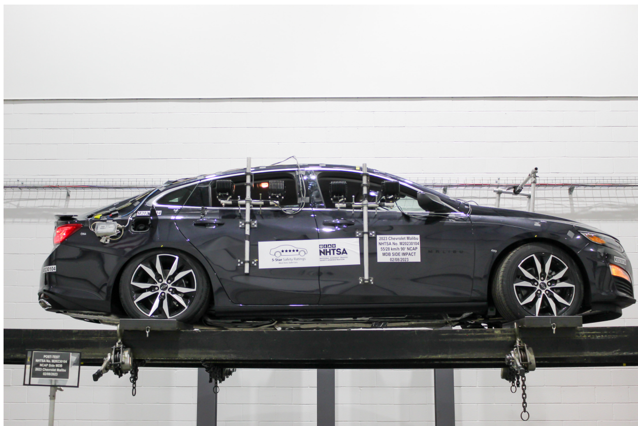
Figure A-96: FMVSS No. 301 Static Rollover 0 Degrees
