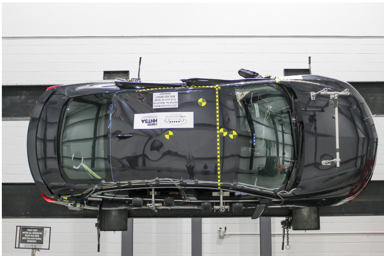
Figure A-97: FMVSS No. 301 Static Rollover 90 Degrees
