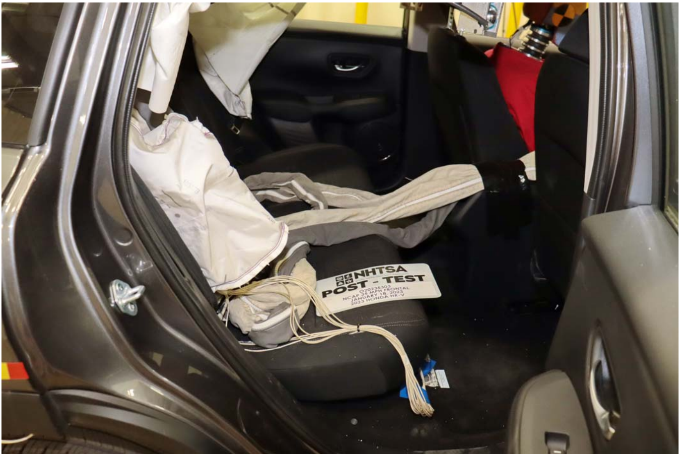
Photo No. 029 - Post-Test Dummy Cable Routing
