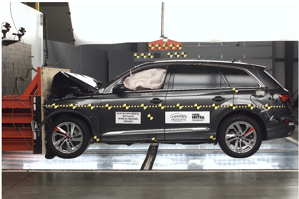
Figure A-82: 2023 Audi Q7 Frontal Impact Event
