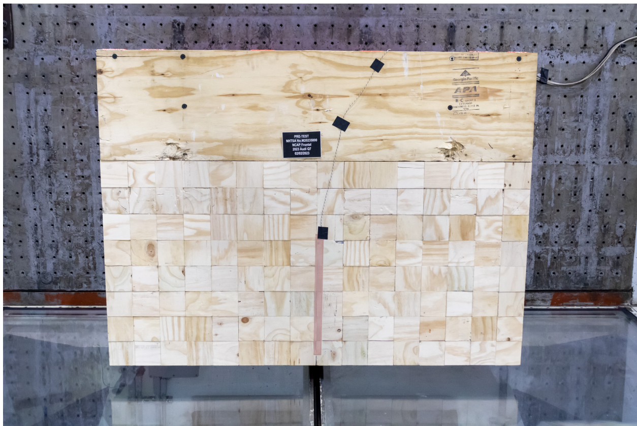
Figure A-2: Pre-Test Load Cell Wall
