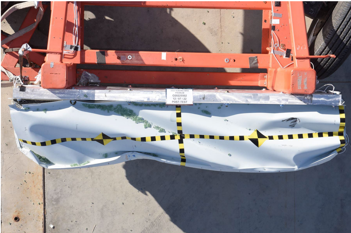
FIGURE 87. Post-Test Top View of MDB Impactor Face
