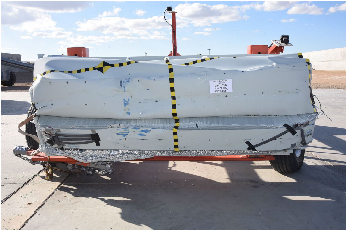
FIGURE 85. Post-Test Front View of MDB Impactor Face
