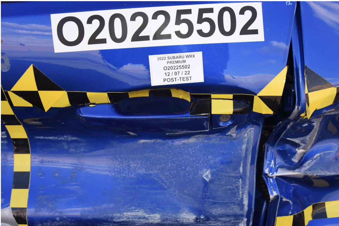
FIGURE 22. Post-Test Left Front Door Latch Close-Up
