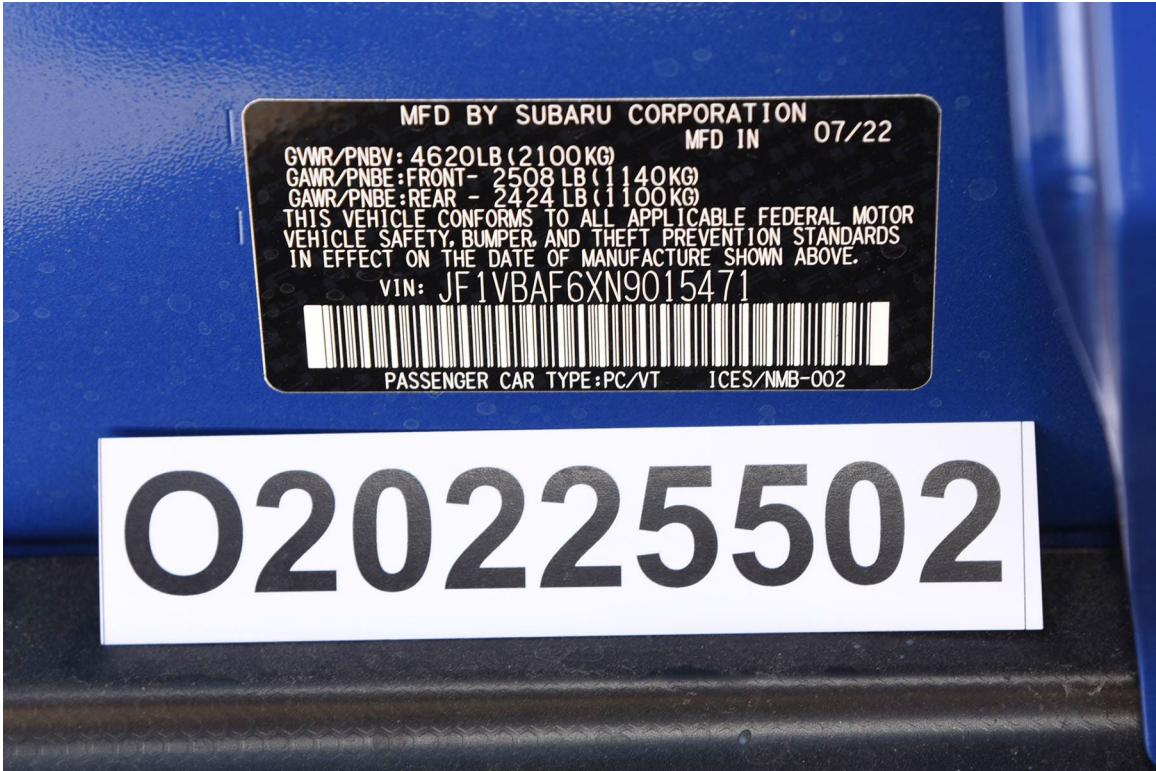
FIGURE 92. Close-Up View of Vehicle's Certification Label
