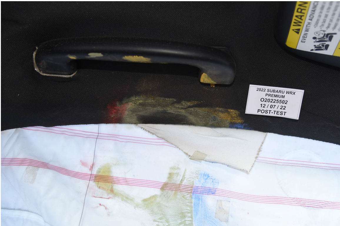
FIGURE 49a. Post-Test Driver Dummy Close-Up Head Contact with Vehicle Interior View
