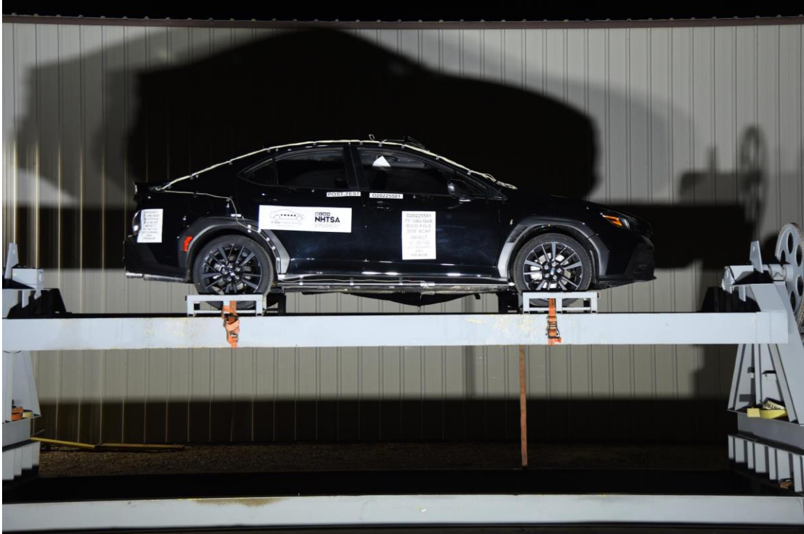
FIGURE 69. FMVSS No. 301 Static Rollover 360 Degrees
