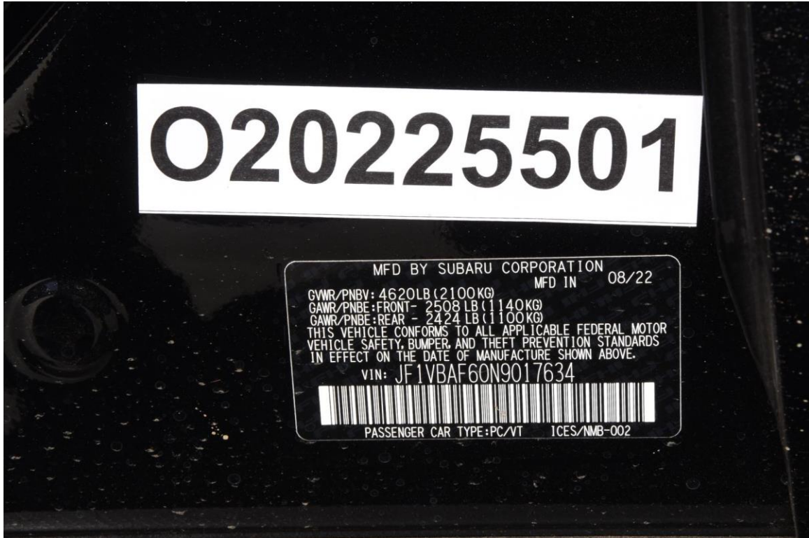
FIGURE 57. Close-Up View of Vehicle's Certification Label
