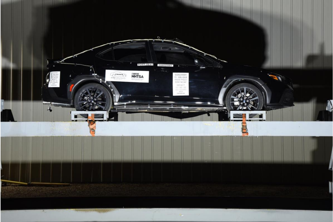
FIGURE 65. FMVSS No. 301 Static Rollover 0 Degrees
