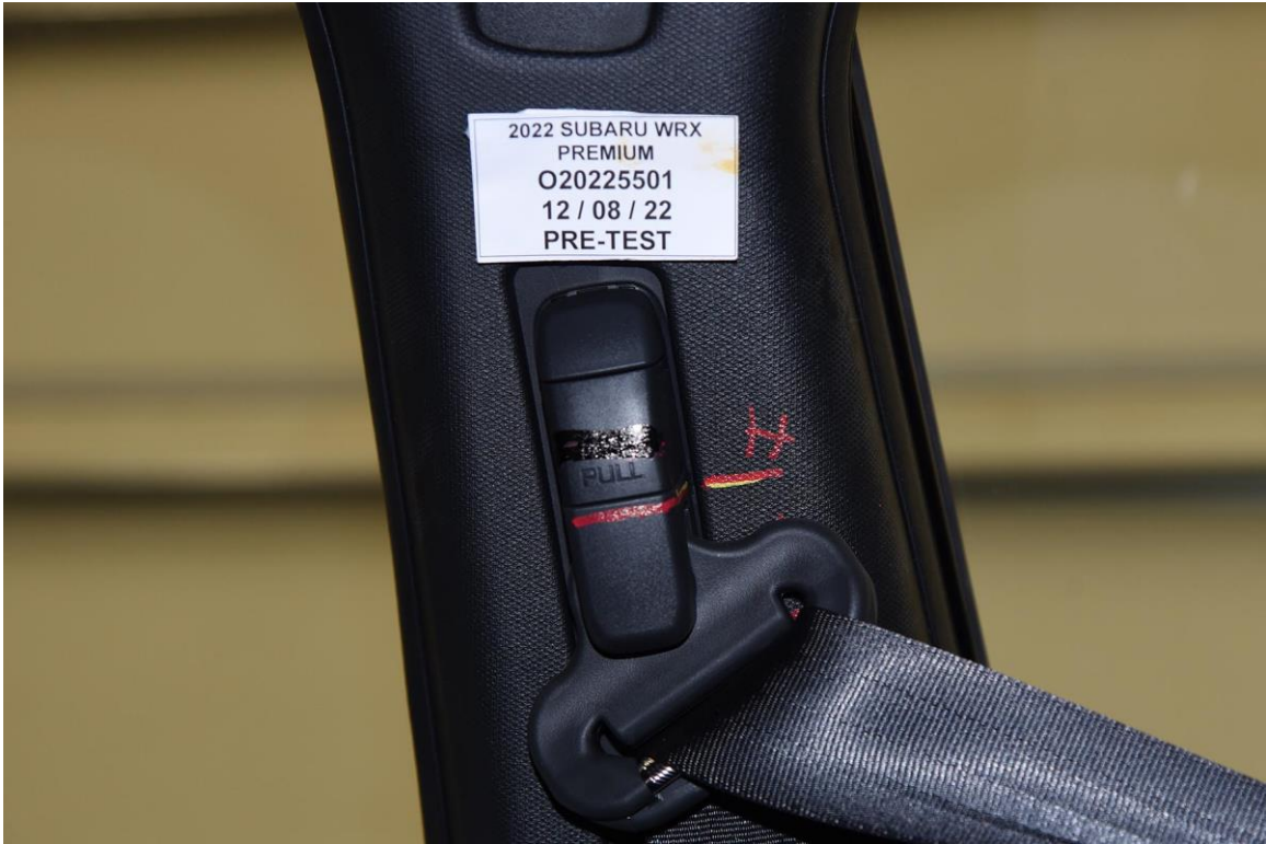
FIGURE 33. Pre-Test View of Belt Anchorage for Dummy
