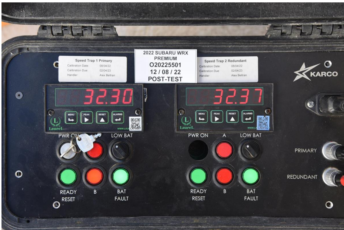
FIGURE 64. Post-Test Primary and Redundant Speed Trap Read-Out
