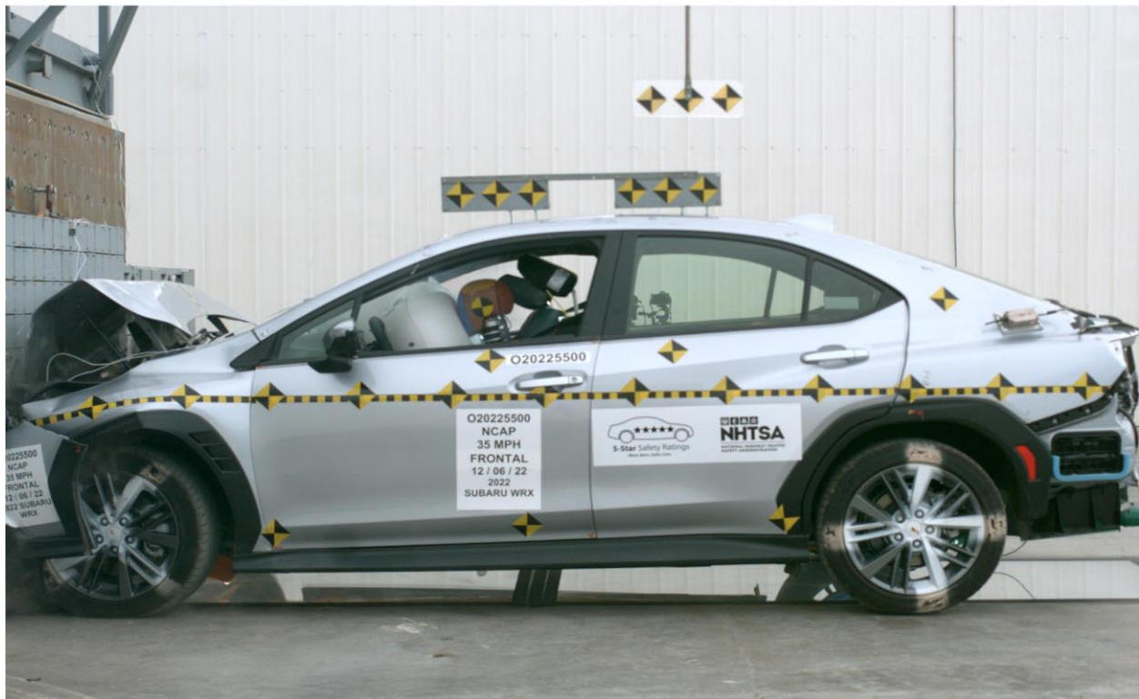
FIGURE 82. 2022 Subaru WRX Frontal Impact Event
