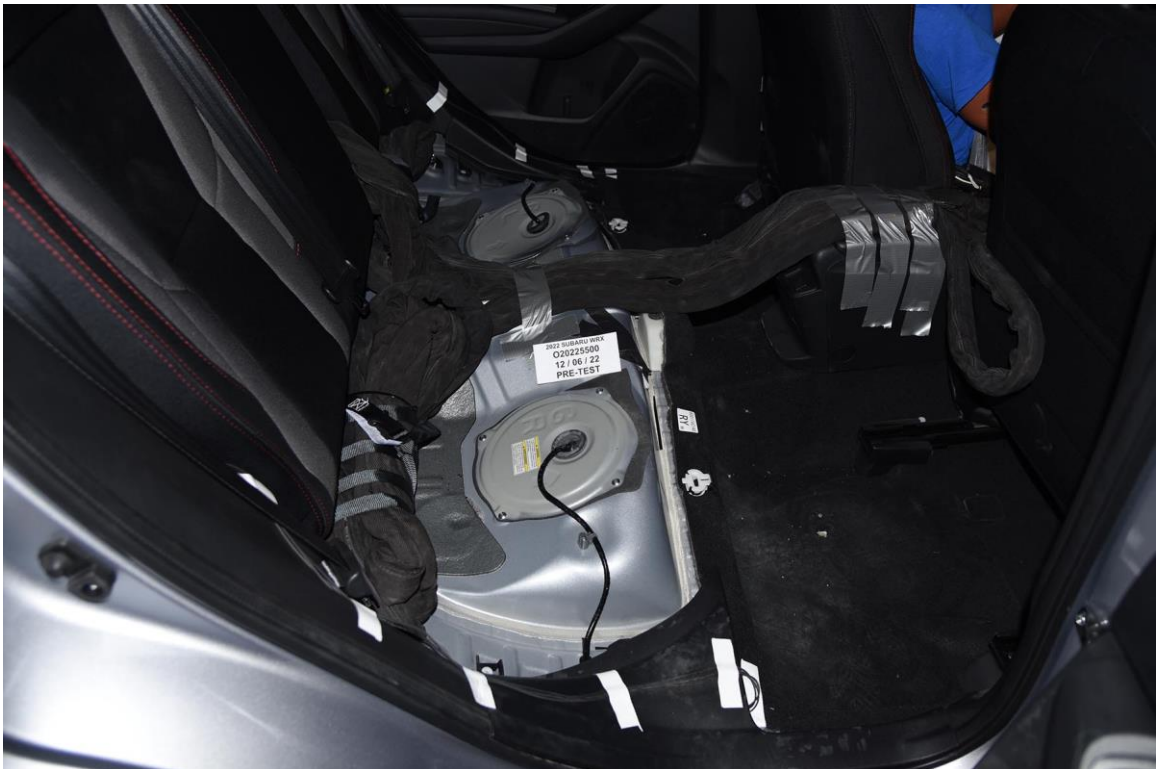
FIGURE 28. Pre-Test Dummy Cable Routing
