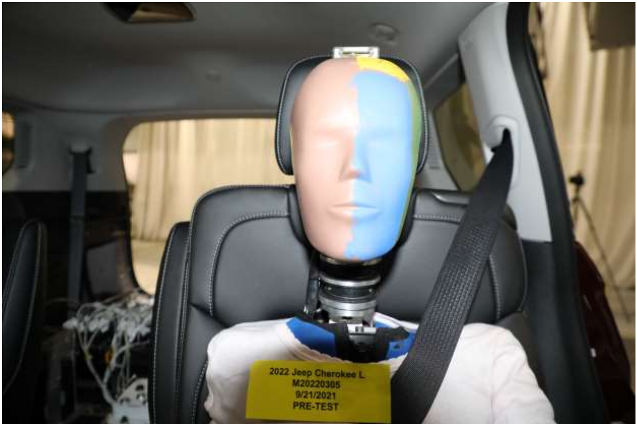
059 Pre-Test Frontal View of Rear Passenger Dummy Head and Shoulders in Relation to Head Restraint 1
