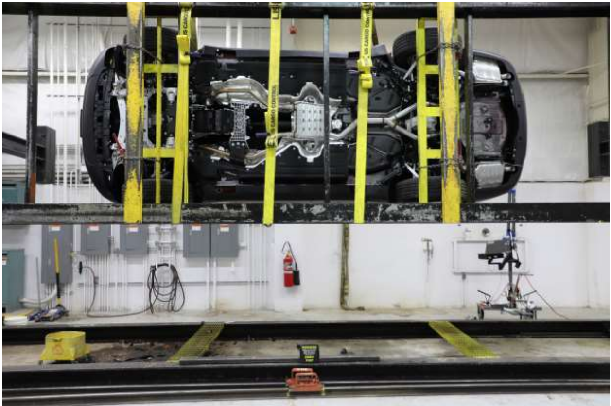
099 FMVSS No. 301 Static Rollover 270 Degrees
