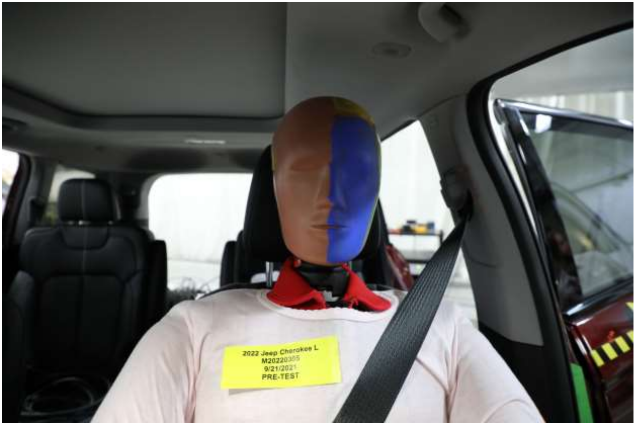
025 Pre-Test Front Close-Up View of Driver Dummy 1
