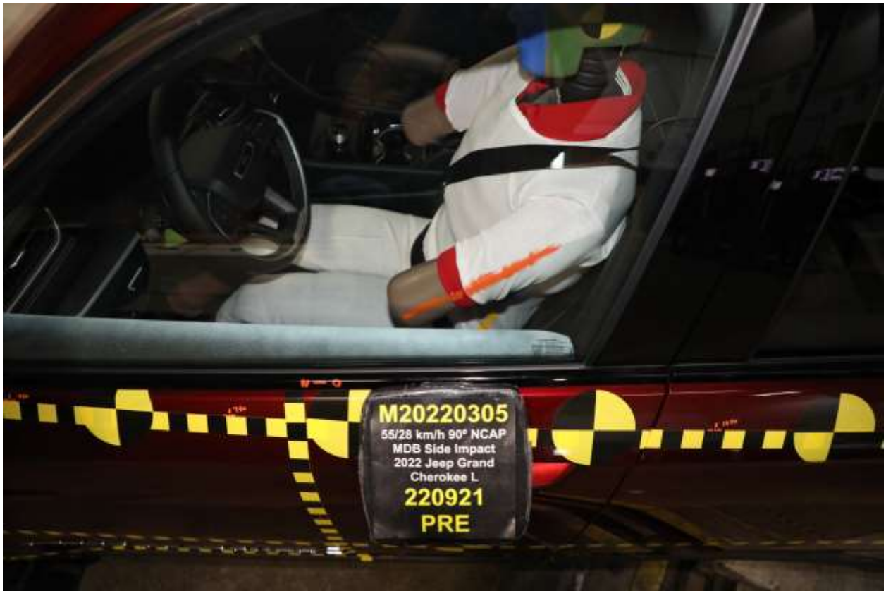
042 Pre-Test Driver Dummy and Door Clearance View
