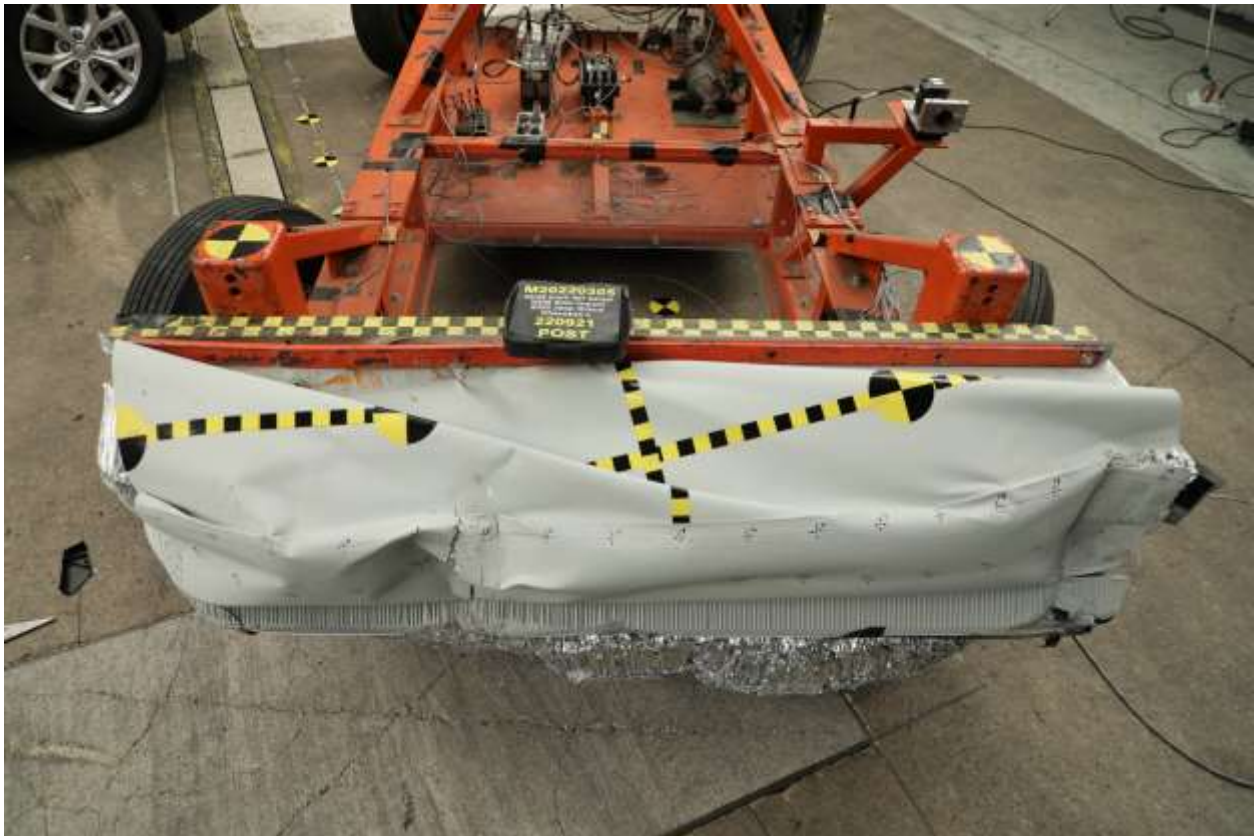
087 Post-Test Top View of MDB Impactor Face
