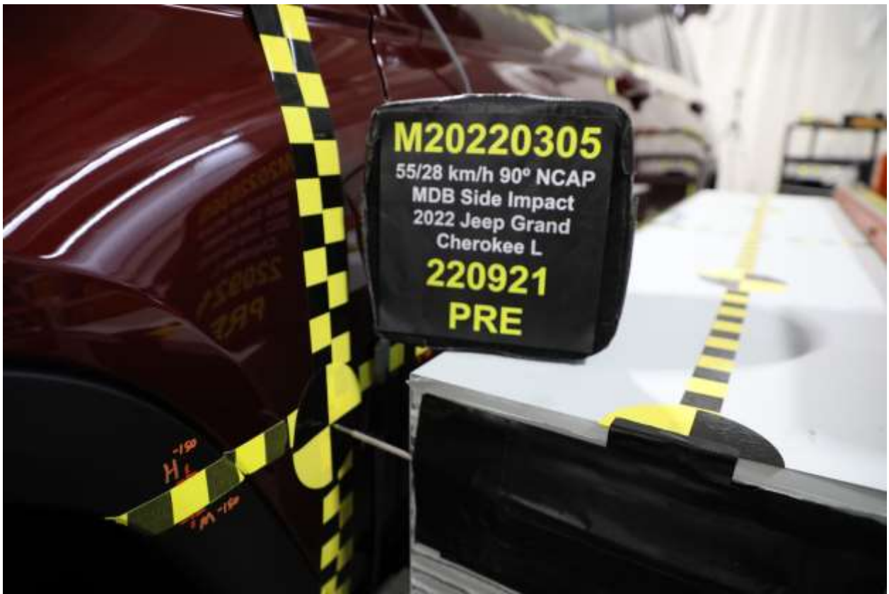
019 Pre-Test Close-Up View of Impact Point Target
