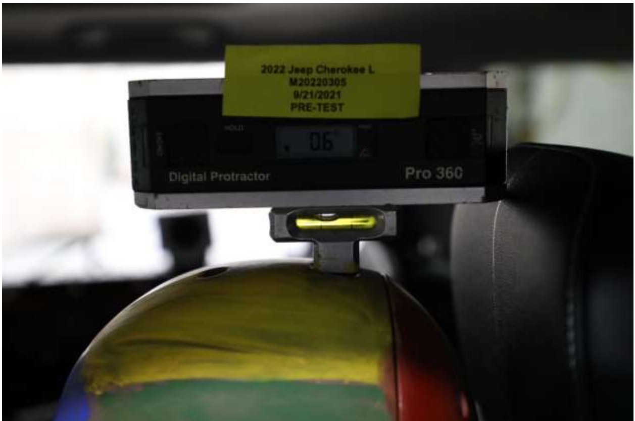
063 Pre-Test View of Rear Passenger Dummy's Head Showing Dummy Head is Level 1
