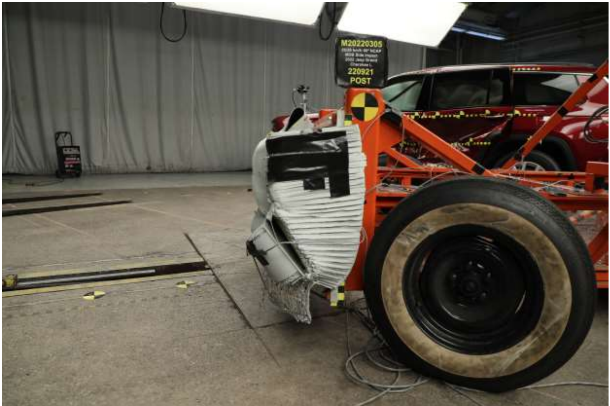
089 Post-Test Left Side View of MDB Impactor Face
