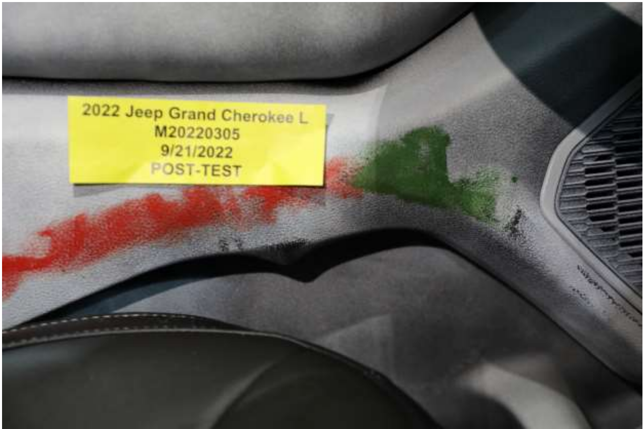
054 Post-Test Driver Dummy Close-Up Knee Contact View
