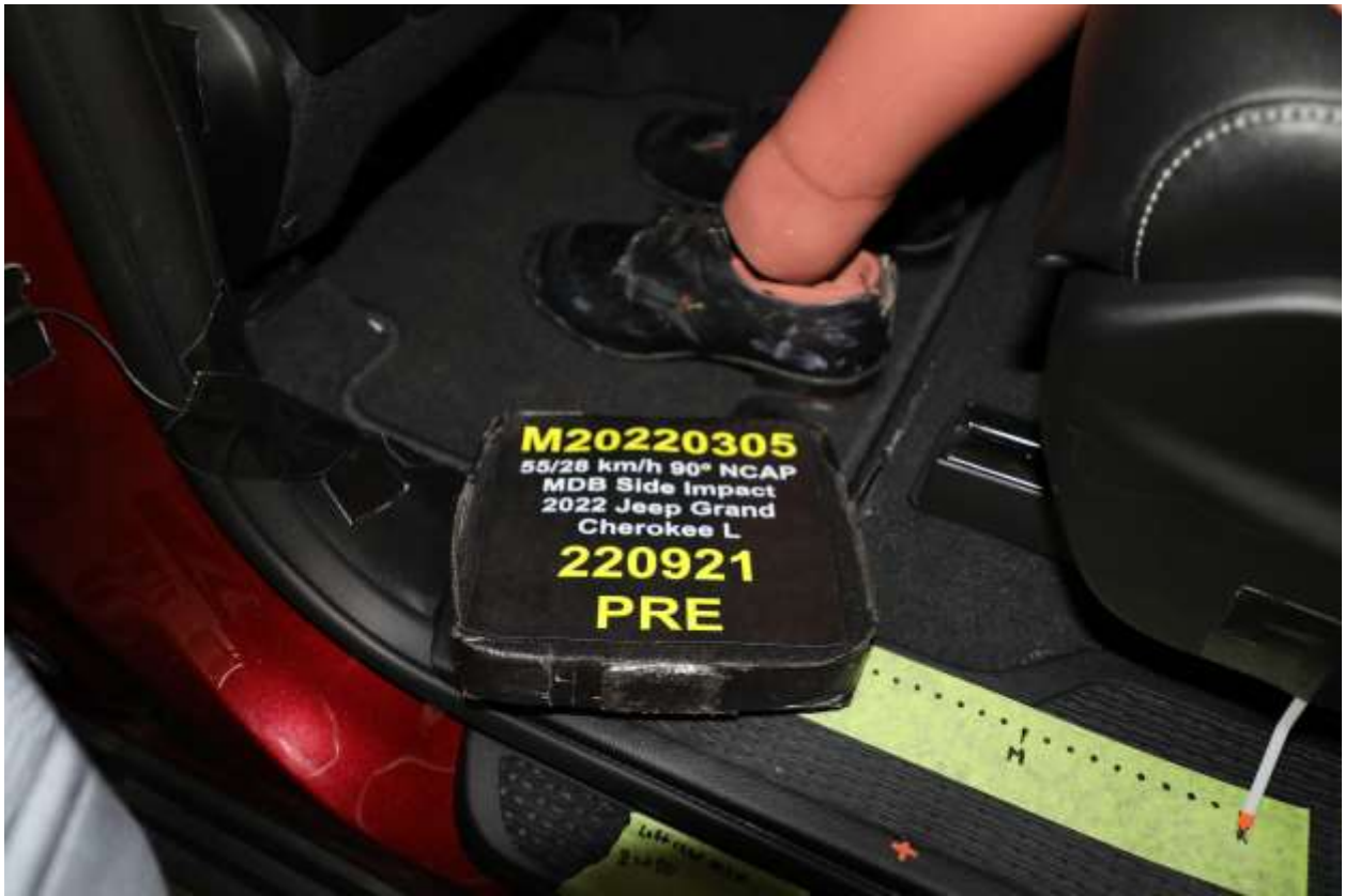
064 Pre-Test Placement of Rear Passenger Dummy's Feet
