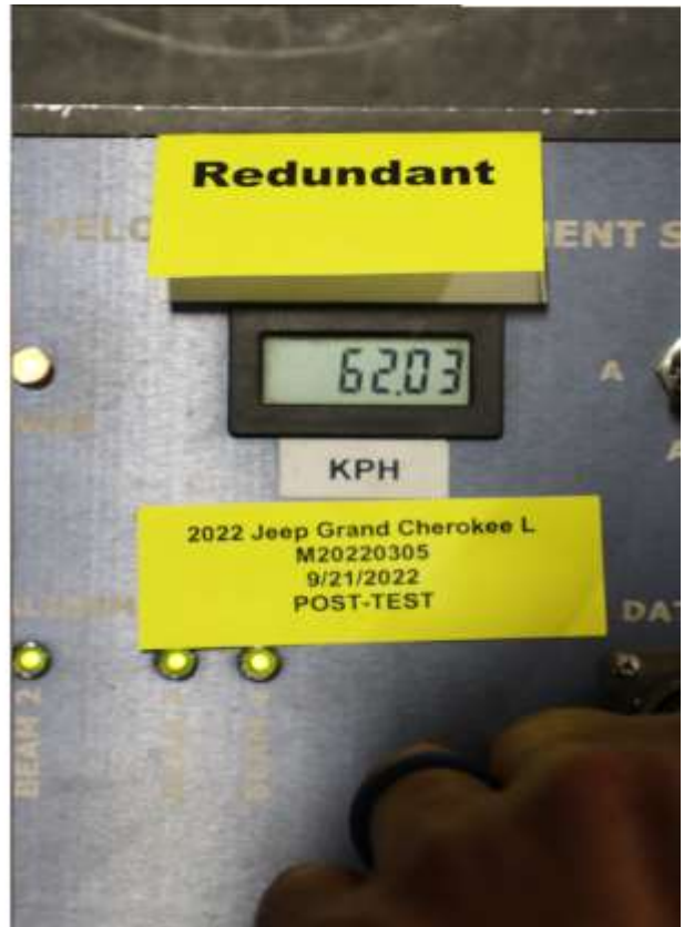
095 Post-Test Primary and Redundant Speed Trap Read-Out
