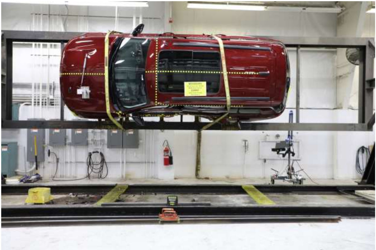
097 FMVSS No. 301 Static Rollover 90 Degrees
