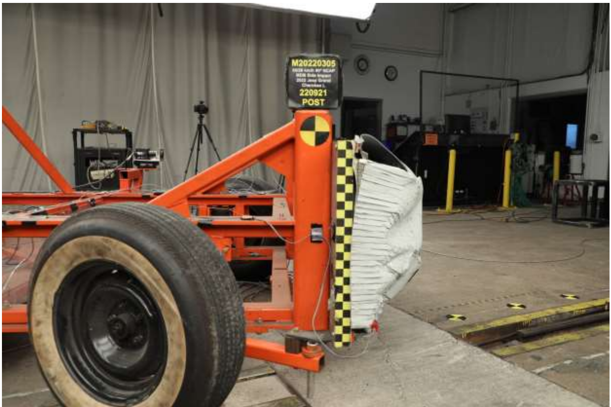
091 Post-Test Right Side View of MDB Impactor Face
