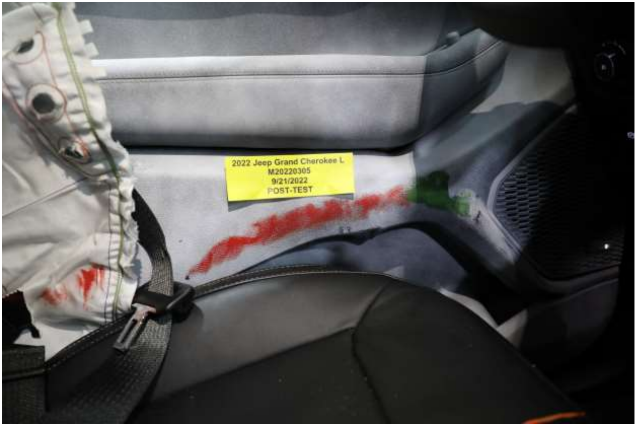
052 Post-Test Driver Dummy Close-Up Pelvis Contact View
