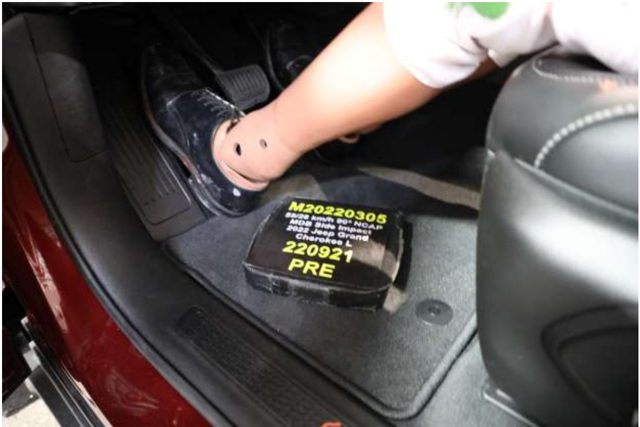
034 Pre-Test Placement of Driver's Dummy Feet
