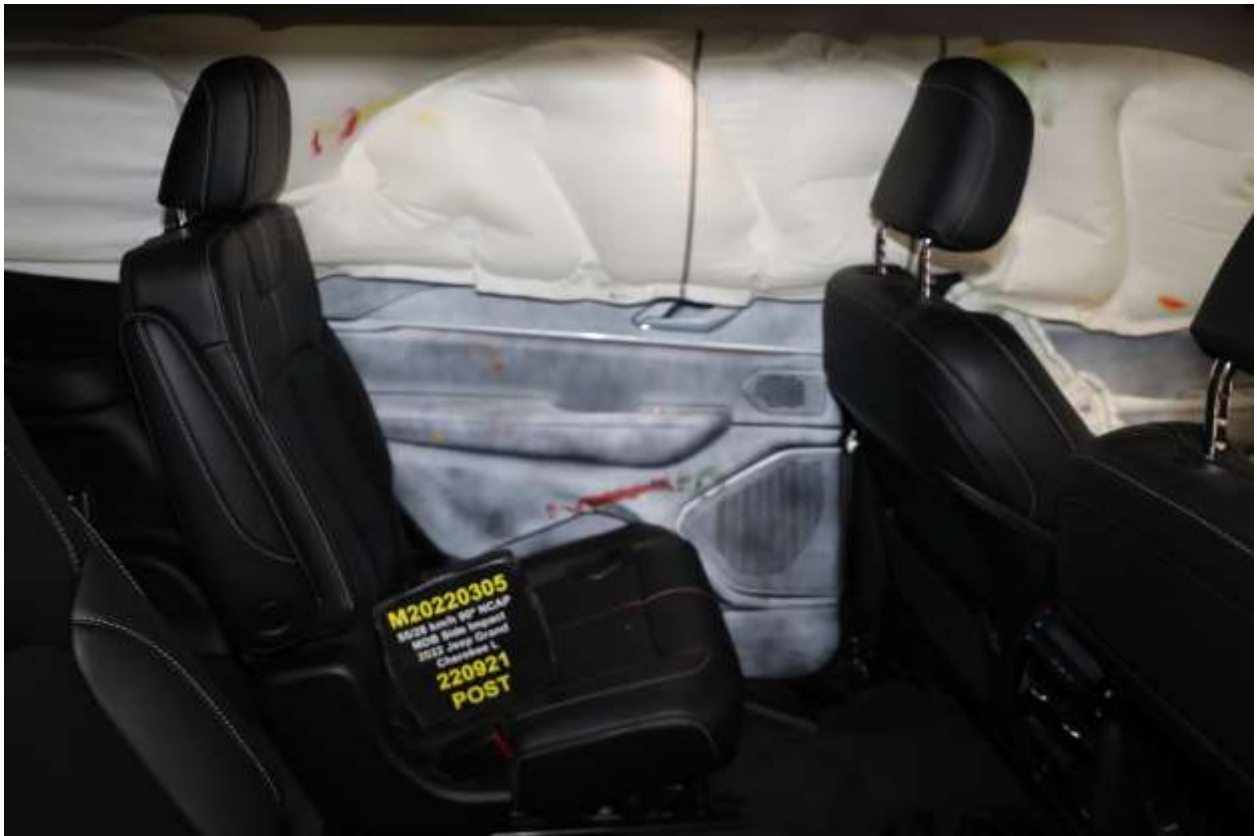
074 Post-Test Rear Passenger Inner Door Panel View
