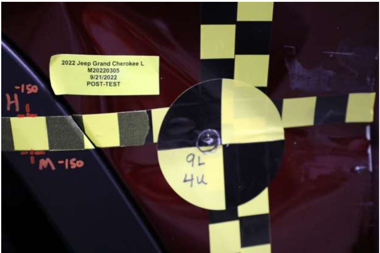
020 Post-Test Close-Up View of Impact Point Target
