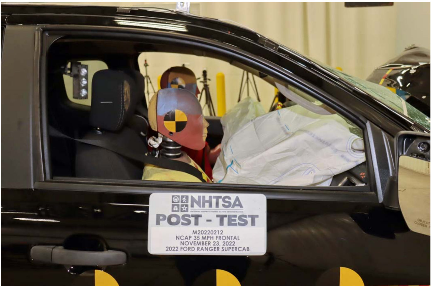
Photo No. 056 - Post-Test Passenger Dummy Window View
