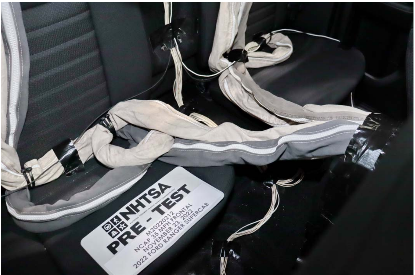
Photo No. 028 - Pre-Test Dummy Cable Routing
