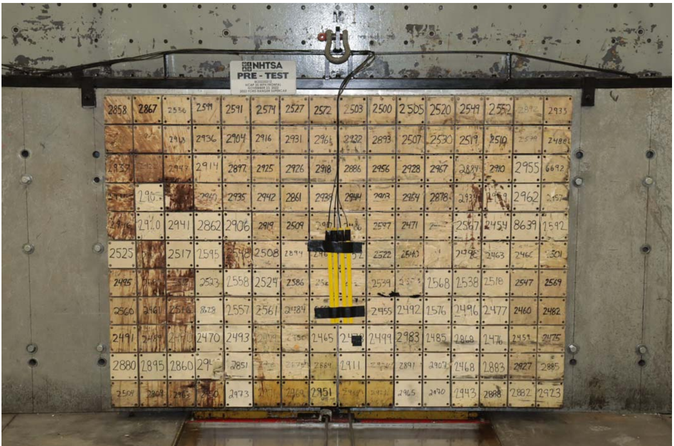
Photo No. 002 - Pre-Test Load Cell Wall
