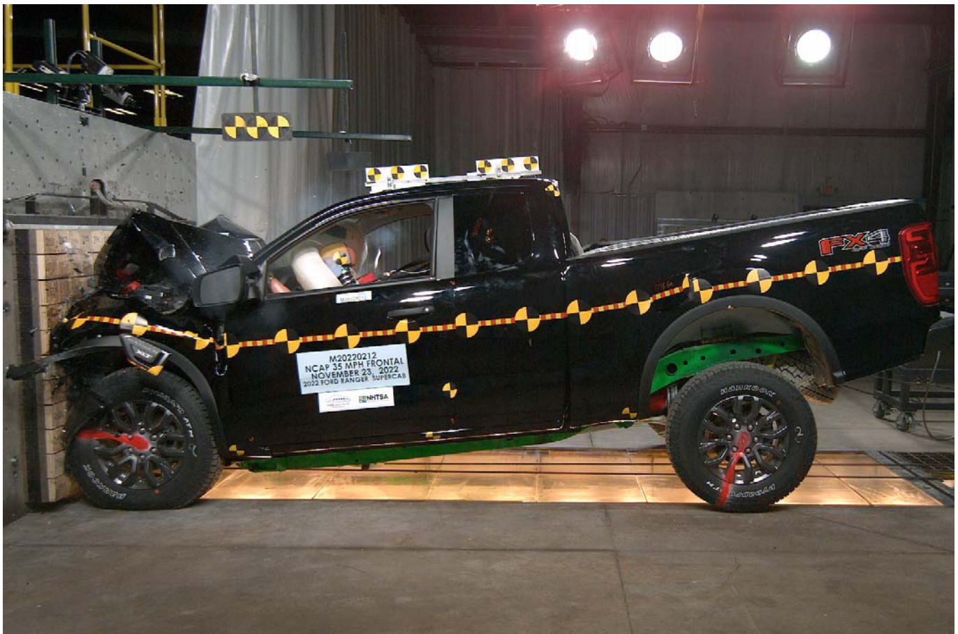
Photo No. 082 - 2022 Ford Ranger XLT SuperCab 4x4 Pickup Truck Frontal Impact Event
