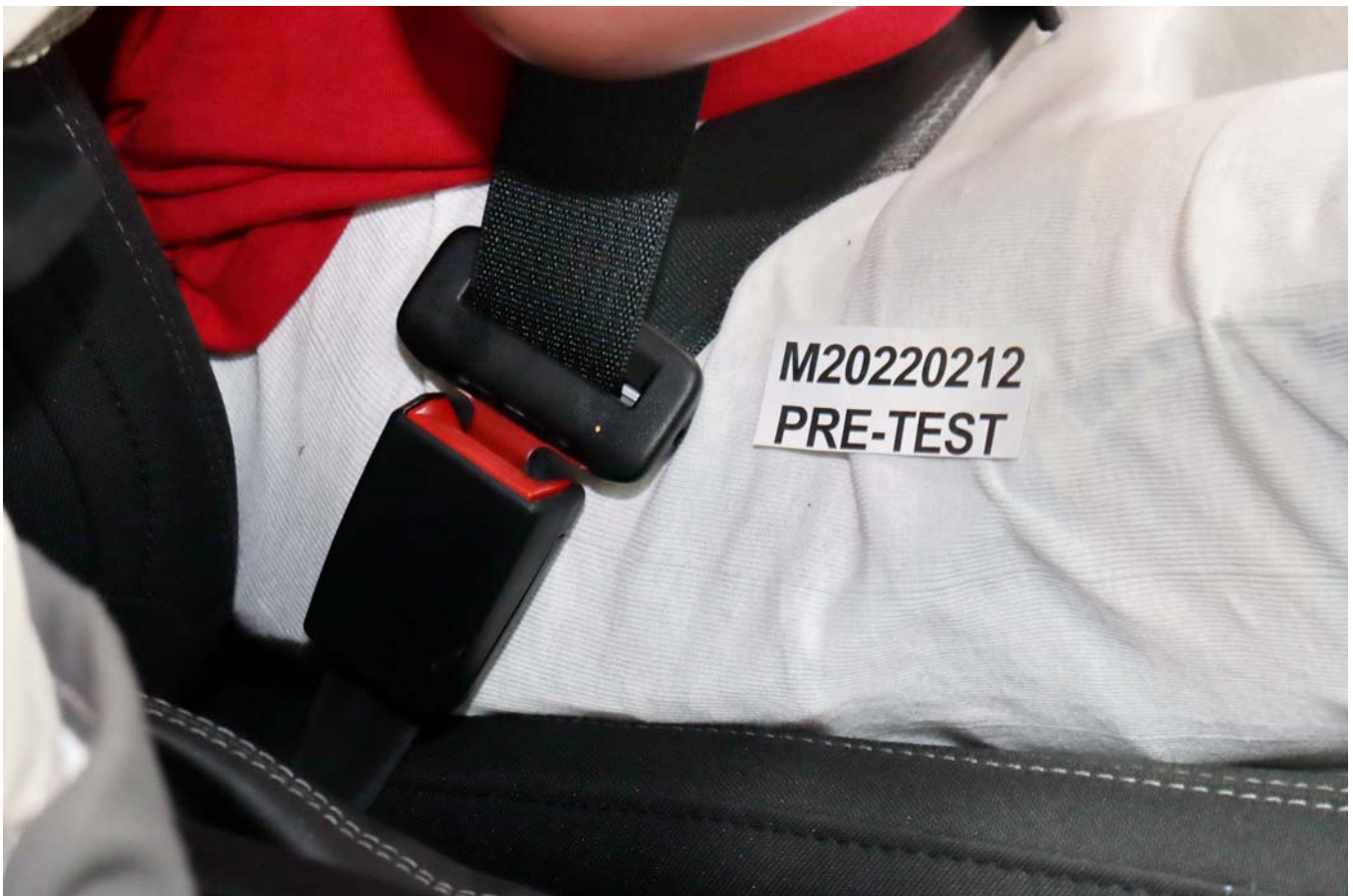
Photo No. 040 - Pre-Test View of Belt Buckle and Latch Plate for Driver Dummy
