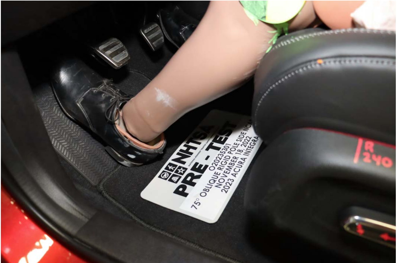
Photo No. 032 - Pre-Test Placement of Dummy's Feet
