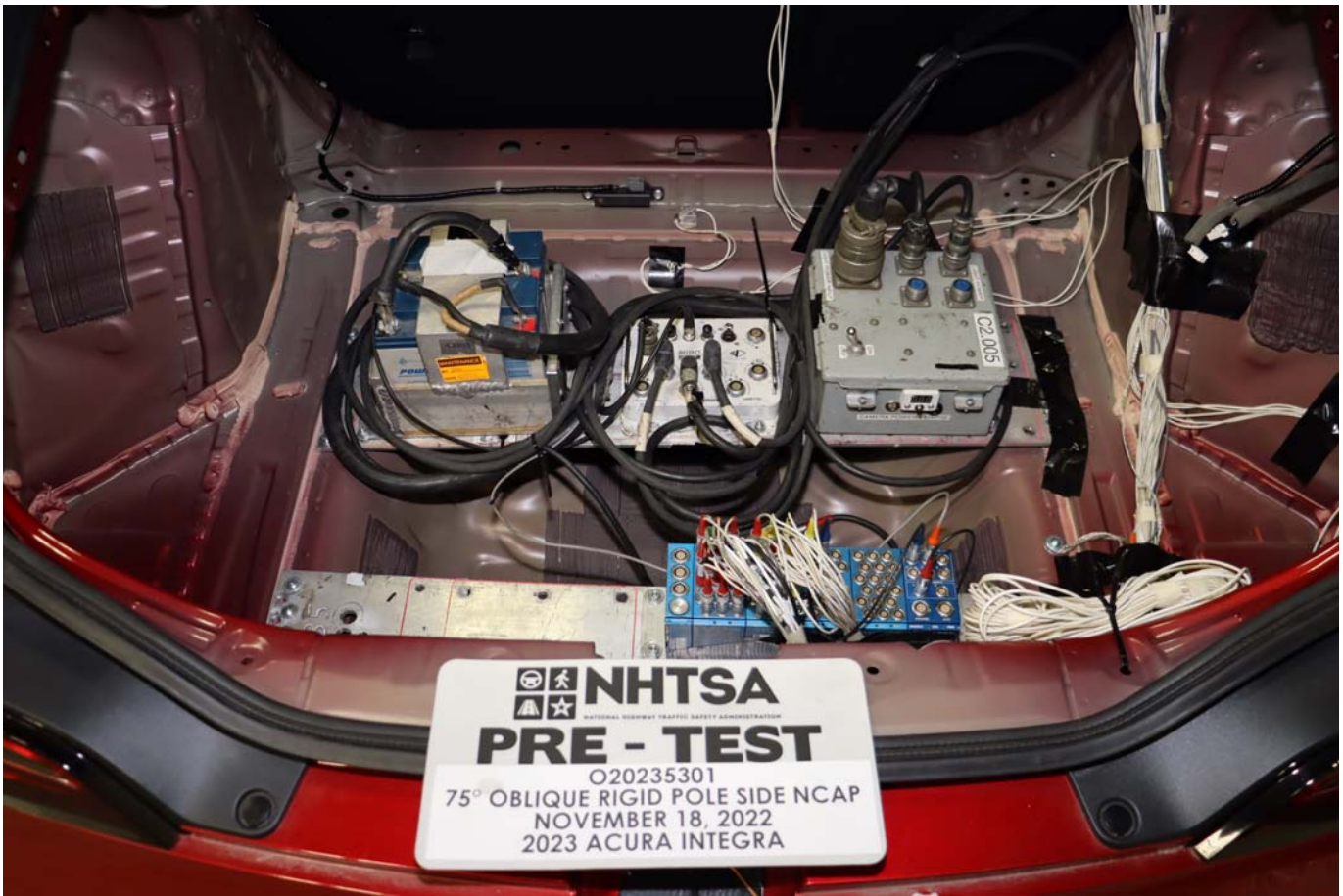
Photo No. 063 - Pre-Test Ballast View
