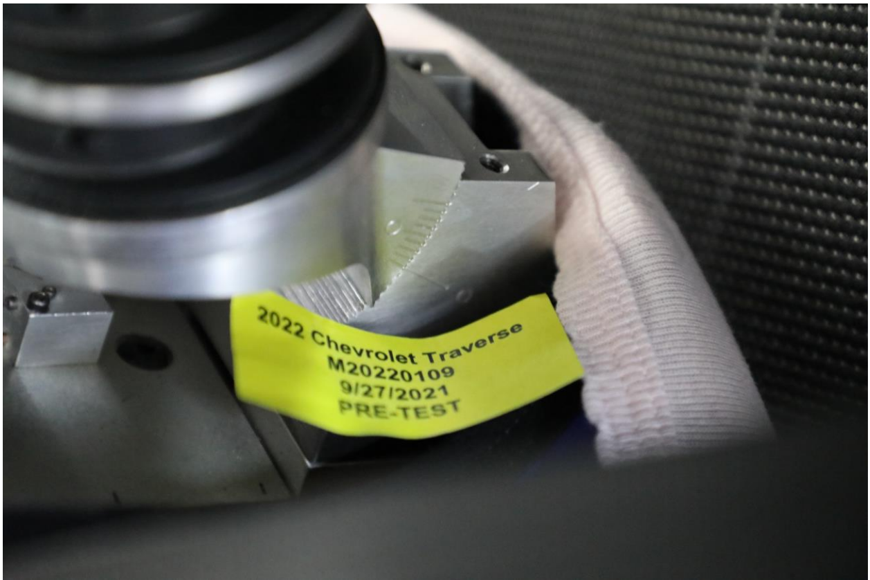
062 Pre-Test View of Rear Passenger Dummy's Neck Showing Position of Adjustable Neck Bracket 1
