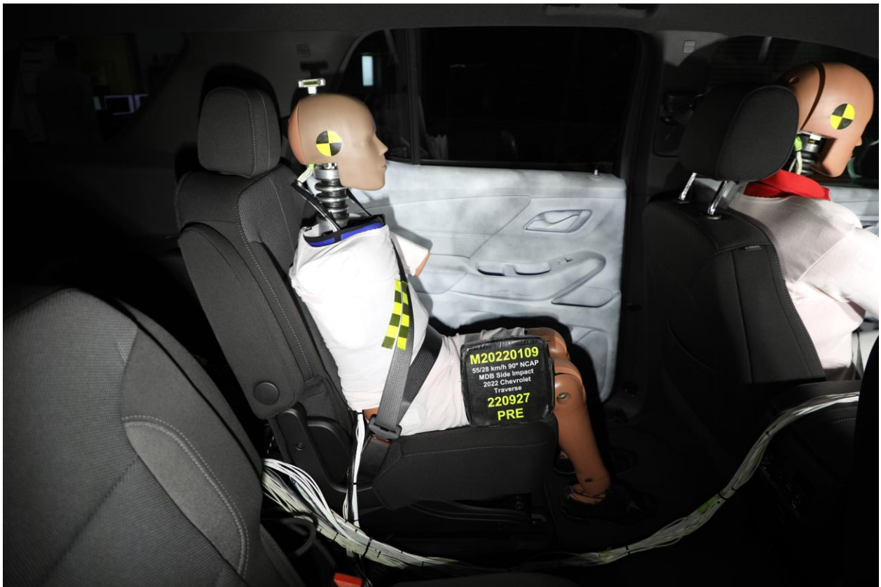
071 Pre-Test Right Side View of Rear Passenger Dummy and Rear Seat Occupant Compartment
