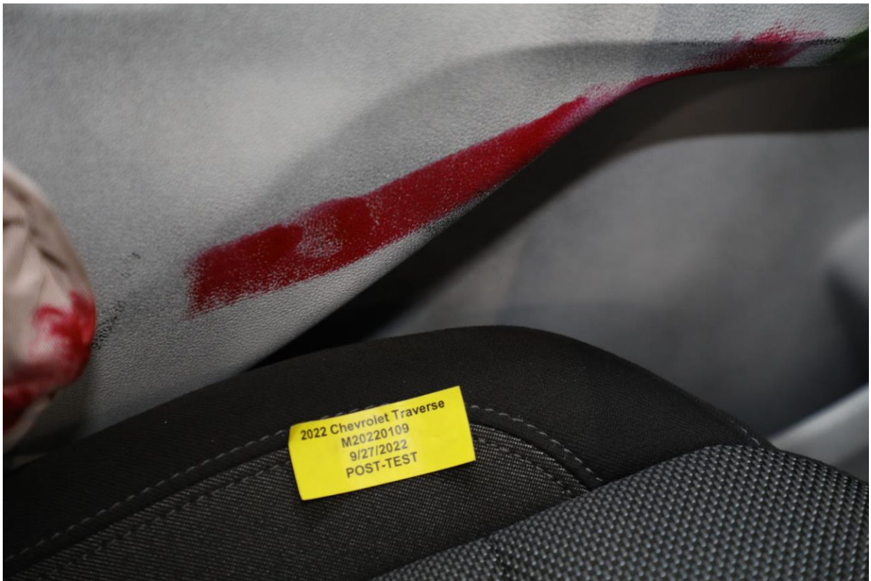
052 Post-Test Driver Dummy Close-Up Pelvis Contact View
