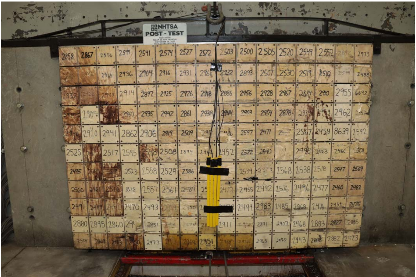
Photo No. 003 - Post-Test Load Cell Wall
