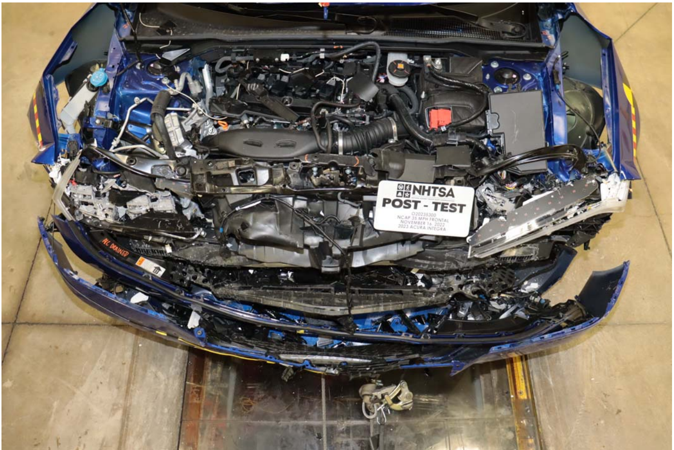
Photo No. 021 - Post-Test Engine Compartment View
