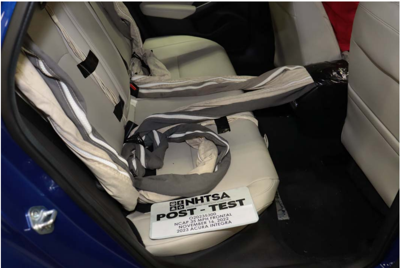
Photo No. 029 - Post-Test Dummy Cable Routing
