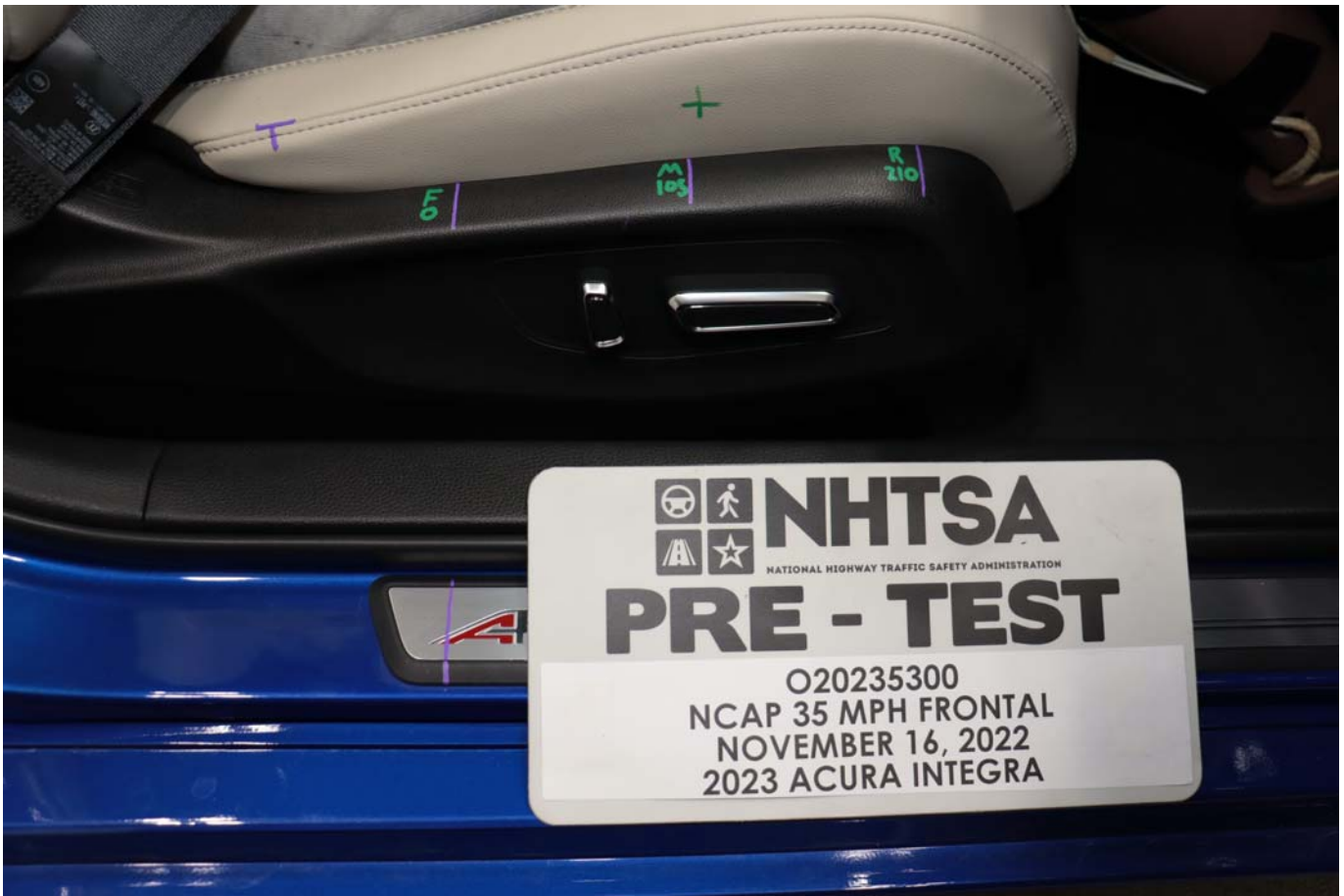
Photo No. 059 - Pre-Test Passenger's Seat Fore-Aft Markings
