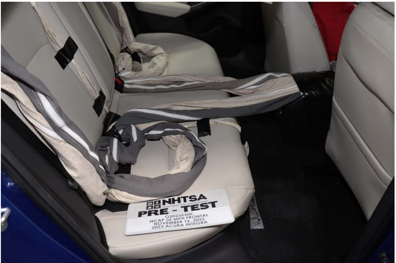
Photo No. 028 - Pre-Test Dummy Cable Routing
