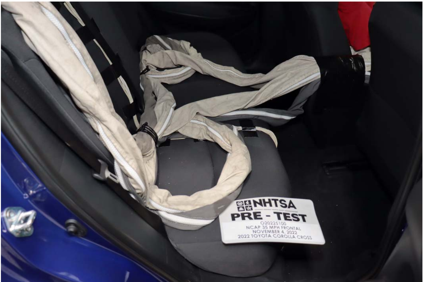
Photo No. 028 - Pre-Test Dummy Cable Routing
