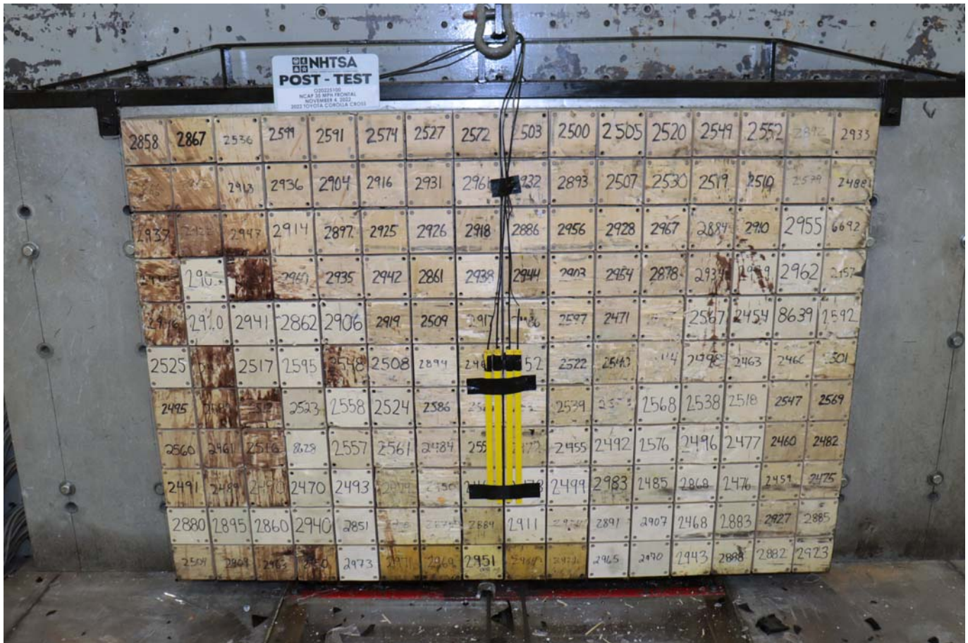
Photo No. 003 - Post-Test Load Cell Wall
