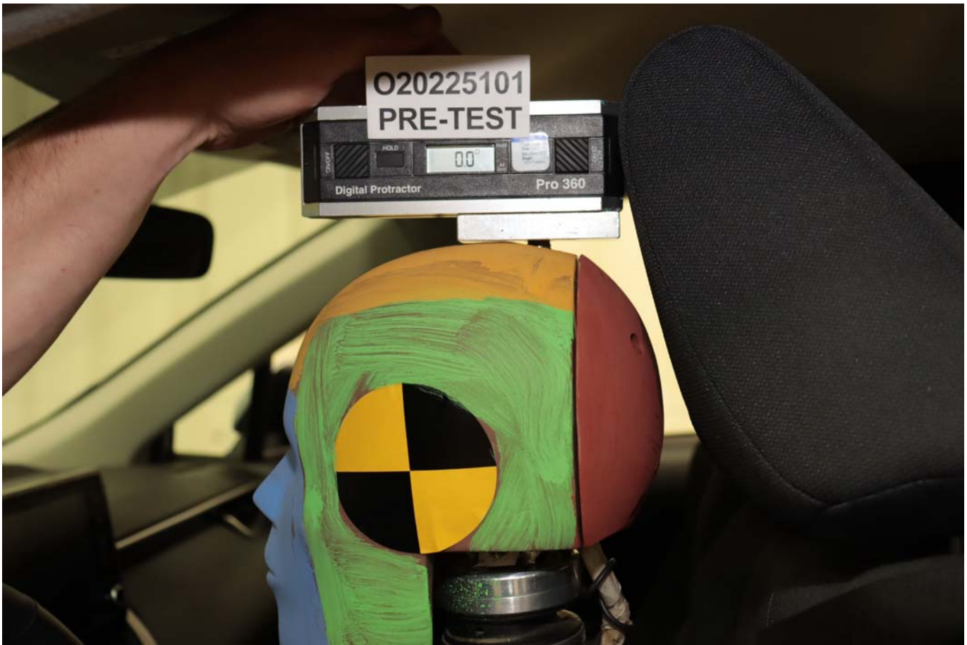
Photo No. 031 - Pre-Test Left Side View of Dummy's Head Showing Dummy's Head is Level
