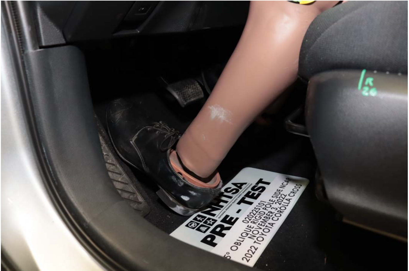
Photo No. 032 - Pre-Test Placement of Dummy's Feet
