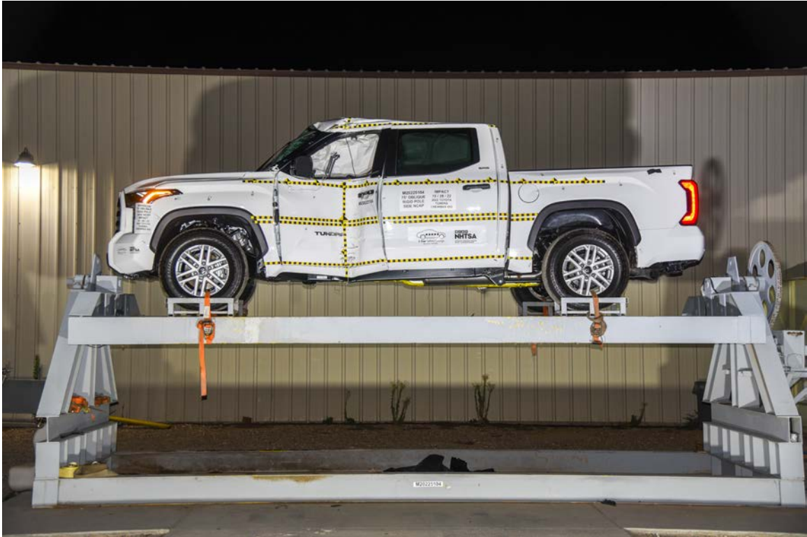
FIGURE 69. FMVSS No. 301 Static Rollover 360 Degrees
