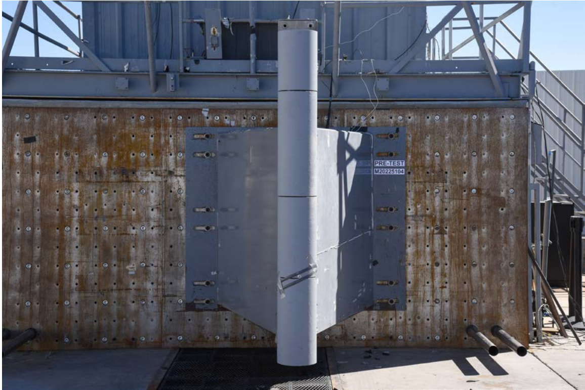
FIGURE 59. Pre-Test Pole Barrier Front View
