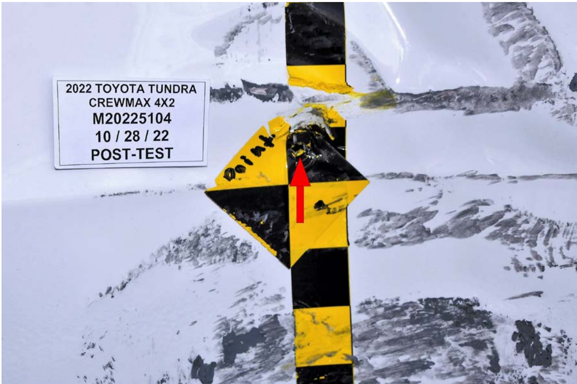
FIGURE 20. Post-Test Close-Up View of Impact Point Target Showing Impact Location
