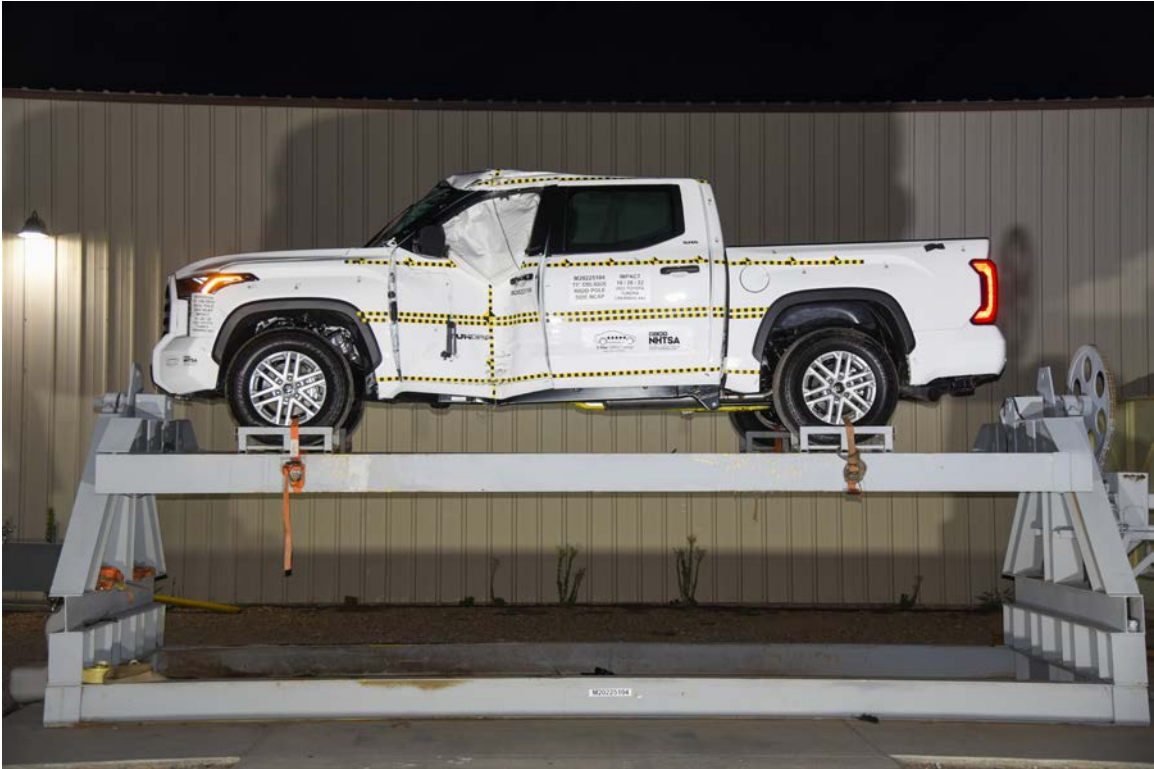
FIGURE 65. FMVSS No. 301 Static Rollover 0 Degrees
