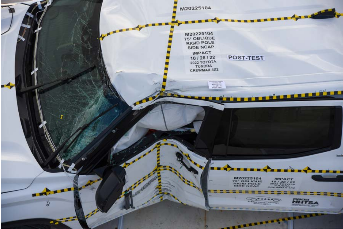
FIGURE 41. Post-Test Dummy and Door Clearance View
