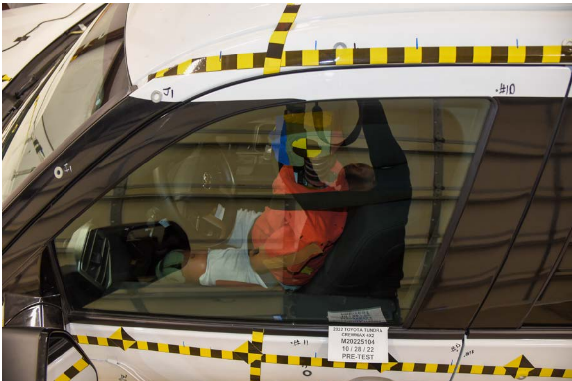
FIGURE 40. Pre-Test Dummy and Door Clearance View
