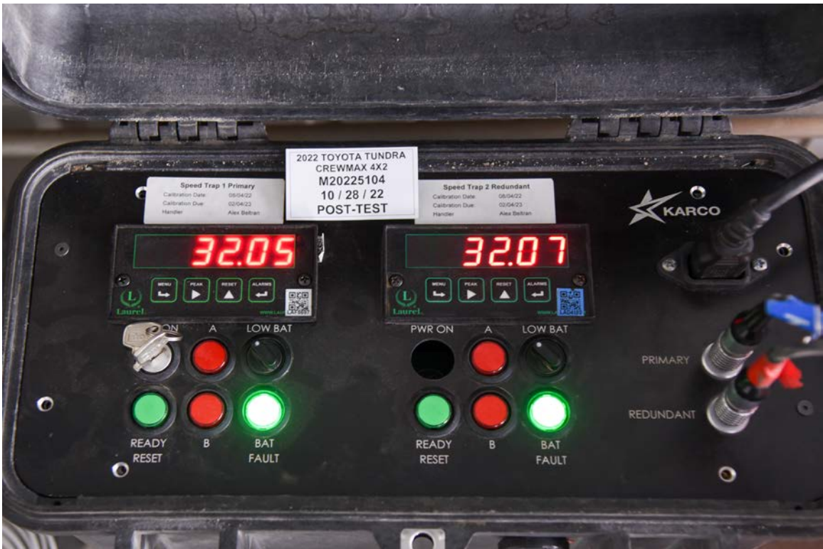
FIGURE 64. Post-Test Primary and Redundant Speed Trap Read-Out
