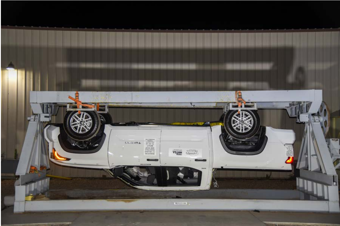
FIGURE 67. FMVSS No. 301 Static Rollover 180 Degrees
