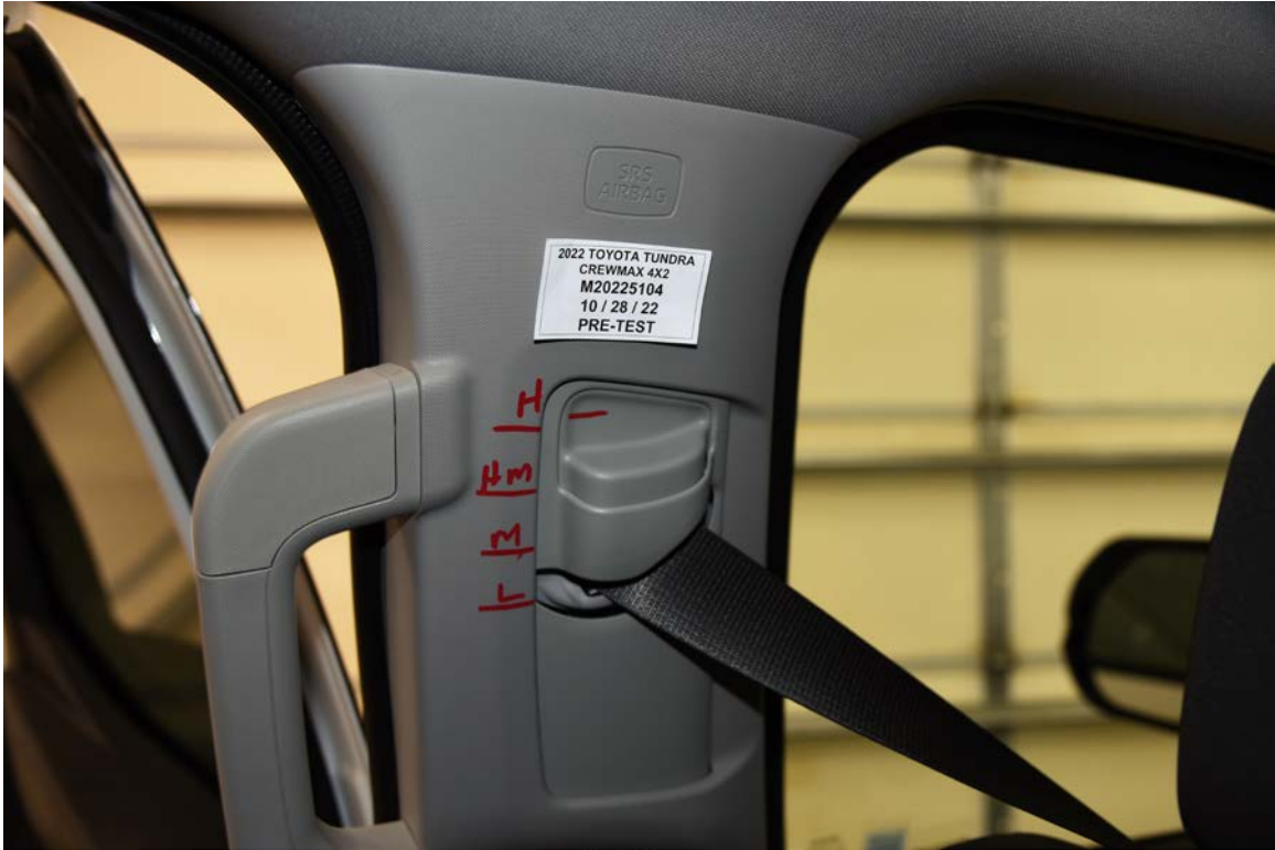
FIGURE 33. Pre-Test View of Belt Anchorage for Dummy
