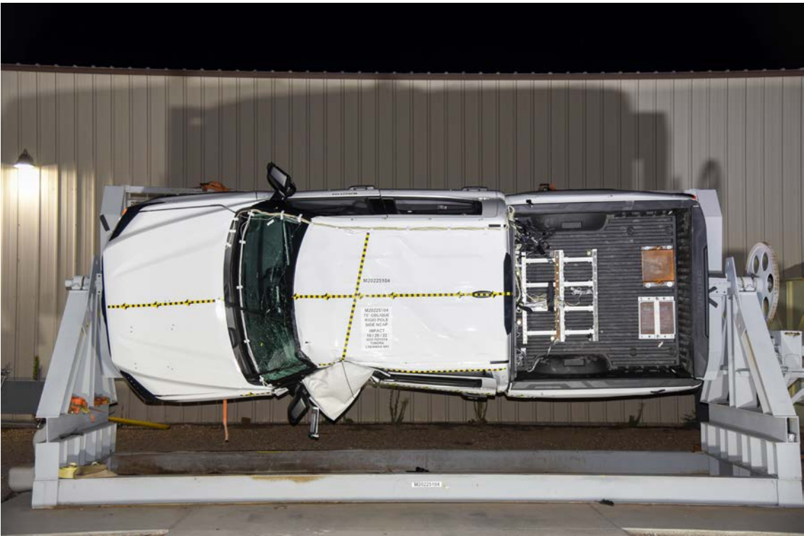
FIGURE 66. FMVSS No. 301 Static Rollover 90 Degrees
