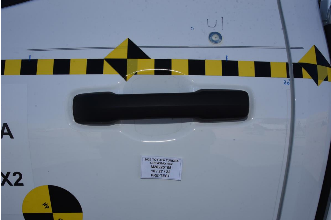
FIGURE 23. Pre-Test Left Rear Door Latch Close-Up
