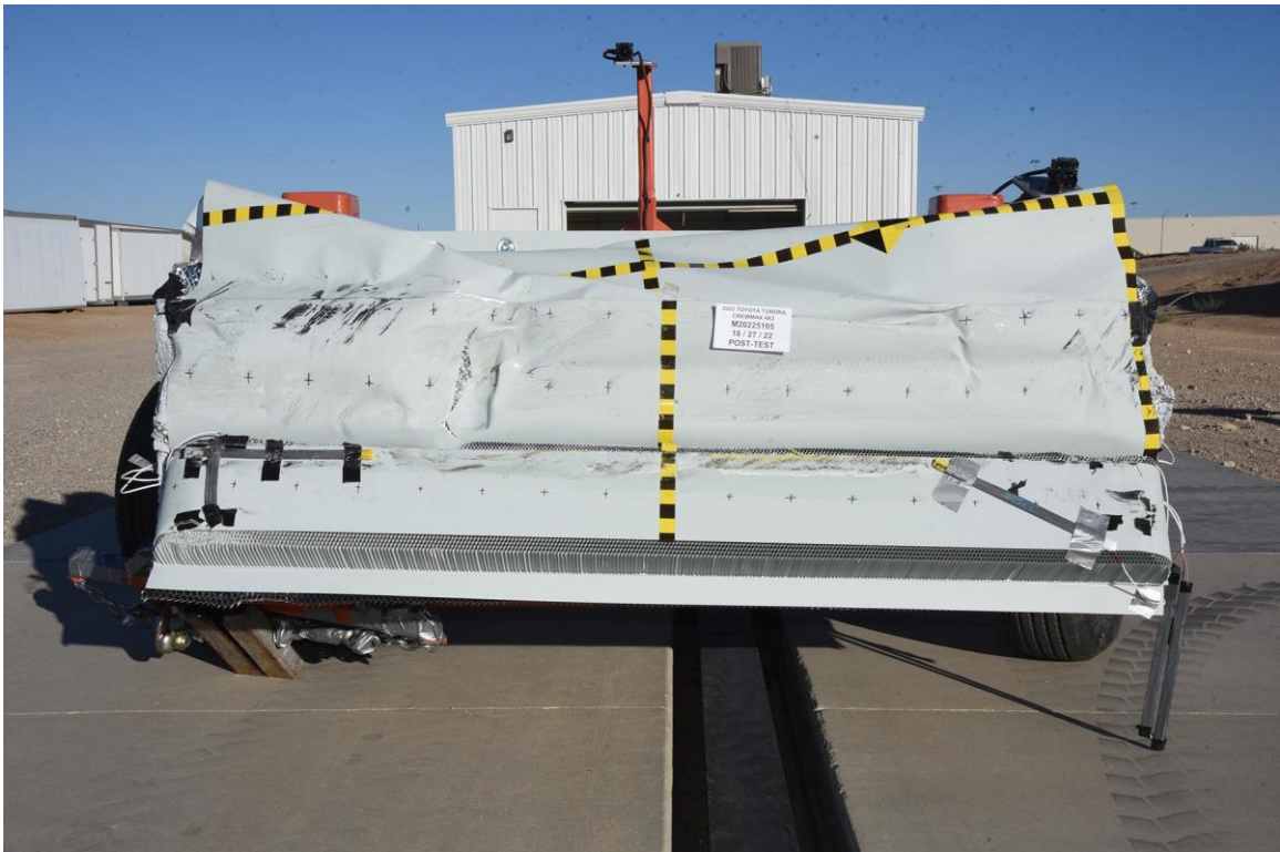
FIGURE 85. Post-Test Front View of MDB Impactor Face
