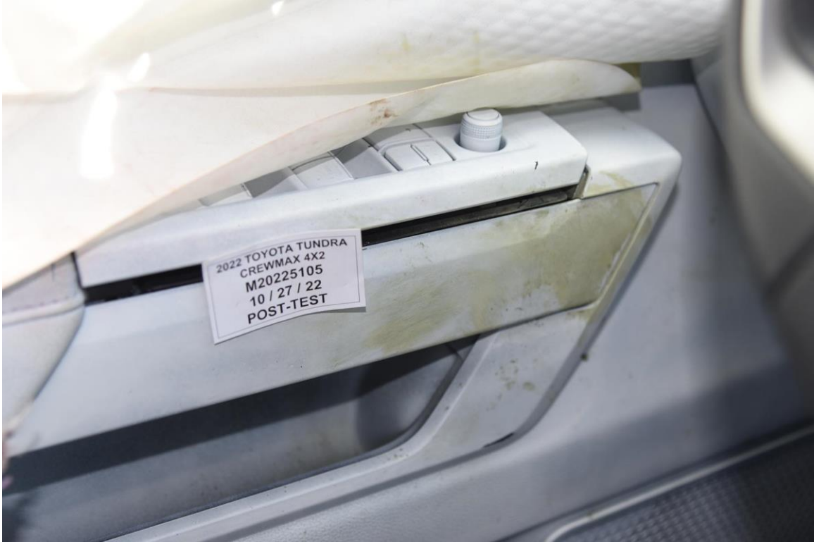
FIGURE 54. Post-Test Driver Dummy Close-Up Knee Contact View
