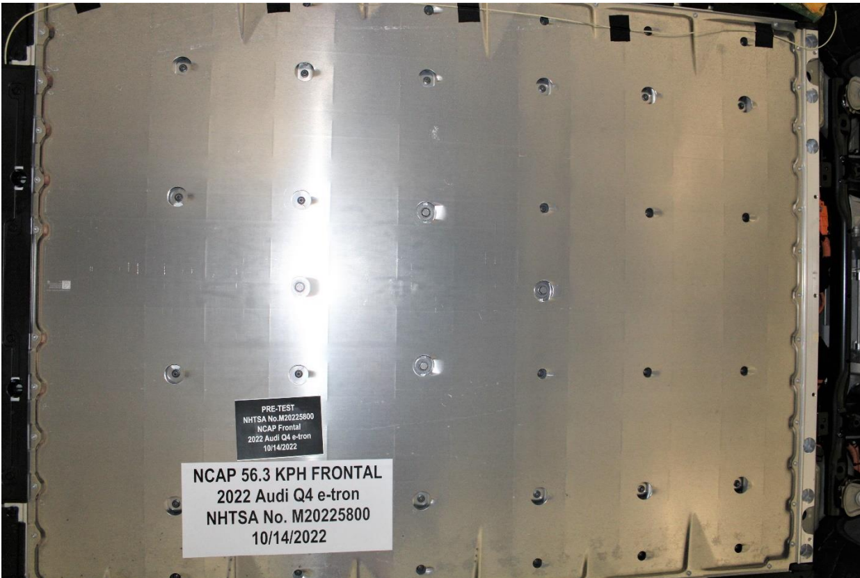
Figure 305-9: Pre-Impact View of Propulsion Battery
