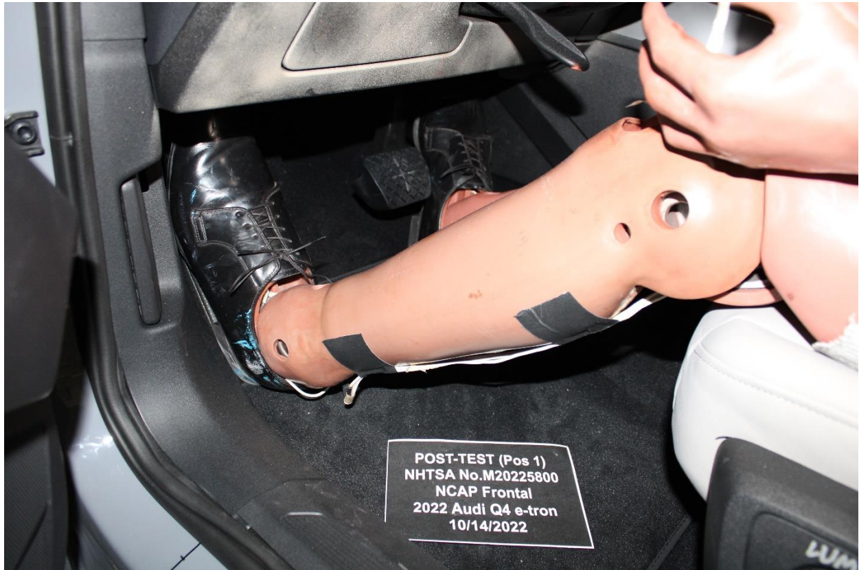
Figure A-43: Post-Test Driver Dummy Feet
