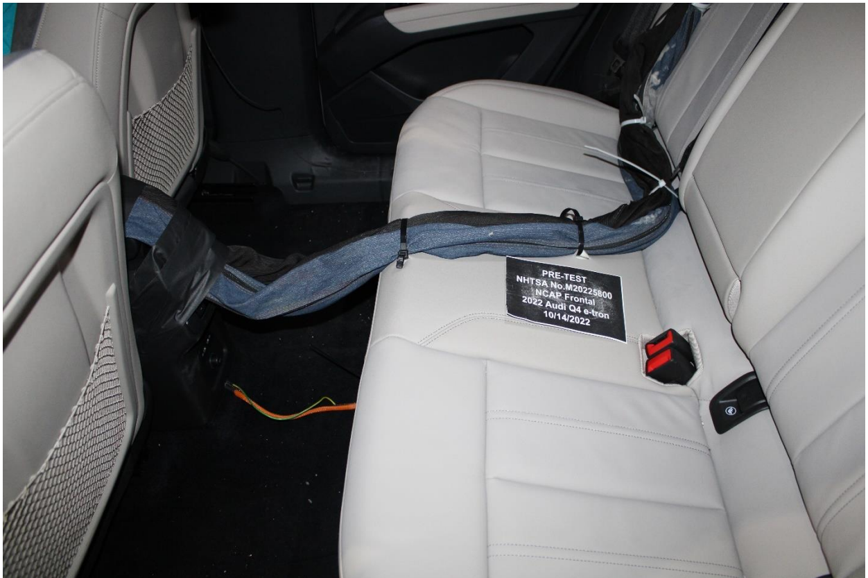
Figure A-28: Pre-Test Dummy Cable Routing
