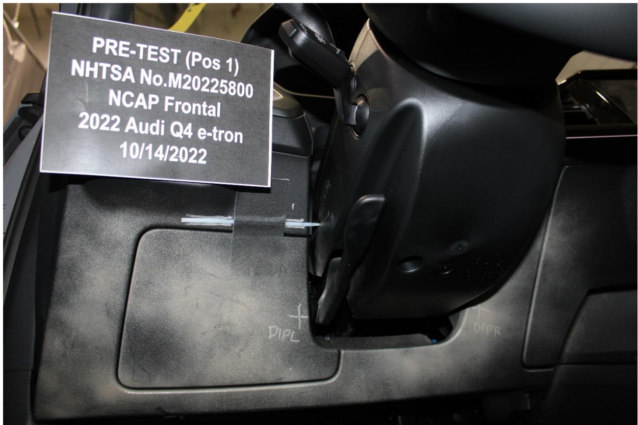
Figure A-44: Pre-Test Driver's Side Knee Bolster
