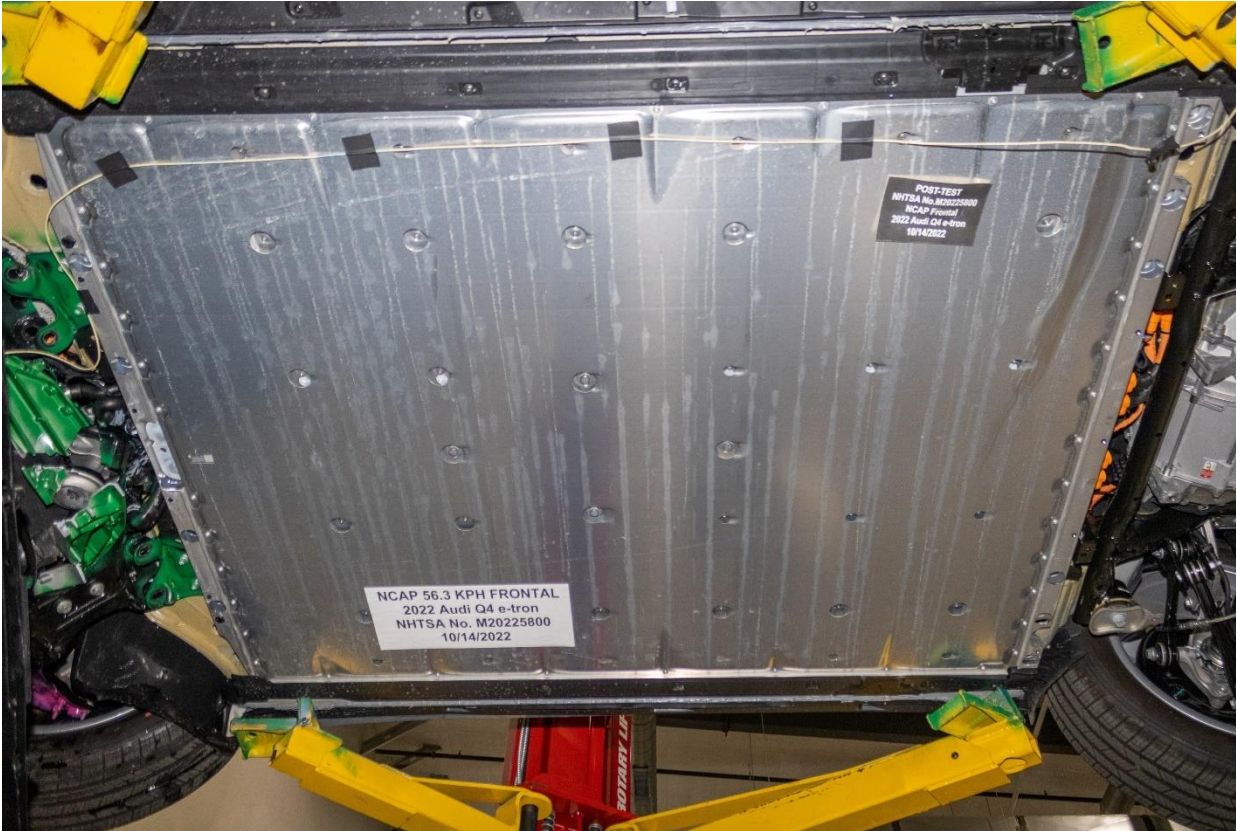
Figure 305-10: Post-Impact Front View of Propulsion Battery
