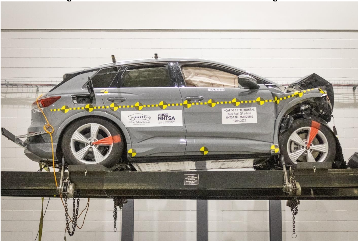
Figure 305-31: FMVSS No. 305 Static Rollover 360 Degrees
