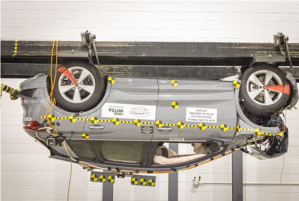
Figure 305-29: FMVSS No. 305 Static Rollover 180 Degrees
