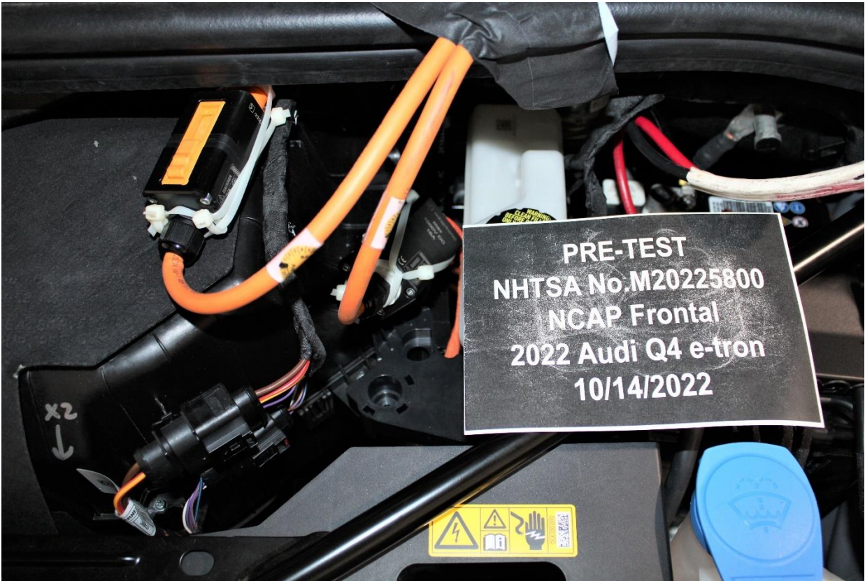
Figure 305-22: Pre-Impact View of High Voltage Leads Attached
