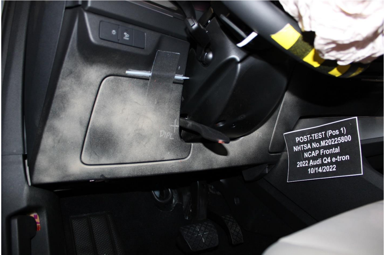
Figure A-45: Post-Test Driver's Side Knee Bolster
