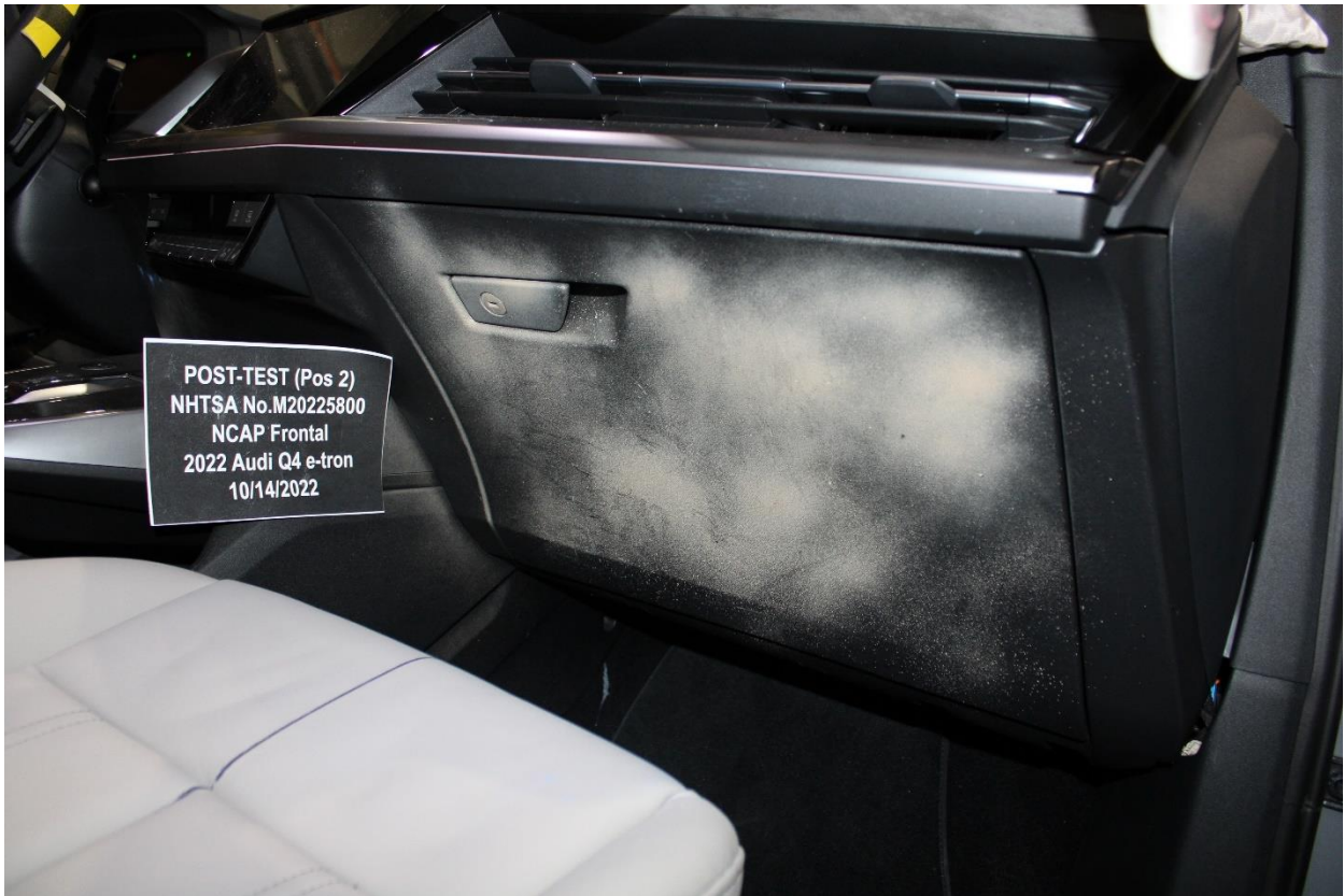
Figure A-68: Post-Test Passenger's Side Knee Bolster
