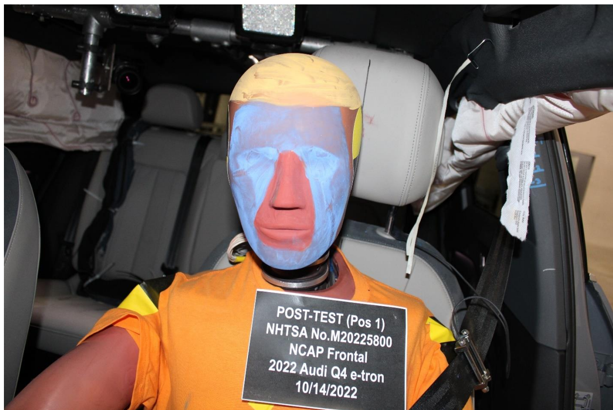
Figure A-48: Post-Test Driver Dummy Face
