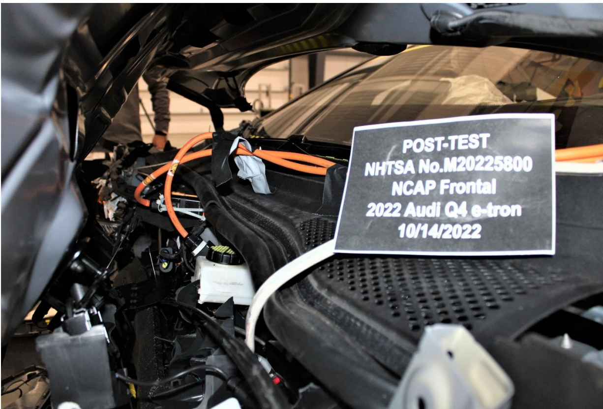
Figure 305-25: Post-Impact View of Installed Test Interface Port
