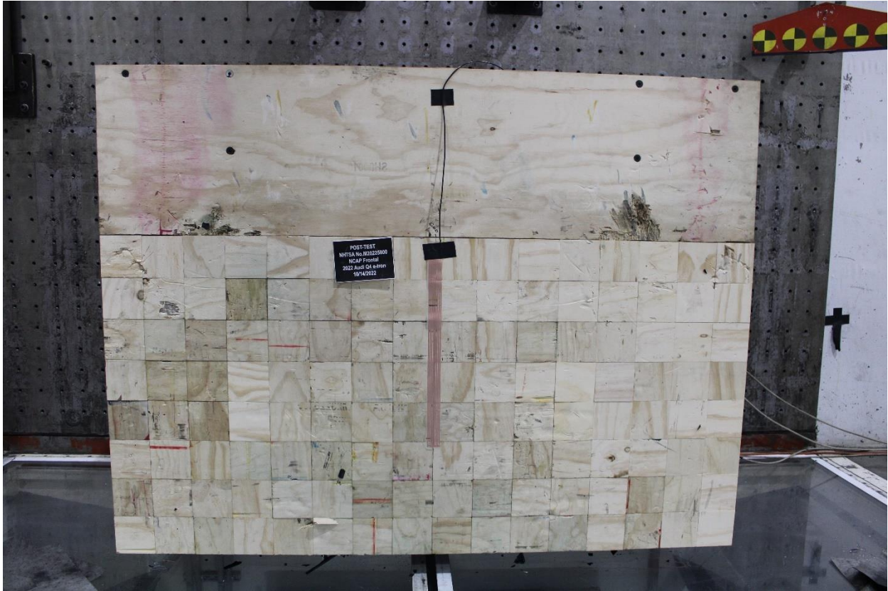
Figure A-3: Post-Test Load Cell Wall
