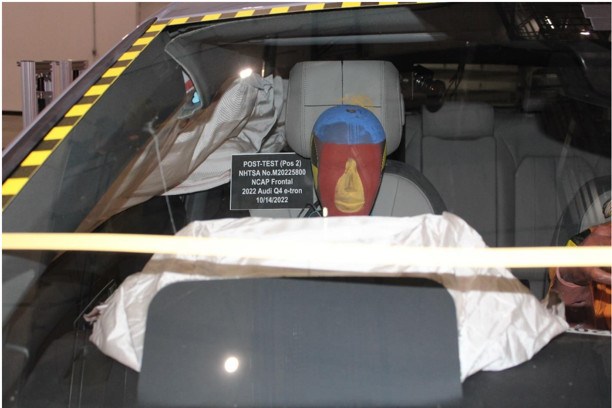
Figure A-54: Post-Test Passenger Dummy Front View
