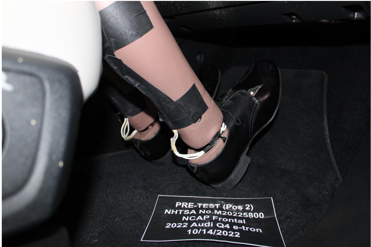
Figure A-65: Pre-Test Passenger Dummy Feet
