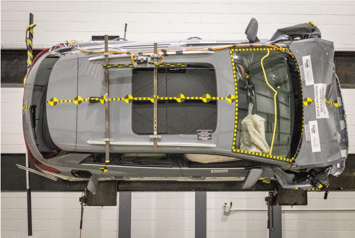
Figure 305-28: FMVSS No. 305 Static Rollover 90 Degrees
