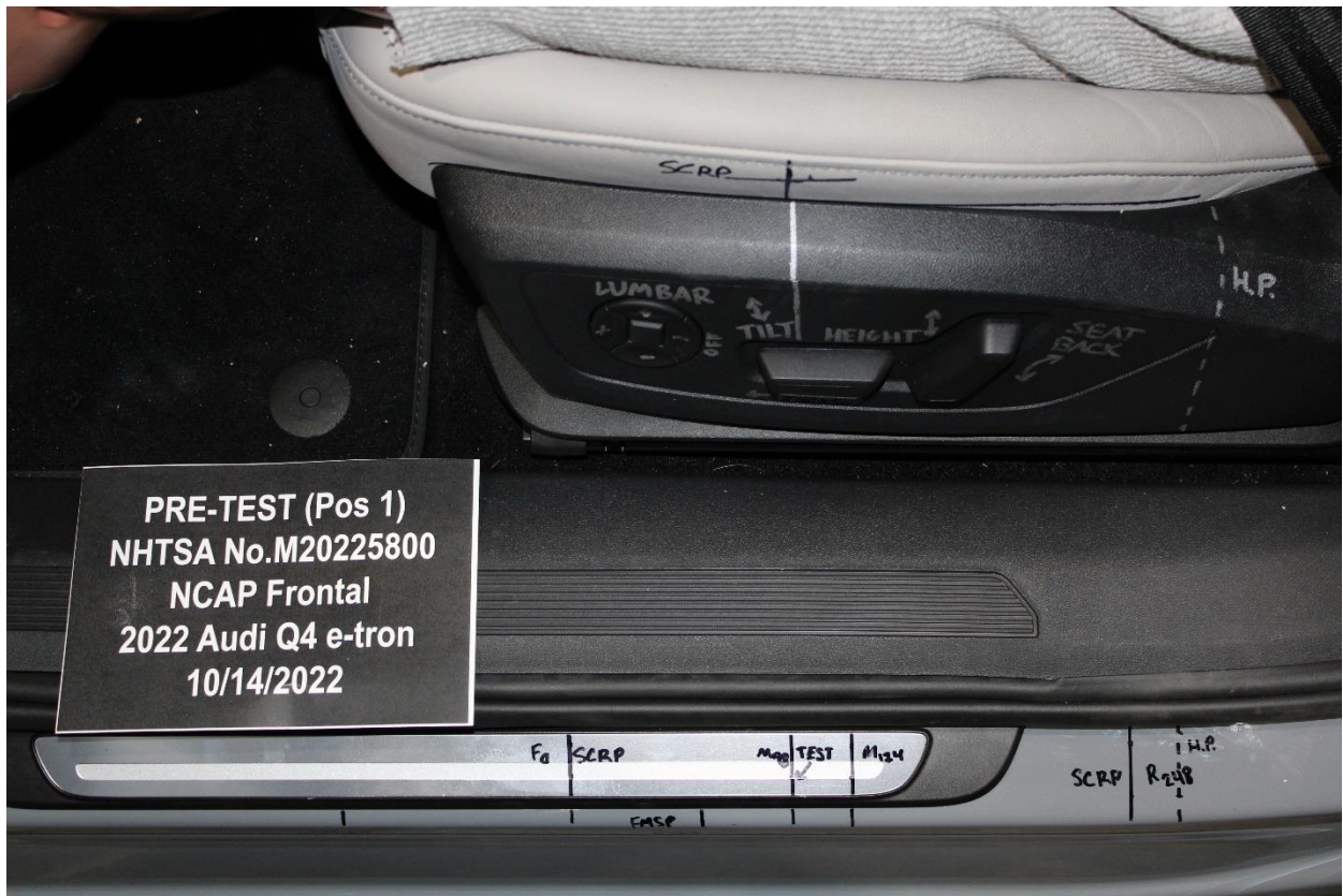
Figure A-36: Pre-Test Driver's Seat Fore-Aft Markings
