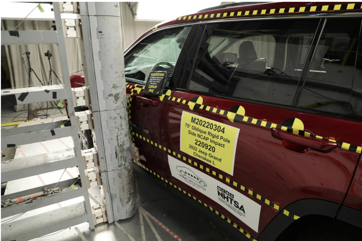
No. 018 Pre-Test Right Side View of Pole Positioned Against Side of Vehicle
