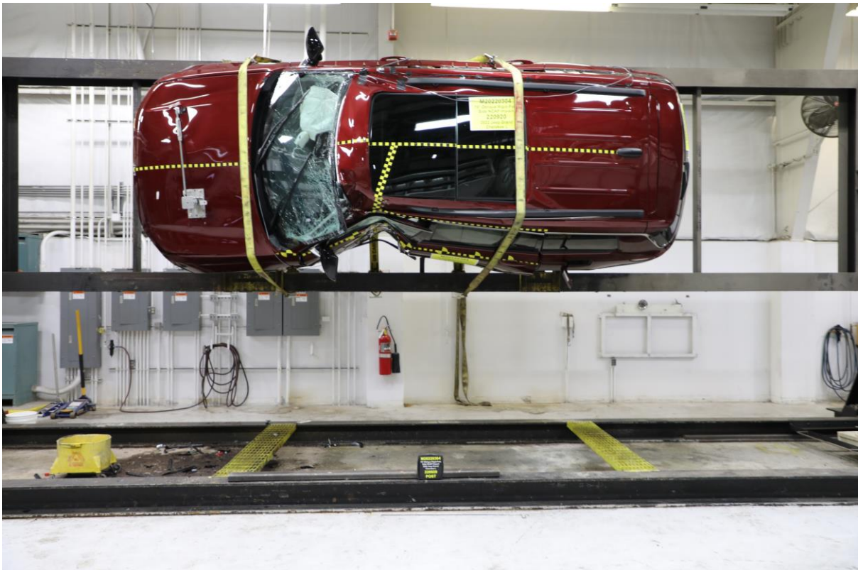
No. 066 FMVSS No. 301 Static Rollover 90 Degrees
