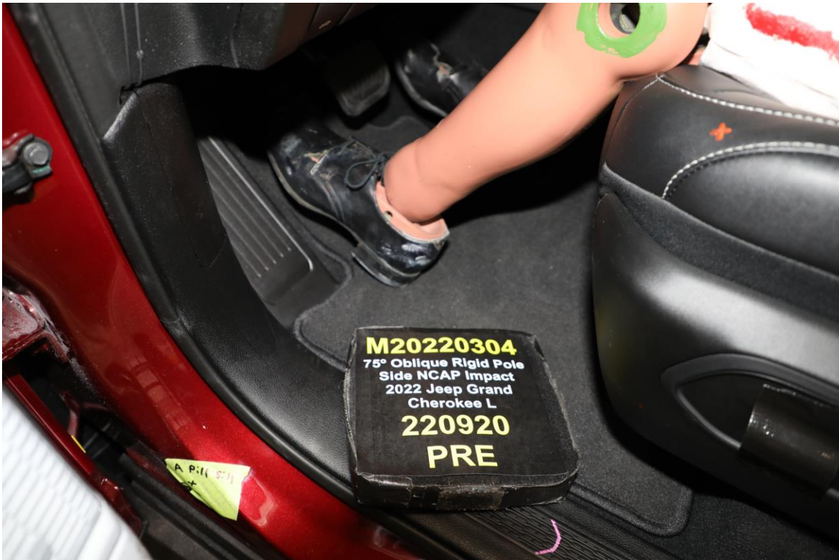
No. 032 Pre-Test Placement of Dummy Feet
