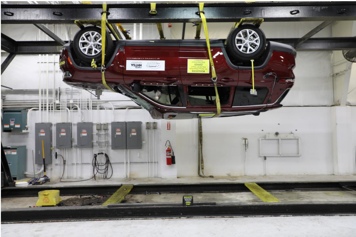
No. 067 FMVSS No. 301 Static Rollover 180 Degrees
