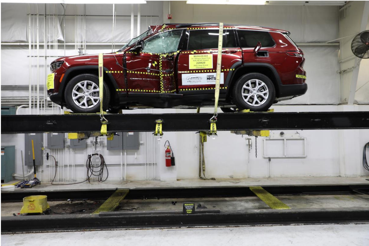
No. 069 FMVSS No. 301 Static Rollover 360 Degrees
