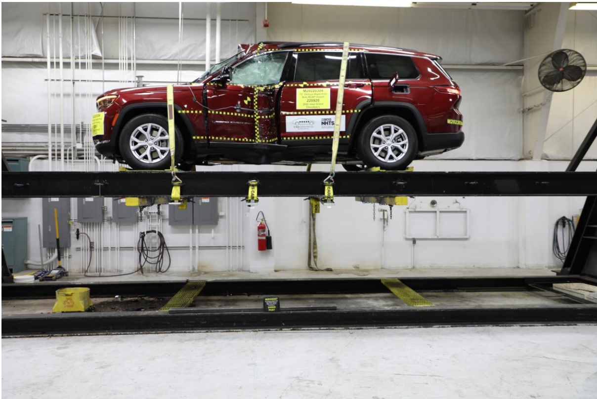
No. 065 FMVSS No. 301 Static Rollover 0 Degrees
