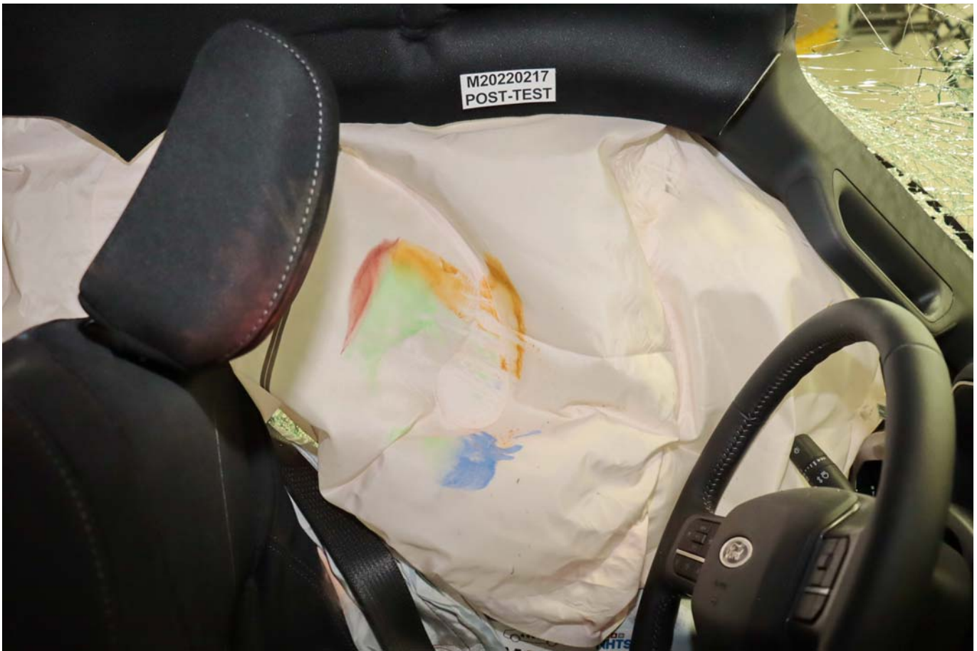
Photo No. 047 - Post-Test Dummy Close-Up Head Contact with Side Air Bag View
