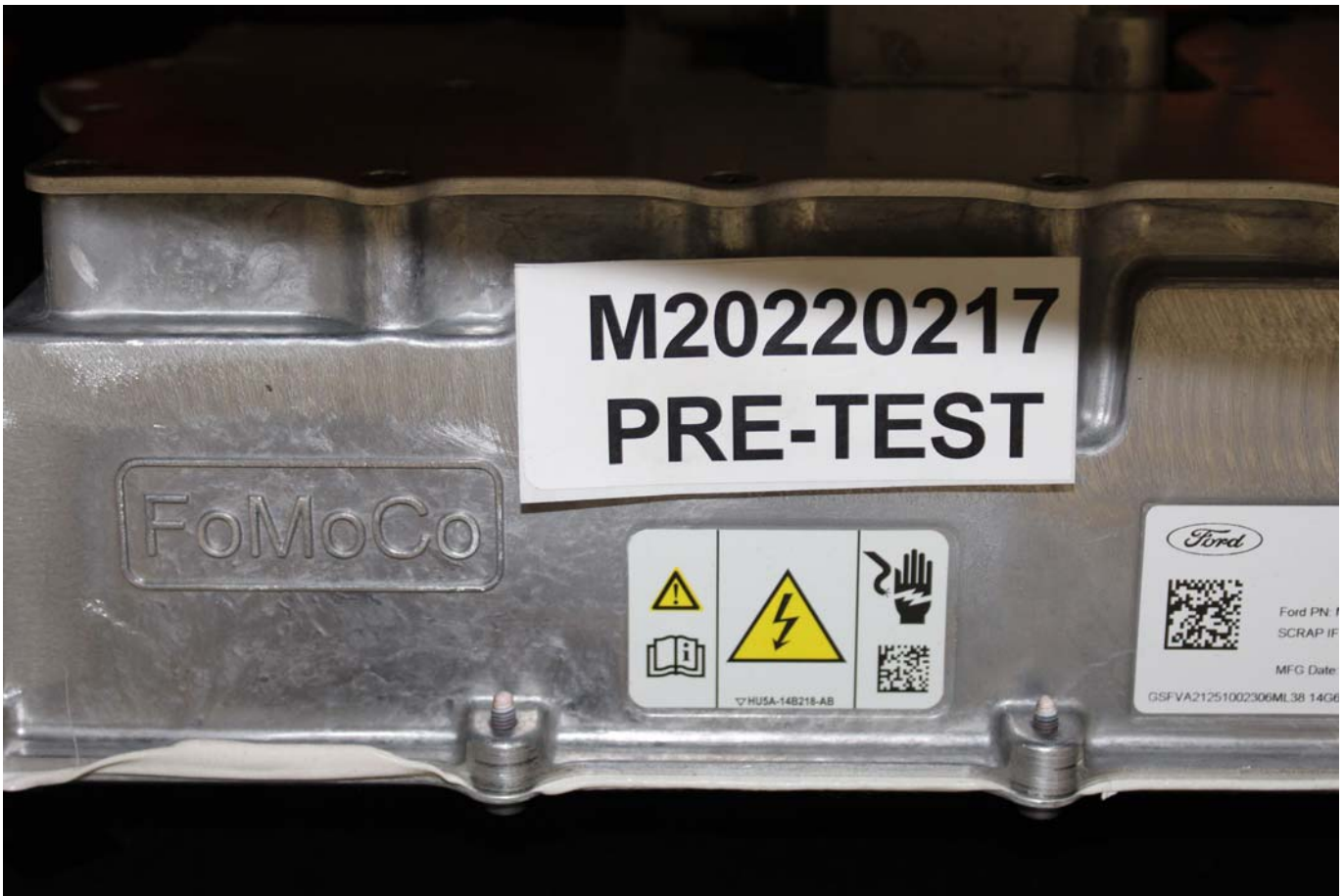
Photo No. 305-02 - Power Inverter Warning Label
