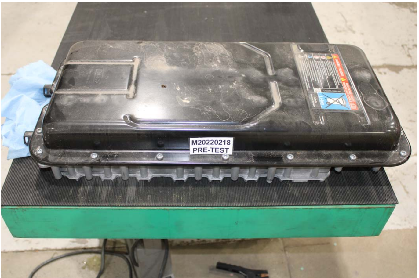
Photo No. 305-12 - Pre-Impact View of Battery Box(s) or Container(s) Which Holds Individual Battery Modules
