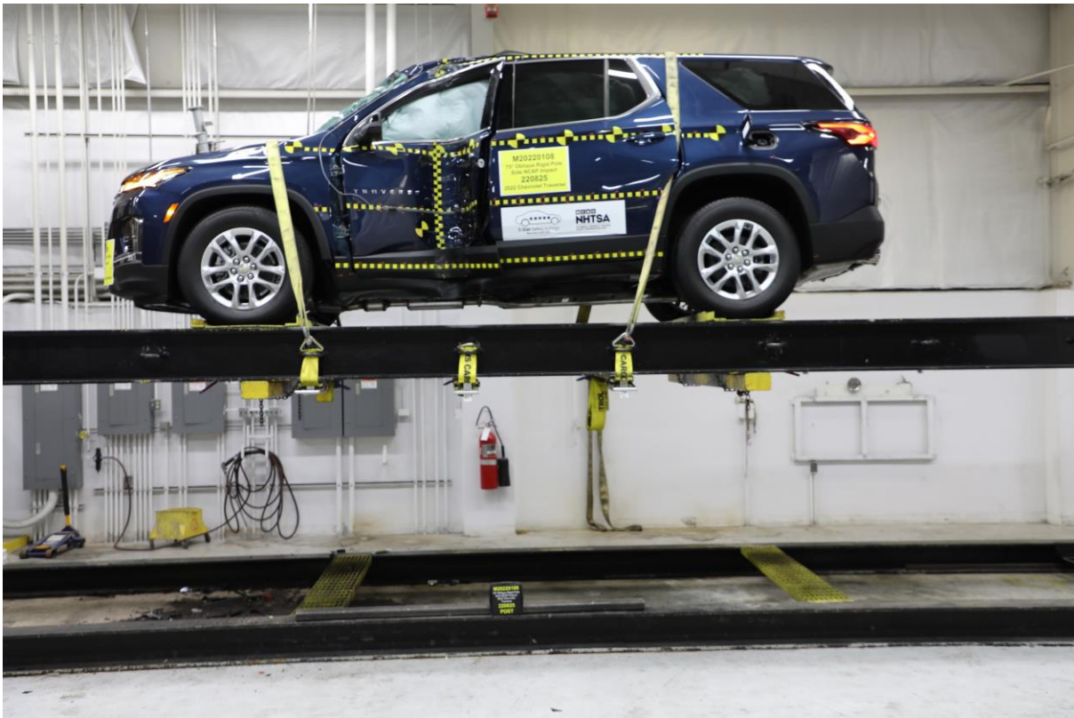
No. 065 FMVSS No. 301 Static Rollover 0 Degrees
