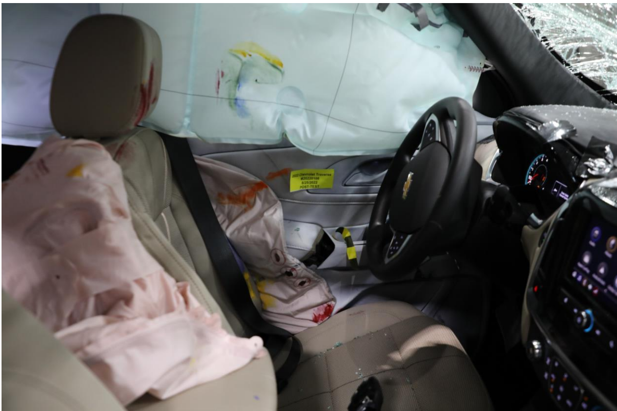
No. 045 Post-Test Inner Driver Door Panel View Showing Dummy Contact Location
