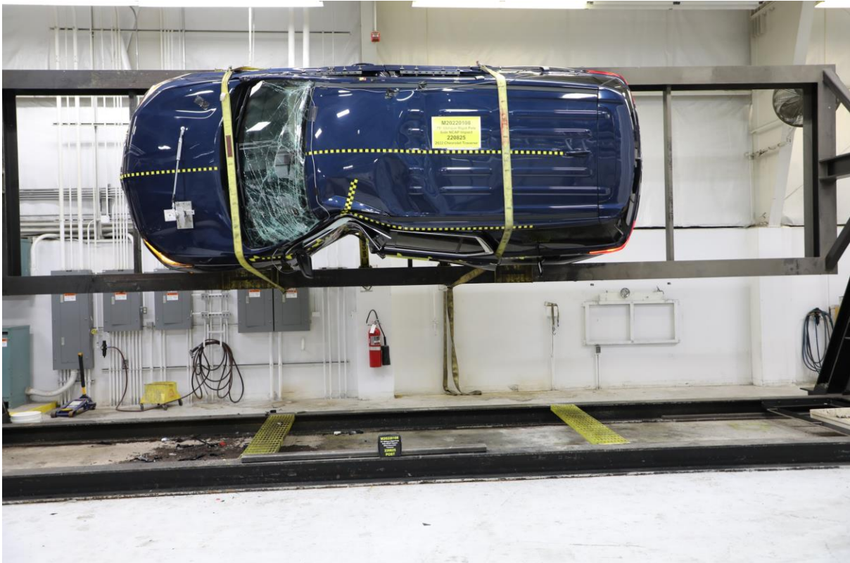
No. 066 FMVSS No. 301 Static Rollover 90 Degrees
