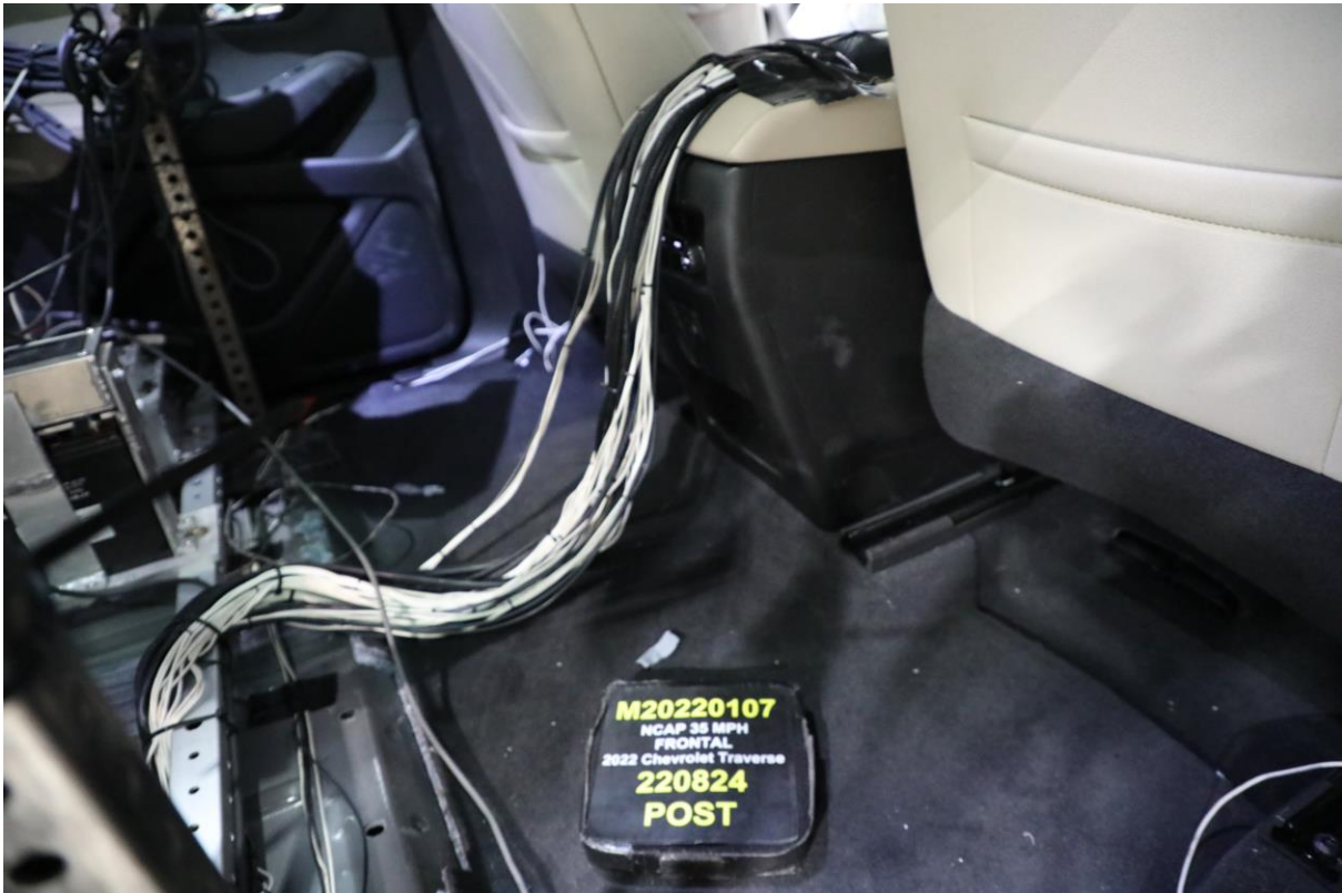
029 Post-Test Dummy Cable Routing
