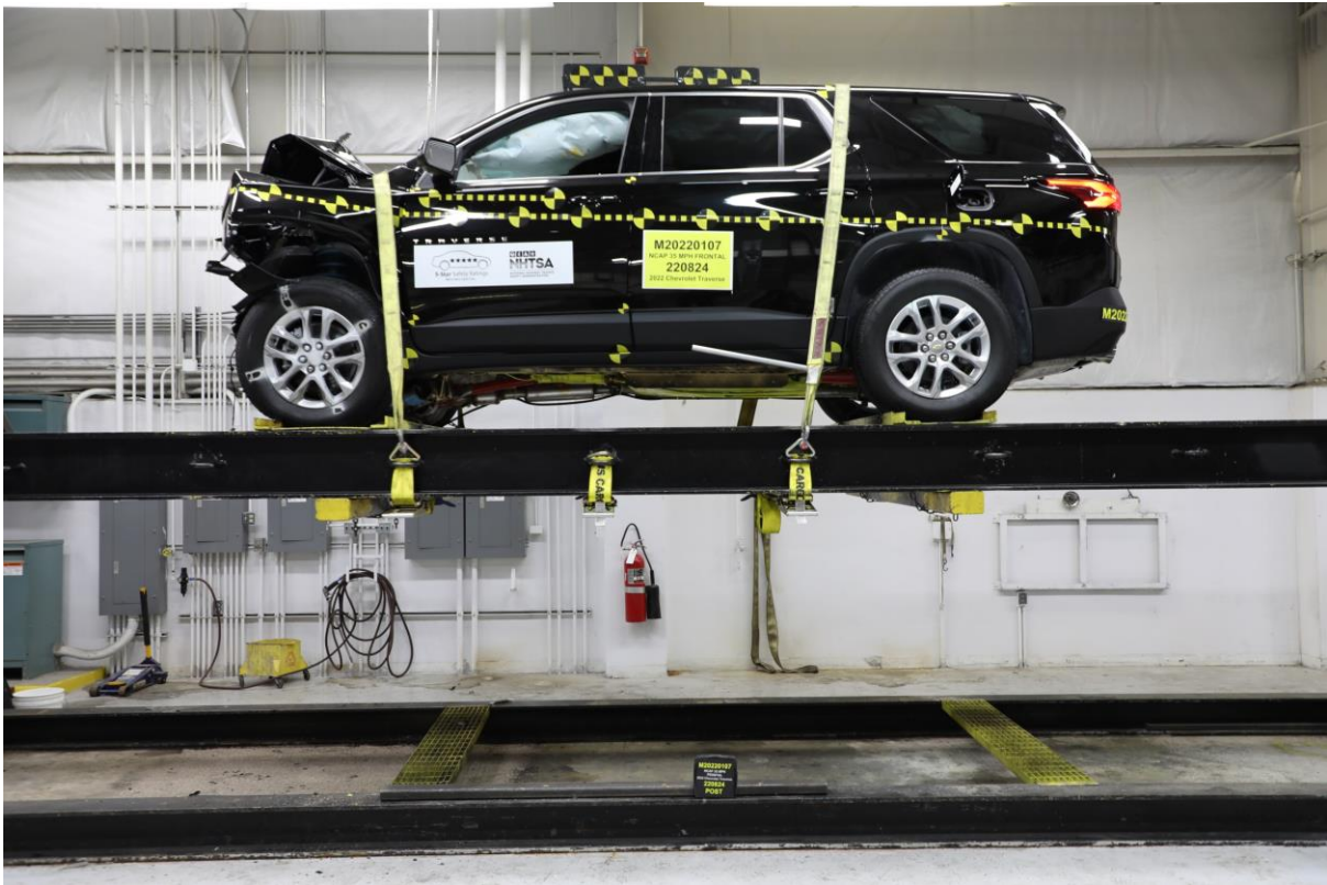
077 Vehicle at 0° on Static Rollover Device
