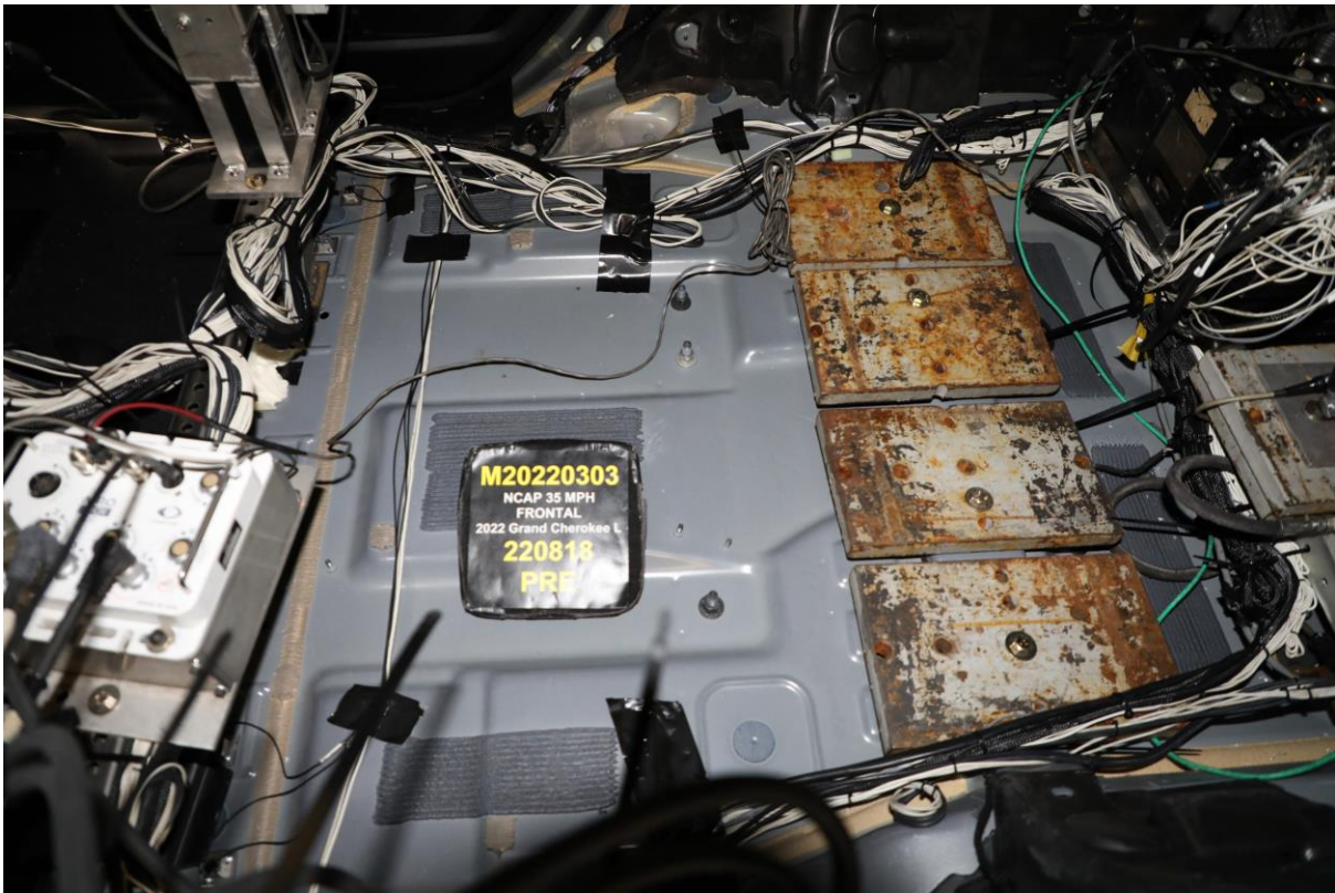
028 Pre-Test Dummy Cable Routing
