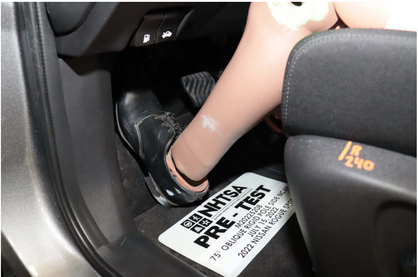
Photo No. 032 - Pre-Test Placement of Dummy's Feet
