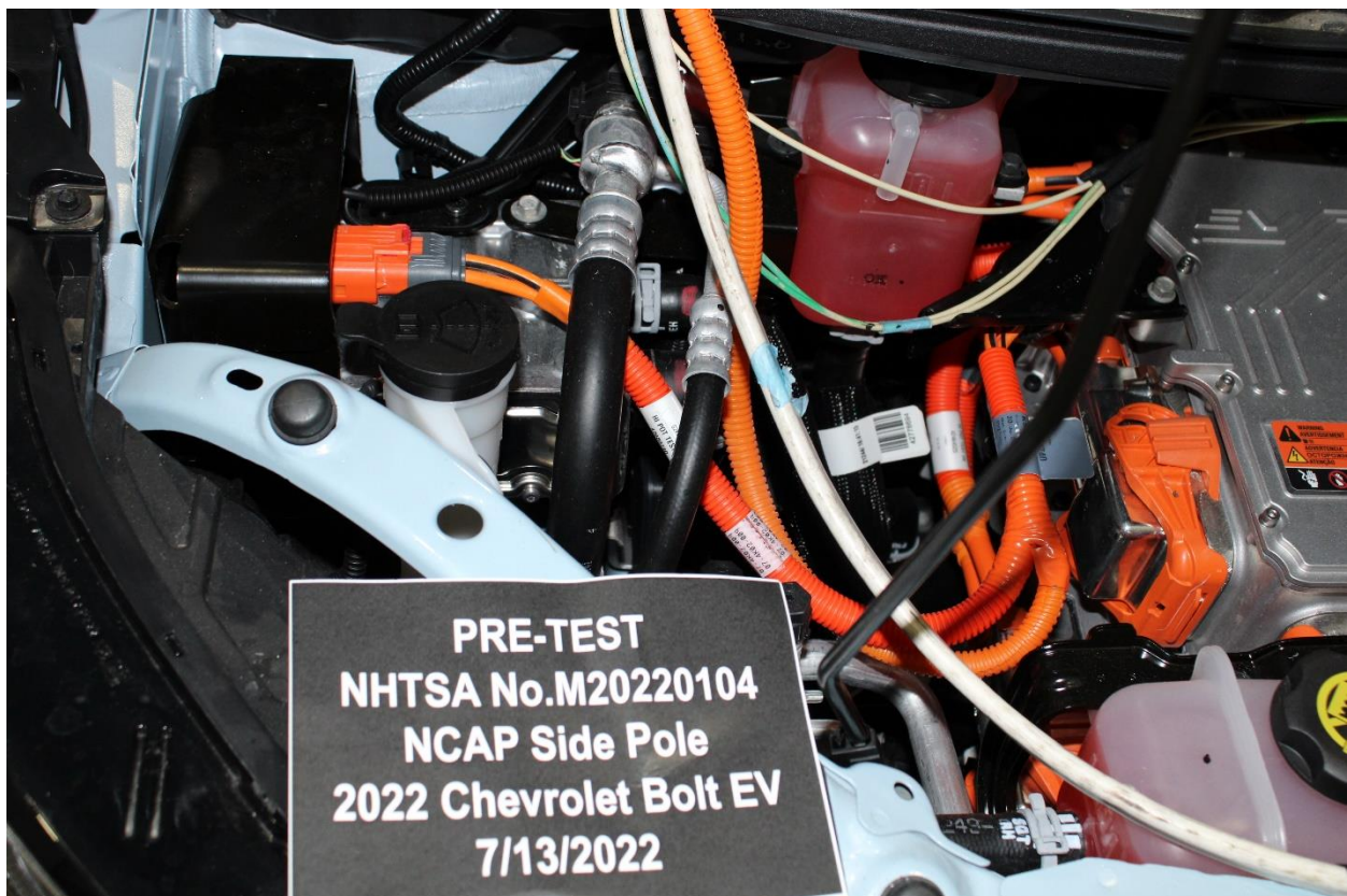
Figure 305-22: Pre-Impact View of High Voltage Leads Attached
