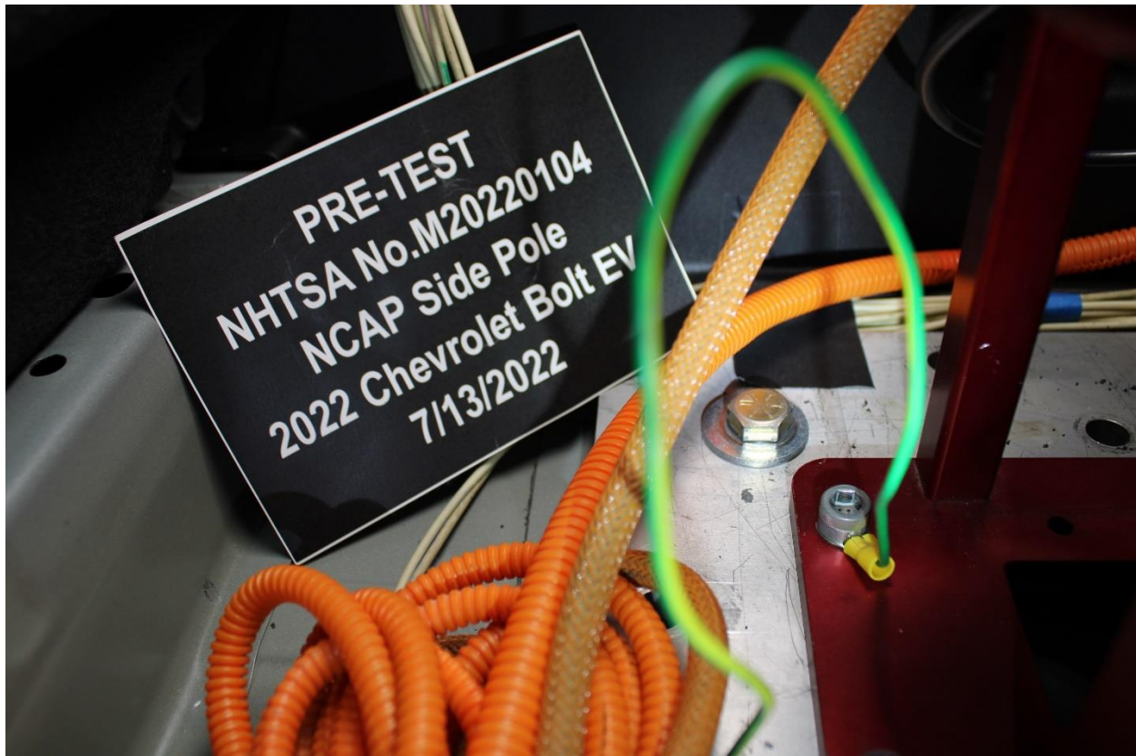
Figure 305-21: Pre-Impact View of Ground Lead Attached
