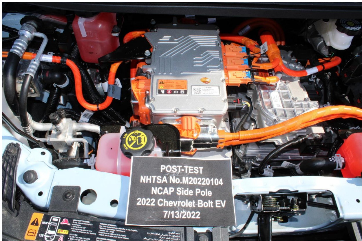
Figure 305-17: Post-Impact View of Electric Propulsion Drive
