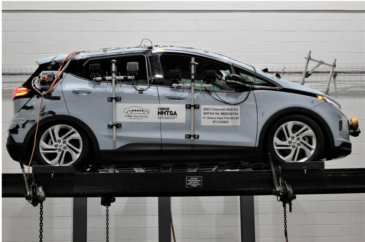
Figure 305-31: FMVSS No. 305 Static Rollover 360 Degrees
