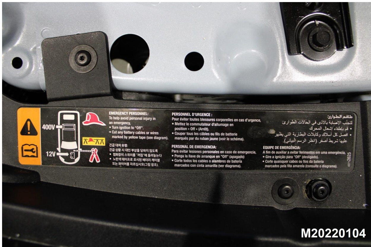
Figure 305-5: Other Vehicle Label Related to Electric Propulsion System
