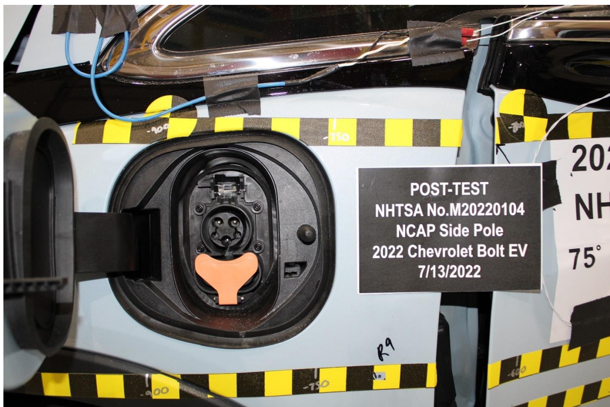
Figure A-56: Post-Test View of Charging Port
