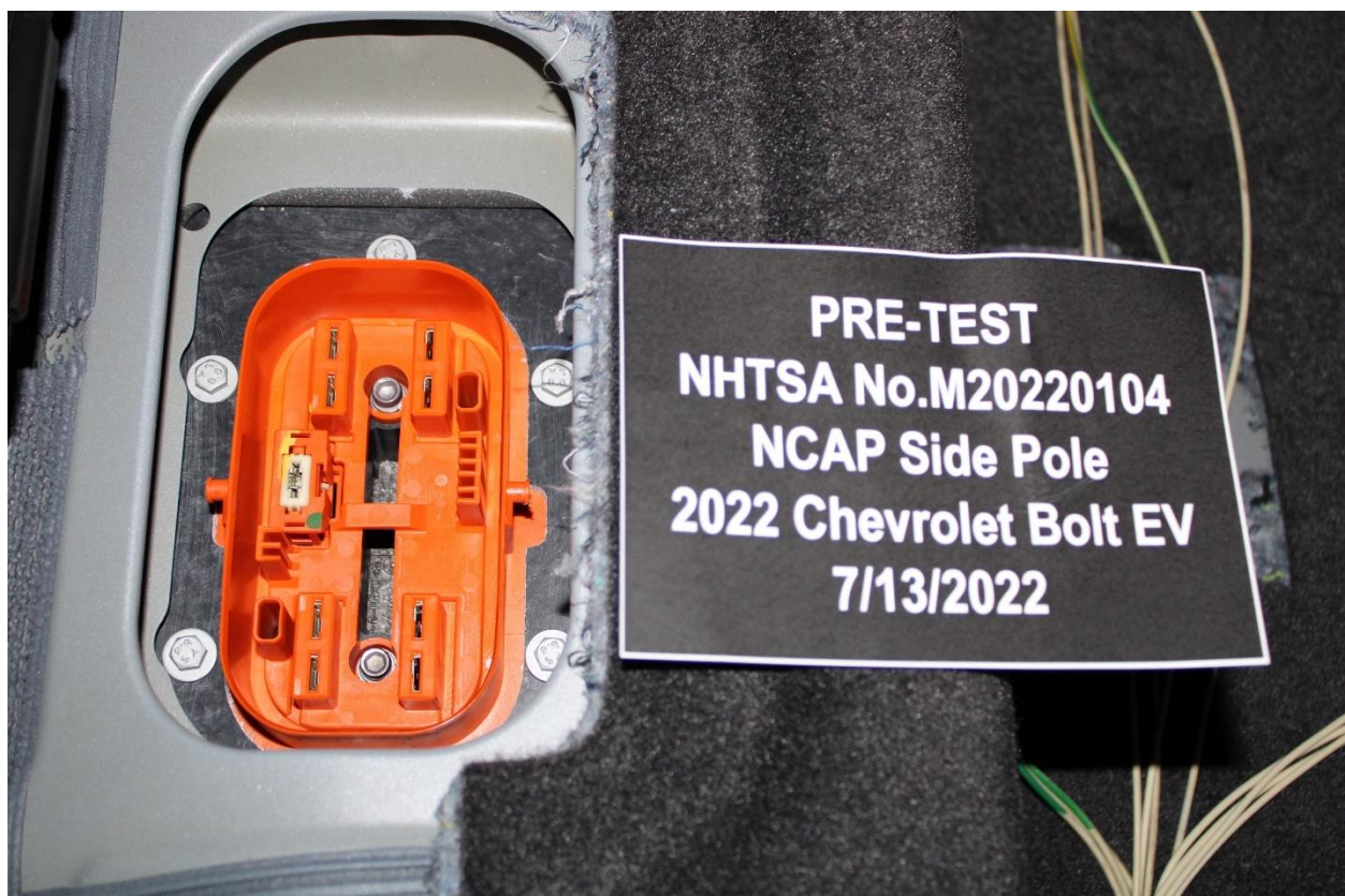
Figure 305-8: Manual High Voltage Service Disconnect Removed Location
