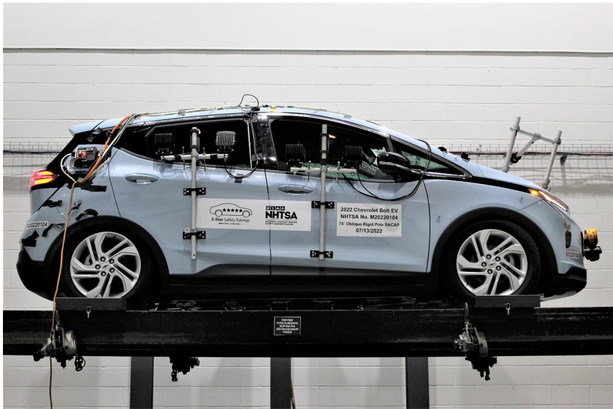
Figure A-65: FMVSS No. 301 Static Rollover 0 Degrees
