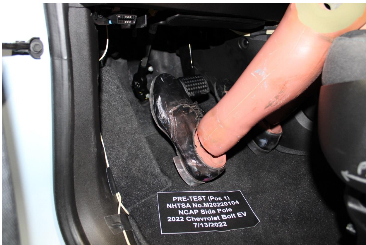
Figure A-32: Pre-Test Placement of Dummy's Feet
