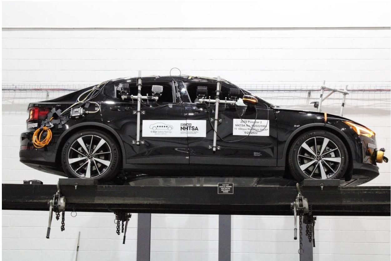
Figure A-65: FMVSS No. 301 Static Rollover 0 Degrees
