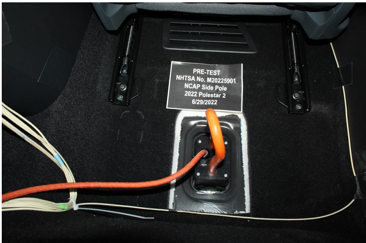
Figure 305-18: Pre-Impact View of High Voltage Interconnects
