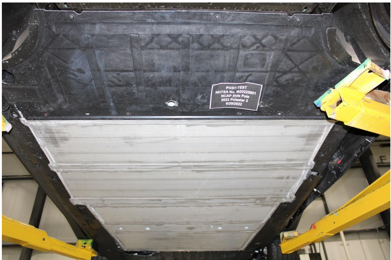
Figure 305-10: Post-Impact Front View of Propulsion Battery
