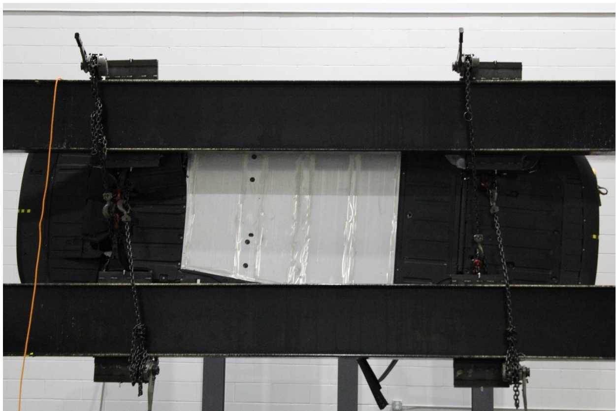
Figure A-66: FMVSS No. 301 Static Rollover 90 Degrees
