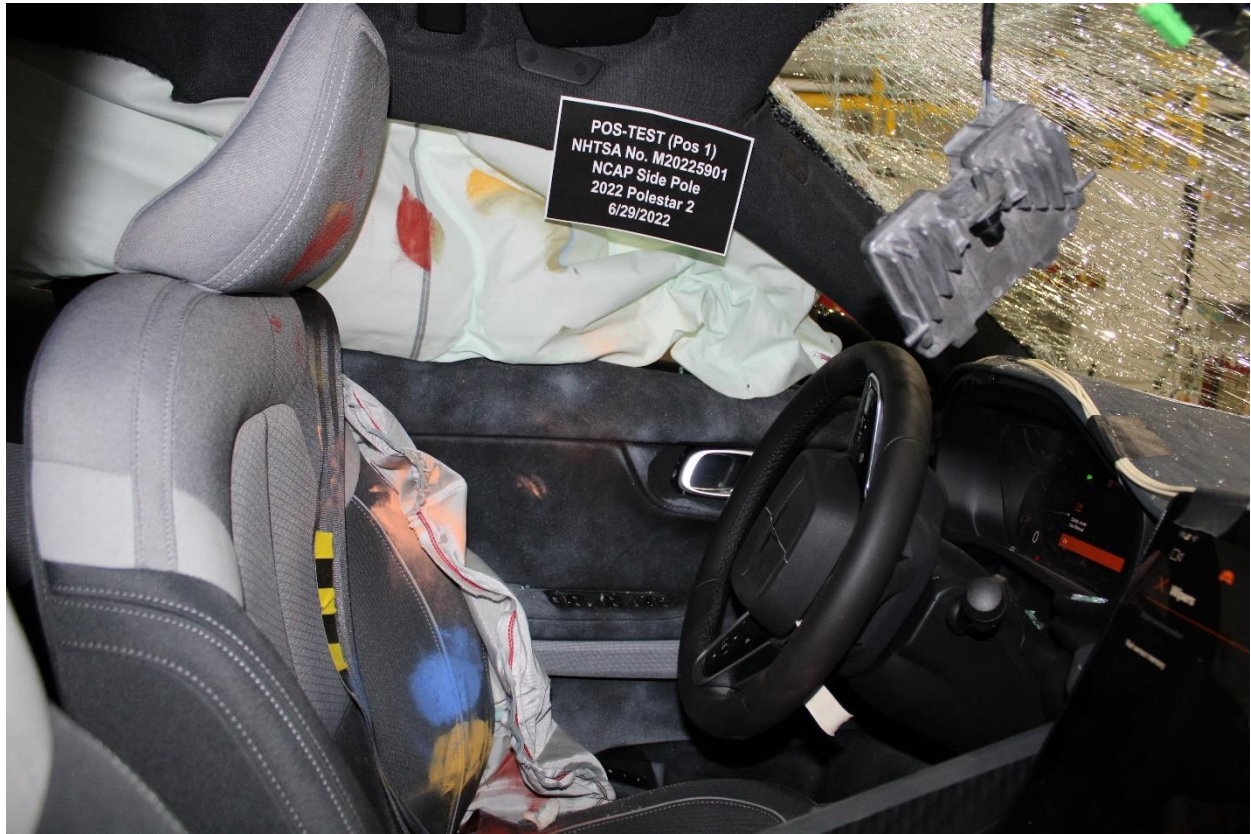
Figure A-73: Post-Test View of Shattered Vehicle Inner Door Panel
