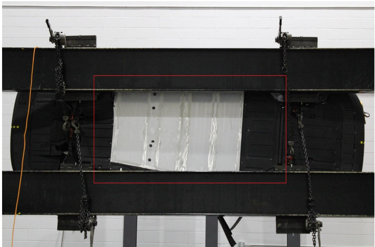
Figure 305-28: FMVSS No. 305 Static Rollover 90 Degrees
