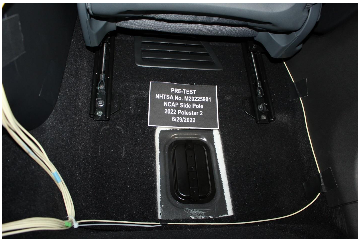
Figure 305-8: Manual High Voltage Service Disconnect Removed Location
