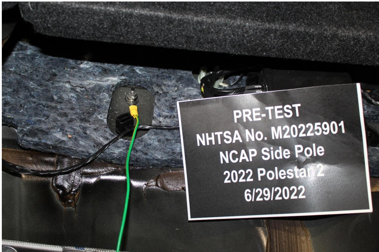
Figure 305-21: Pre-Impact View of Ground Lead Attached
