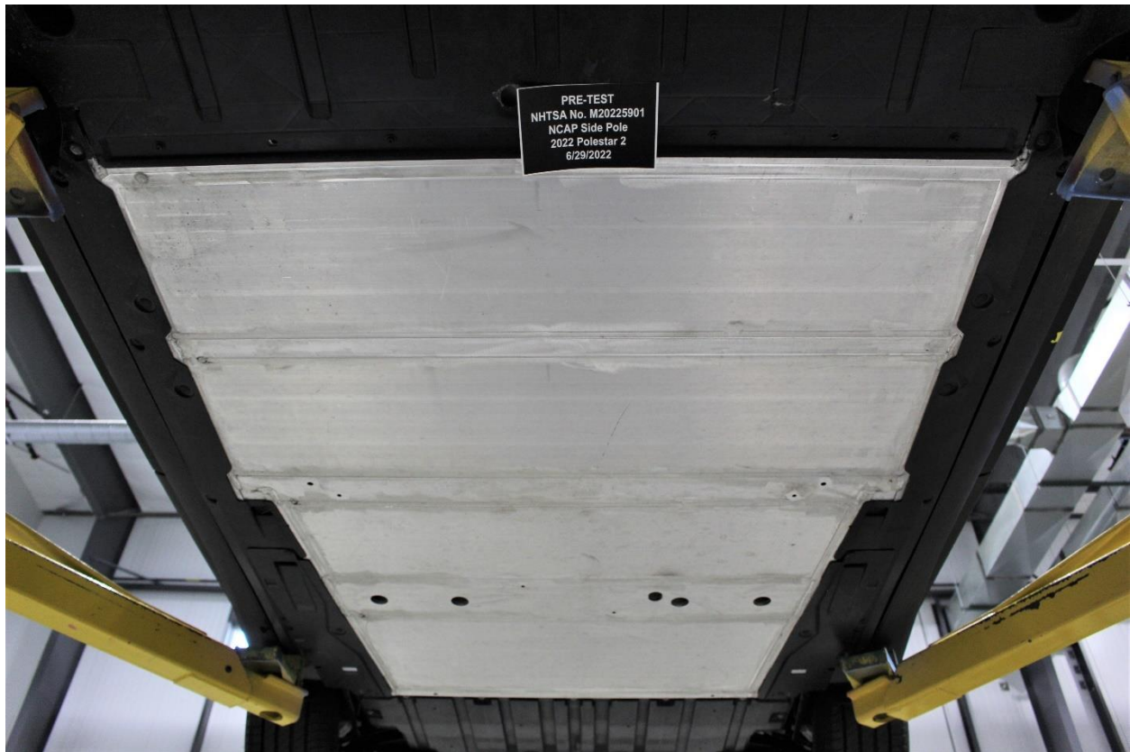
Figure 305-9: Pre-Impact View of Propulsion Battery
