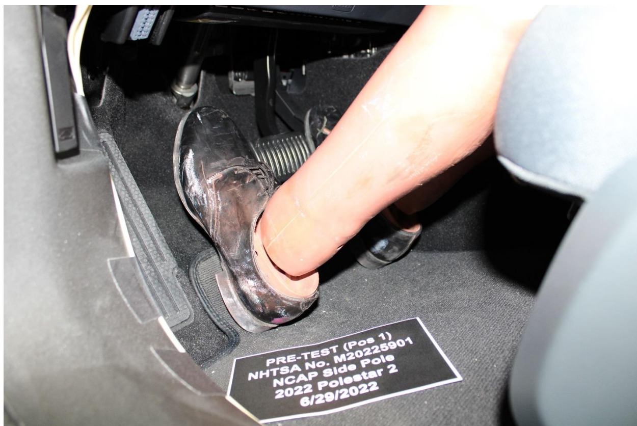
Figure A-32: Pre-Test Placement of Dummy's Feet
