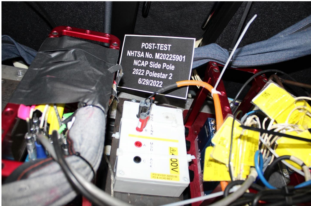
Figure 305-25: Post-Impact View of Installed Test Interface Port
