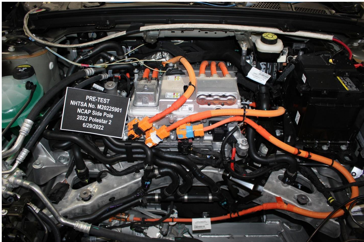
Figure 305-16: Pre-Impact View of Electric Propulsion Drive
