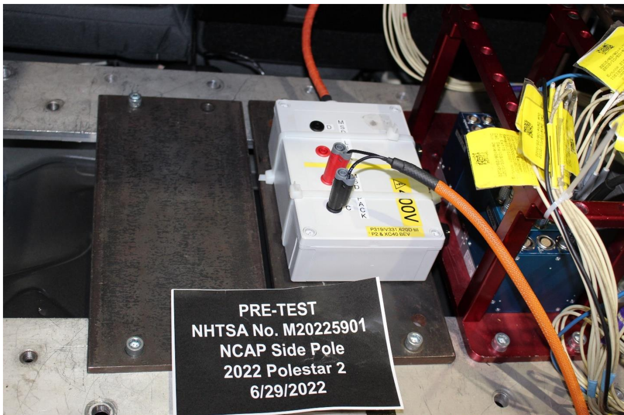
Figure 305-22: Pre-Impact View of High Voltage Leads Attached
