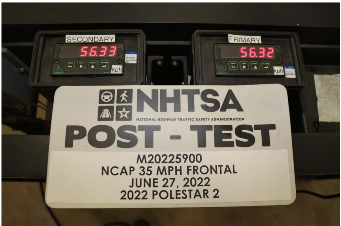
Photo No. 076 - Post-Test Speed Trap Read-Out
