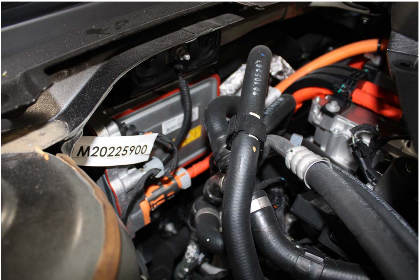
Photo No. 305-02 - Power Inverter Warning Label
