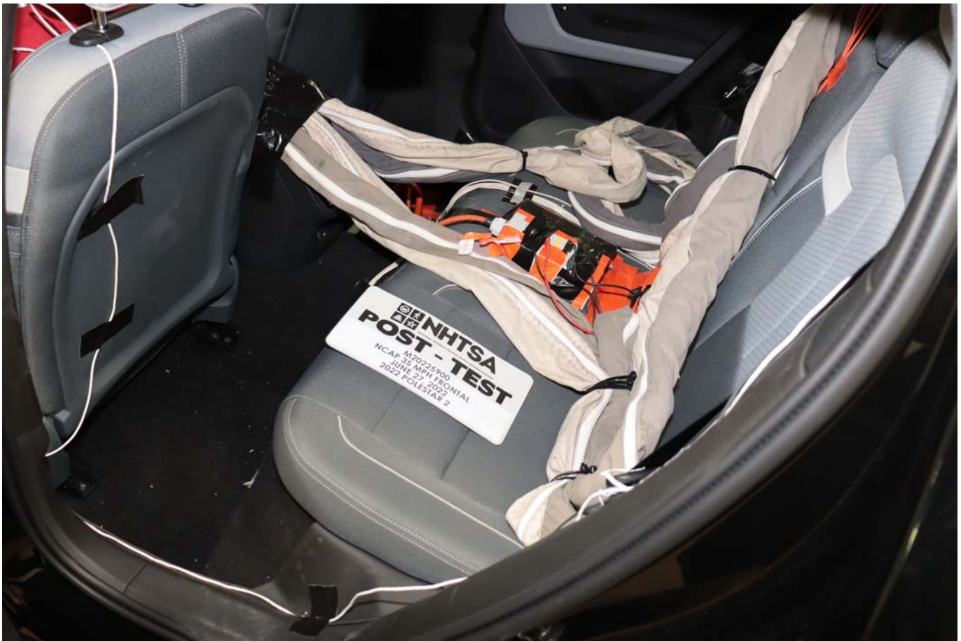
Photo No. 029 - Post-Test Dummy Cable Routing
