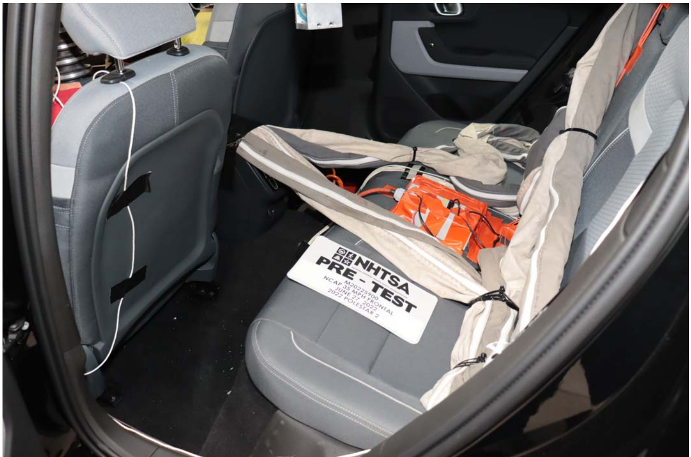
Photo No. 028 - Pre-Test Dummy Cable Routing
