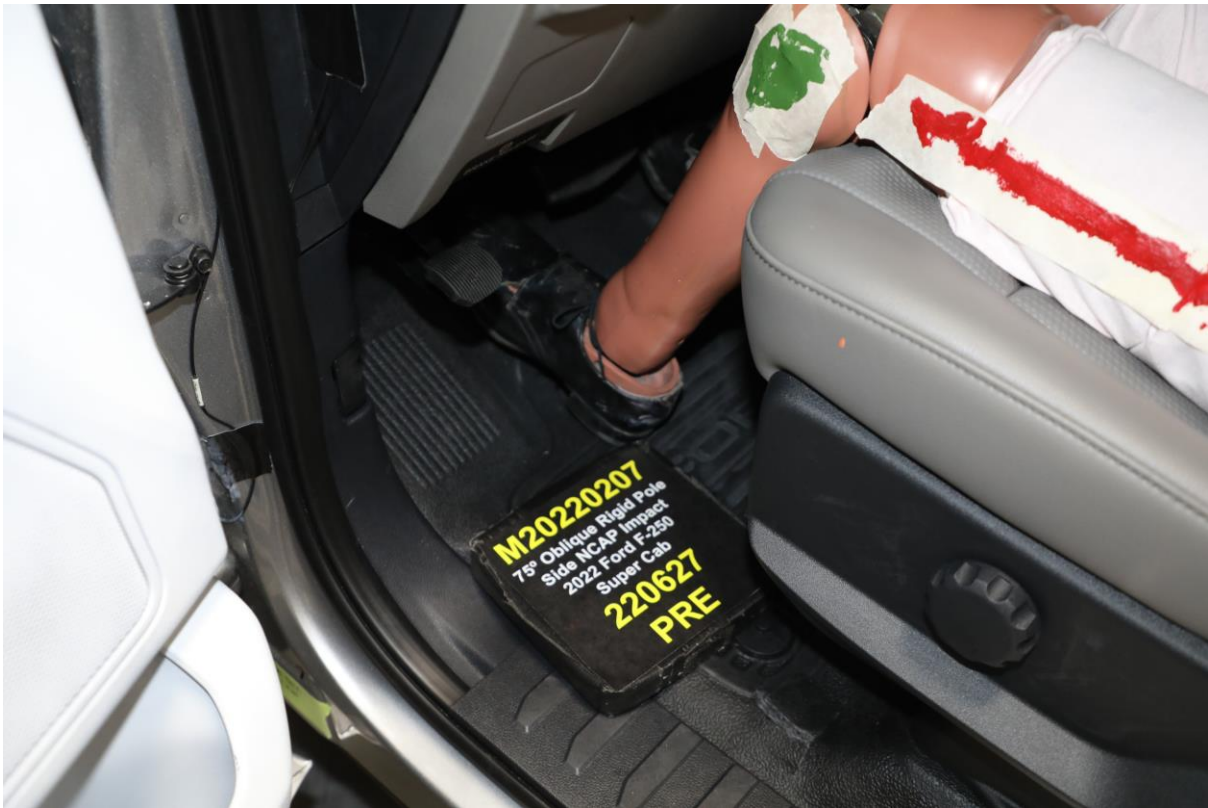
No. 032 Pre-Test Placement of Dummy Feet
