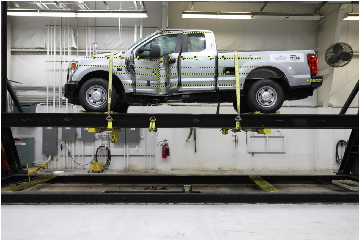
No. 069 FMVSS No. 301 Static Rollover 360 Degrees
