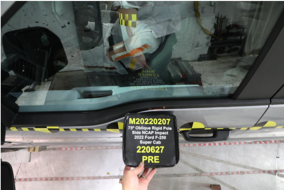
No. 040 Pre-Test Dummy and Door Clearance View
