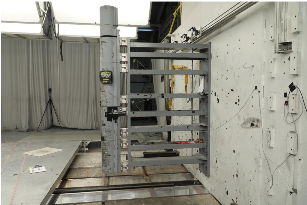
No. 062 Post-Test Pole Barrier Side View
