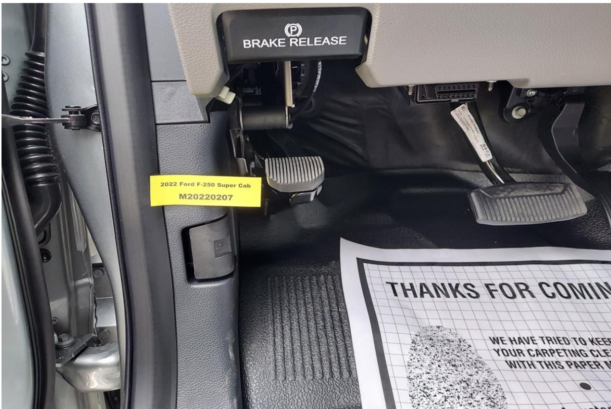
No. 035 Pre-Test View of Disengaged Parking Brake
