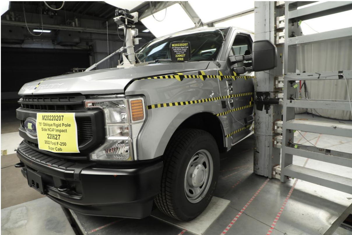
No. 017 Pre-Test Left Side View of Pole Positioned Against Side of Vehicle
