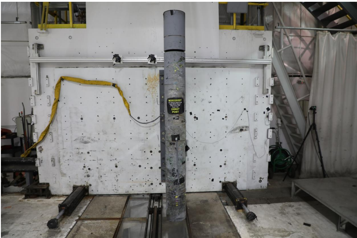
No. 060 Post-Test Pole Barrier Front View
