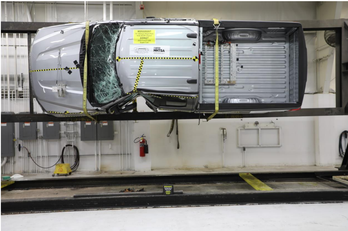
No. 066 FMVSS No. 301 Static Rollover 90 Degrees
