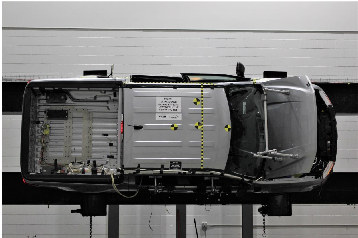
Figure A-99: FMVSS No. 301 Static Rollover 270 Degrees
