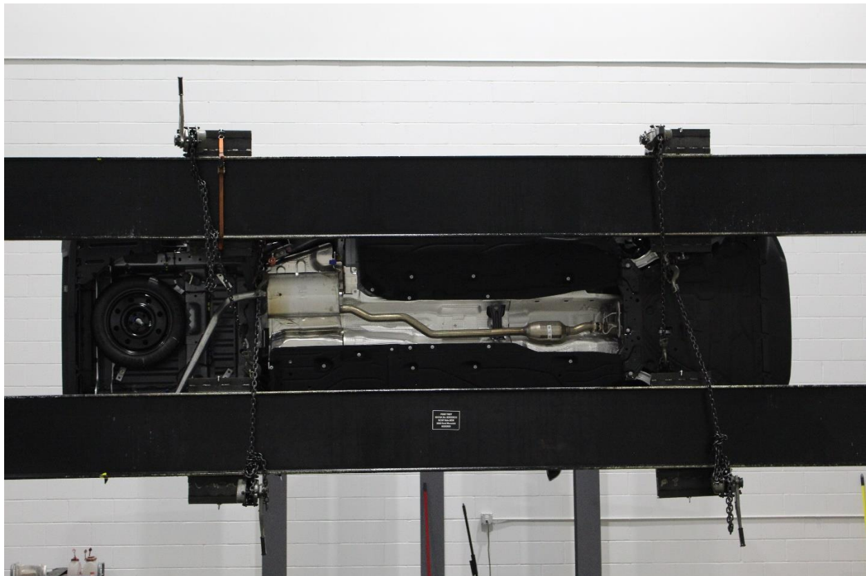
Figure A-97: FMVSS No. 301 Static Rollover 90 Degrees
