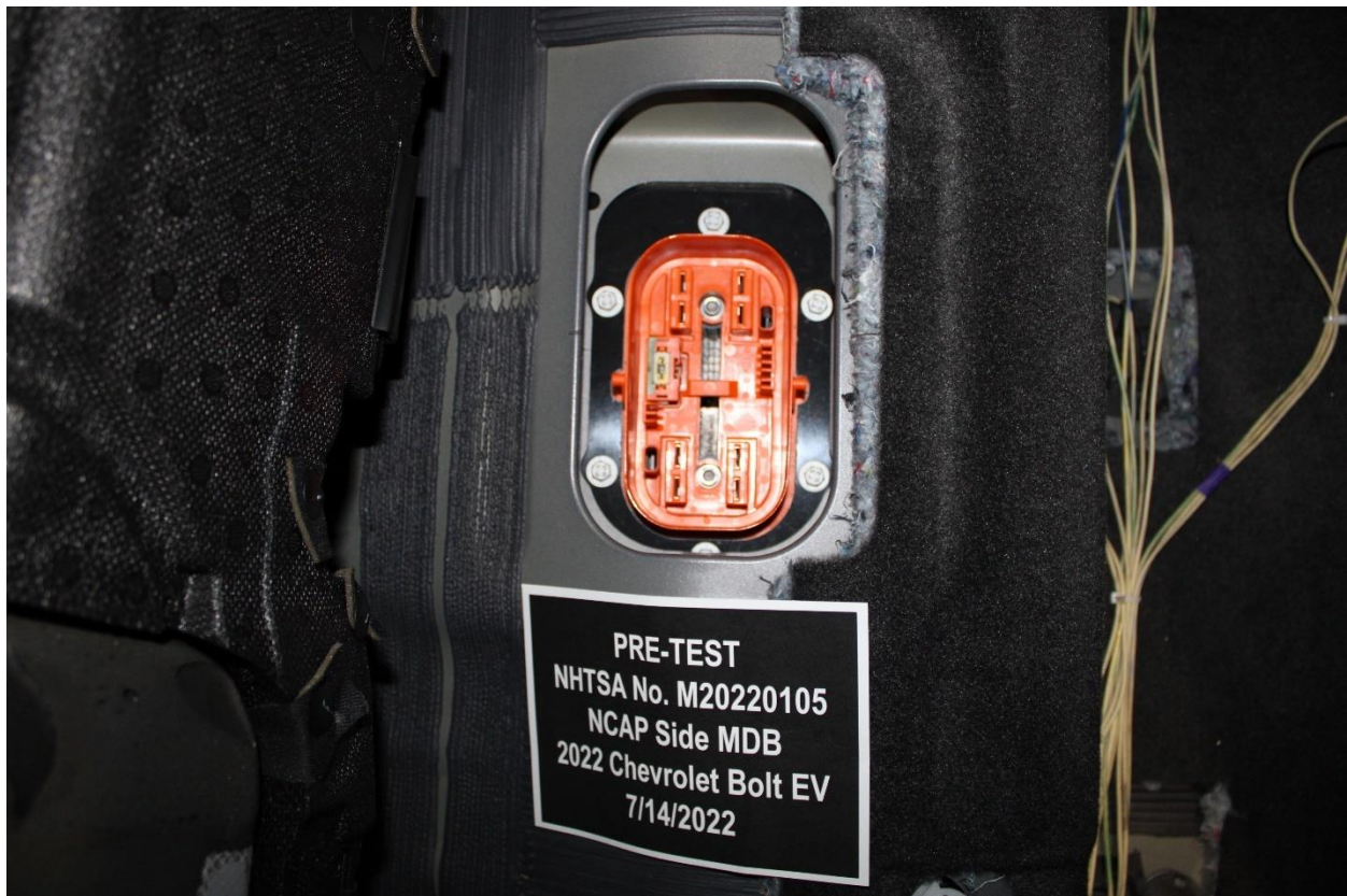
Figure 305-8: Manual High Voltage Service Disconnect Removed Location
