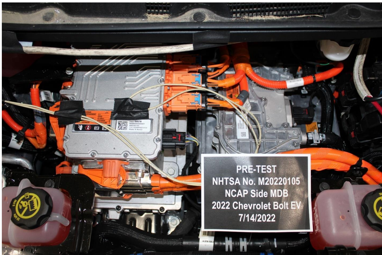
Figure 305-16: Pre-Impact View of Electric Propulsion Drive
