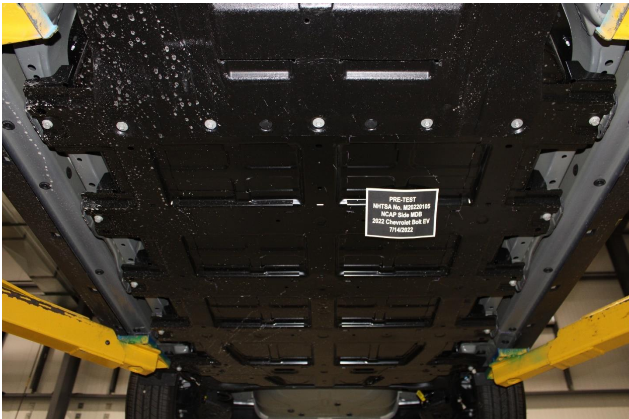
Figure 305-12: Pre-Impact View of Battery Box(s) or Container(s) Which Holds Individual Battery Modules
