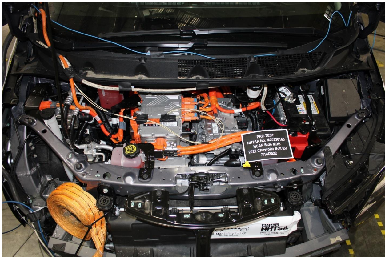
Figure 305-18: Pre-Impact View of High Voltage Interconnects
