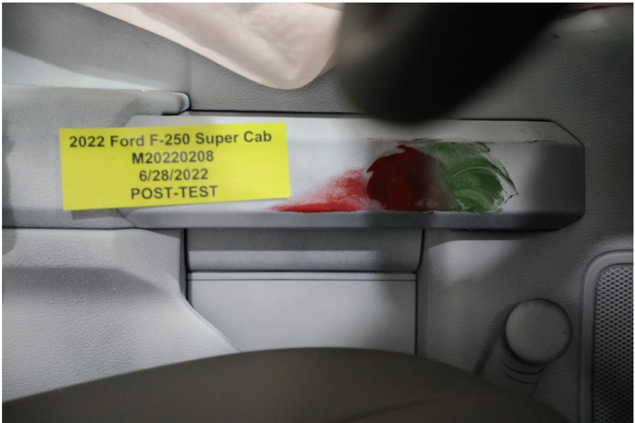
054 Post-Test Driver Dummy Close-Up Knee Contact View
