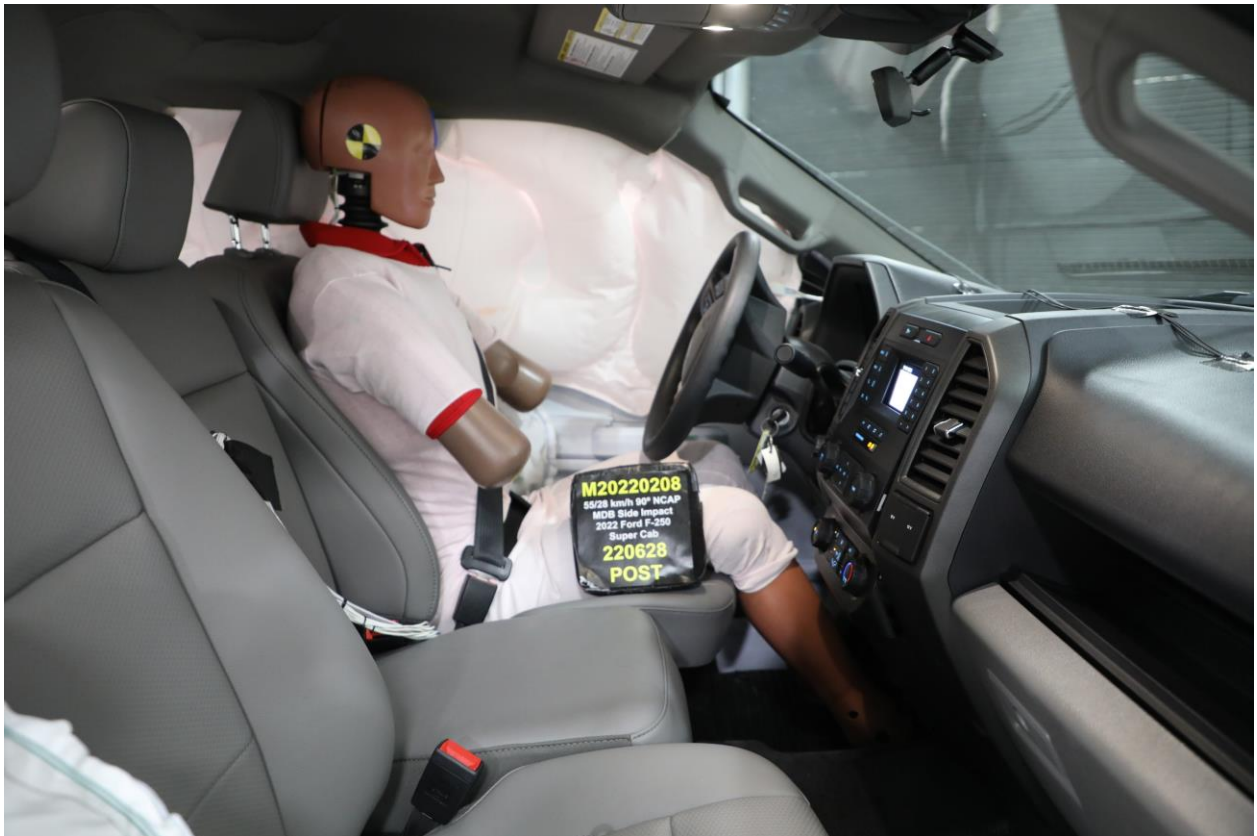
045 Post-Test Right Side View of Driver Dummy and Front Seat of Occupant Compartment
