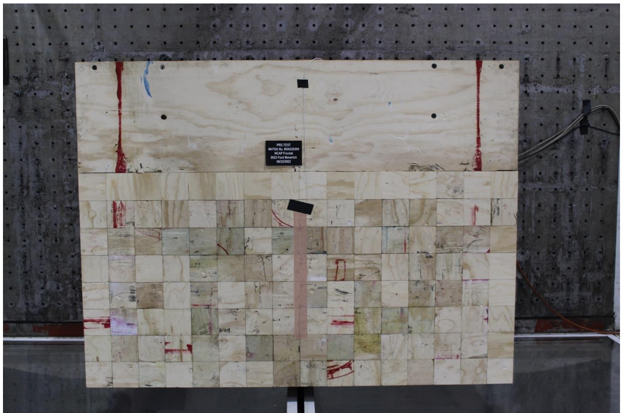
Figure A-2: Pre-Test Load Cell Wall
