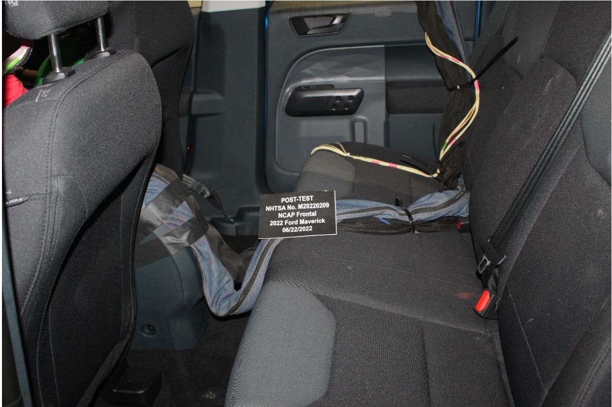
Figure A-29: Post-Test Dummy Cable Routing
