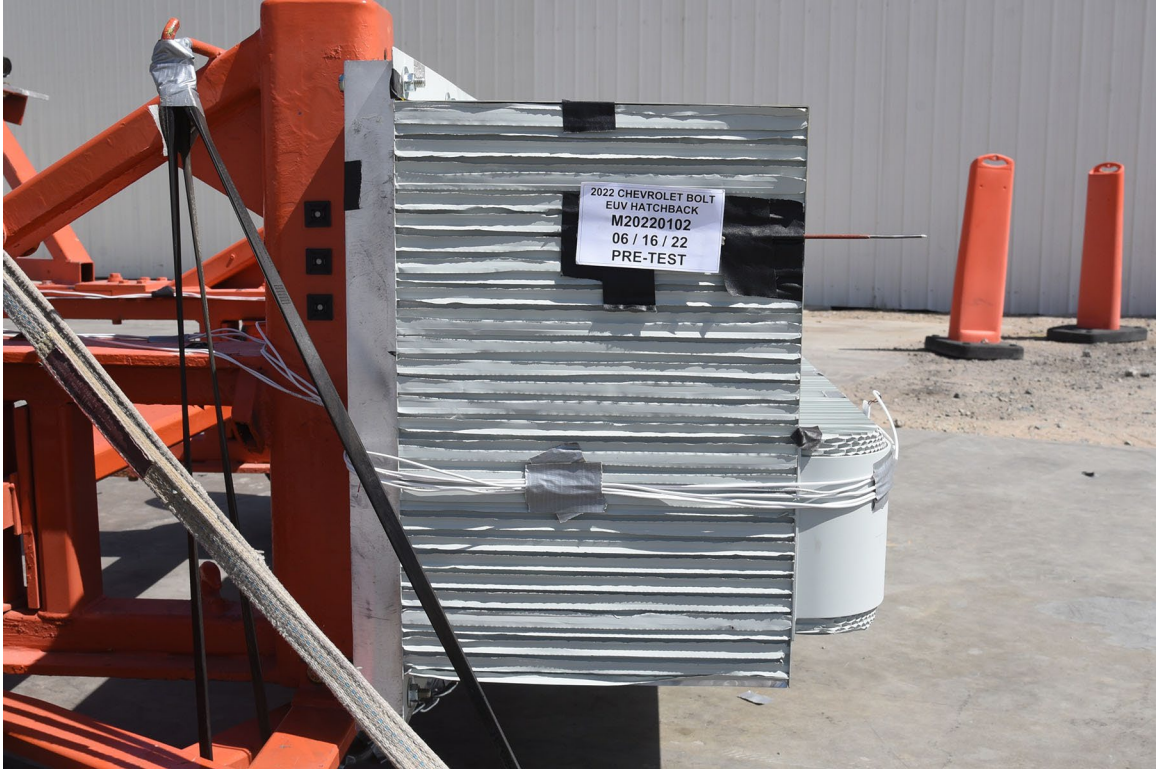
FIGURE 90. Pre-Test Right Side View of MDB Impactor Face
