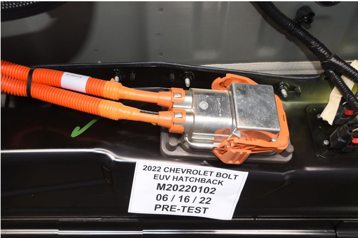
FIGURE 305-018. Pre-Impact View of High Voltage Interconnect(s)
