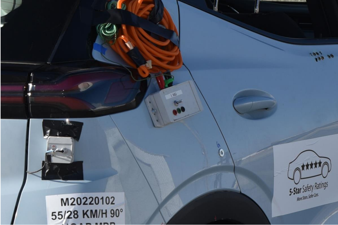
FIGURE 305-025. Post-Impact View of Installed Test Interface Port
