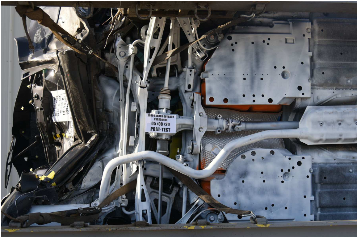
FIGURE 20. Post-Test Rear Underbody View of Test Vehicle
