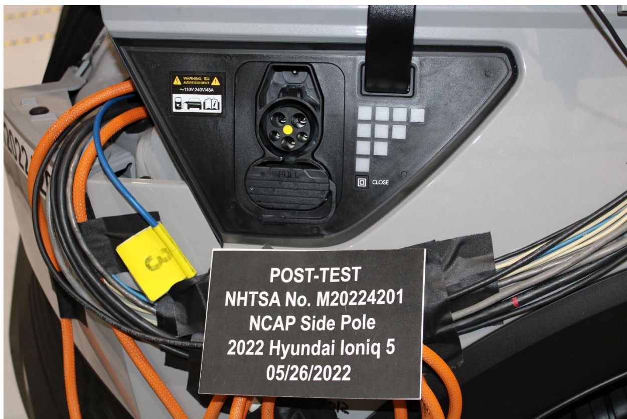
Figure A-56: Post-Test View of Charging Port
