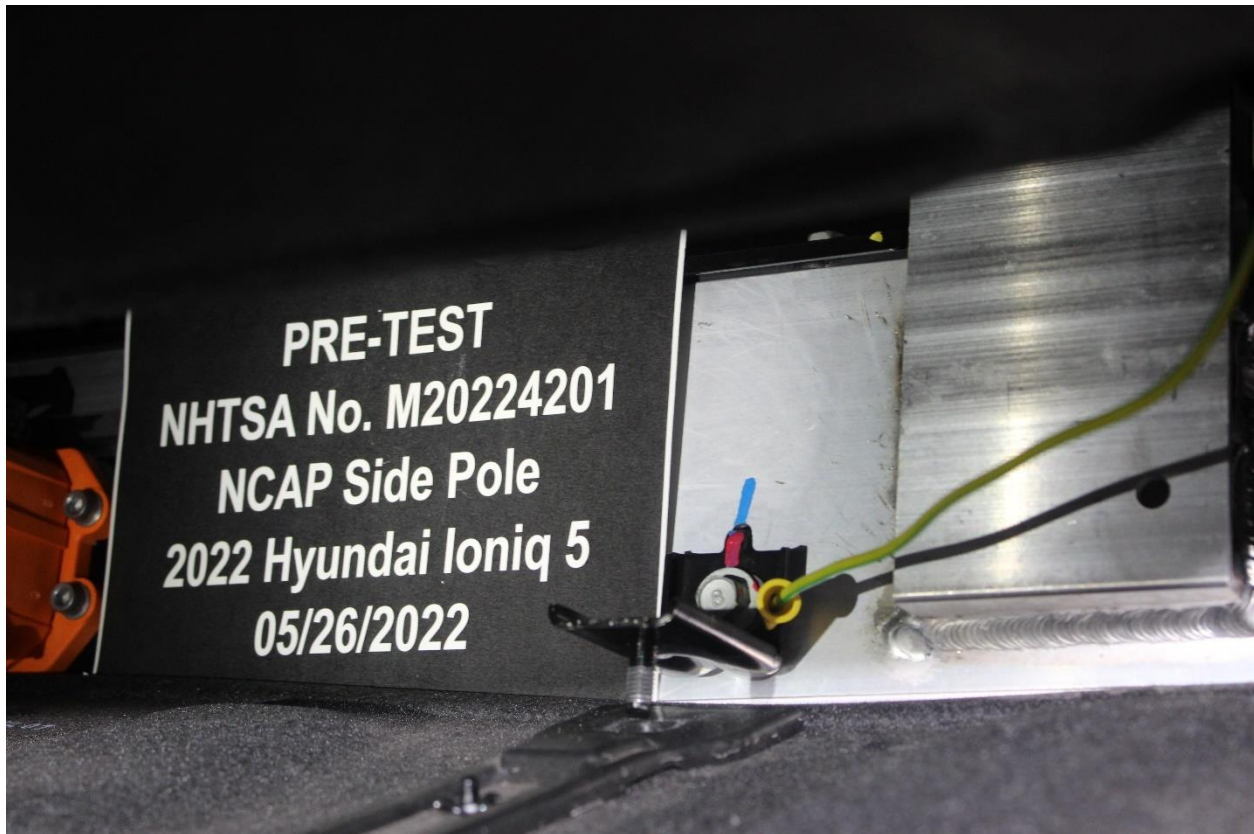
Figure 305-21: Pre-Impact View of Ground Lead Attached
