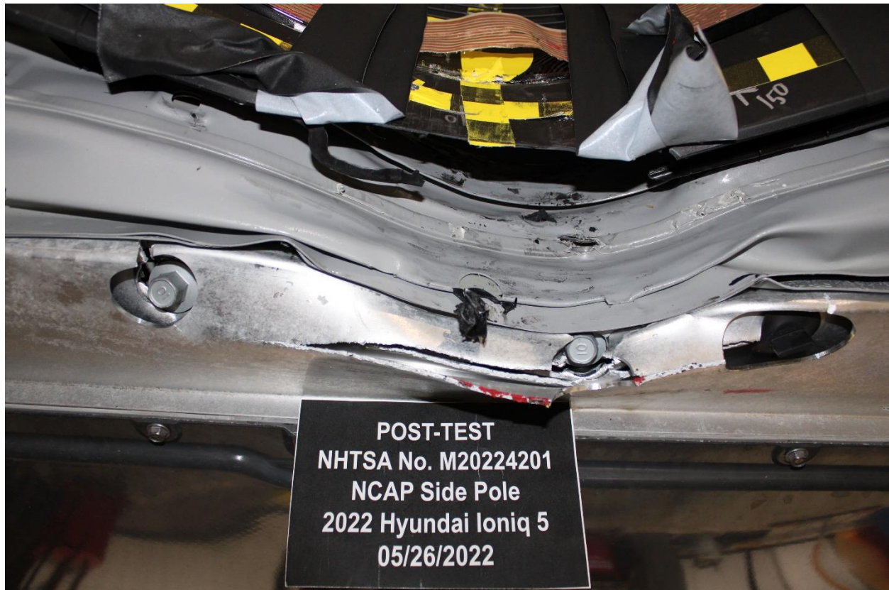
Figure 305-35: Post-Impact View of Battery Component Intrusion (if applicable)
