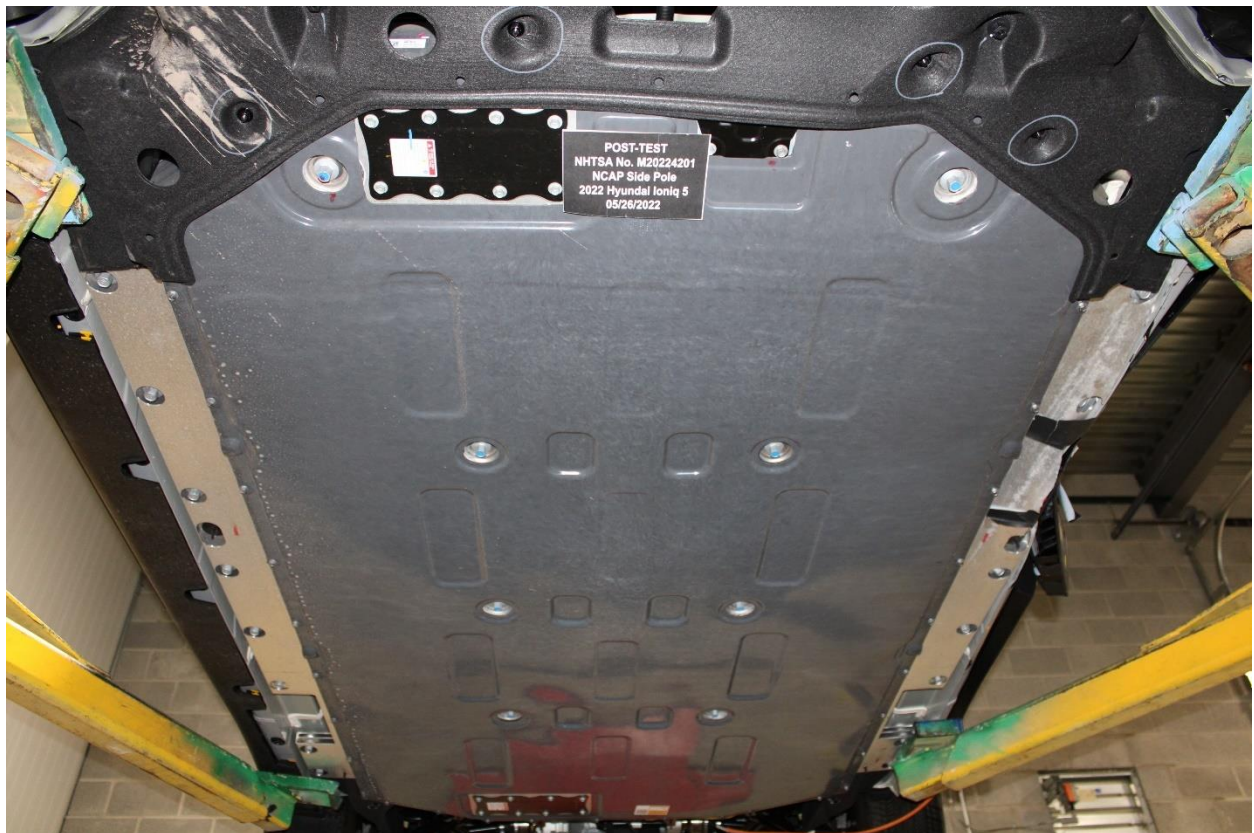
Figure 305-10: Post-Impact Front View of Propulsion Battery
