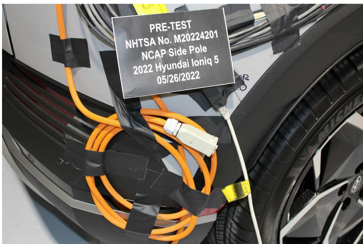
Figure 305-24: Pre-Impact View of Installed Test Interface Port
