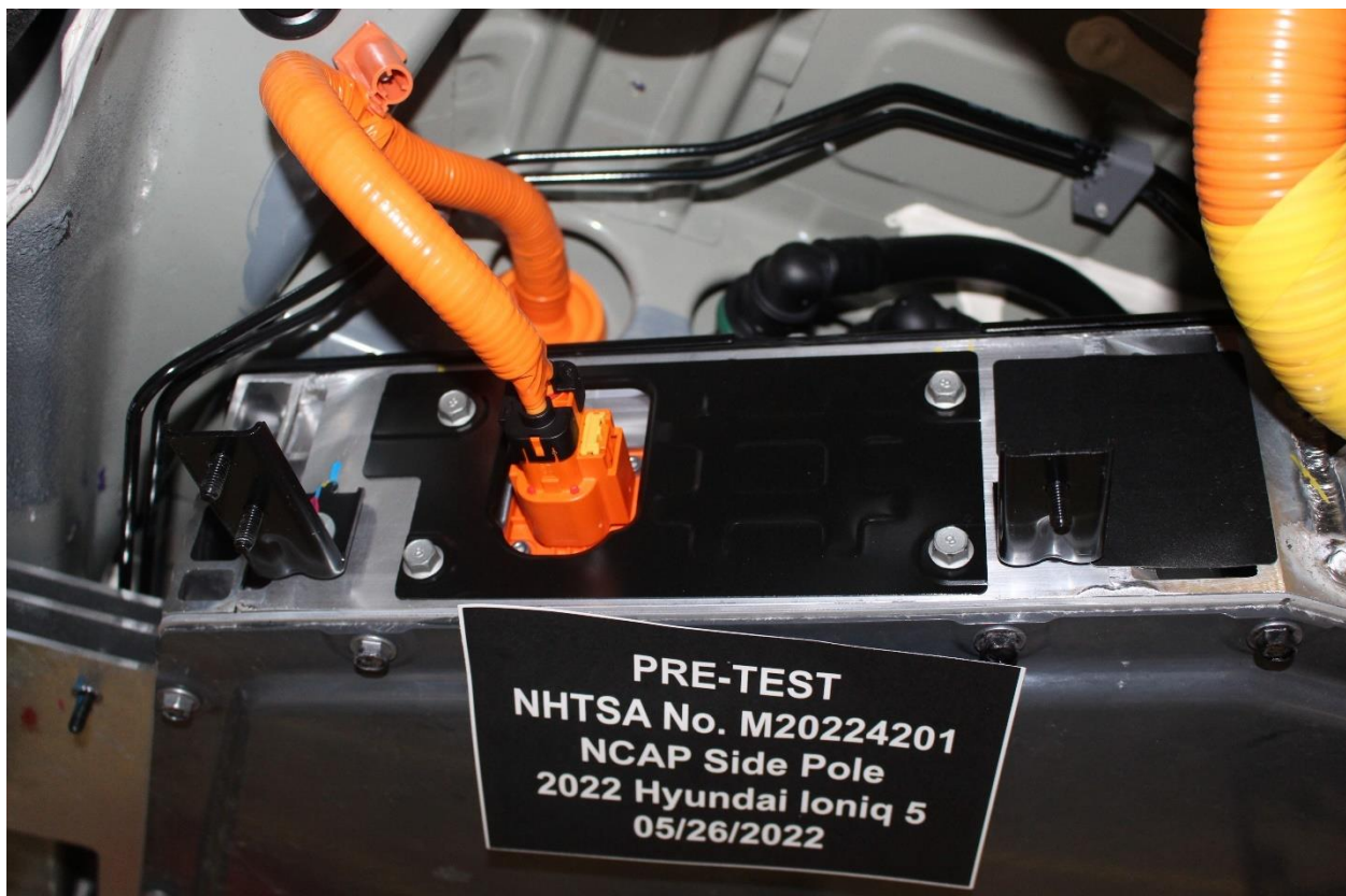
Figure 305-18: Pre-Impact View of High Voltage Interconnects
