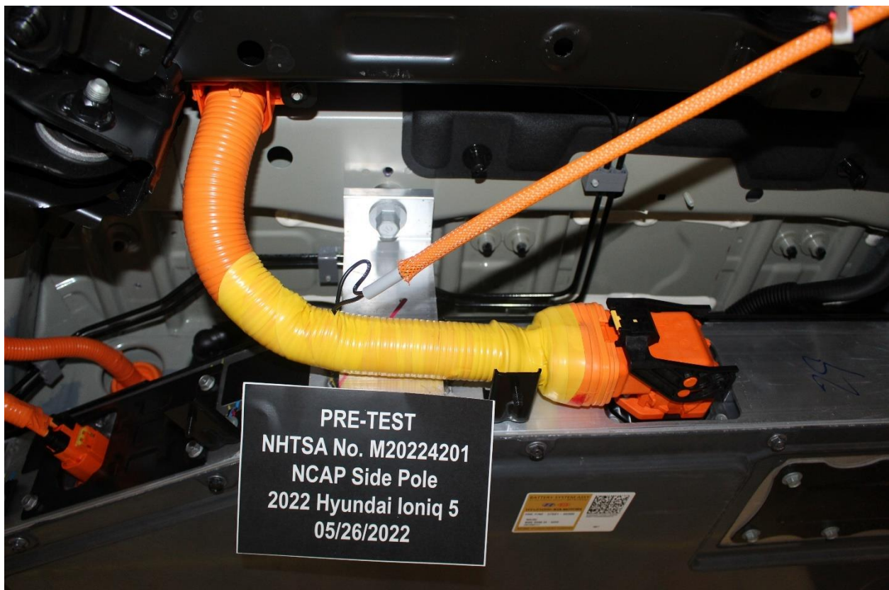
Figure 305-22: Pre-Impact View of High Voltage Leads Attached
