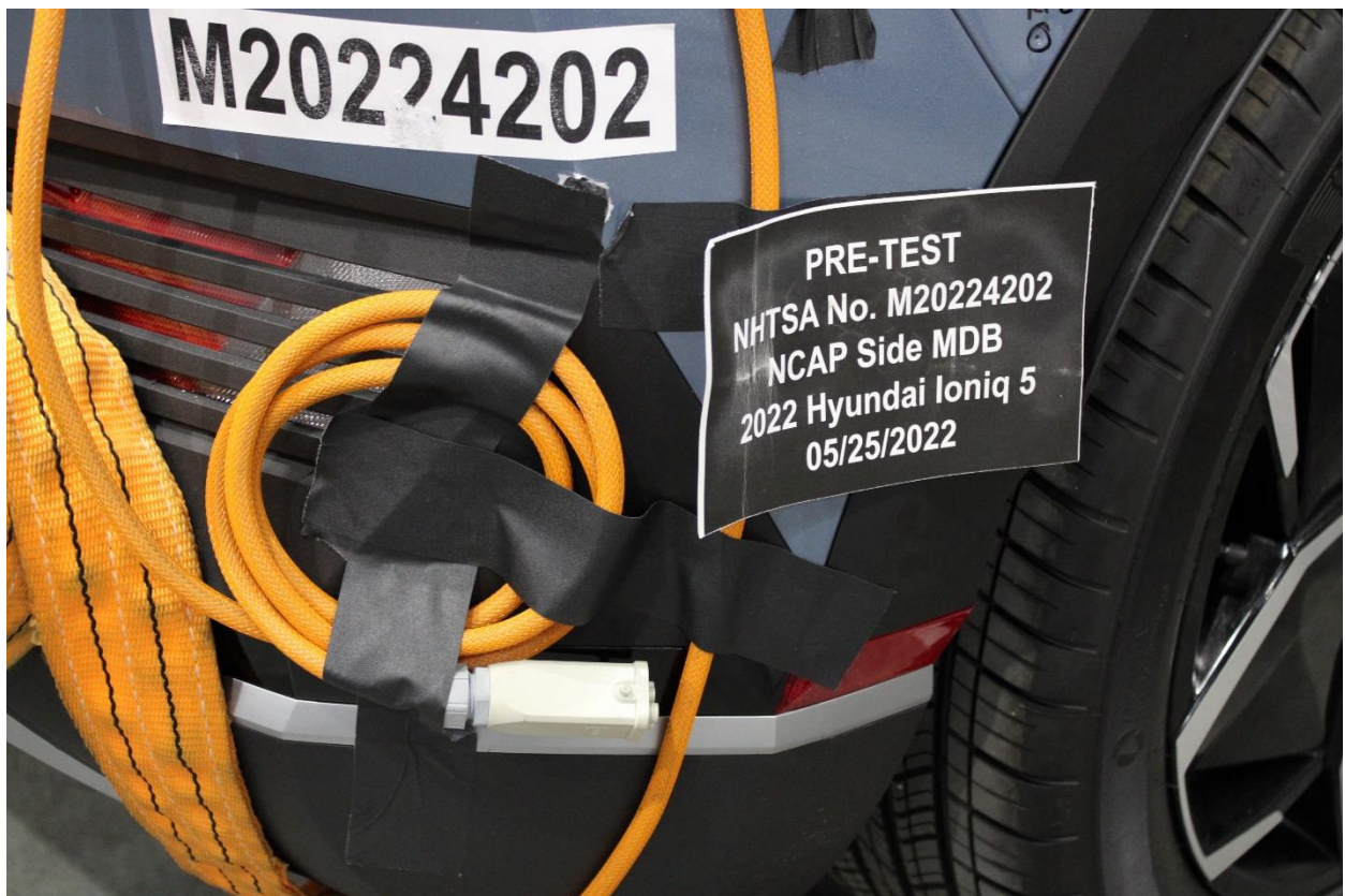
Figure 305-24: Pre-Impact View of Installed Test Interface Port
