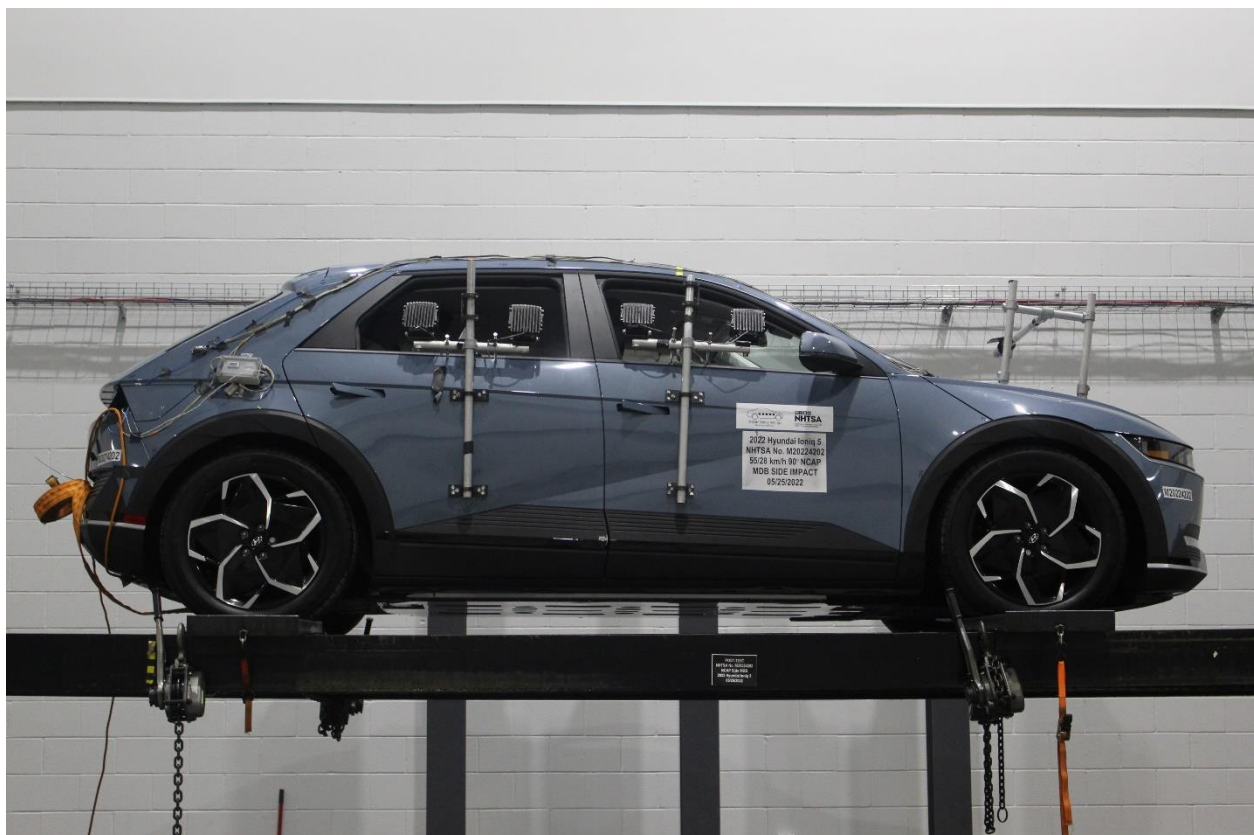
Figure A-100: FMVSS No. 301 Static Rollover 360 Degrees
