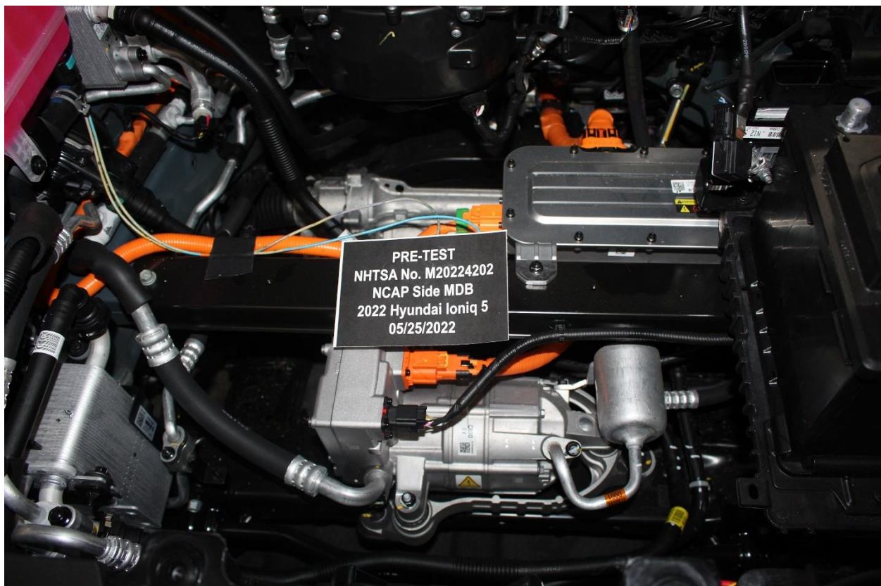
Figure 305-18: Pre-Impact View of High Voltage Interconnects
