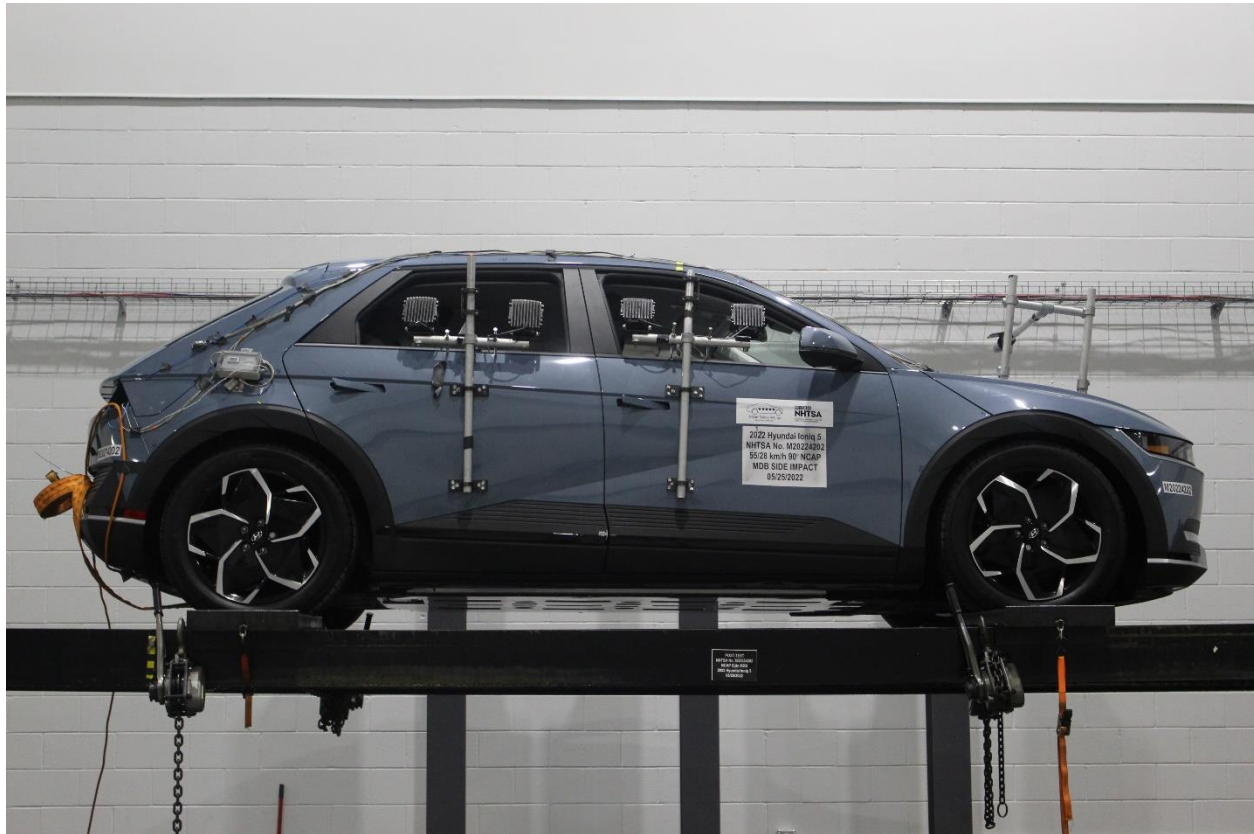
Figure 305-31: FMVSS No. 305 Static Rollover 360 Degrees
