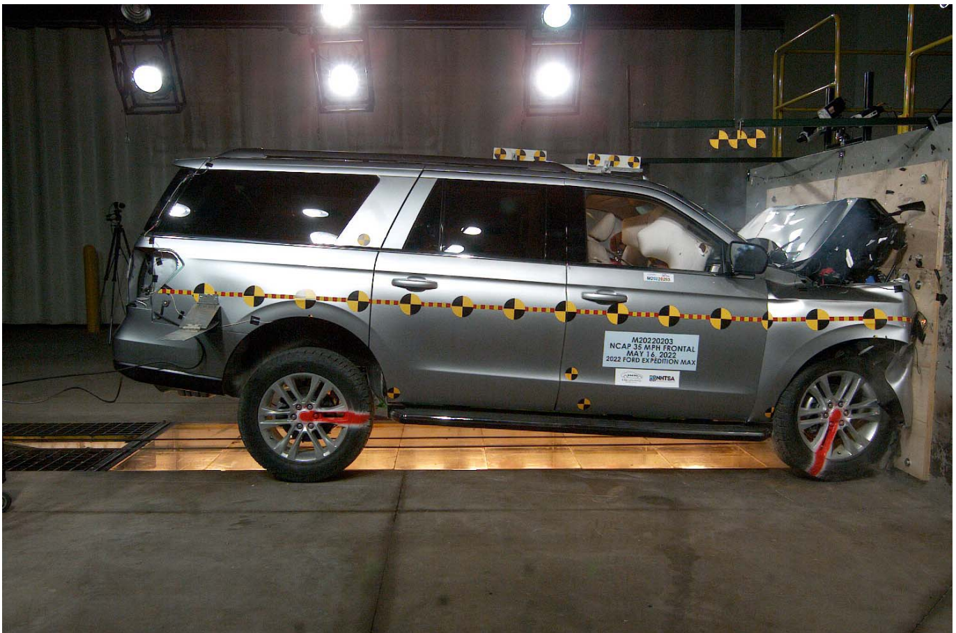
Photo No. 082 - 2022 Ford Expedition MAX 5-Door SUV Frontal Impact Event
