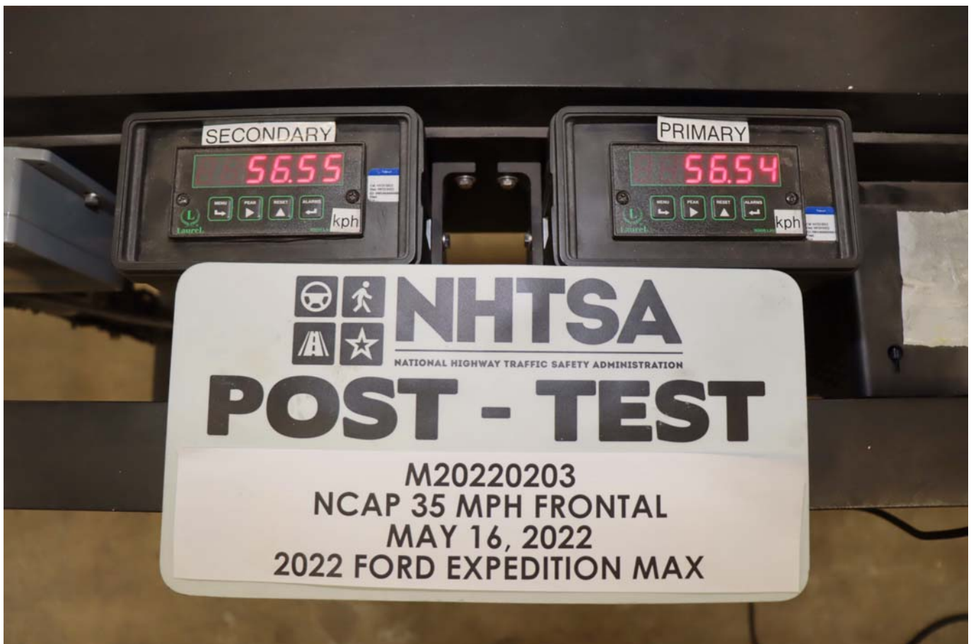
Photo No. 076 - Post-Test Speed Trap Read-Out
