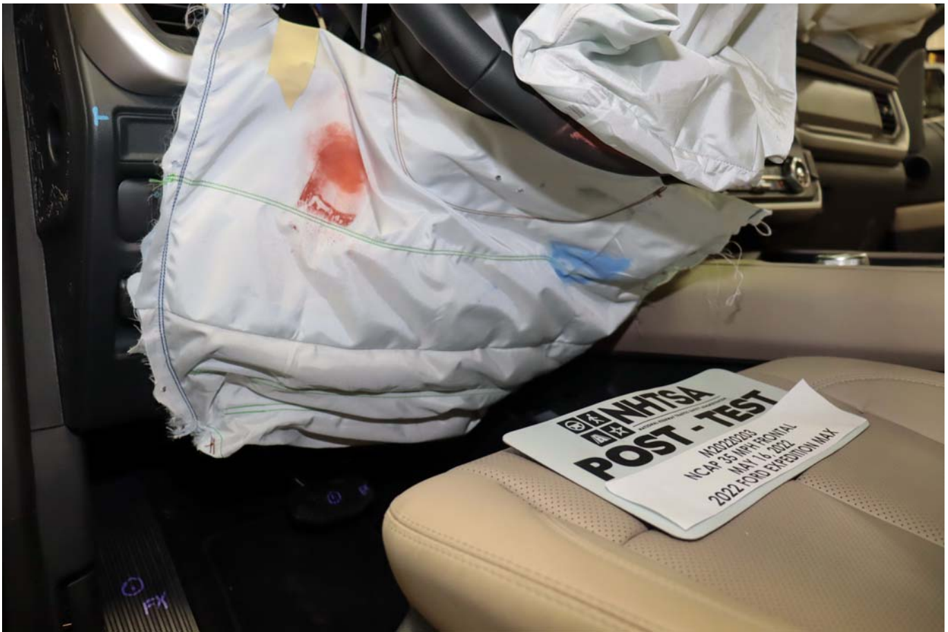
Photo No. 045 - Post-Test Driver's Side Knee Bolster
