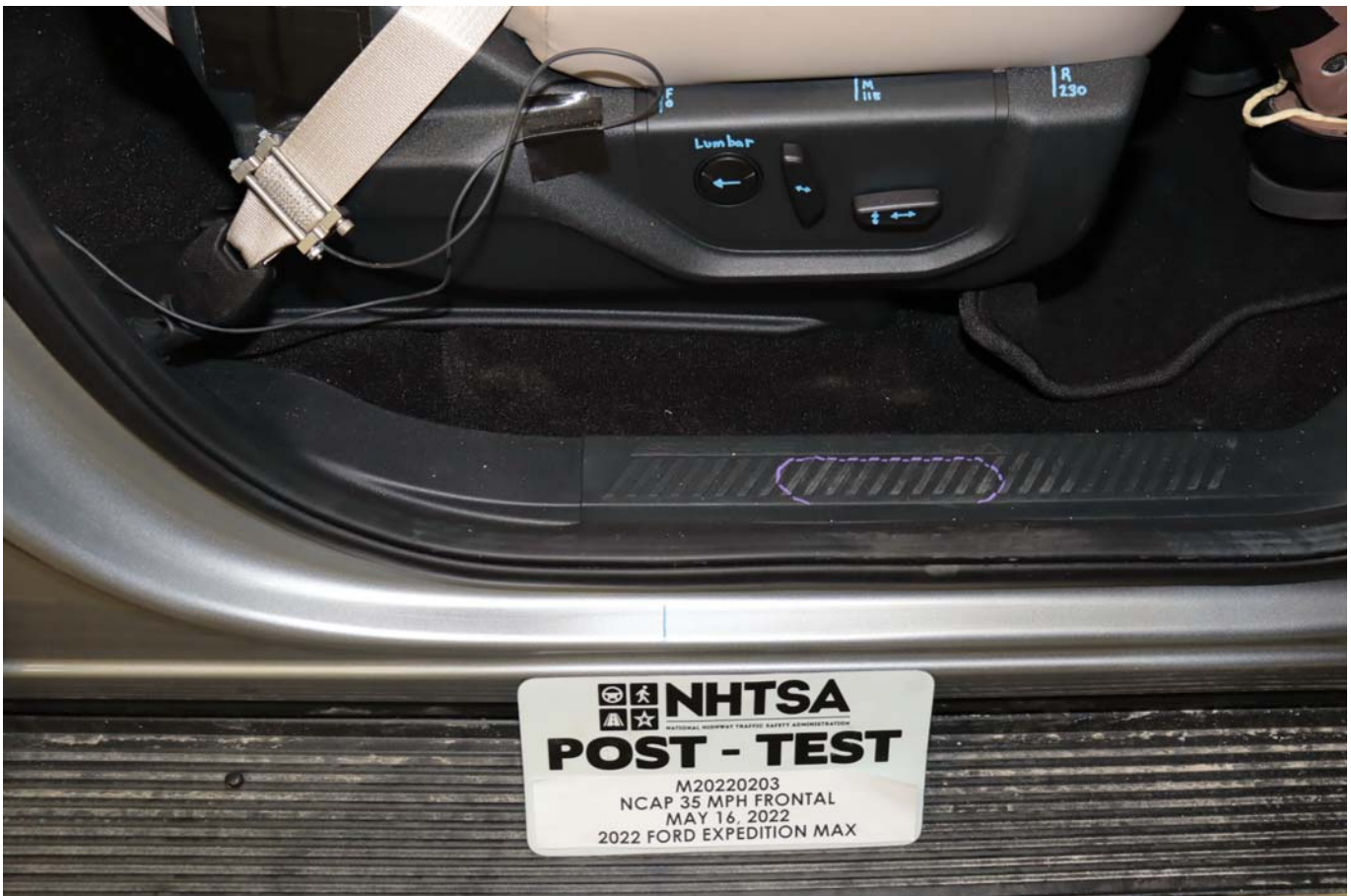
Photo No. 060 - Post-Test Passenger's Seat Fore-Aft Markings
