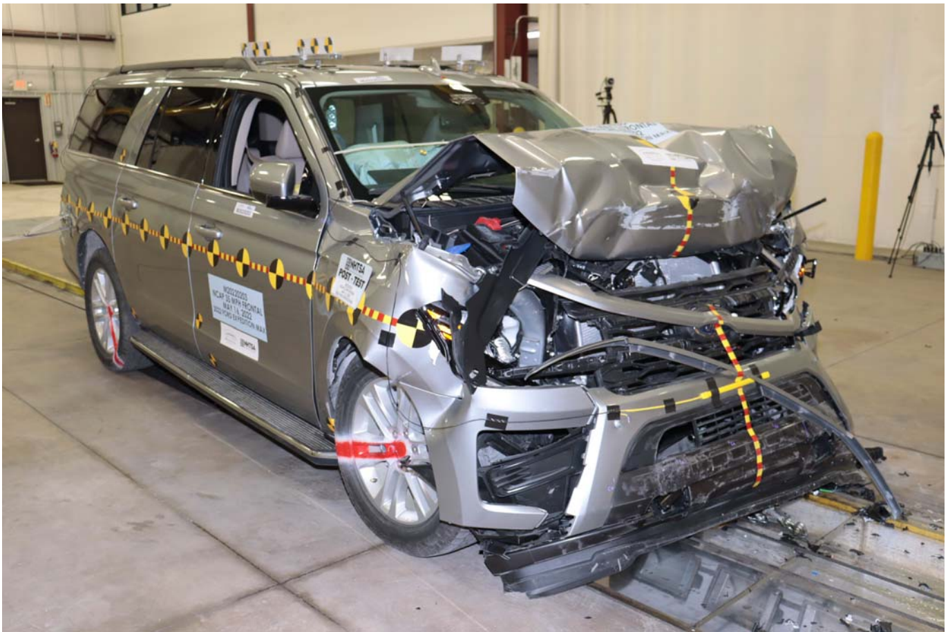
Photo No. 015 - Post-Test Right Front 3-4 View
