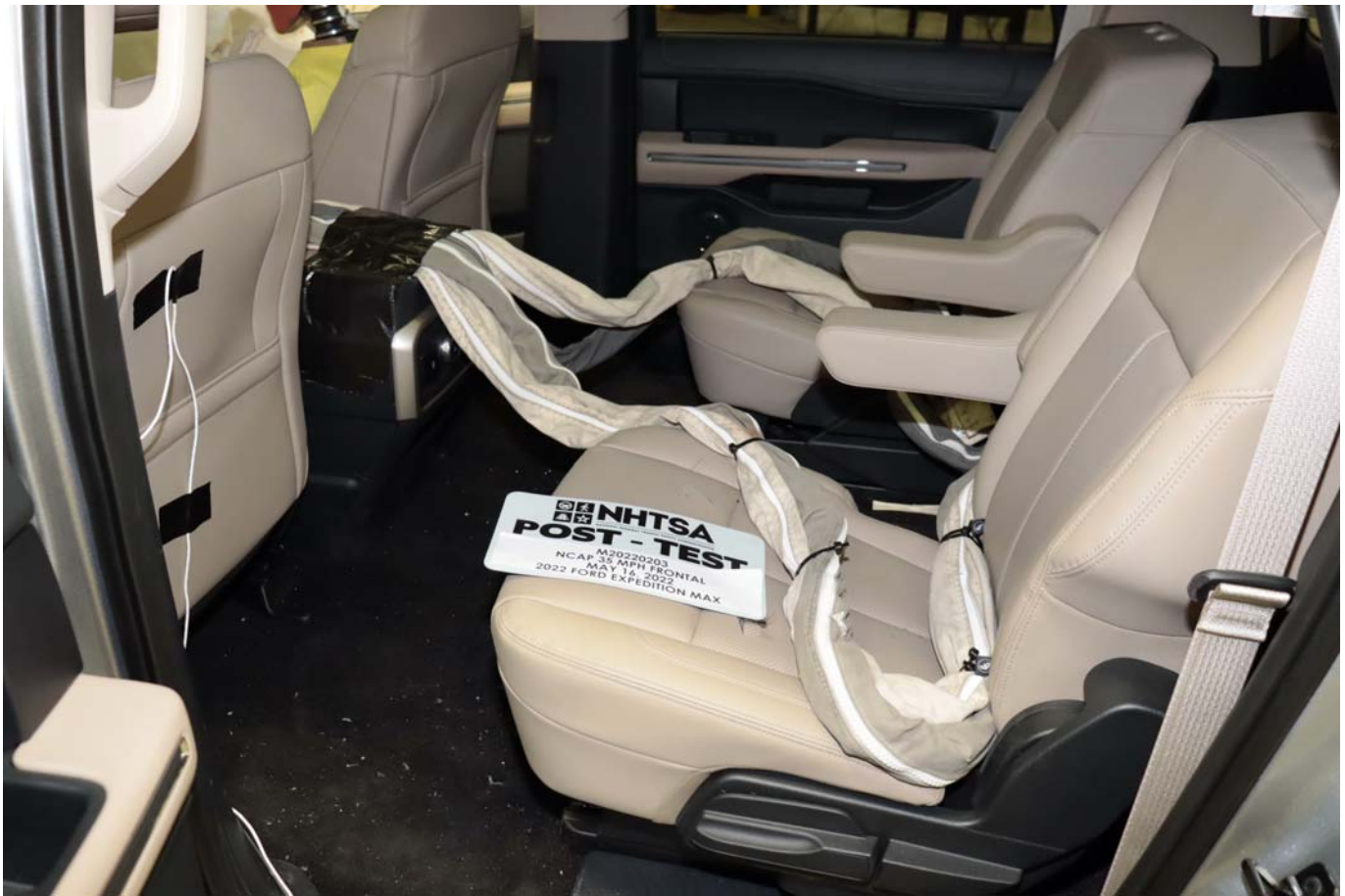
Photo No. 029 - Post-Test Dummy Cable Routing
