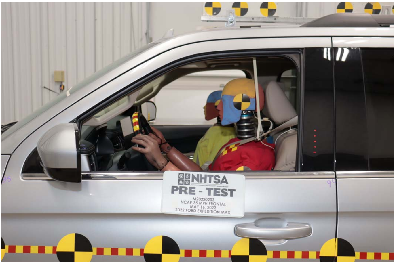
Photo No. 032 - Pre-Test Driver Dummy Window View
