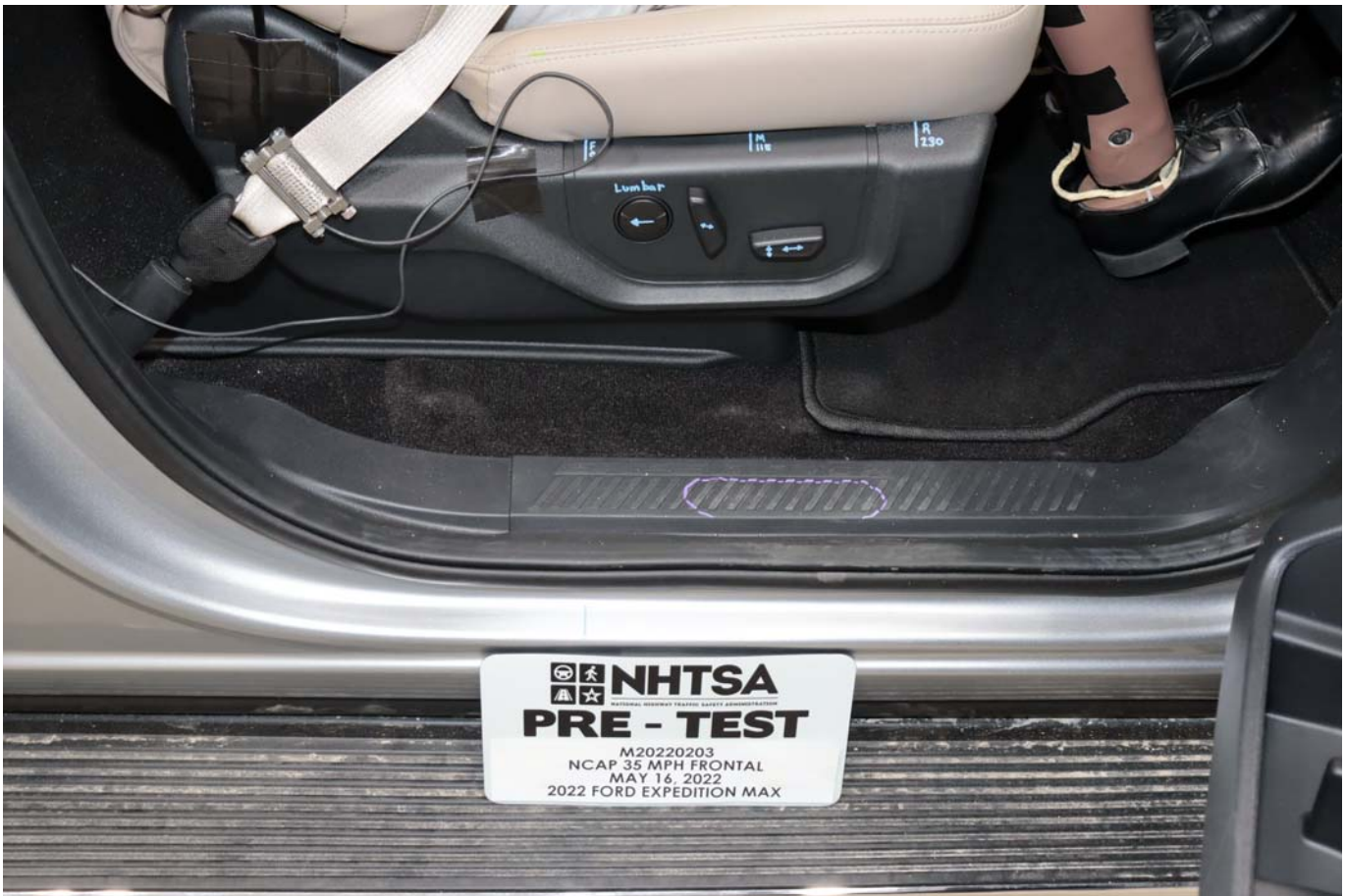
Photo No. 059 - Pre-Test Passenger's Seat Fore-Aft Markings
