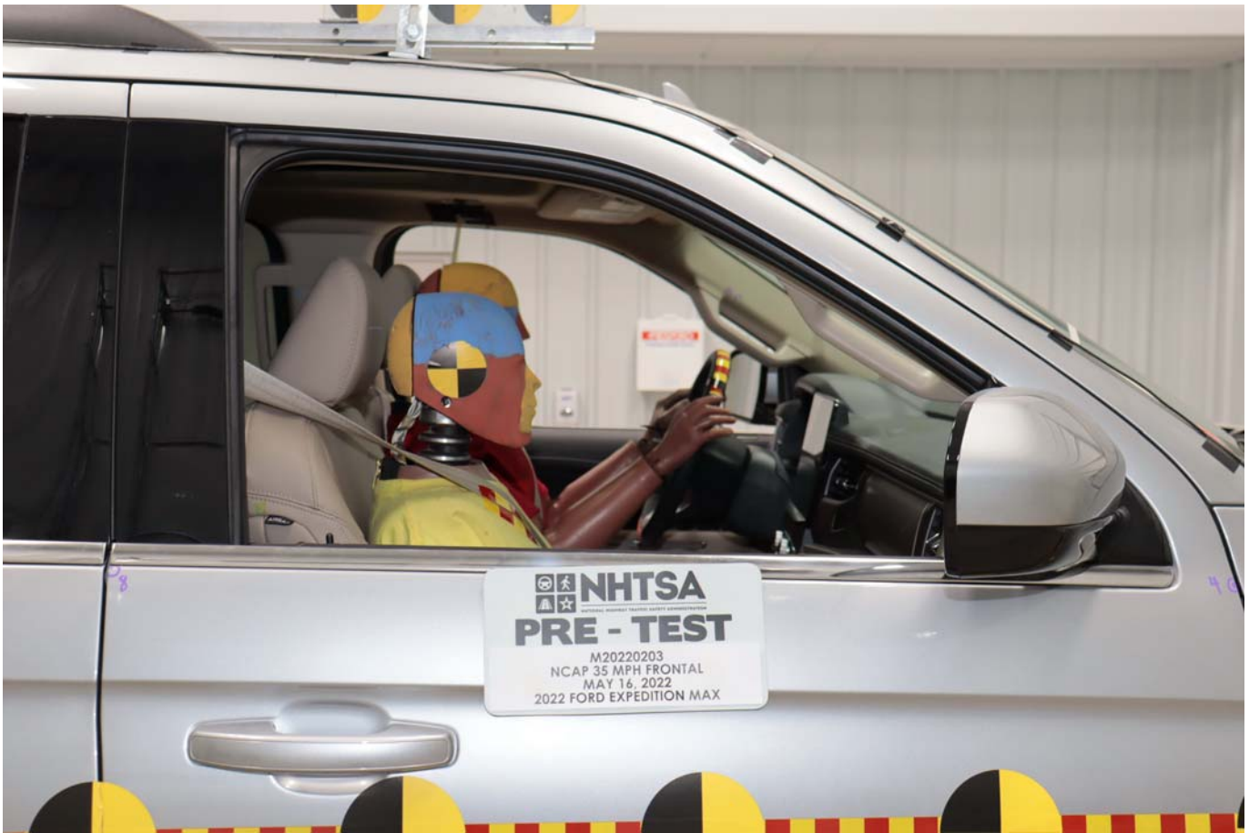
Photo No. 055 - Pre-Test Passenger Dummy Window View
