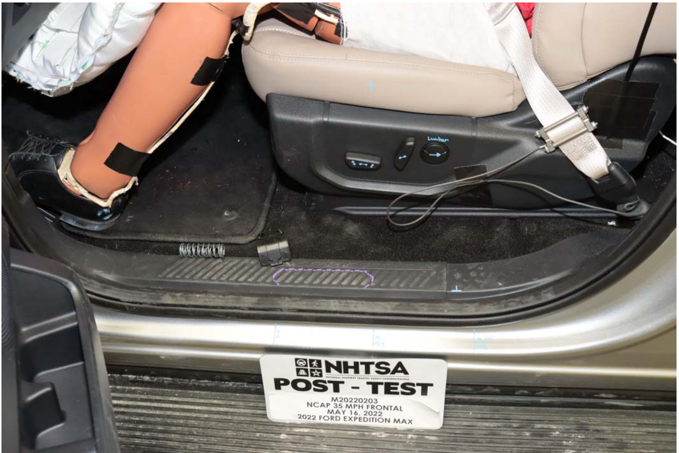
Photo No. 037 - Post-Test Driver's Seat Fore-Aft Markings
