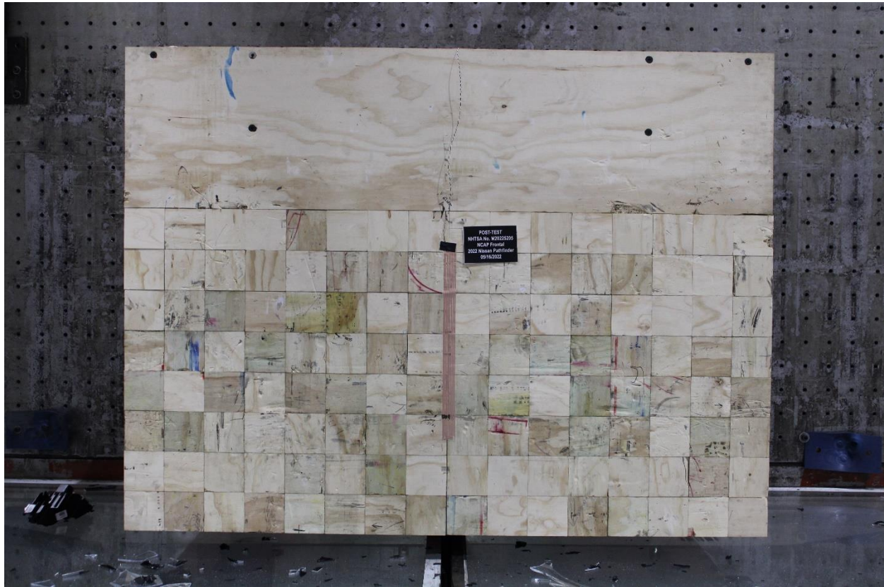
Figure A-3: Post-Test Load Cell Wall
