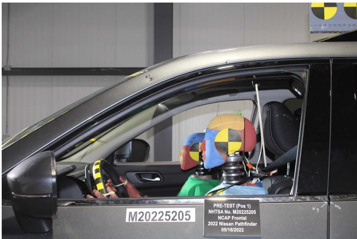
Figure A-32: Pre-Test Driver Dummy Window View
