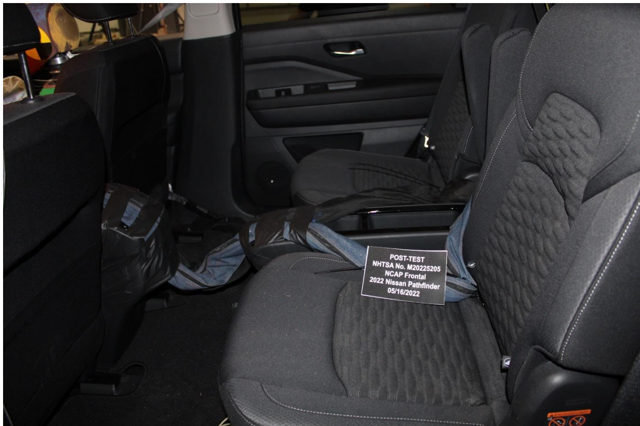
Figure A-29: Post-Test Dummy Cable Routing
