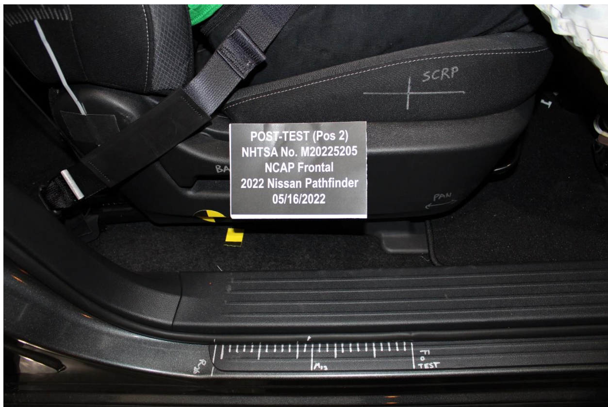
Figure A-60: Post-Test Passenger's Seat Fore-Aft Markings
