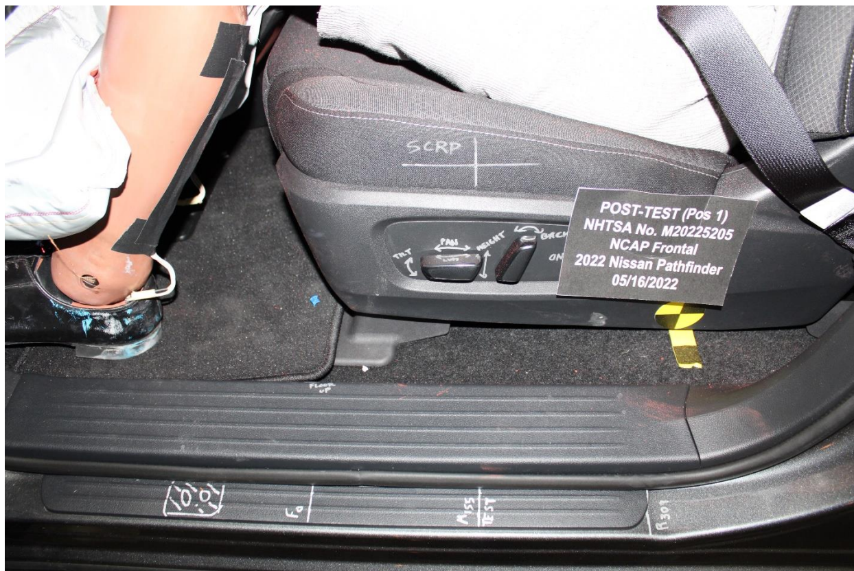
Figure A-37: Post-Test Driver's Seat Fore-Aft Markings
