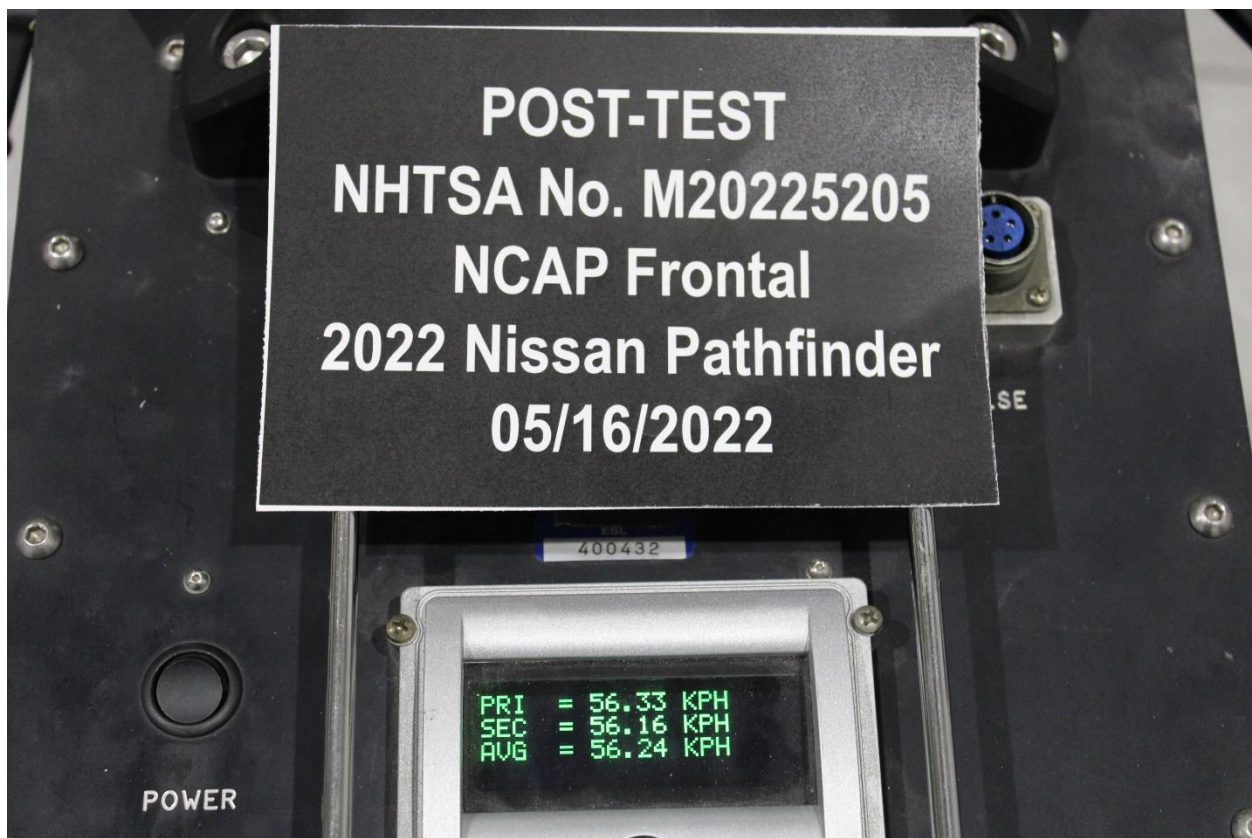
Figure A-76: Post-Test Speed Trap Read-Out
