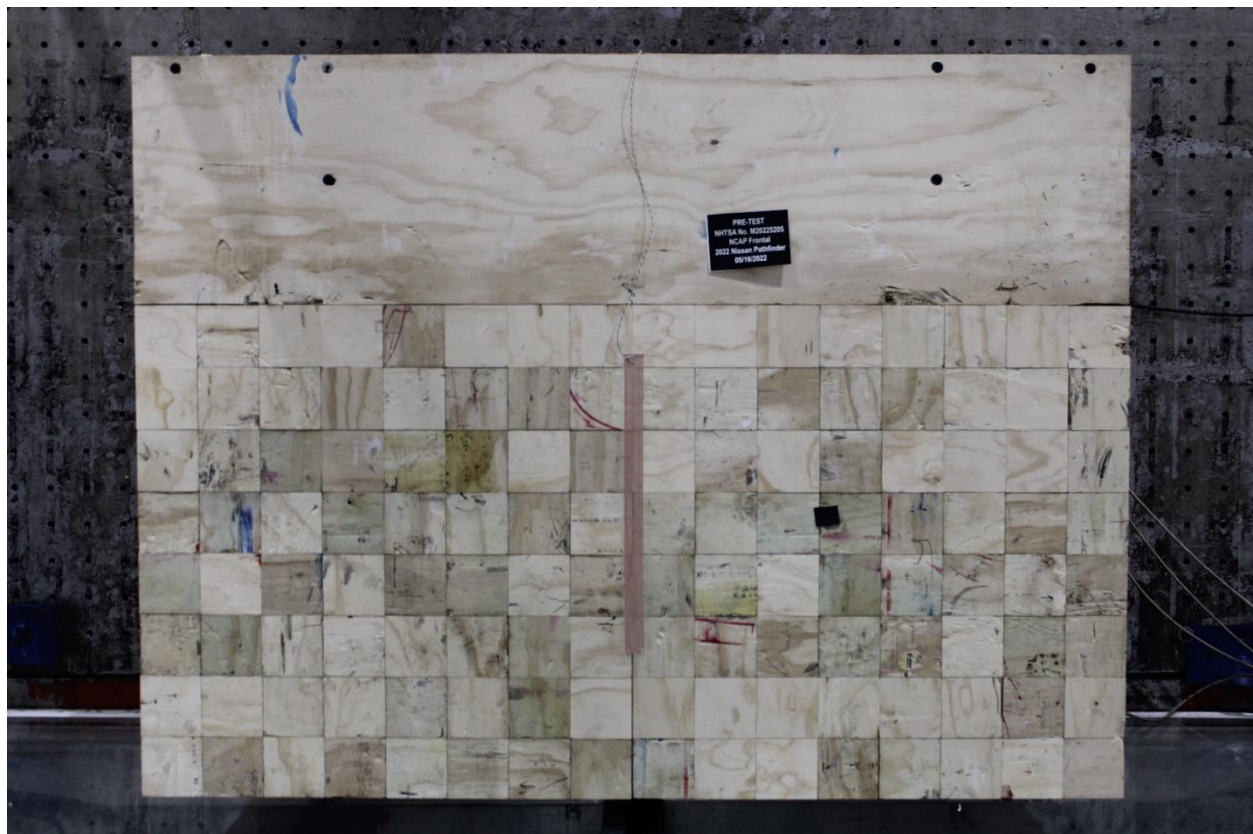
Figure A-2: Pre-Test Load Cell Wall
