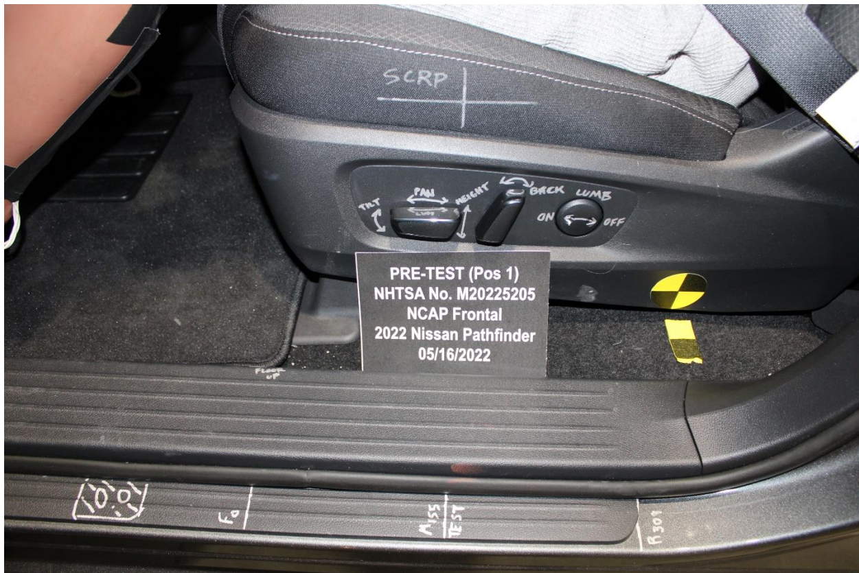
Figure A-36: Pre-Test Driver's Seat Fore-Aft Markings
