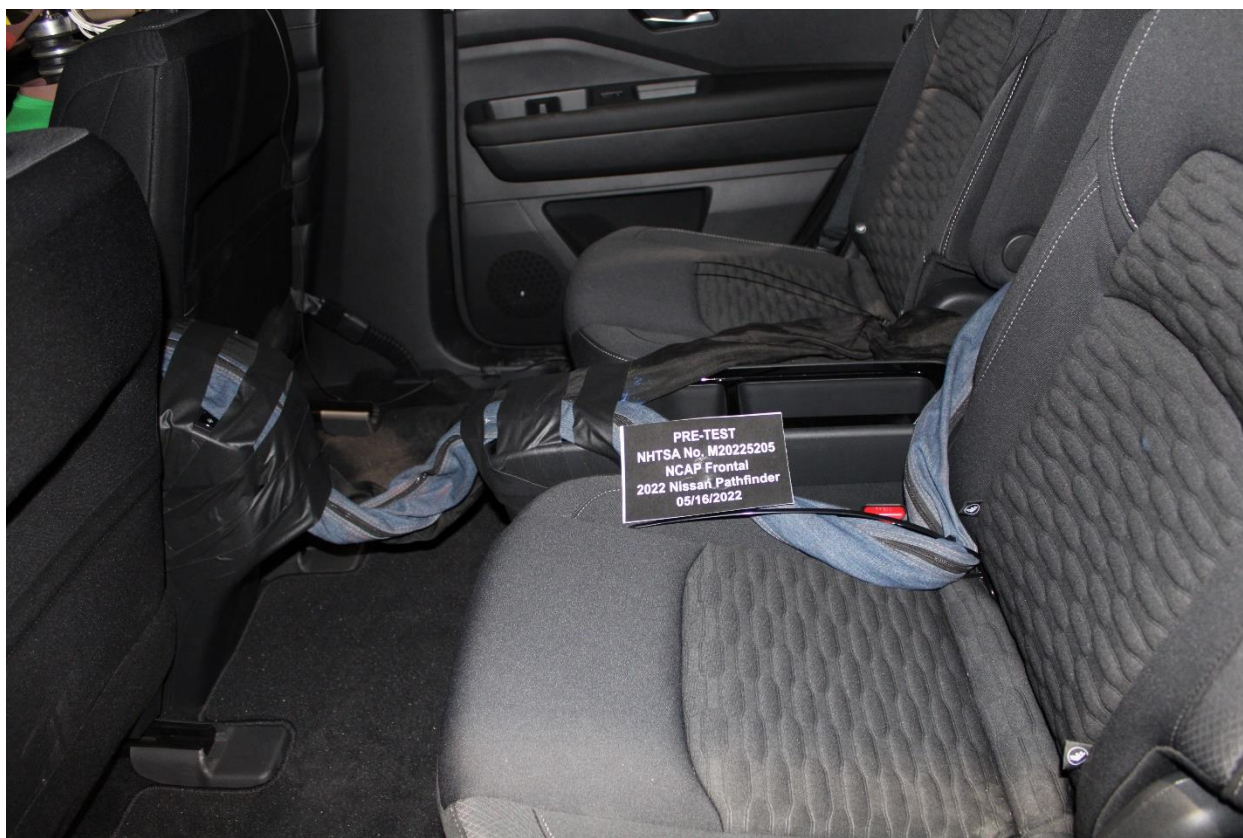
Figure A-28: Pre-Test Dummy Cable Routing
