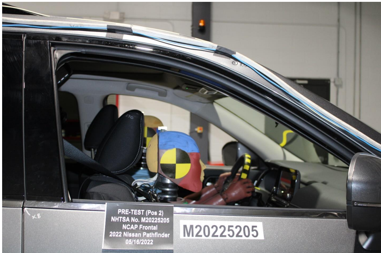
Figure A-55: Pre-Test Passenger Dummy Window View
