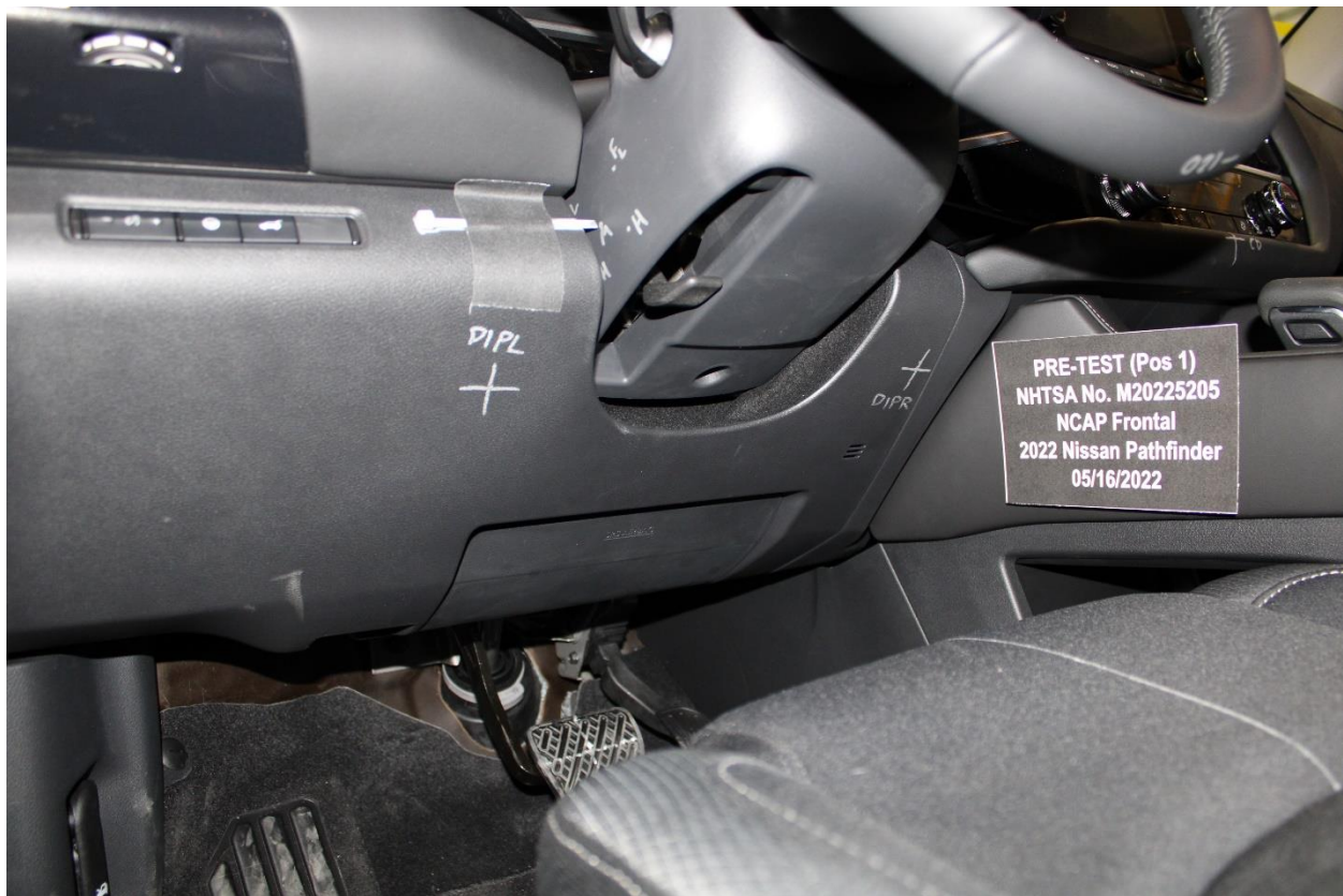
Figure A-44: Pre-Test Driver's Side Knee Bolster
