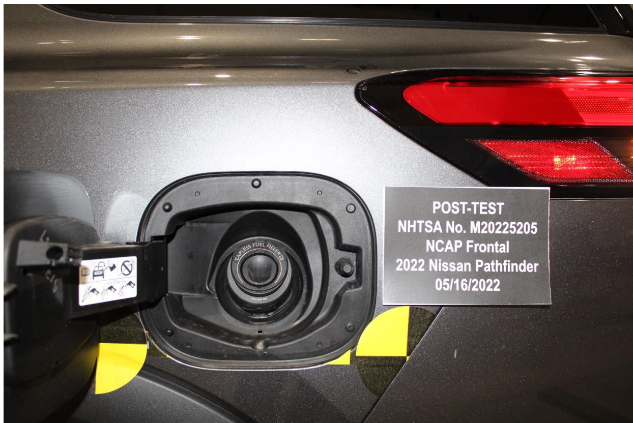
Figure A-23: Post-Test Fuel Filler Cap View
