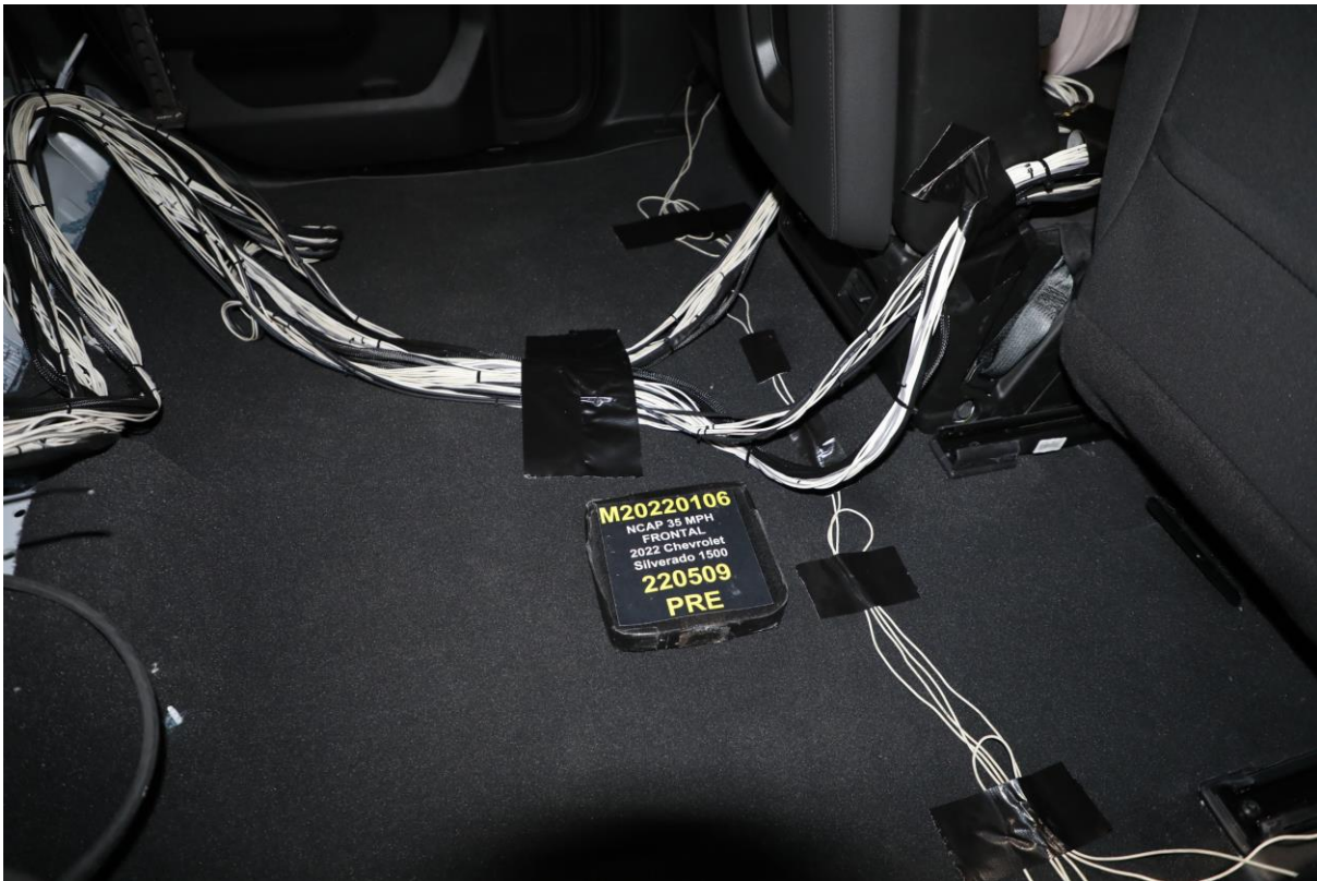
028 Pre-Test Dummy Cable Routing
