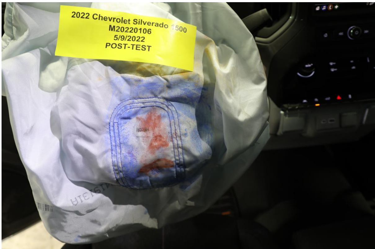
049 Post-Test Driver Dummy Contact with Airbag
