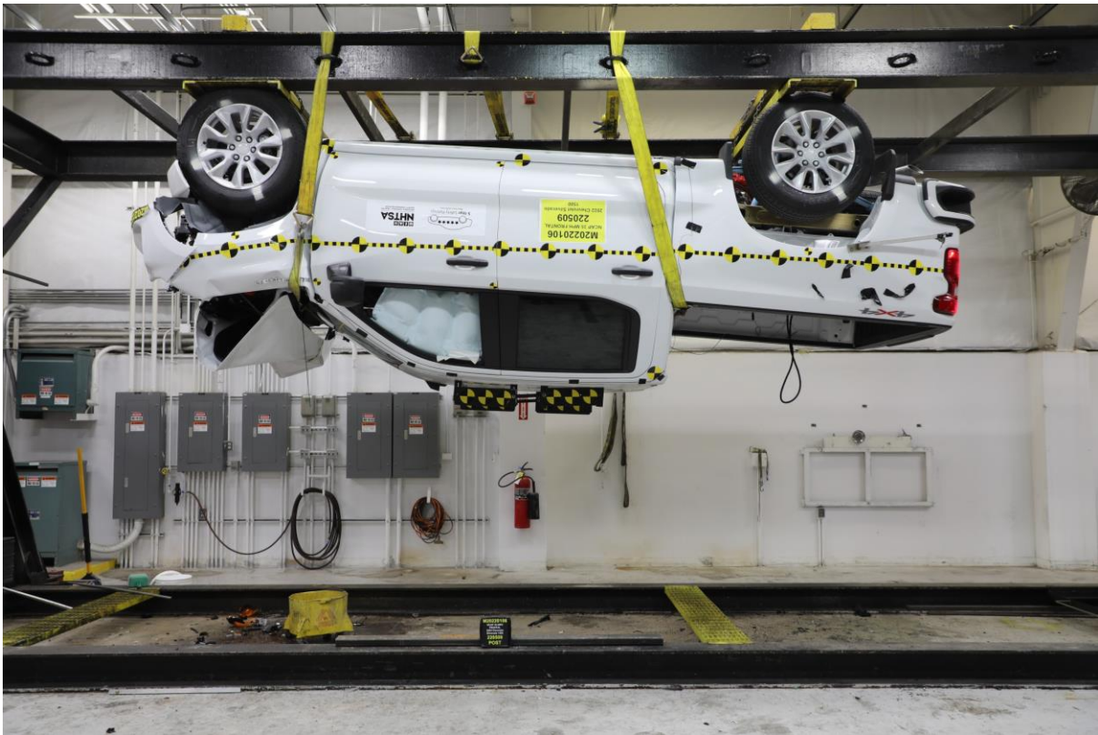
079 Vehicle at 180° on Static Rollover Device
