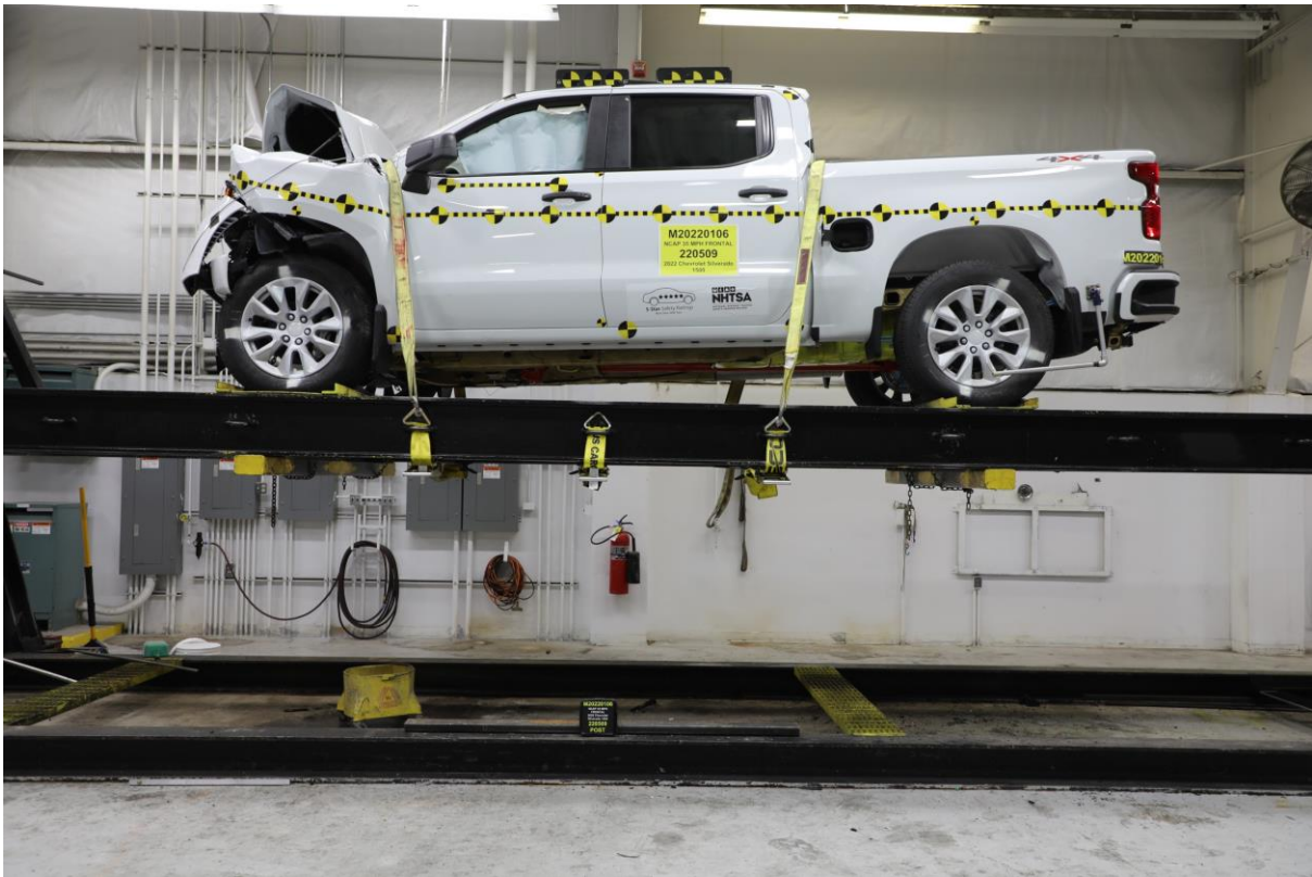
077 Vehicle at 0° on Static Rollover Device
