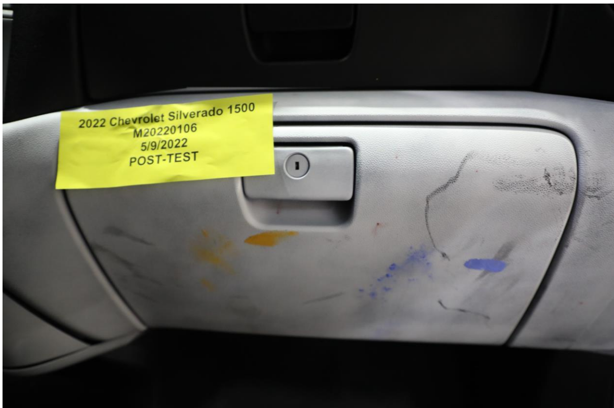
068 Post-Test Passenger's Side Knee Bolster
