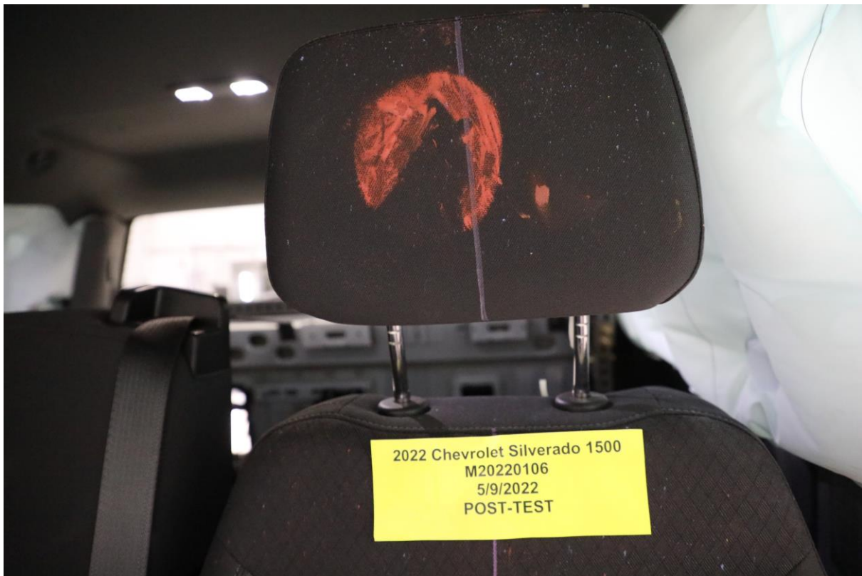
050 Post-Test Driver Dummy Contact with Headrest
