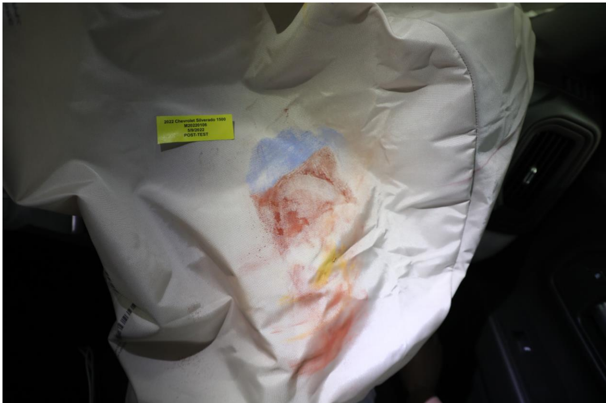
072 Post-Test Passenger Dummy Contact with Airbag
