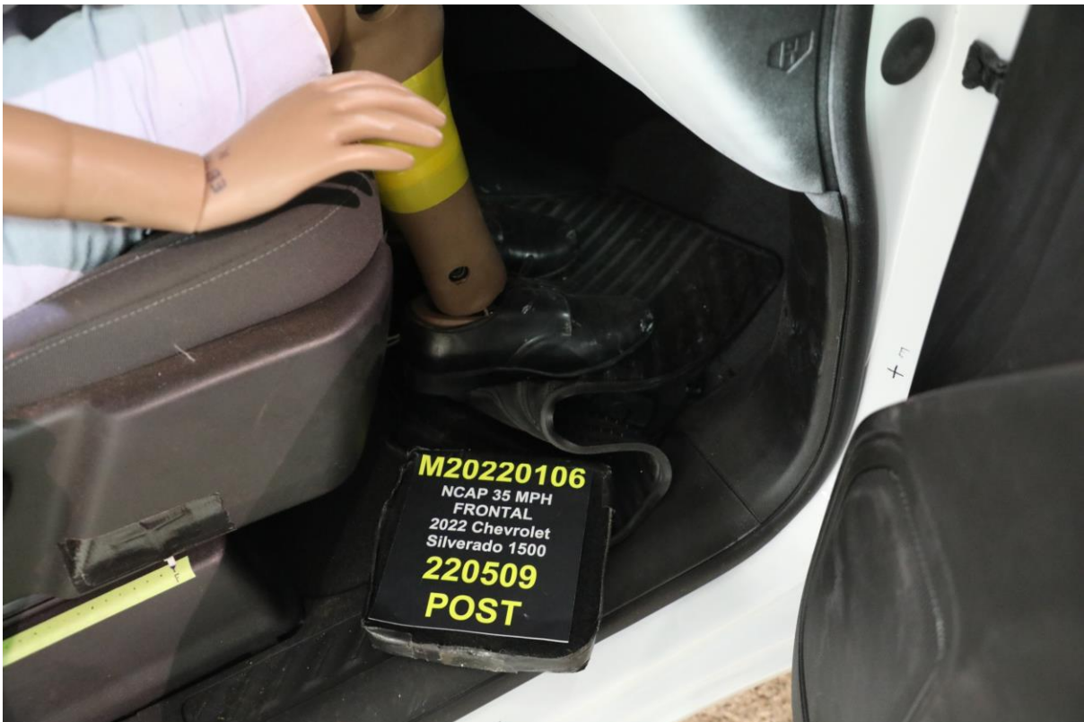
066 Post-Test Passenger Dummy Feet
