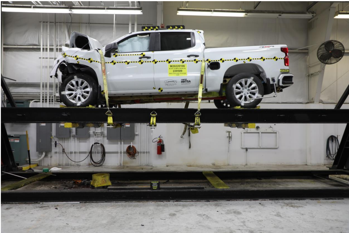
081 Vehicle at 360° on Static Rollover Device
