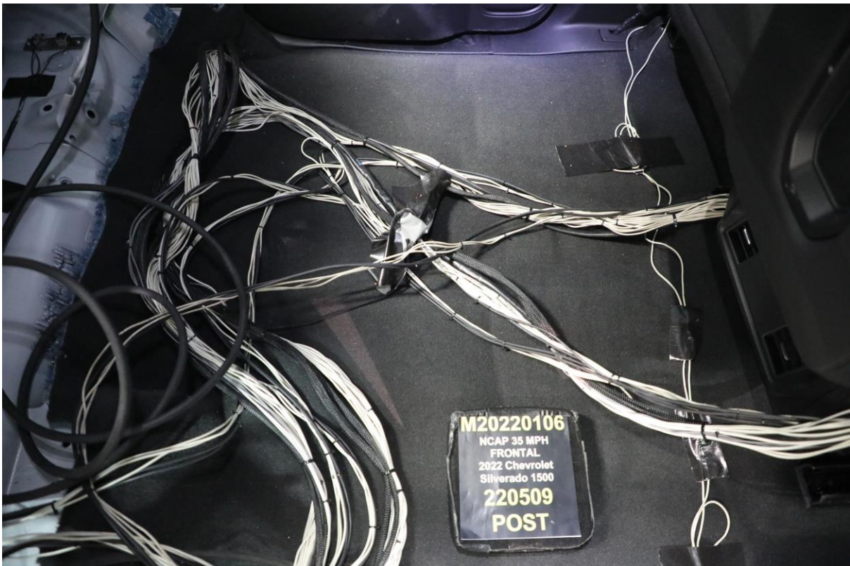
029 Post-Test Dummy Cable Routing
