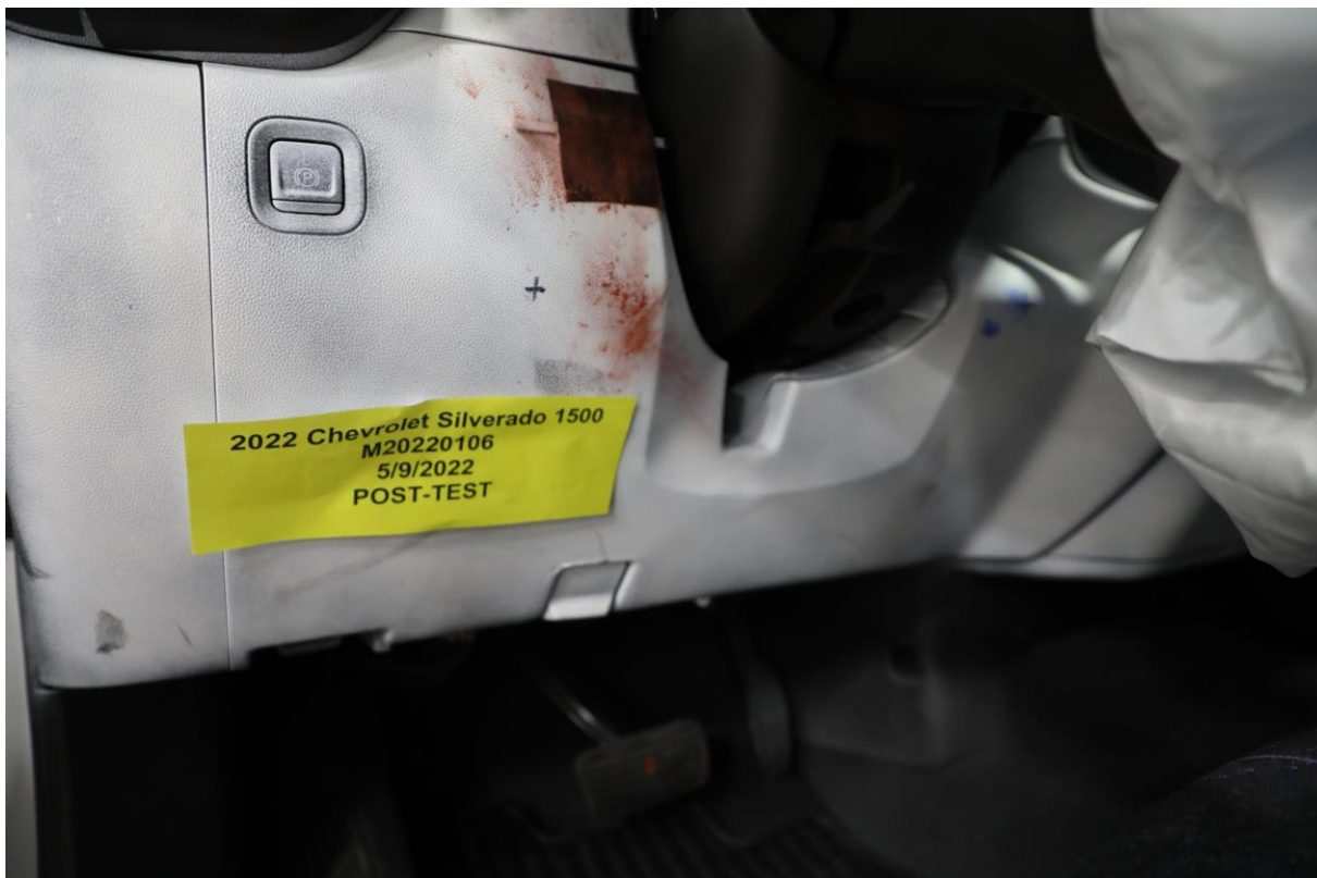
045 Post-Test Driver's Side Knee Bolster
