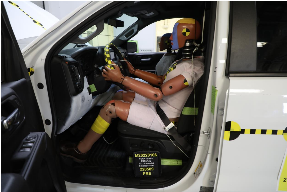
034 Pre-Test Driver Dummy and Vehicle Interior View
