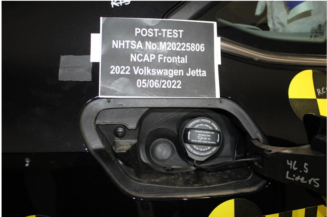
Figure A-23: Post-Test Fuel Filler Cap View
