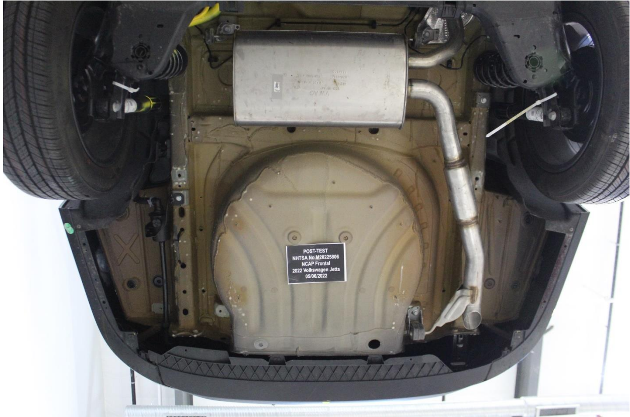
Figure A-27: Post-Test Rear Underbody View
