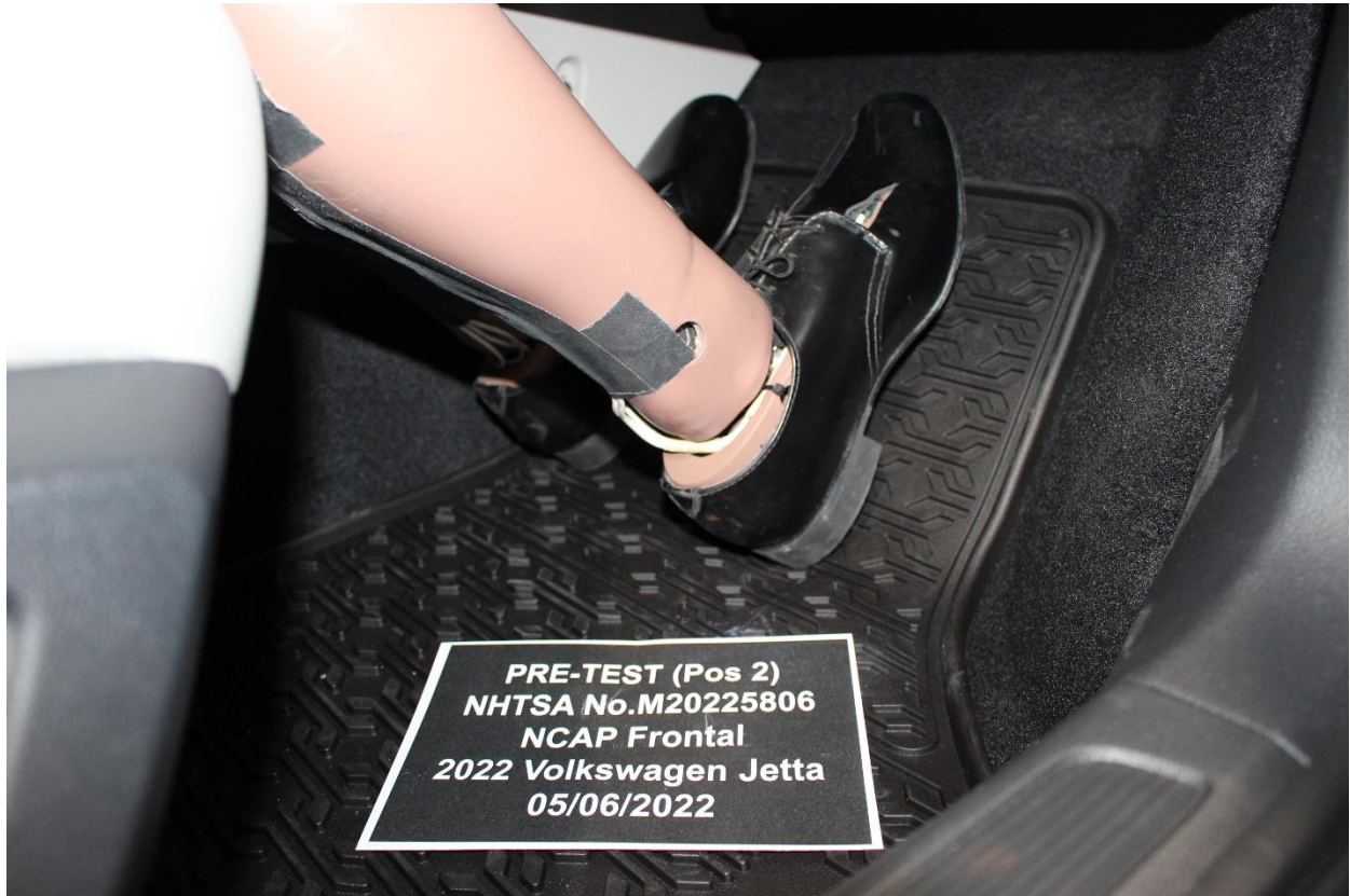
Figure A-65: Pre-Test Passenger Dummy Feet
