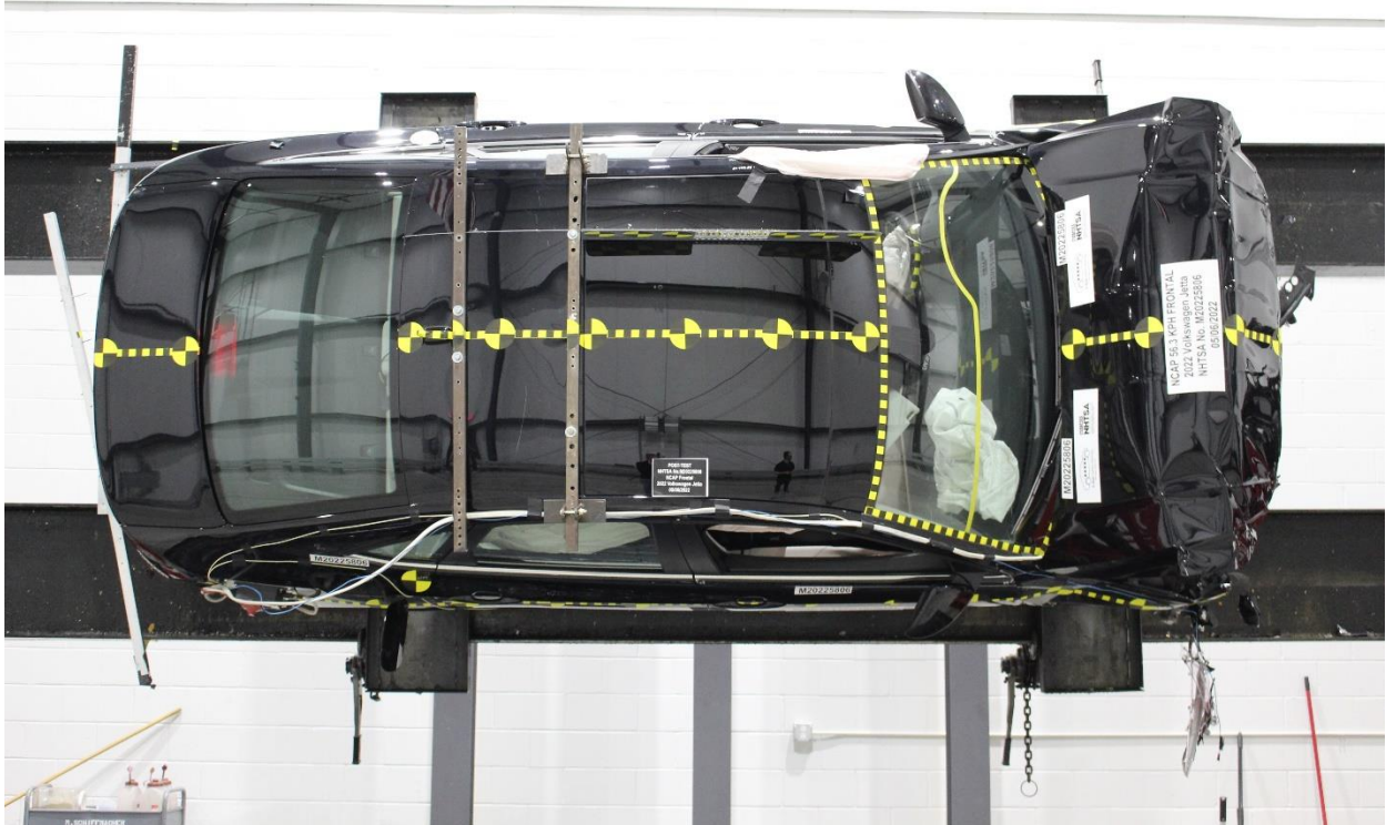
Figure A-78: Vehicle at 90° on Static Rollover Device
