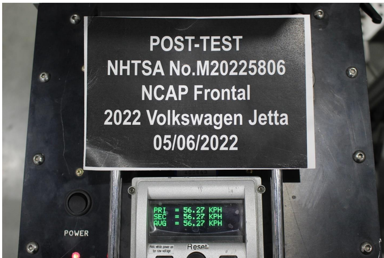
Figure A-76: Post-Test Speed Trap Read-Out
