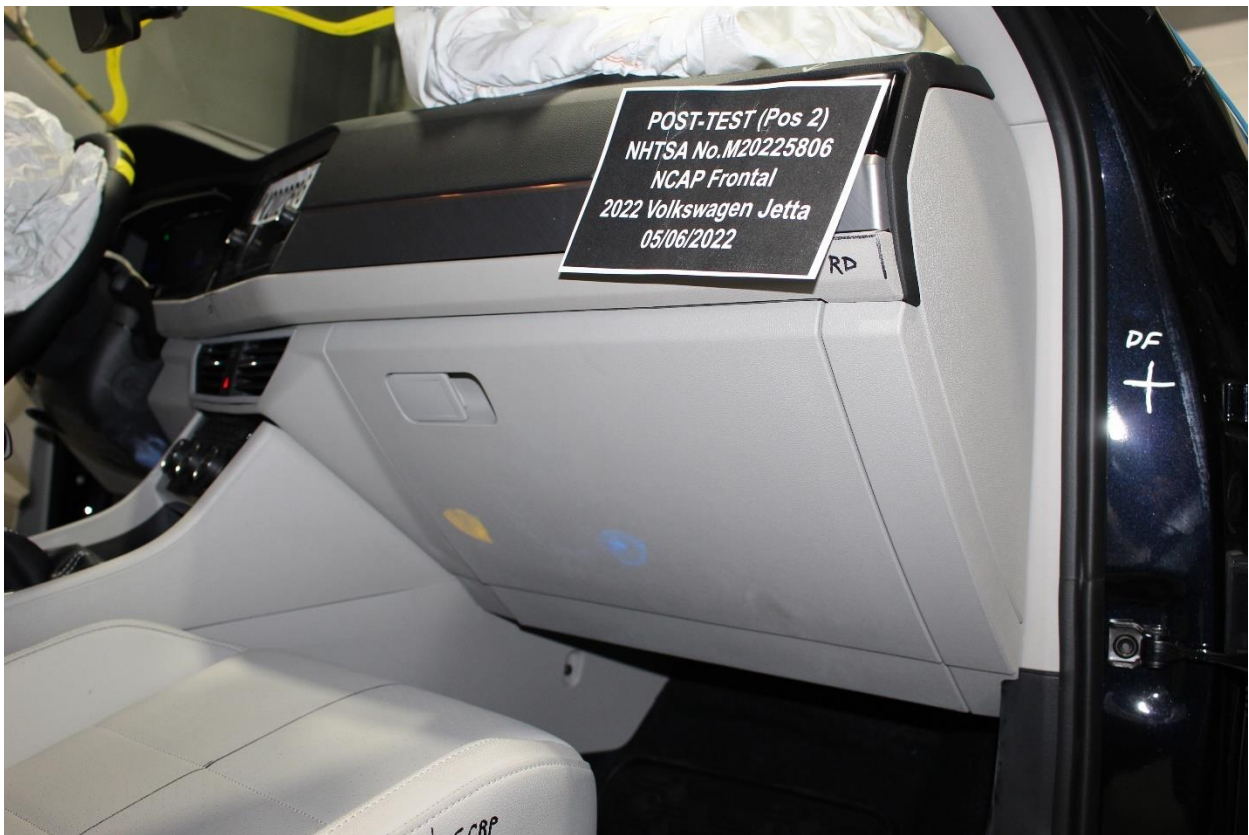
Figure A-68: Post-Test Passenger's Side Knee Bolster
