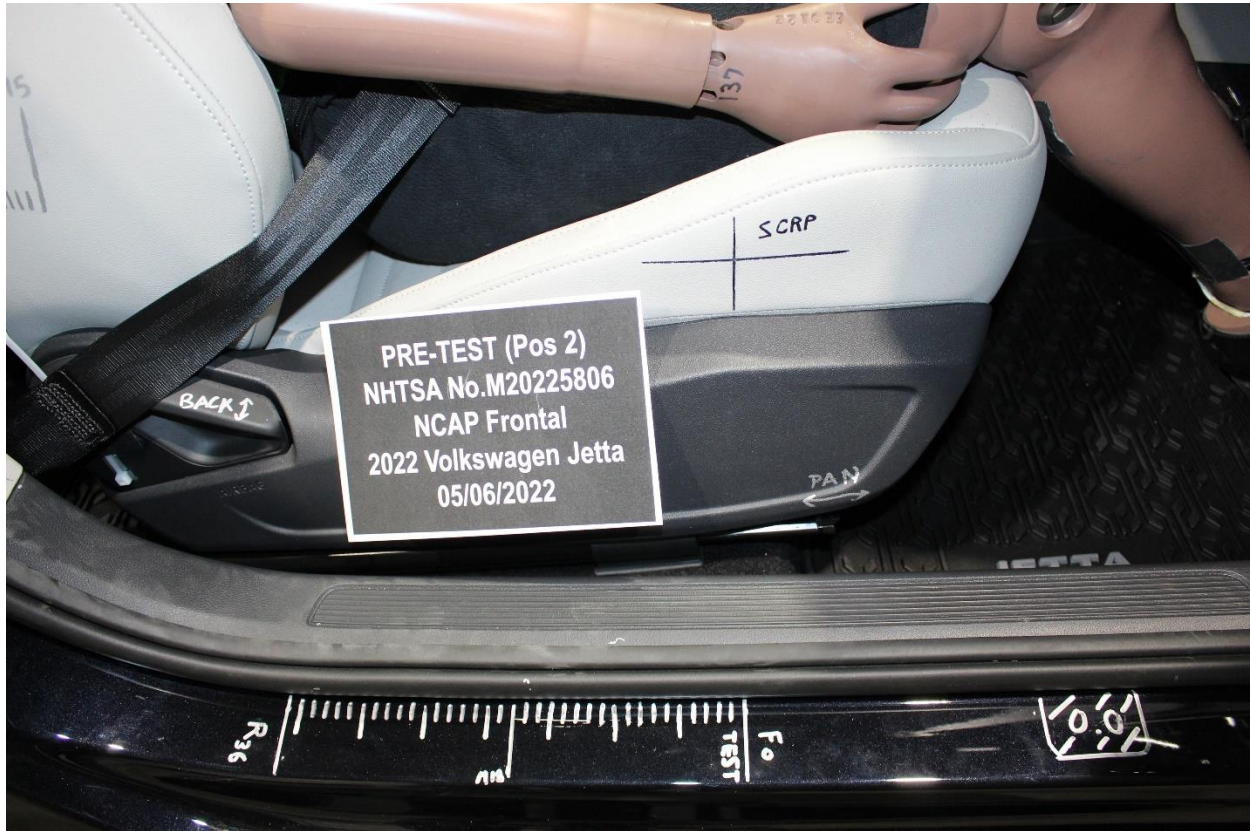
Figure A-59: Pre-Test Passenger's Seat Fore-Aft Markings
