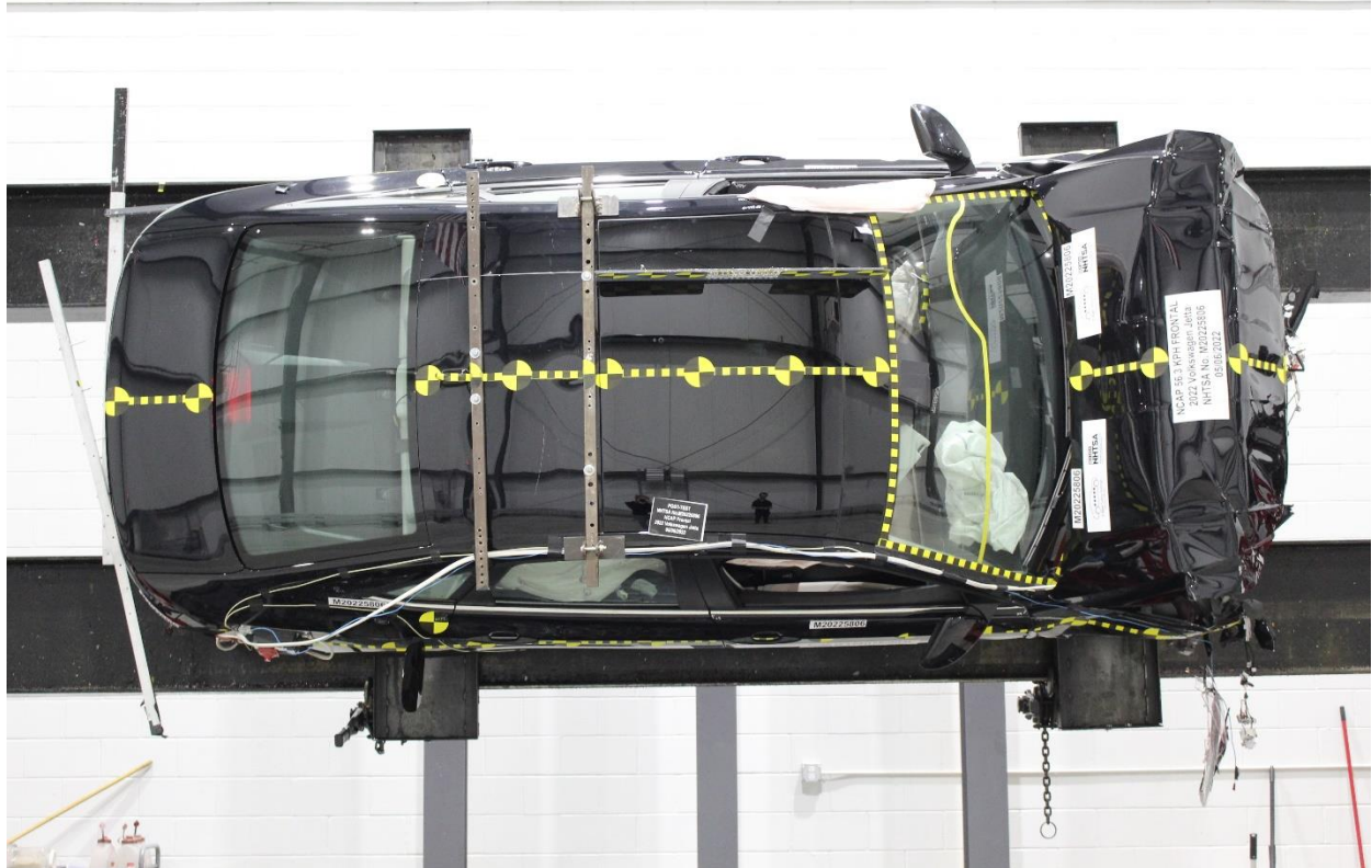
Figure A-80: Vehicle at 270° on Static Rollover Device
