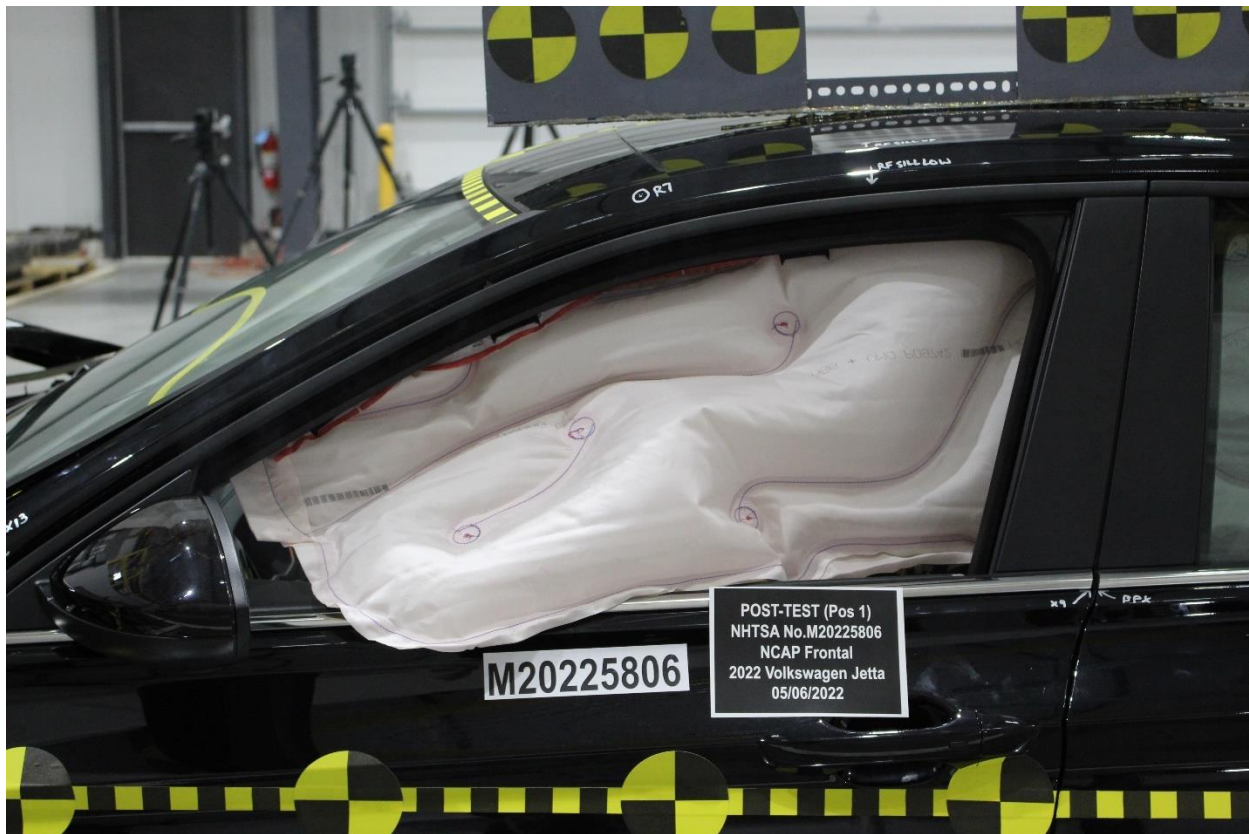
Figure A-33: Post-Test Driver Dummy Window View
