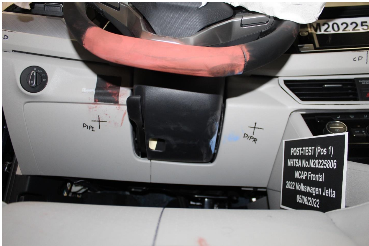
Figure A-45: Post-Test Driver's Side Knee Bolster
