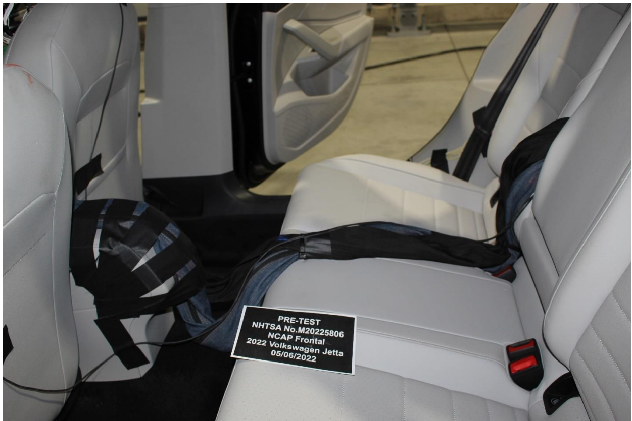
Figure A-28: Pre-Test Dummy Cable Routing
