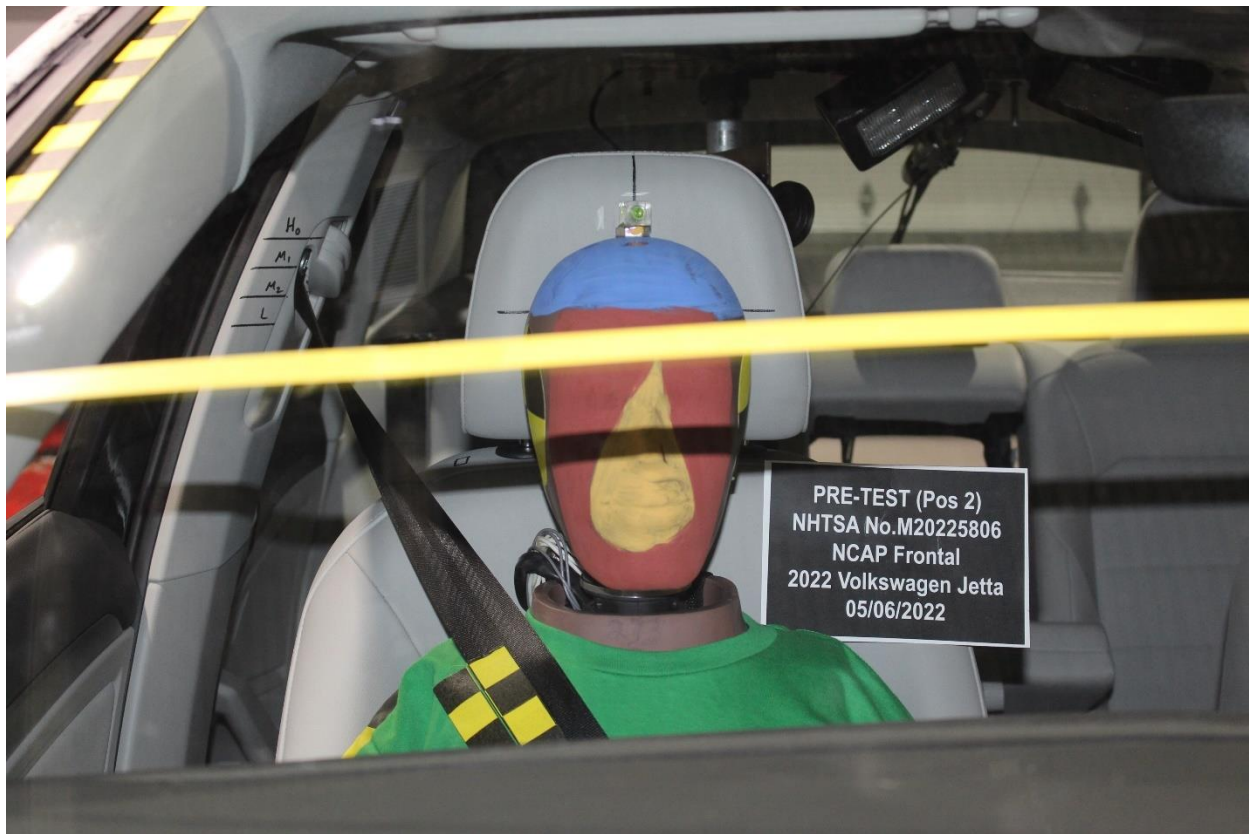
Figure A-53: Pre-Test Passenger Dummy Front View
