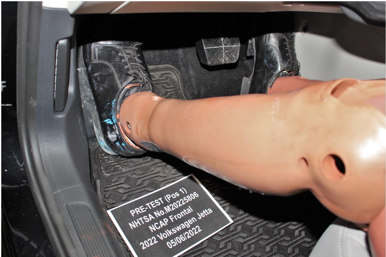
Figure A-42: Pre-Test Driver Dummy Feet
