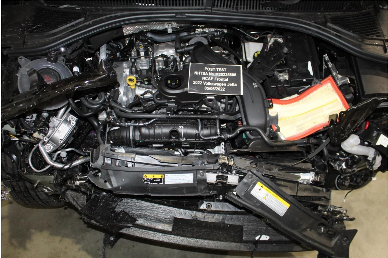
Figure A-21: Post-Test Engine Compartment View
