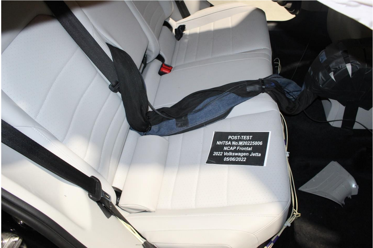
Figure A-29: Post-Test Dummy Cable Routing
