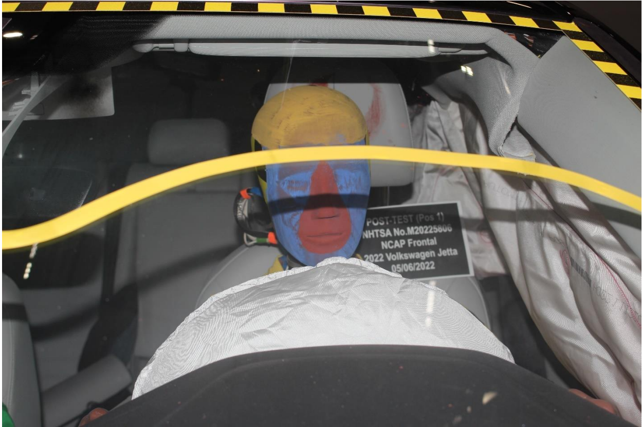
Figure A-31: Post-Test Driver Dummy Front View
