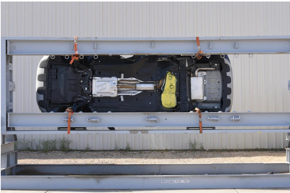
FIGURE 66. FMVSS No. 301 Static Rollover 90 Degrees
