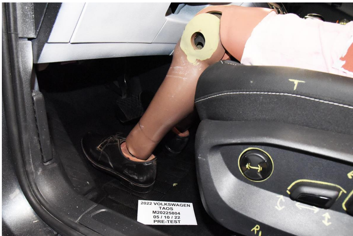
FIGURE 32. Pre-Test Placement of Dummy's Feet
