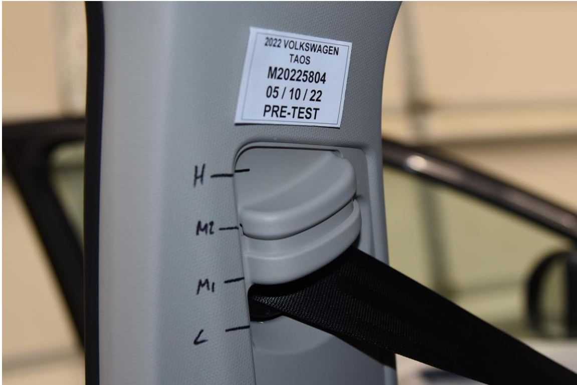
FIGURE 33. Pre-Test View of Belt Anchorage for Dummy
