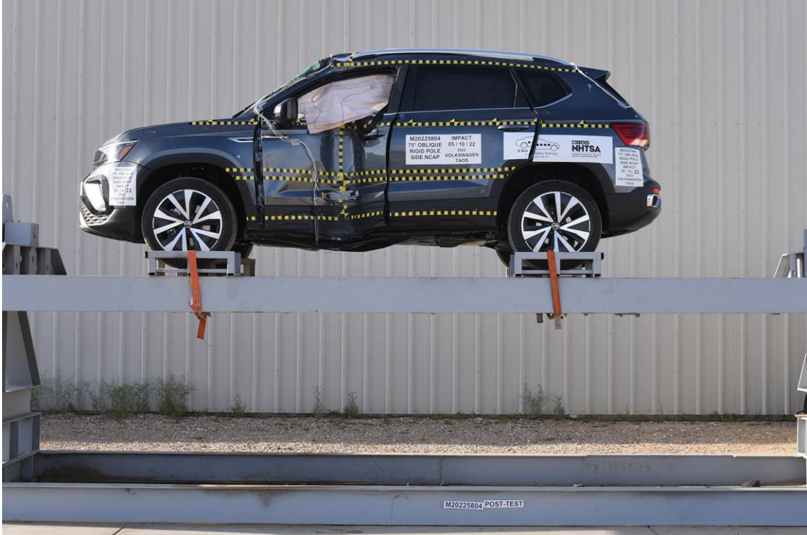
FIGURE 69. FMVSS No. 301 Static Rollover 360 Degrees
