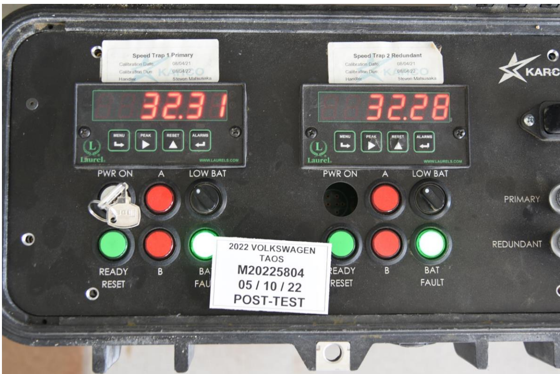
FIGURE 64. Post-Test Primary and Redundant Speed Trap Read-Out
