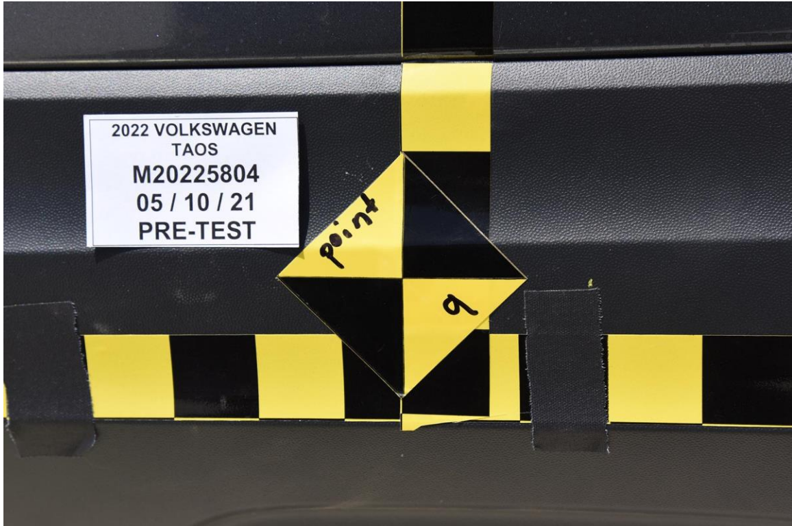
FIGURE 19. Pre-Test Close-Up View of Impact Point Target
