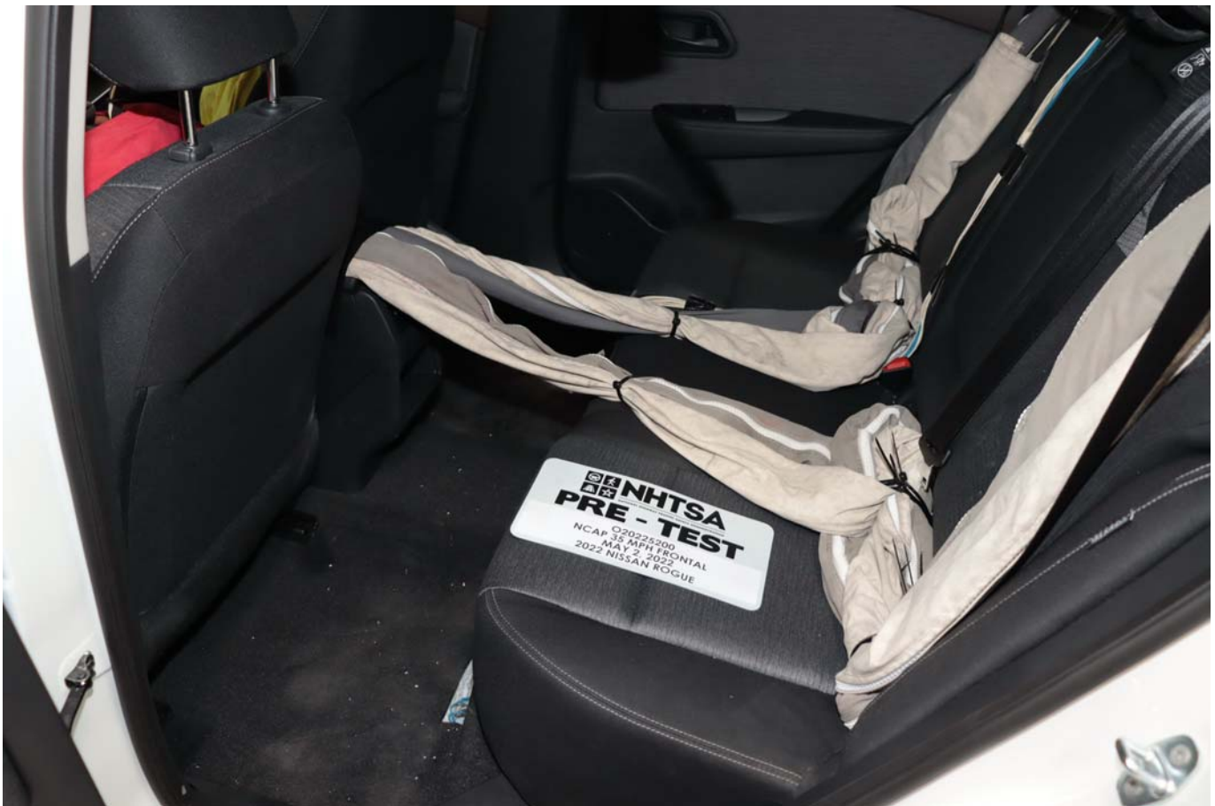
Photo No. 028 - Pre-Test Dummy Cable Routing
