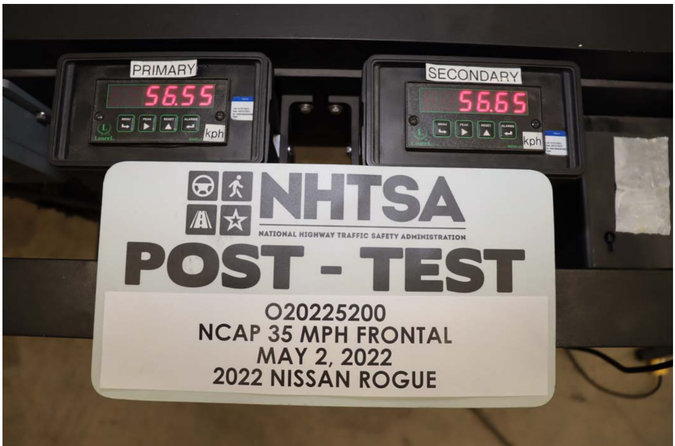
Photo No. 076 - Post-Test Speed Trap Read-Out
