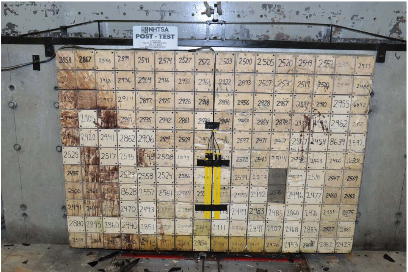
Photo No. 003 - Post-Test Load Cell Wall
