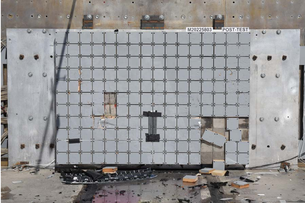
FIGURE 3. Post-Test Load Cell Wall
