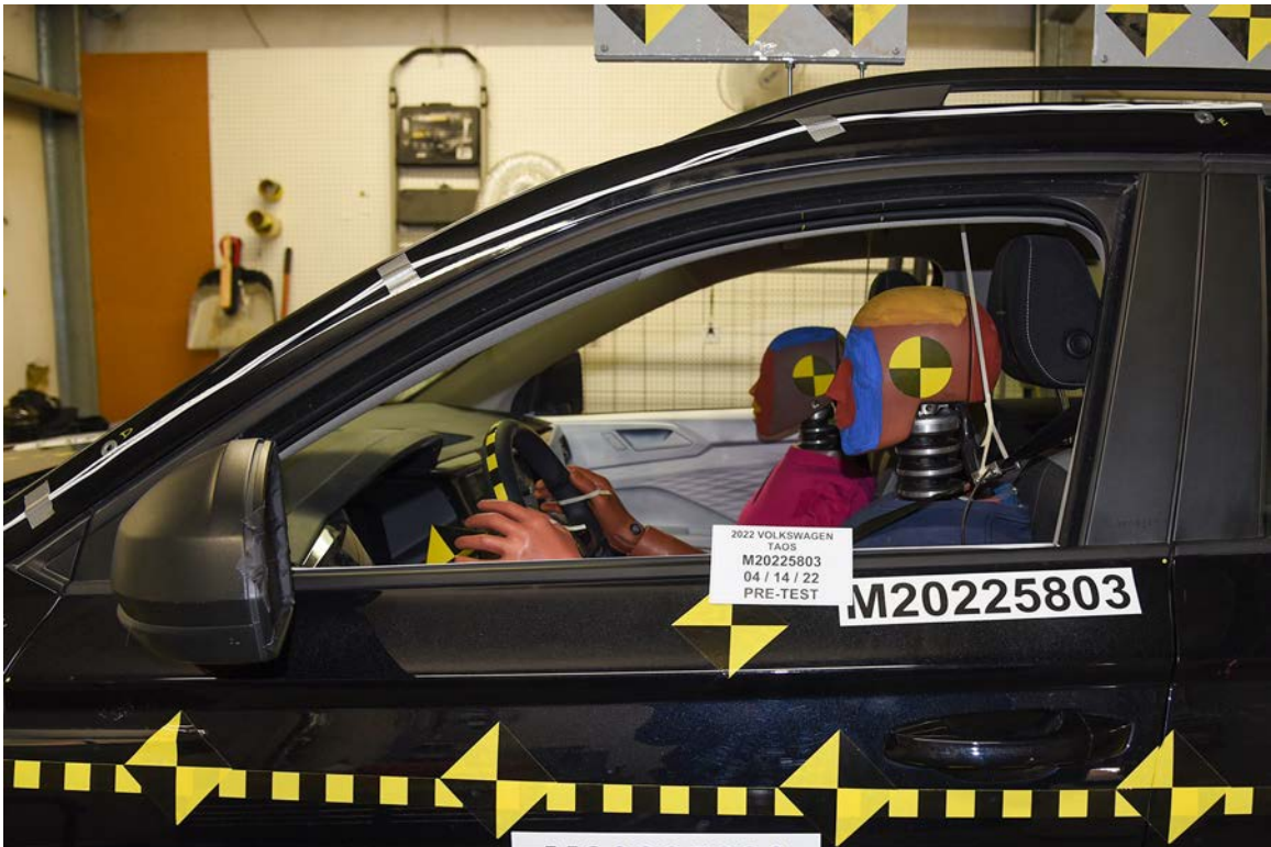
FIGURE 32. Pre-Test Driver Dummy Window View
