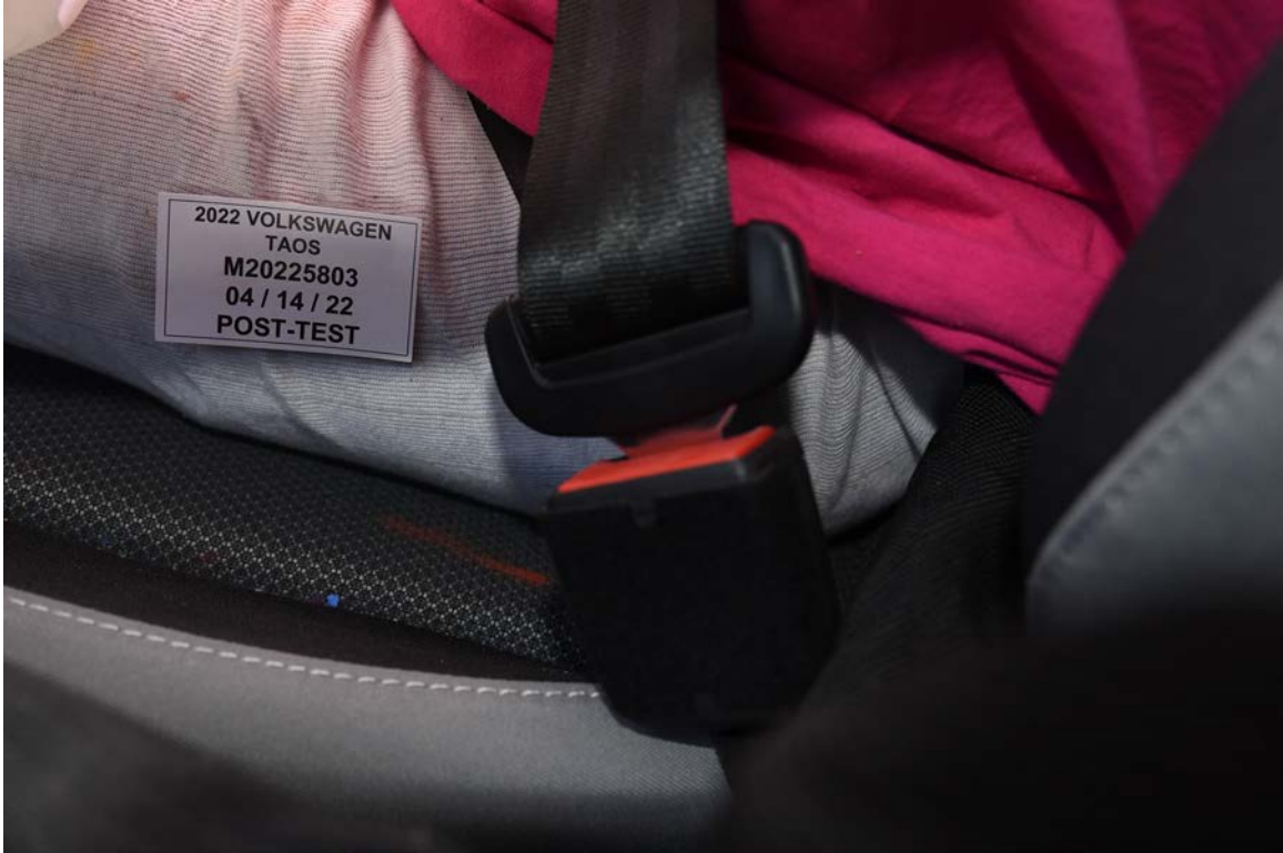
FIGURE 64. Post-Test View of Belt Buckle and Latch Plate for Passenger Dummy
