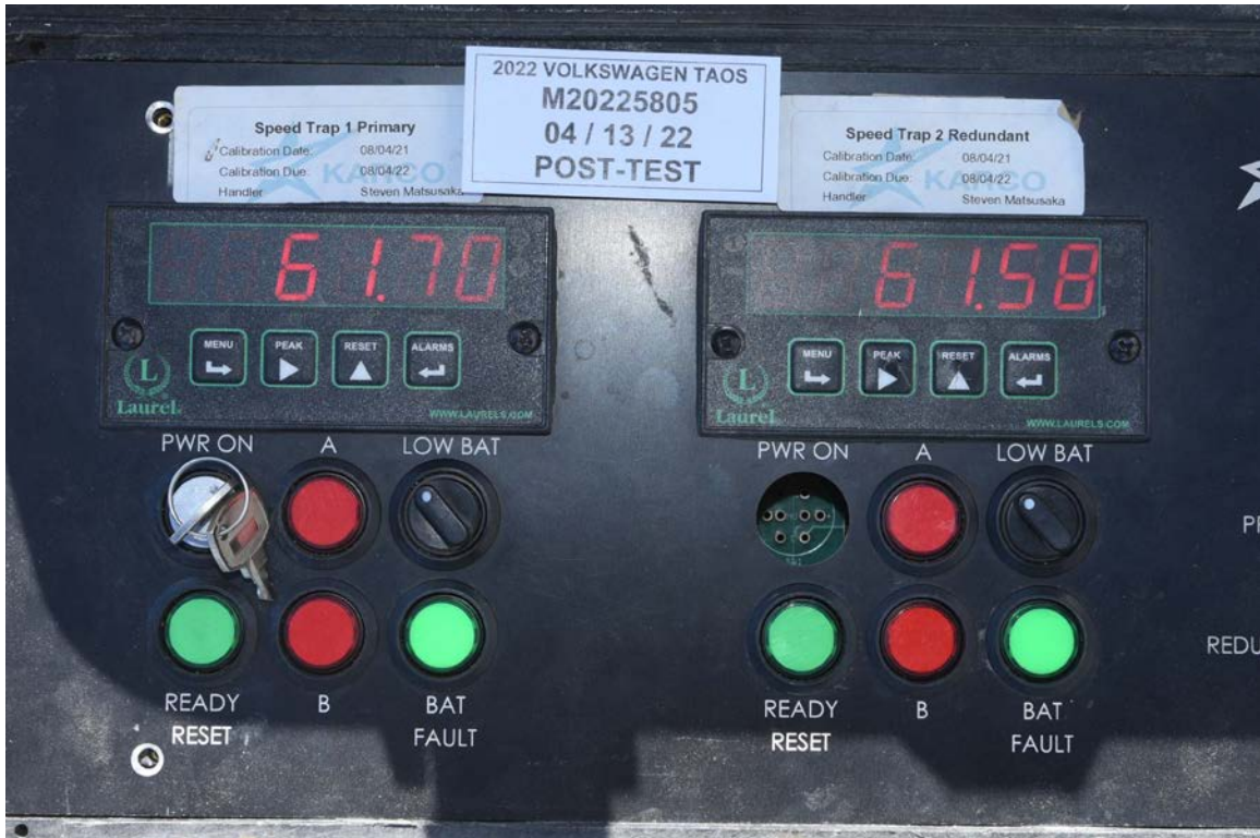
FIGURE 95. Post-Test Primary and Redundant Speed Trap Read-Out
