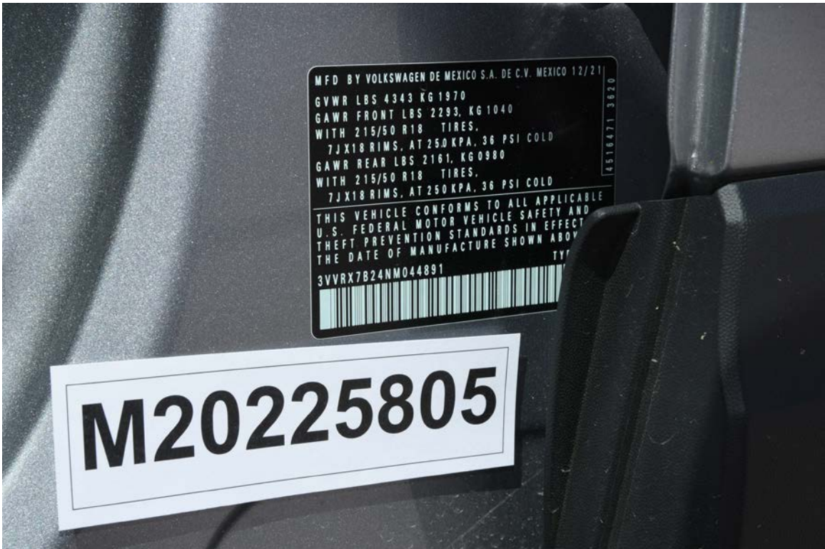
FIGURE 92. Close-Up View of Vehicle's Certification Label
