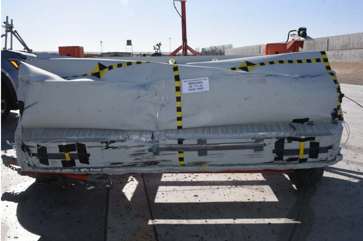
FIGURE 85. Post-Test Front View of MDB Impactor Face
