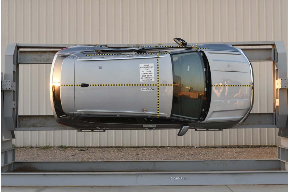
FIGURE 97. FMVSS No. 301 Static Rollover 90 Degrees
