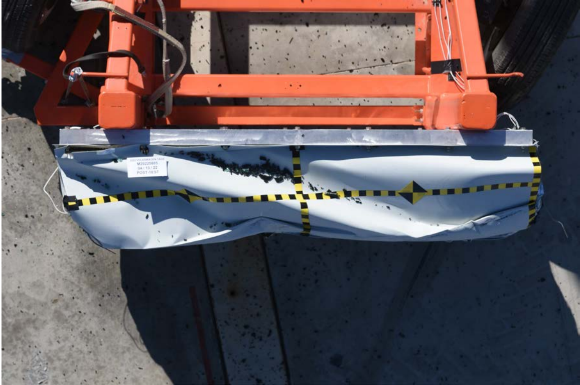
FIGURE 87. Post-Test Top View of MDB Impactor Face
