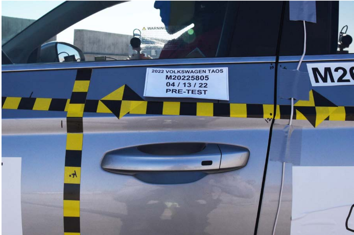
FIGURE 21. Pre-Test Left Front Door Latch Close-Up
