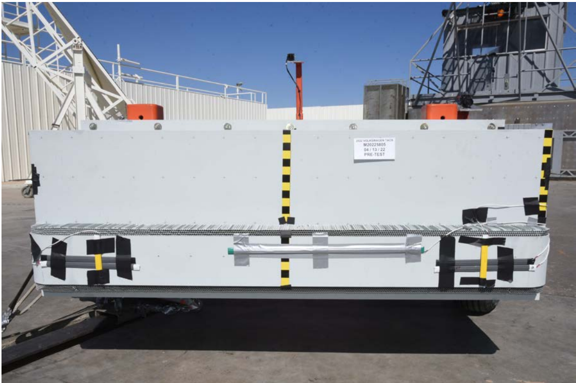
FIGURE 84. Pre-Test Front View of MDB Impactor Face
