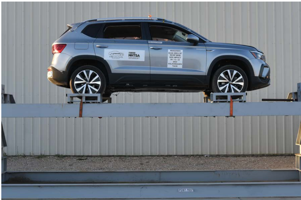
FIGURE 96. FMVSS No. 301 Static Rollover 0 Degrees
