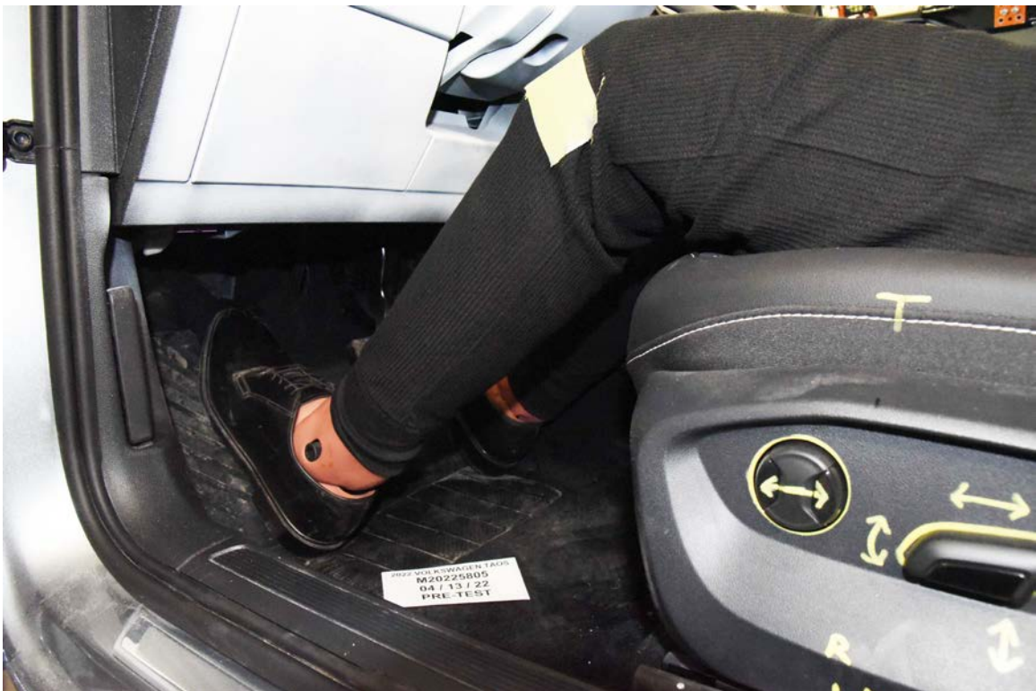
FIGURE 34. Pre-Test Placement of Driver Dummy's Feet
