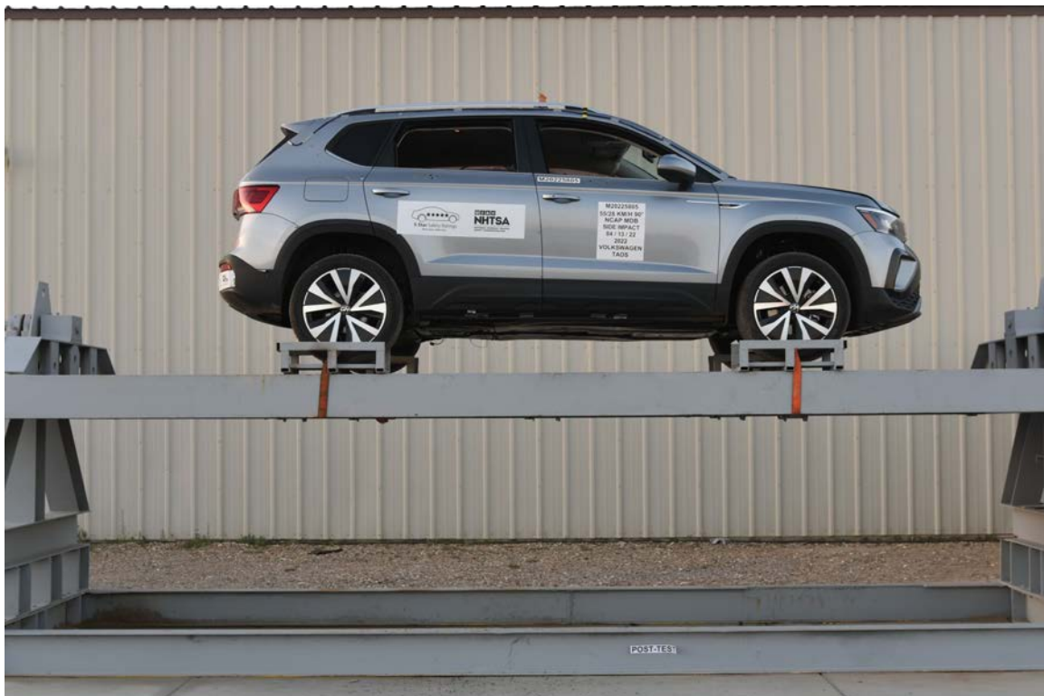
FIGURE 100. FMVSS No. 301 Static Rollover 360 Degrees
