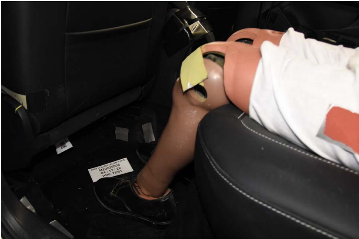
FIGURE 64. Pre-Test Placement of Rear Passenger Dummy's Feet
