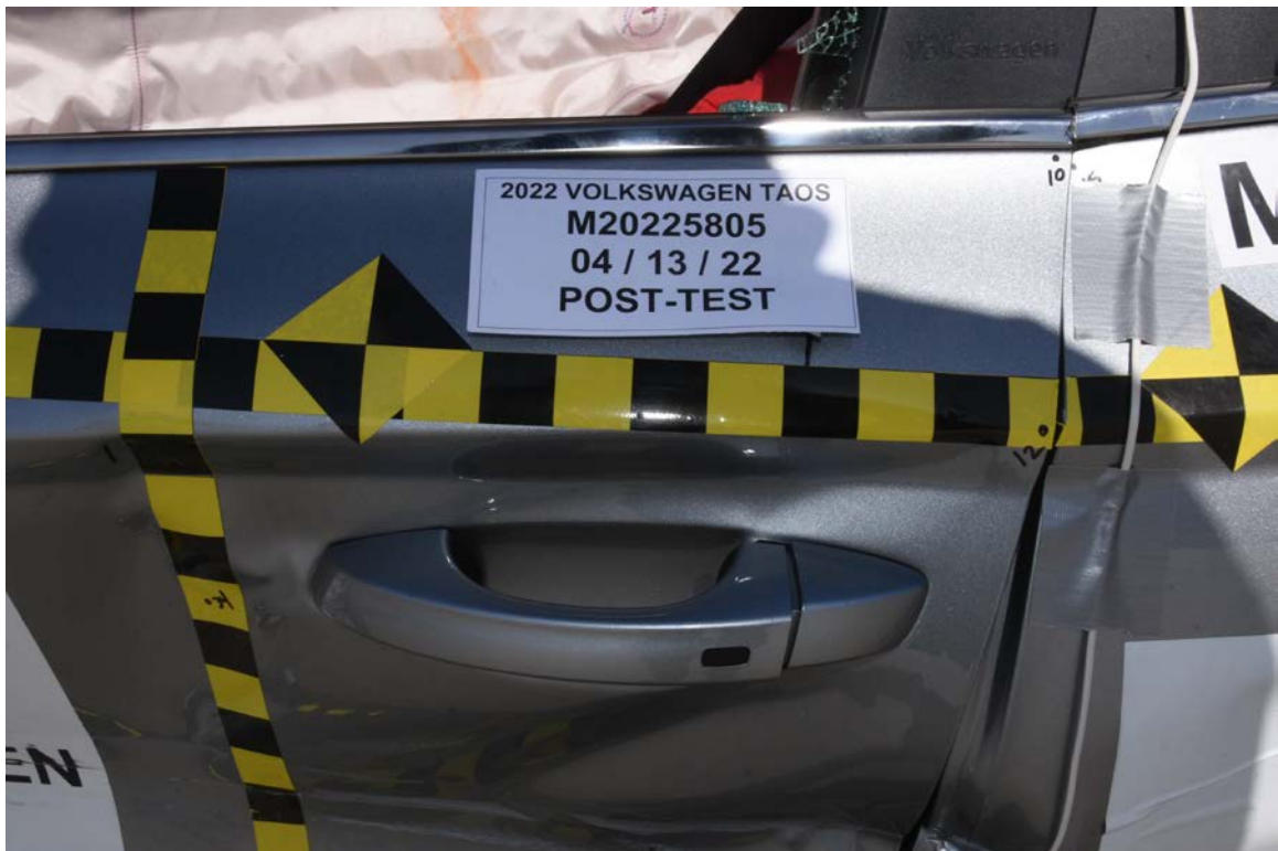
FIGURE 22. Post-Test Left Front Door Latch Close-Up
