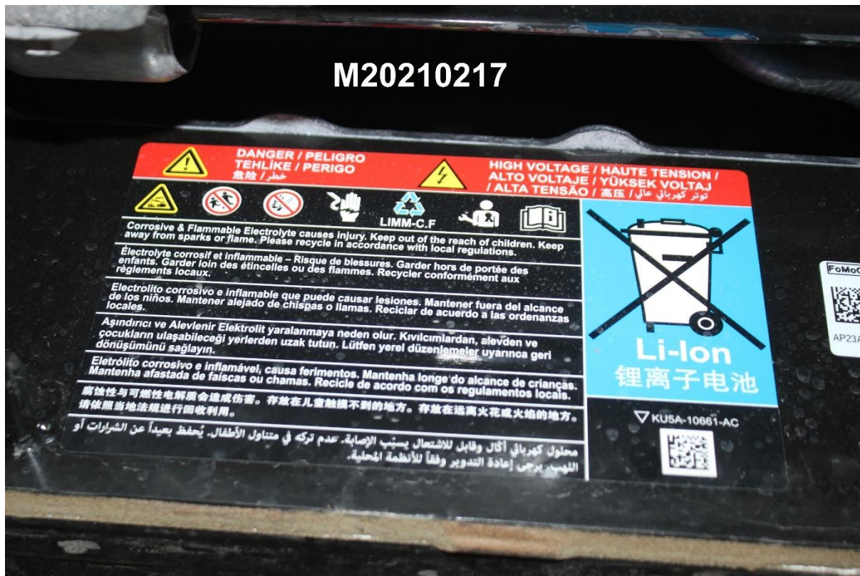
Figure 305-1: Auxiliary Power Module Warning Label
