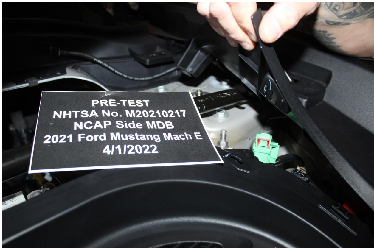
Figure 305-6: Manual High Voltage Service Disconnect in Place
