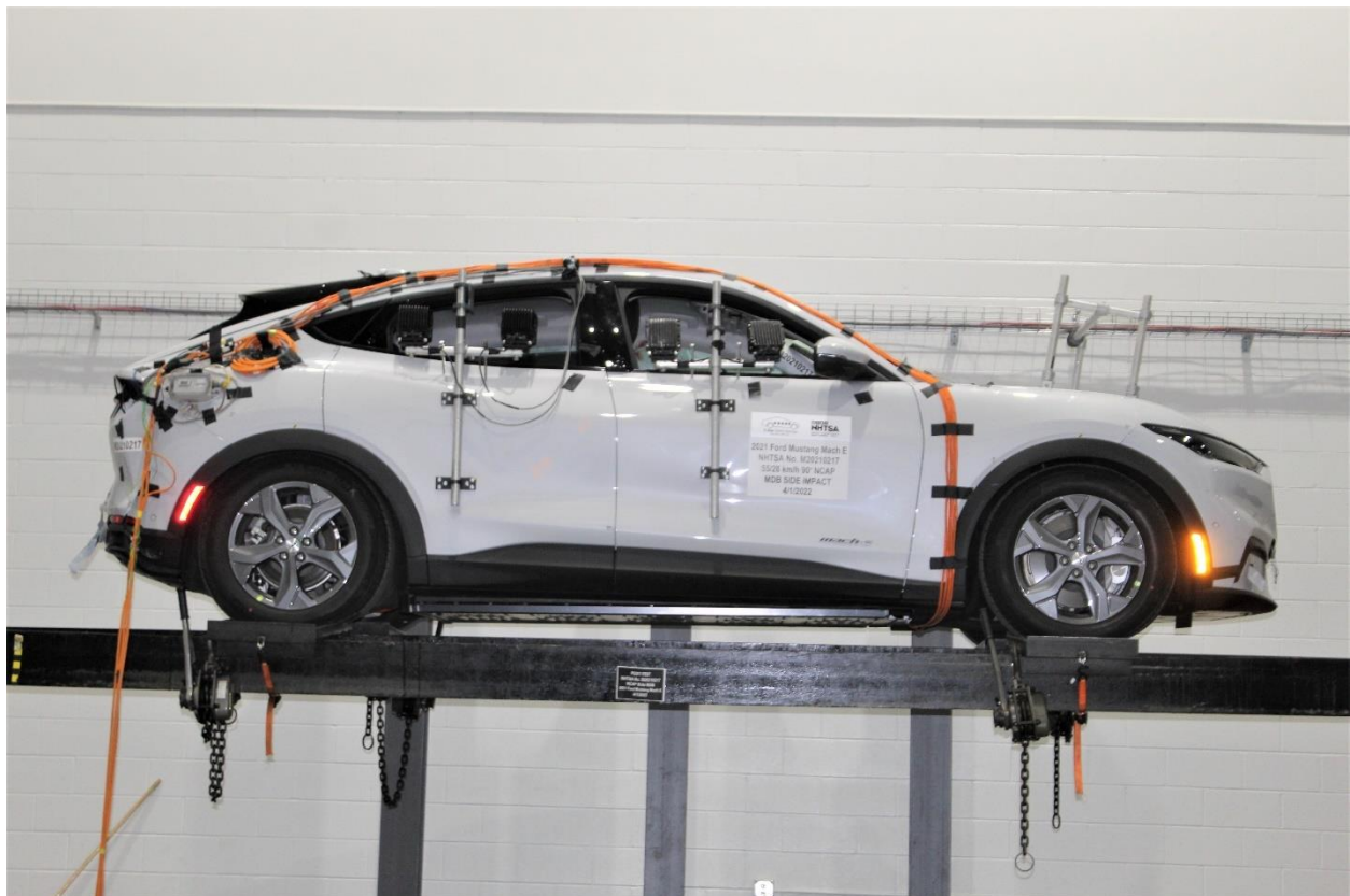
Figure A-100: FMVSS No. 301 Static Rollover 360 Degrees
