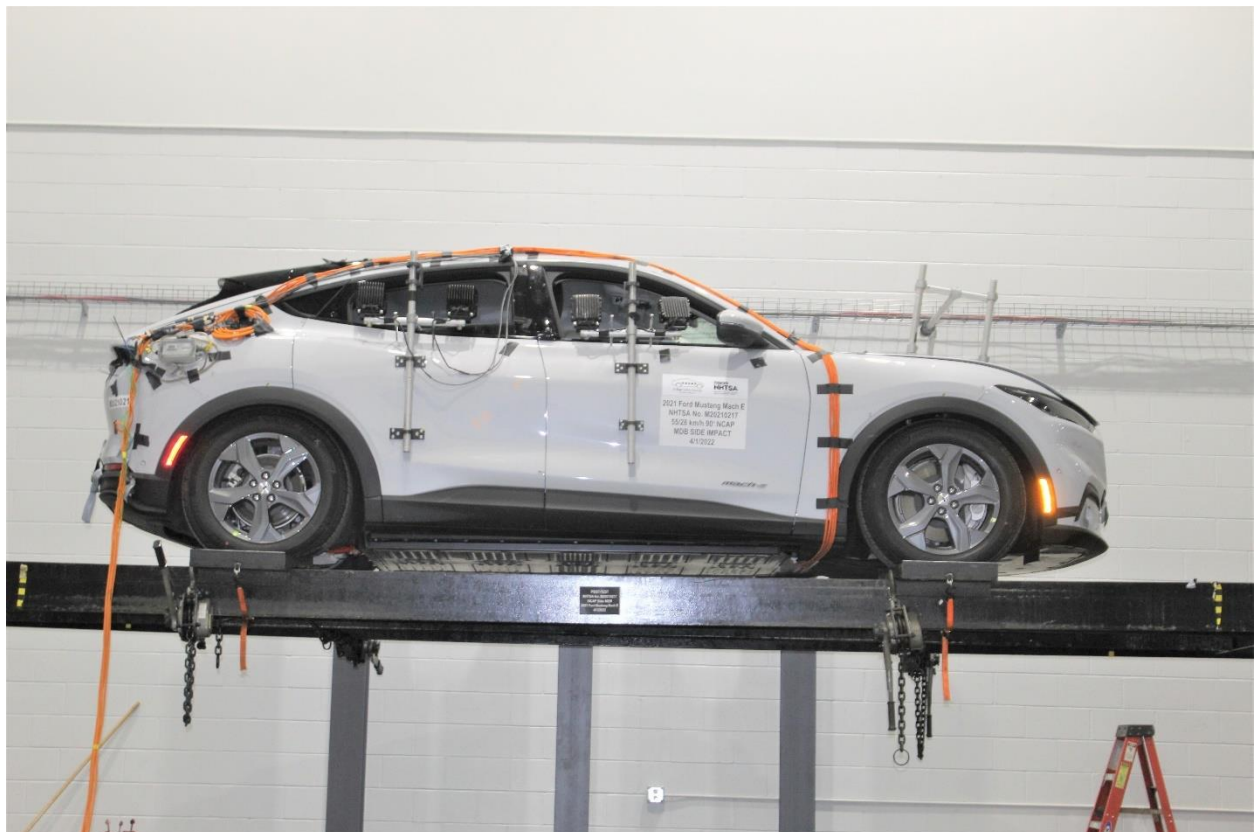
Figure A-96: FMVSS No. 301 Static Rollover 0 Degrees
