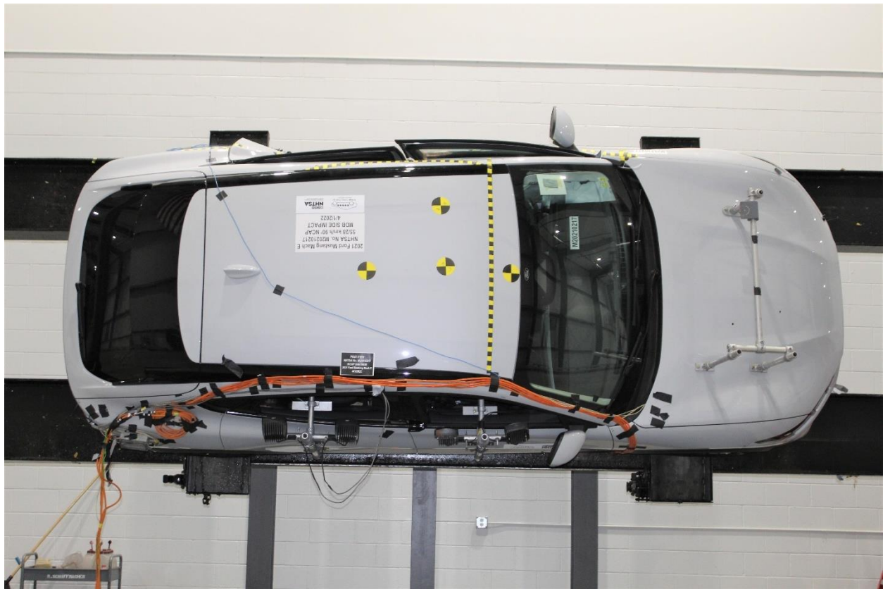
Figure A-99: FMVSS No. 301 Static Rollover 270 Degrees
