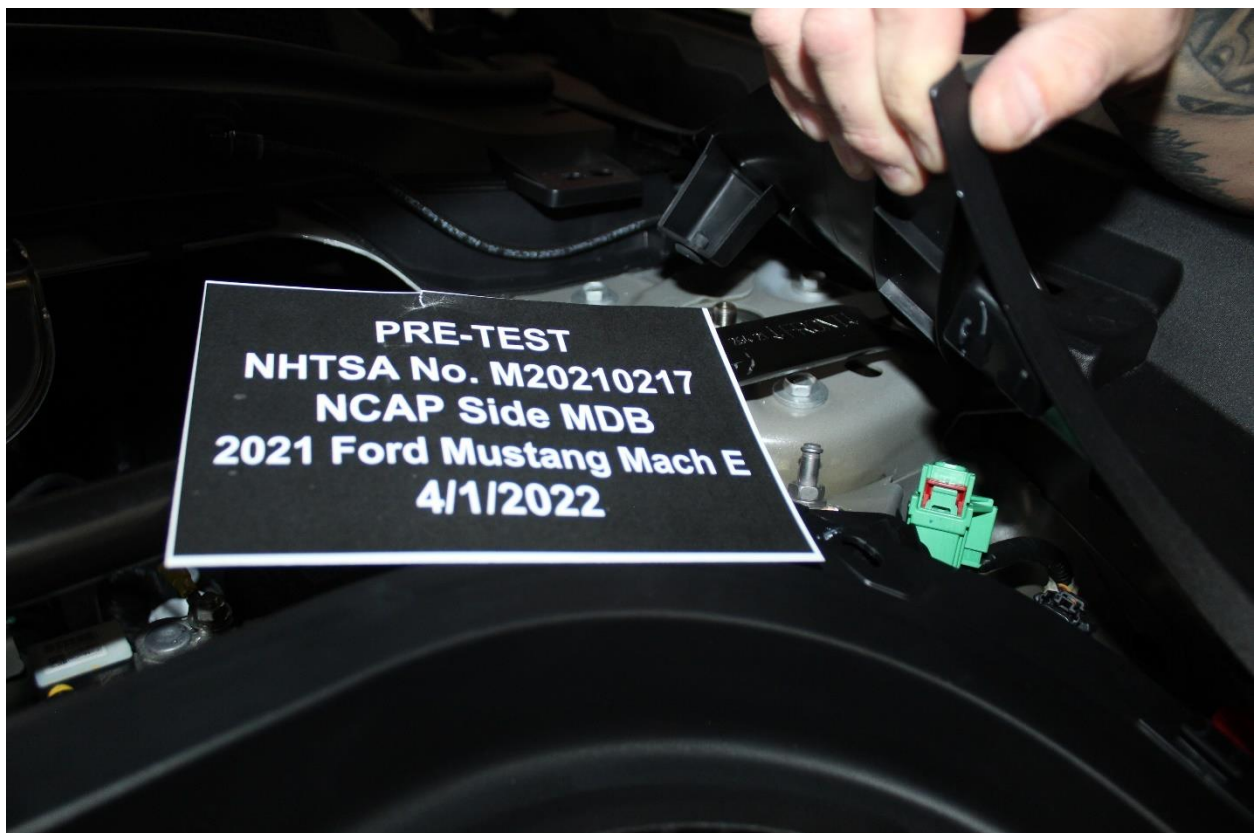
Figure 305-8: Manual High Voltage Service Disconnect Removed Location
