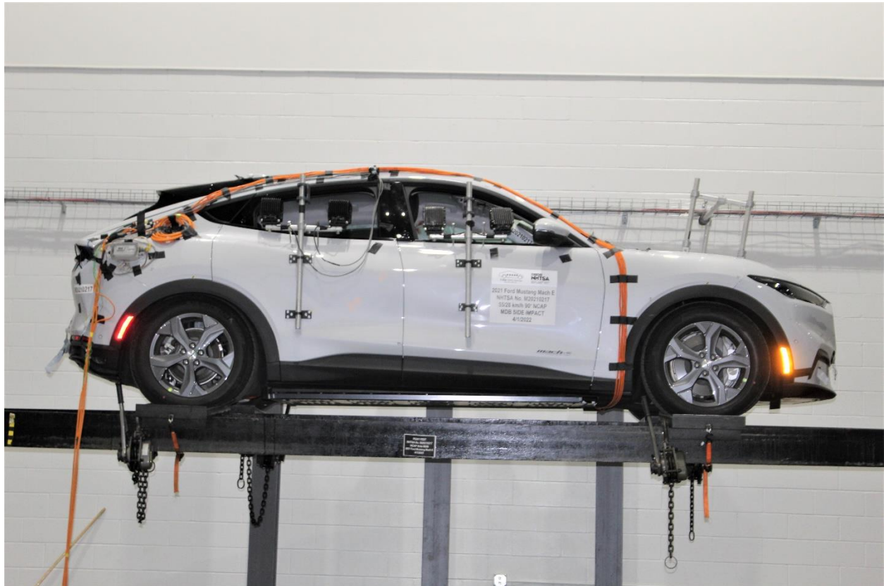
Figure 305-31: FMVSS No. 305 Static Rollover 360 Degrees
