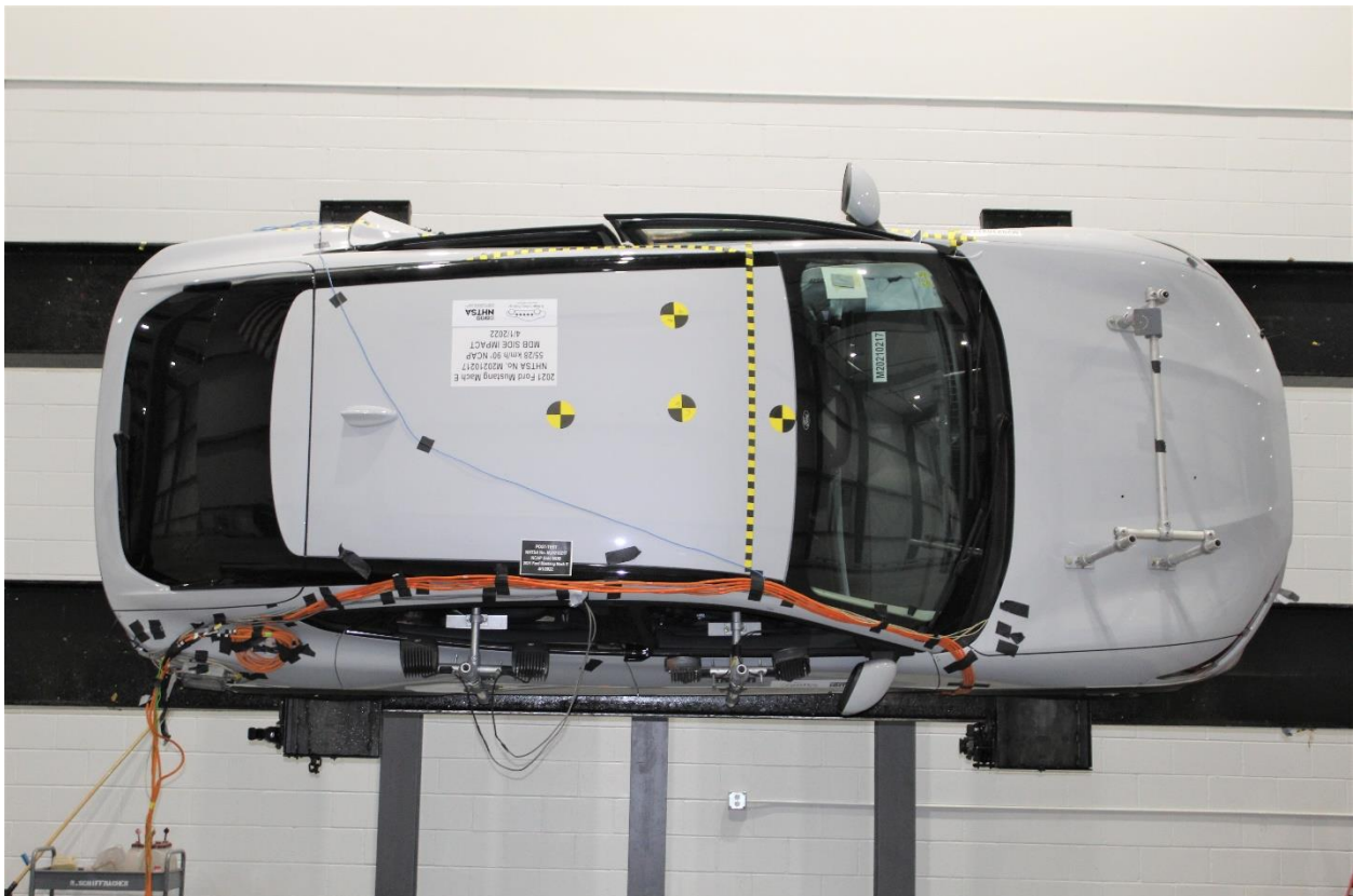
Figure 305-30: FMVSS No. 305 Static Rollover 270 Degrees
