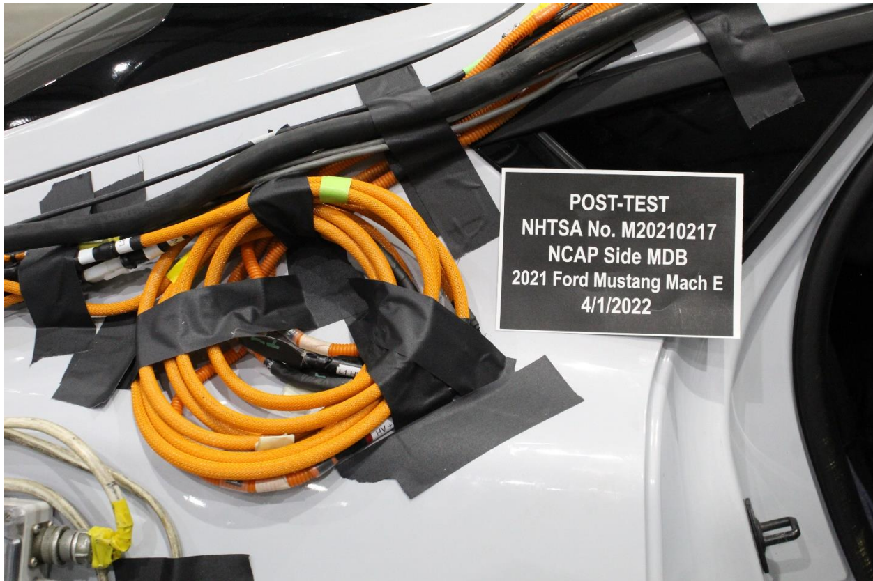
Figure 305-25: Post-Impact View of Installed Test Interface Port
