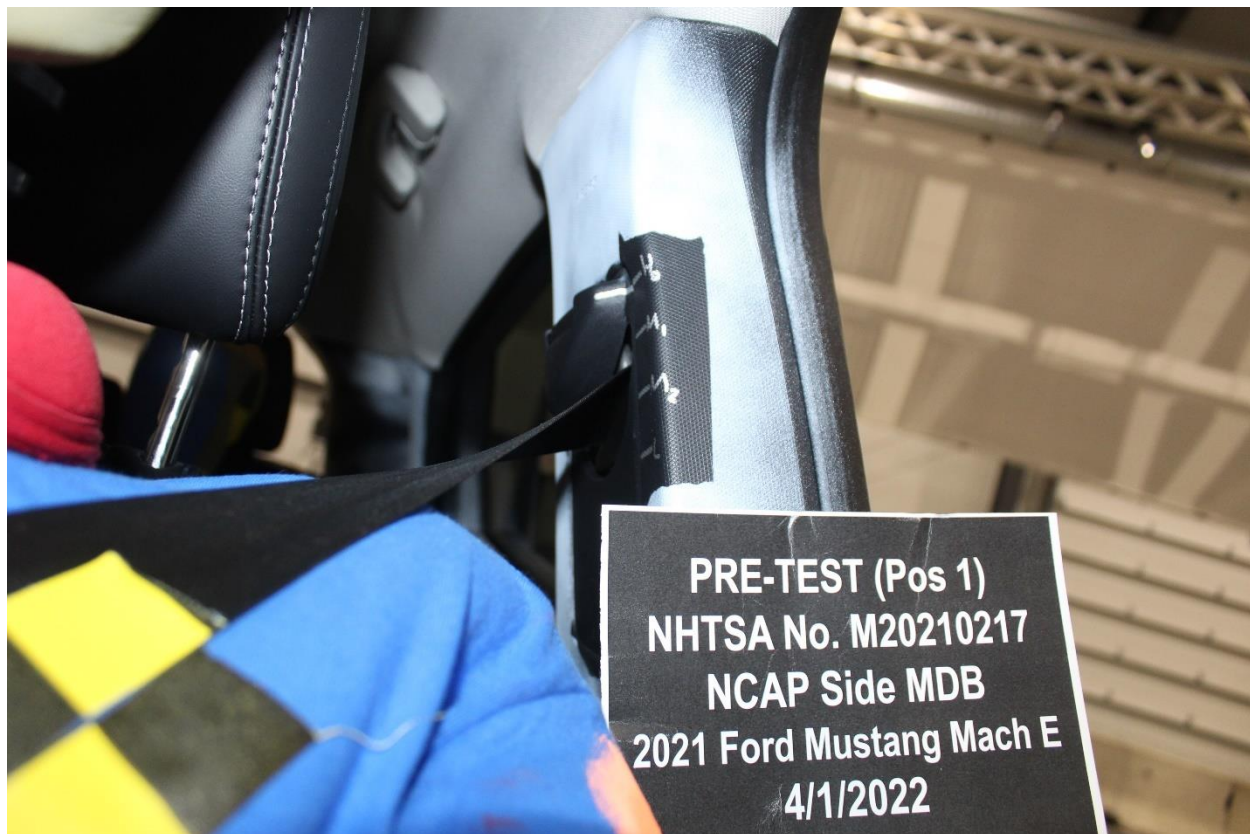
Figure A-35: Pre-Test View of Belt Anchorage for Driver Dummy
