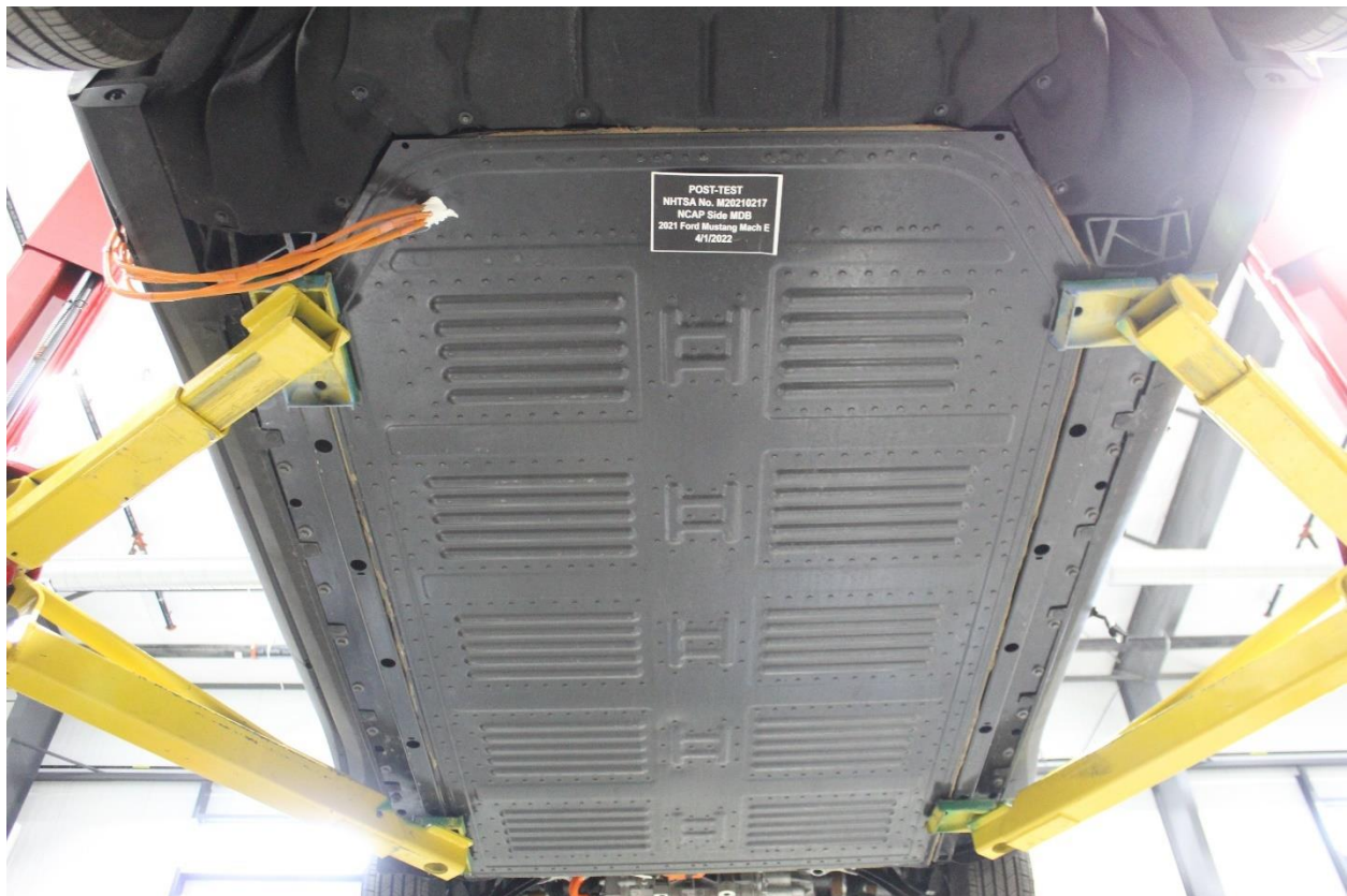
Figure 305-10: Post-Impact Front View of Propulsion Battery
