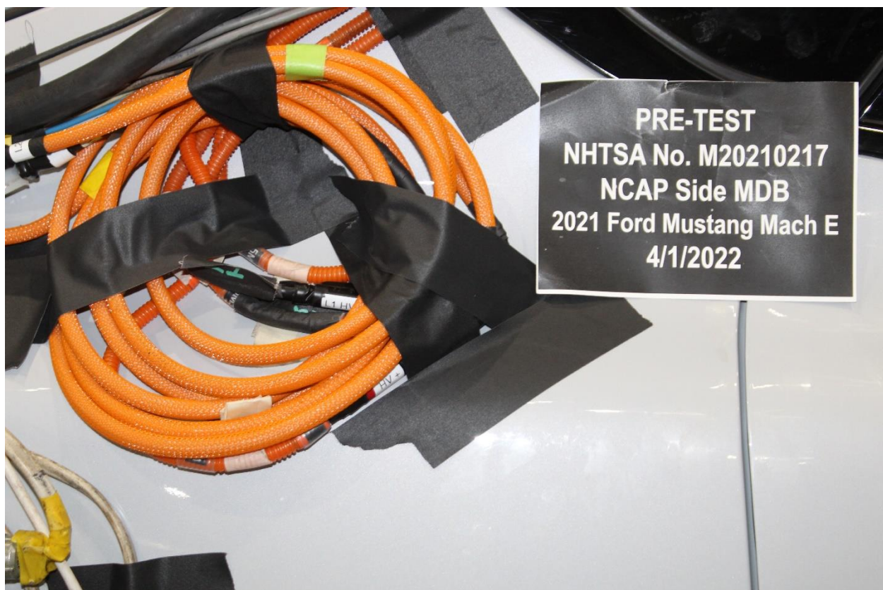
Figure 305-24: Pre-Impact View of Installed Test Interface Port
