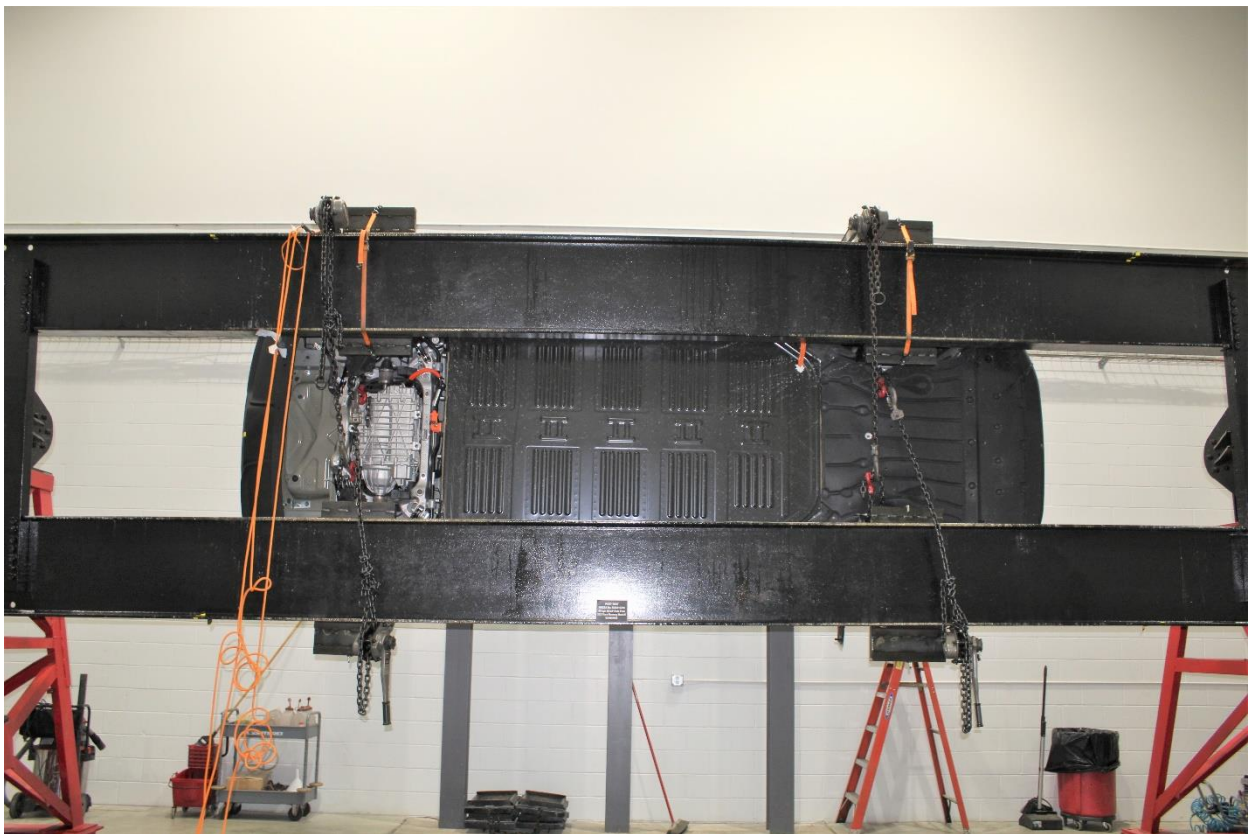
Figure A-66: FMVSS No. 301 Static Rollover 90 Degrees
