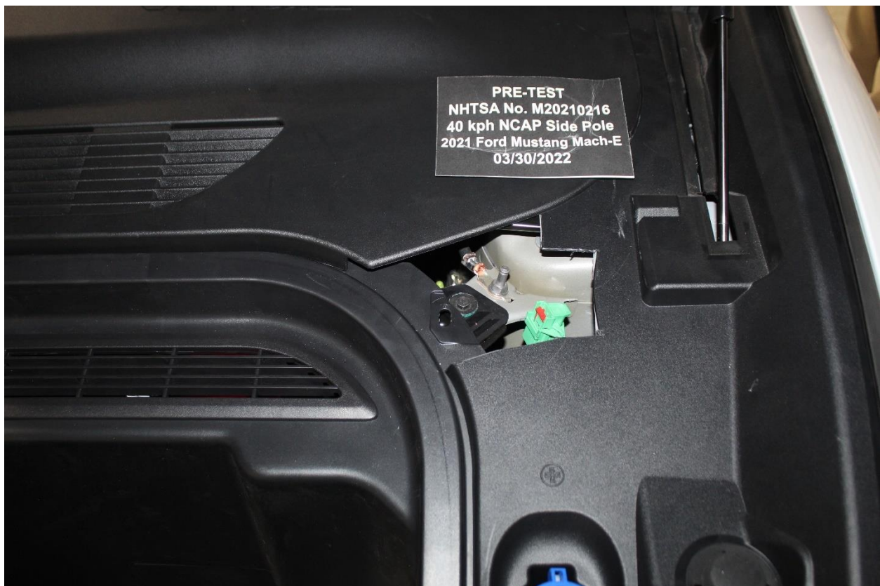
Figure 305-8: Manual High Voltage Service Disconnect Removed Location
