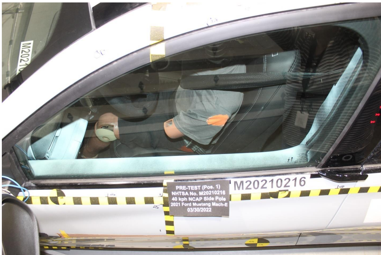
Figure A-40: Pre-Test Dummy and Door Clearance View
