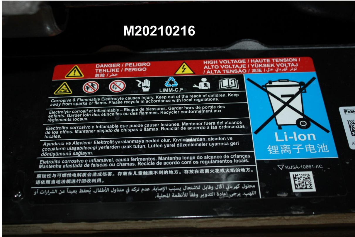
Figure 305-1: Auxiliary Power Module Warning Label
