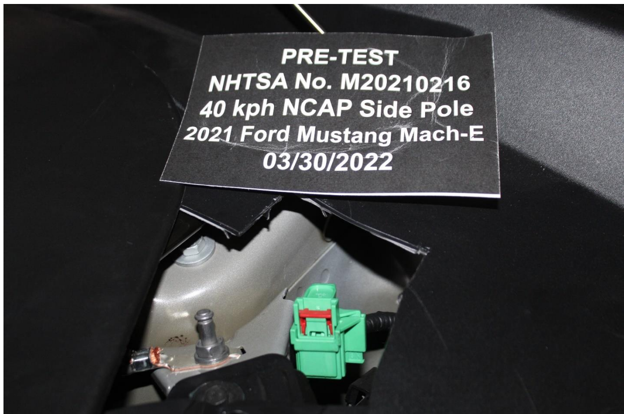
Figure 305-6: Manual High Voltage Service Disconnect in Place
