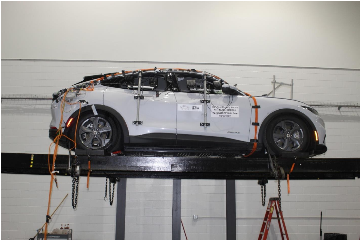
Figure A-69: FMVSS No. 301 Static Rollover 360 Degrees
