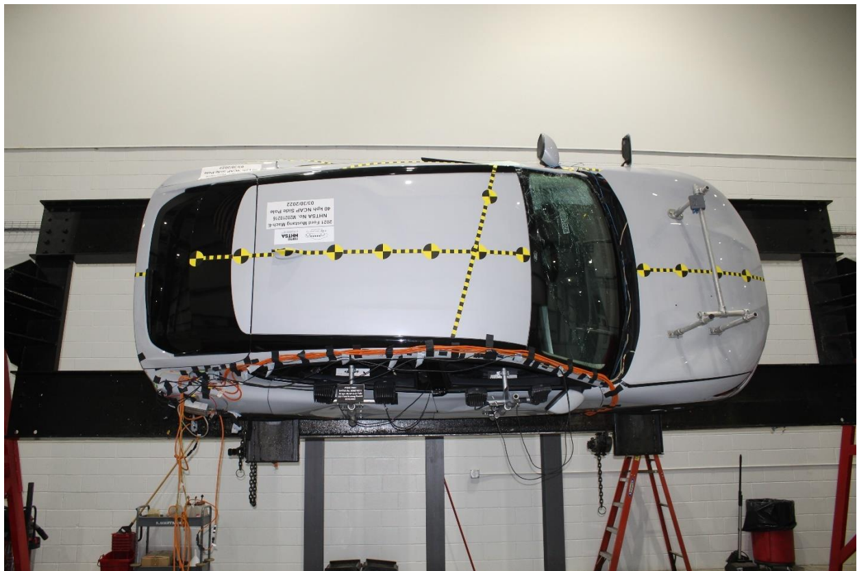
Figure A-68: FMVSS No. 301 Static Rollover 270 Degrees
