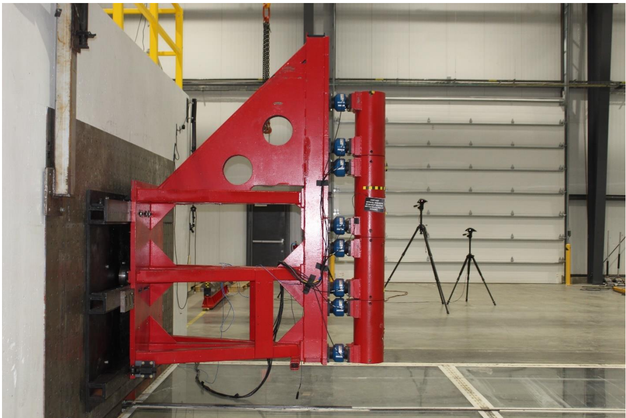
Figure A-62: Post-Test Pole Barrier Side View
