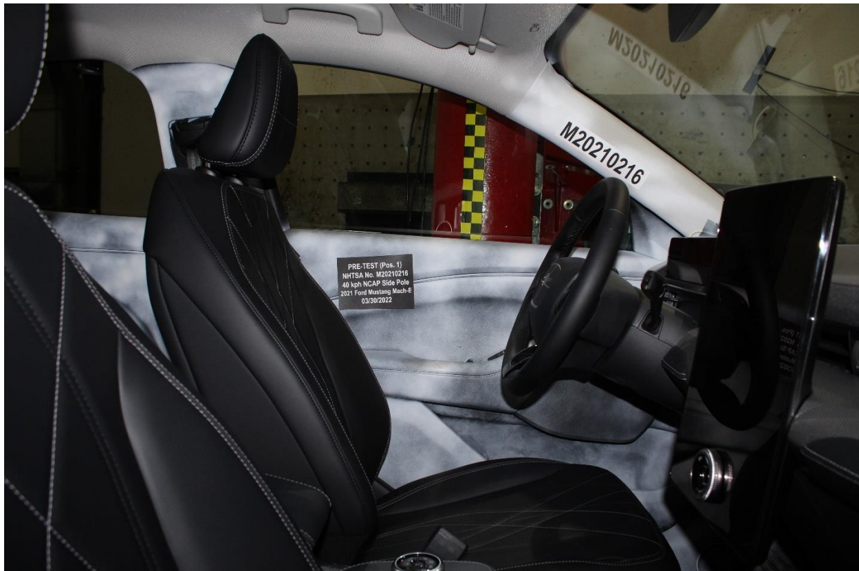
Figure A-44: Pre-Test Inner Door Panel View
