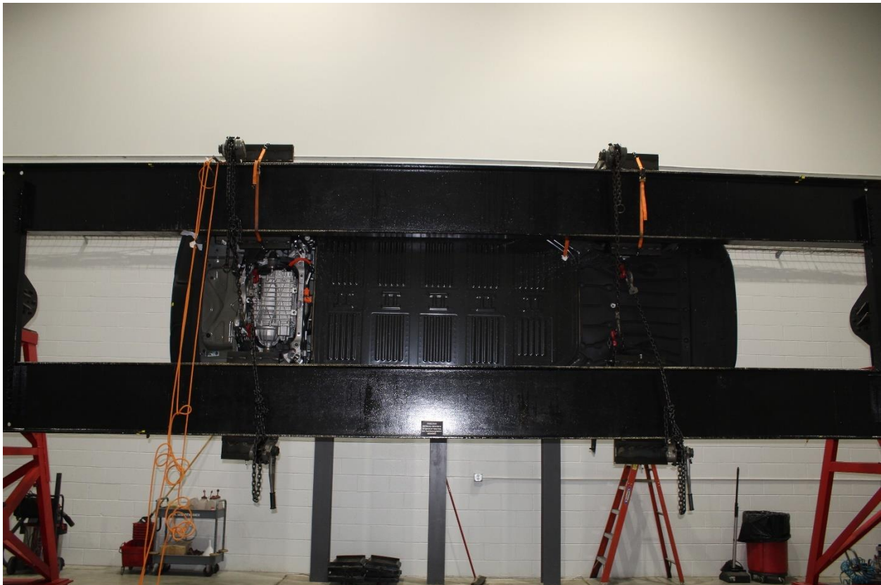
Figure 305-28: FMVSS No. 305 Static Rollover 90 Degrees
