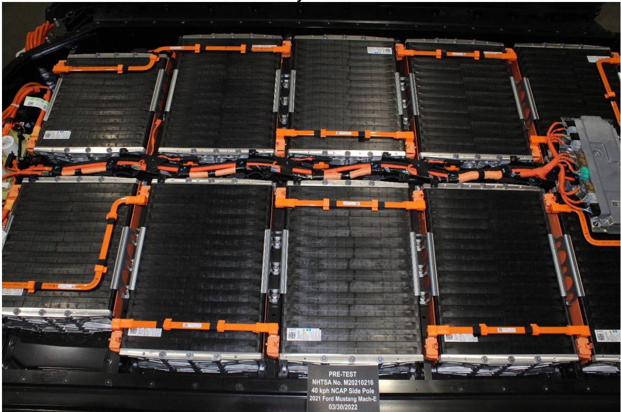
Figure 305-14: Pre-Impact View of Propulsion Battery Module(s)
