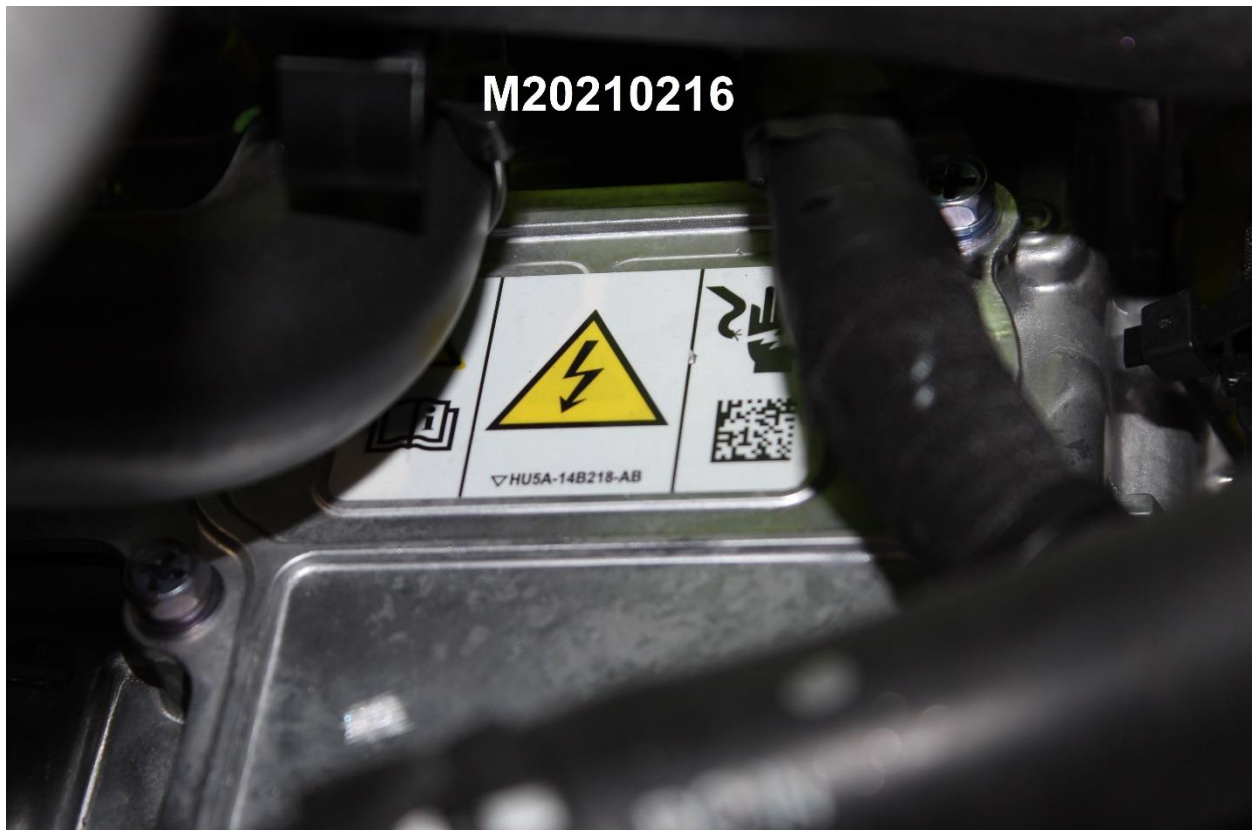
Figure 305-2: Power Inverter Warning Label
