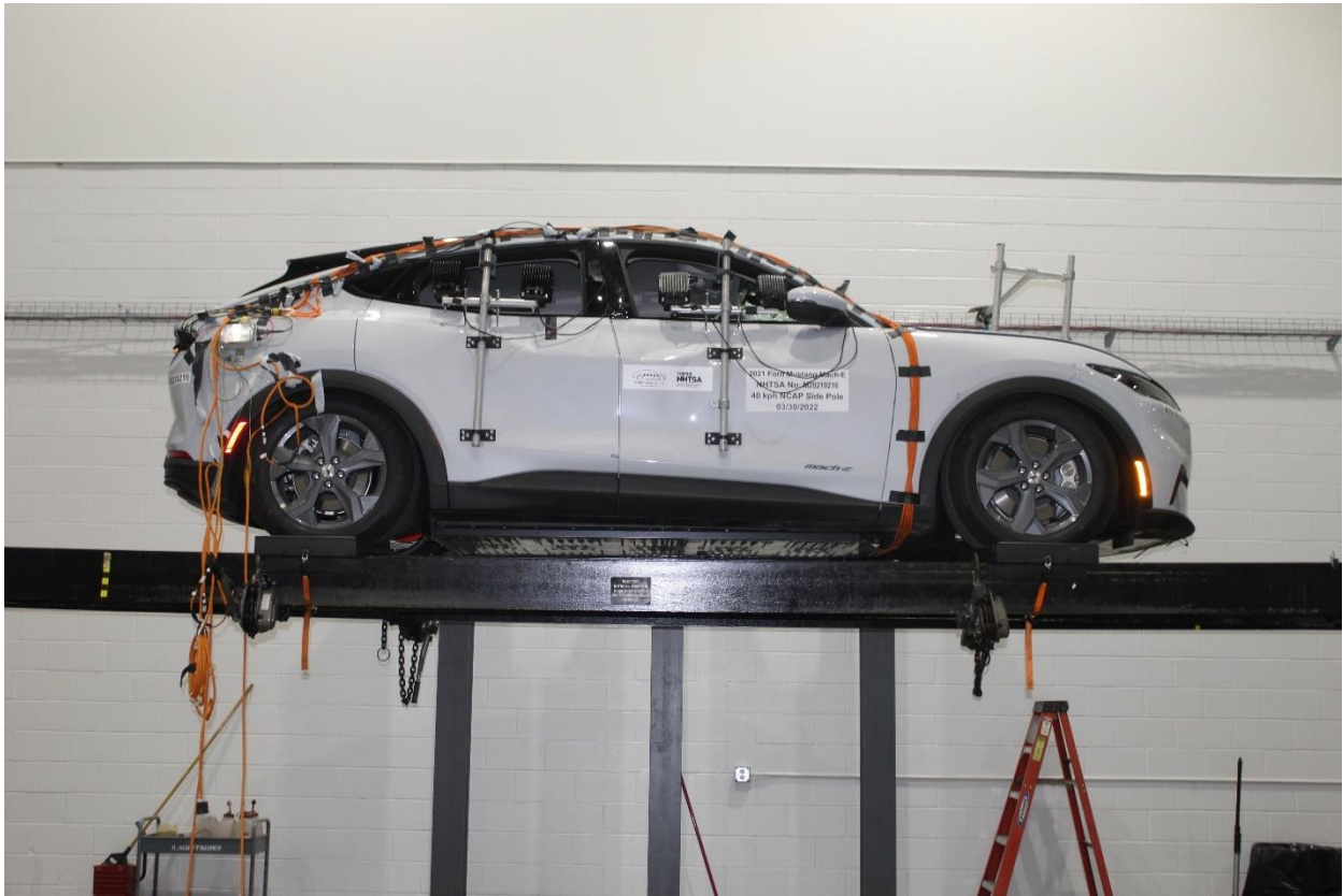
Figure A-65: FMVSS No. 301 Static Rollover 0 Degrees
