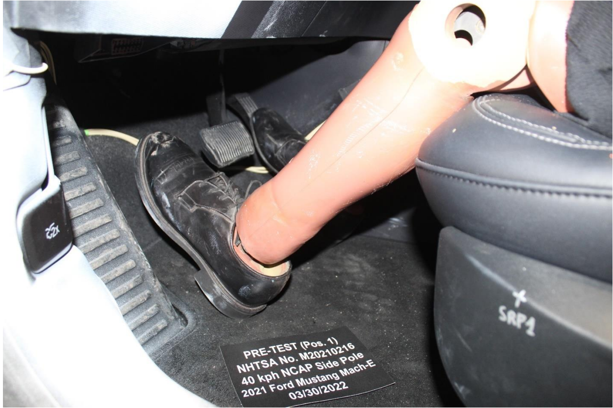
Figure A-32: Pre-Test Placement of Dummy's Feet
