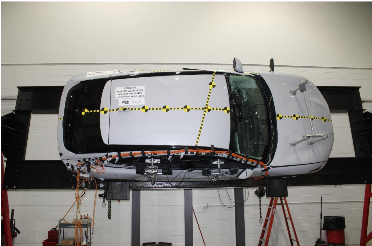
Figure 305-30: FMVSS No. 305 Static Rollover 270 Degrees
