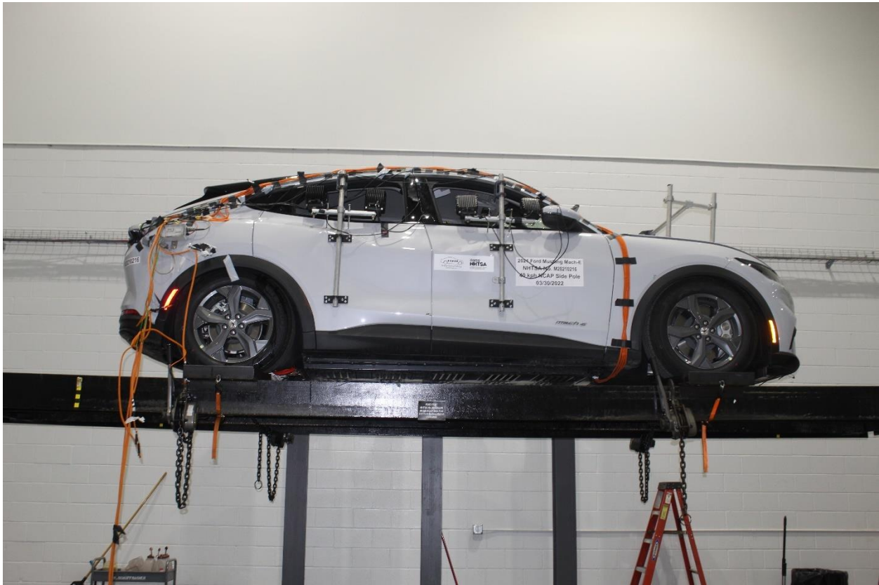
Figure 305-31: FMVSS No. 305 Static Rollover 360 Degrees
